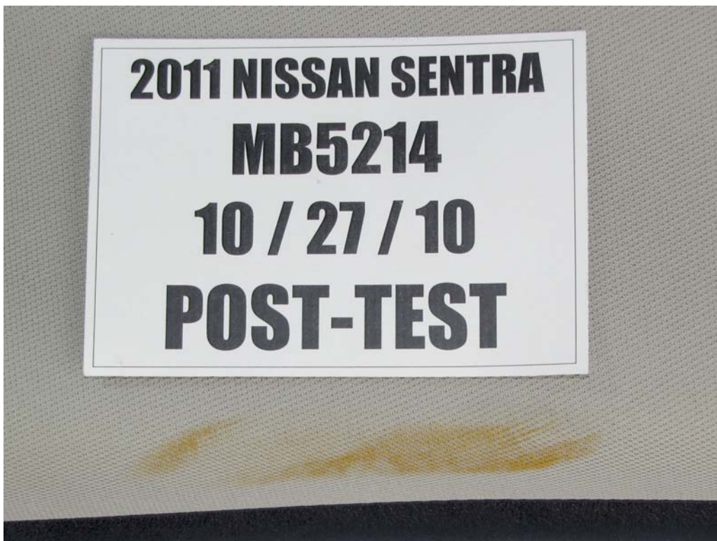
FIGURE 43c. Post-Test Driver Dummy Contact With Side Header
