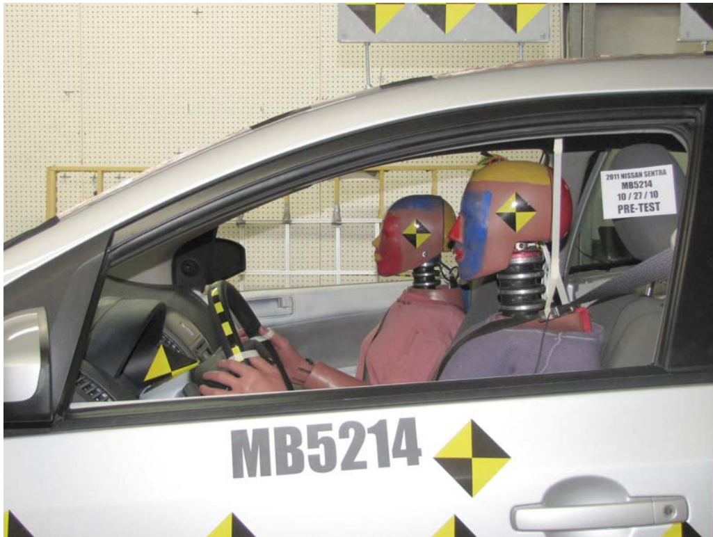
FIGURE 31. Pre-Test Driver Dummy Window View
