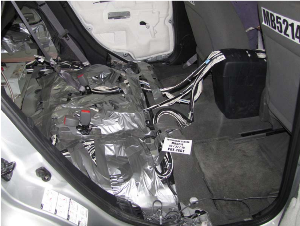
FIGURE 27. Pre-Test Dummy Cable Routing
