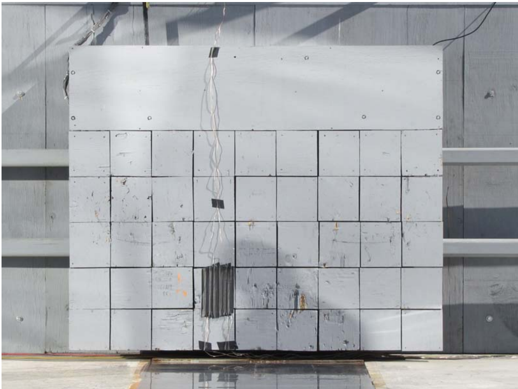
FIGURE 2. Load Cell Wall
