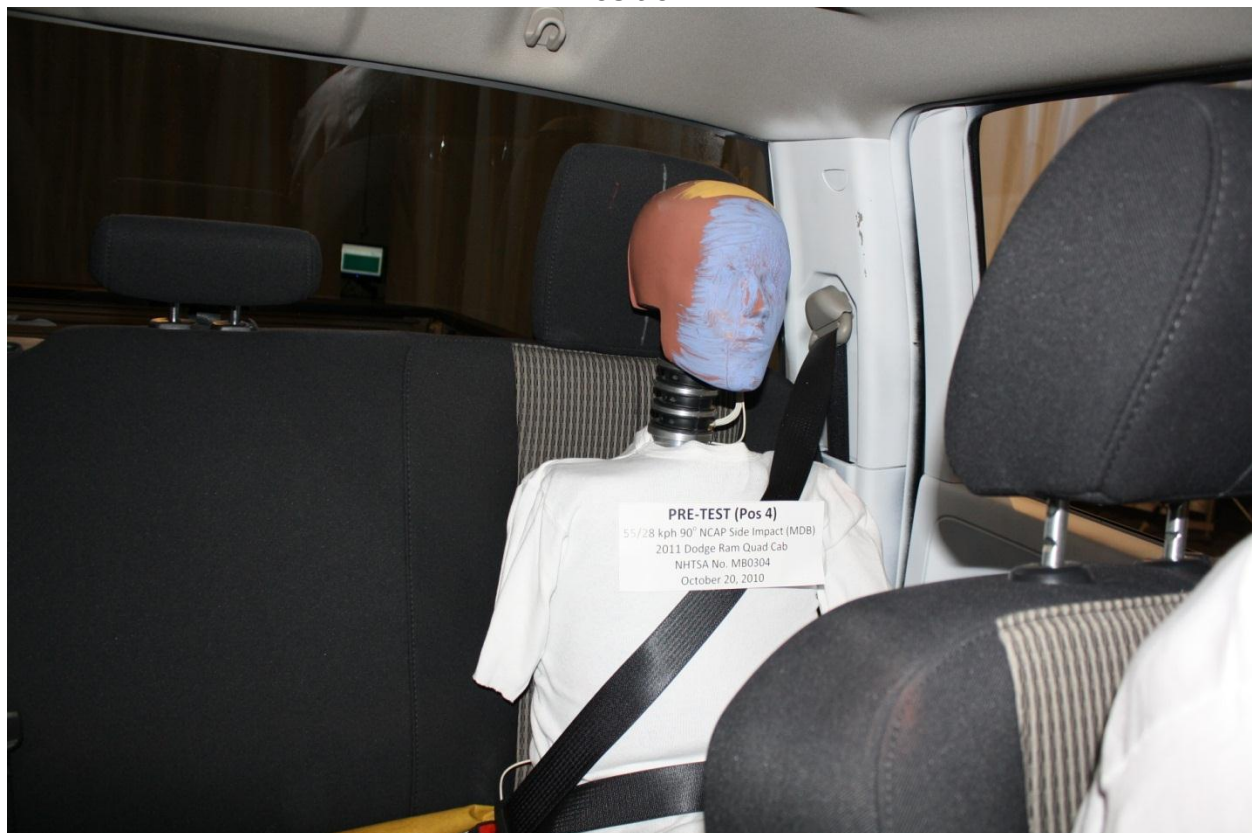
Figure A-66: Pre-Test Close-Up View of Rear Passenger Seat Back or Head Restraint Showing Seat Back Test Position
