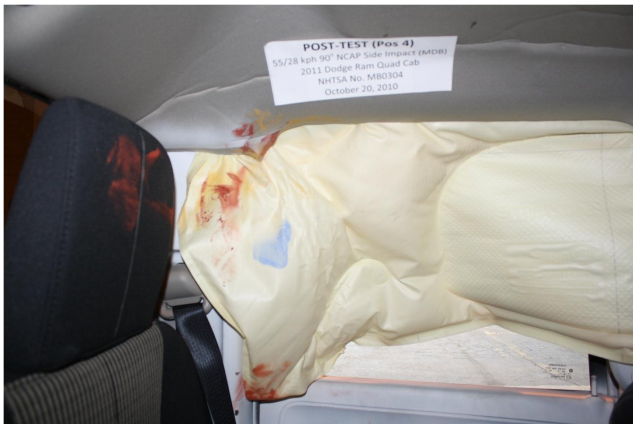
Figure A-73: Post-test Rear Passenger Dummy Close-Up Head Contact with Vehicle View
