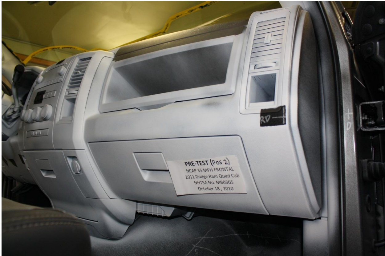
Figure A-57: Post-Test Passenger's Side Knee Bolster
