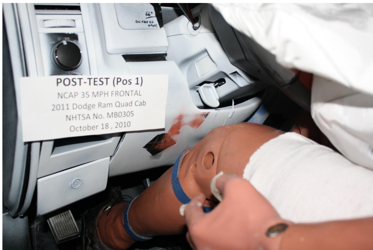
Figure A-40: Post-Test Driver's Side Knee Bolster
