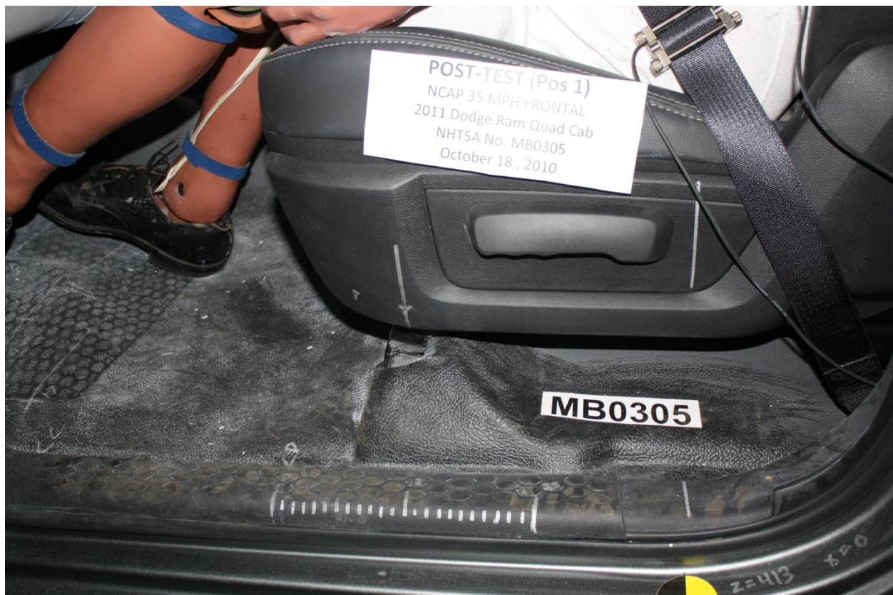
Figure A-36: Post-Test Driver's Seat Fore-Aft Markings
