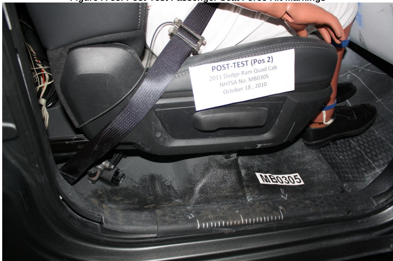
Figure A-53: Post-Test Passenger Seat Force-Aft Markings
