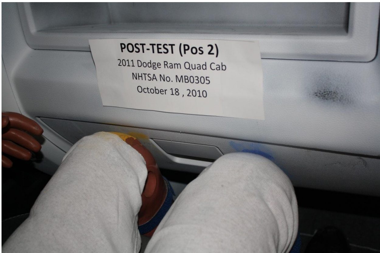
Figure A-57: Post-Test Passenger's Side Knee Bolster
