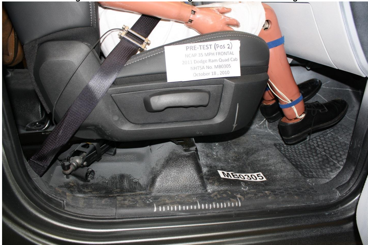
Figure A-52: Pre-Test Passenger Seat Force-Aft Markings
