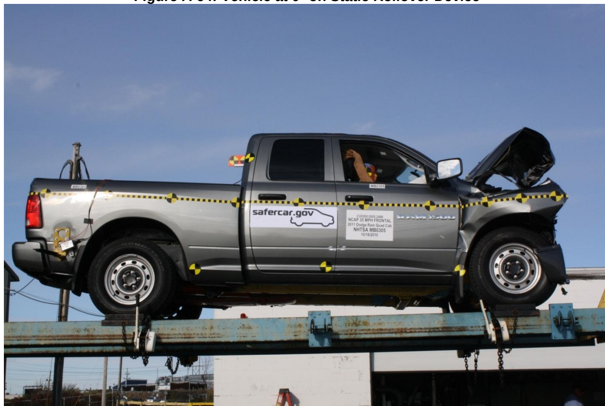
Figure A-64: Vehicle at 0° on Static Rollover Device
