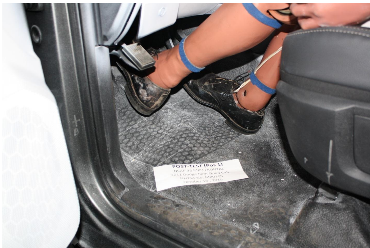
Figure A-38: Post-Test Driver Dummy Feet
