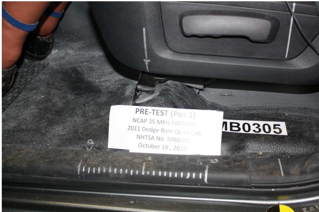
Figure A-36: Post-Test Driver's Seat Fore-Aft Markings
