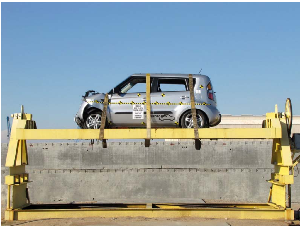
FIGURE 68. Vehicle at 360 Degrees on Static Rollover Device
