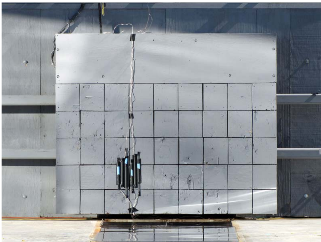
FIGURE 2. Load Cell Wall
