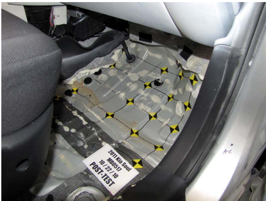
FIGURE 59. Post-Test Passenger's Side Floorpan
