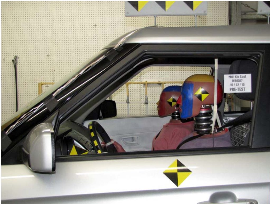
FIGURE 31. Pre-Test Driver Dummy Window View
