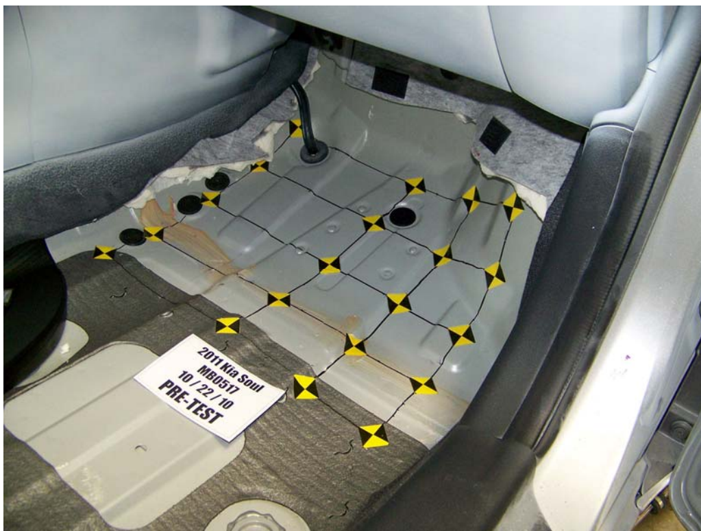
FIGURE 58. Pre-Test Passenger's Side Floorpan
