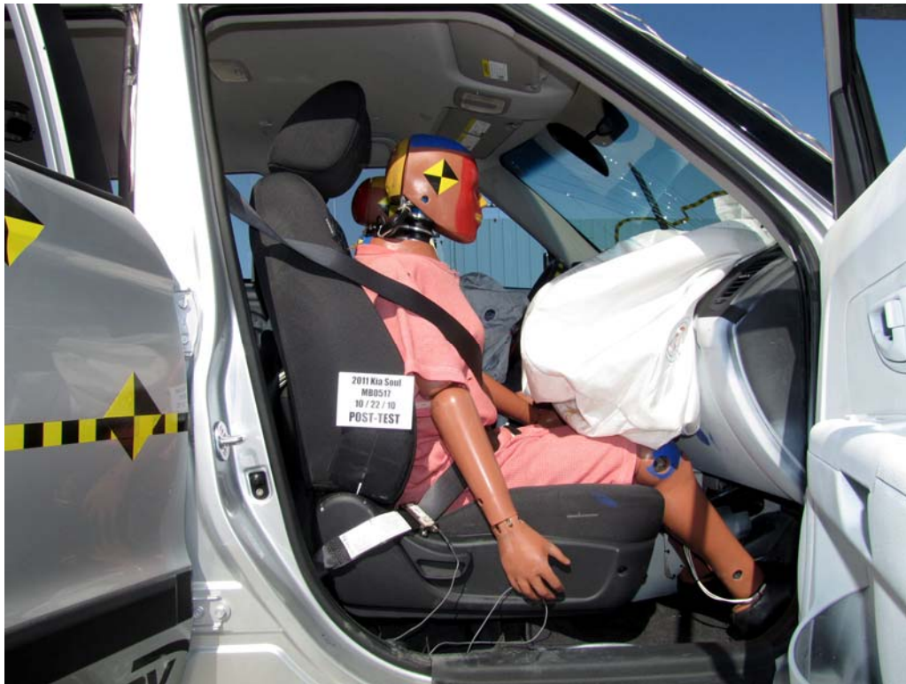
FIGURE 51. Post-Test Passenger Dummy and Vehicle Interior View
