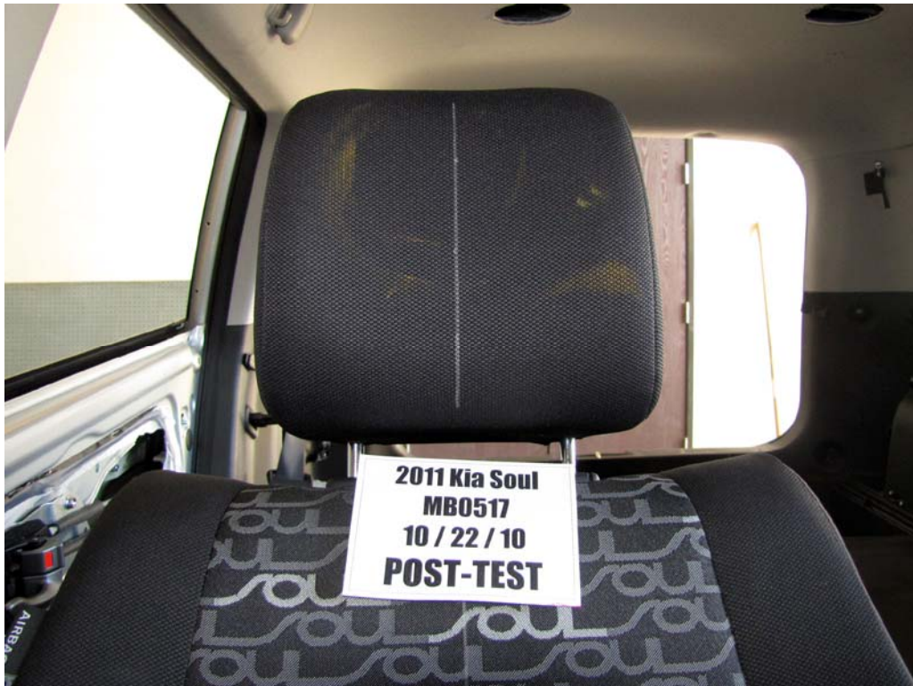
FIGURE 60a. Post-Test Passenger Dummy Contact With Headrest
