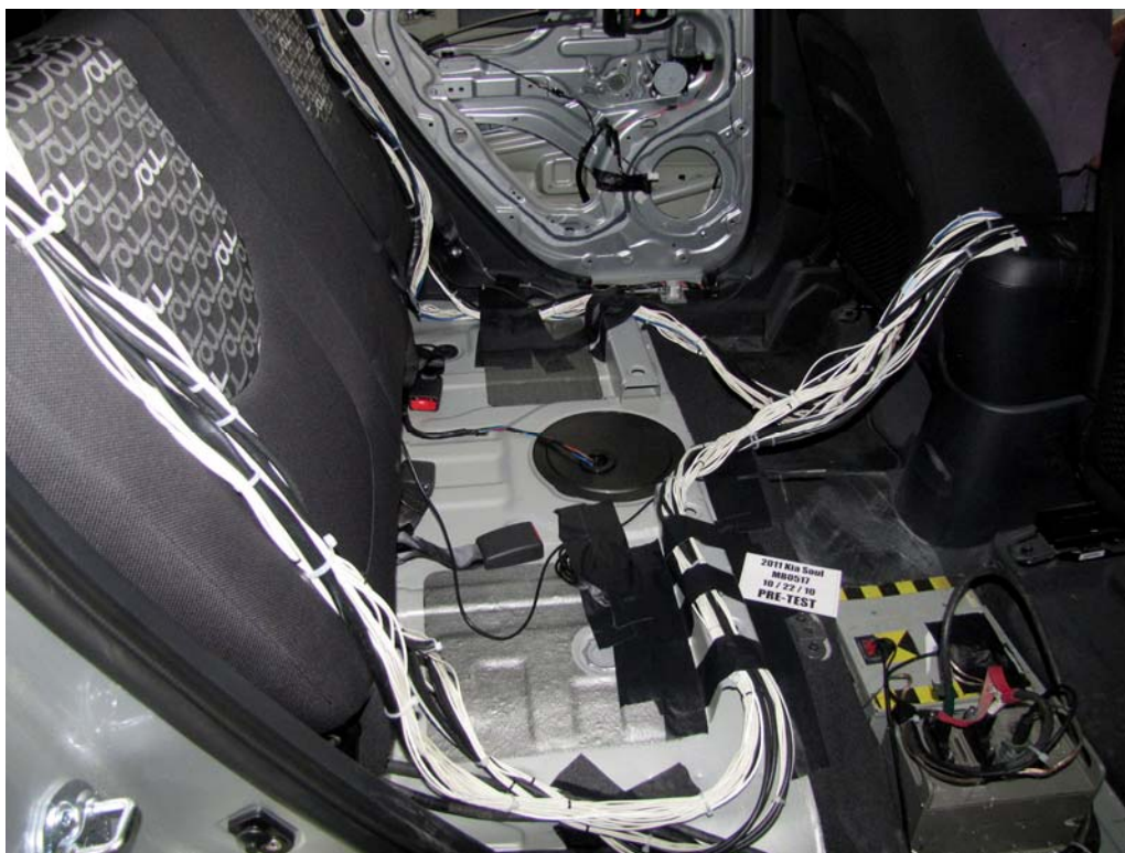
FIGURE 27. Pre-Test Dummy Cable Routing
