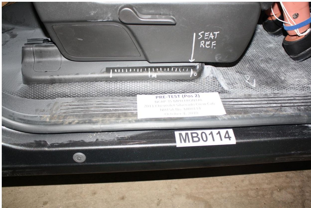
Figure A-52: Pre-Test Passenger's Seat Fore-Aft Markings
