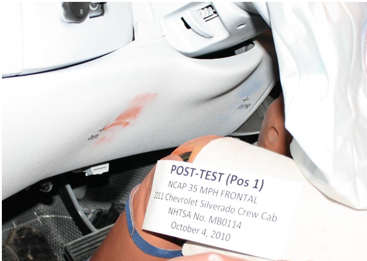
Figure A-40: Post-Test Driver's Side Knee Bolster
