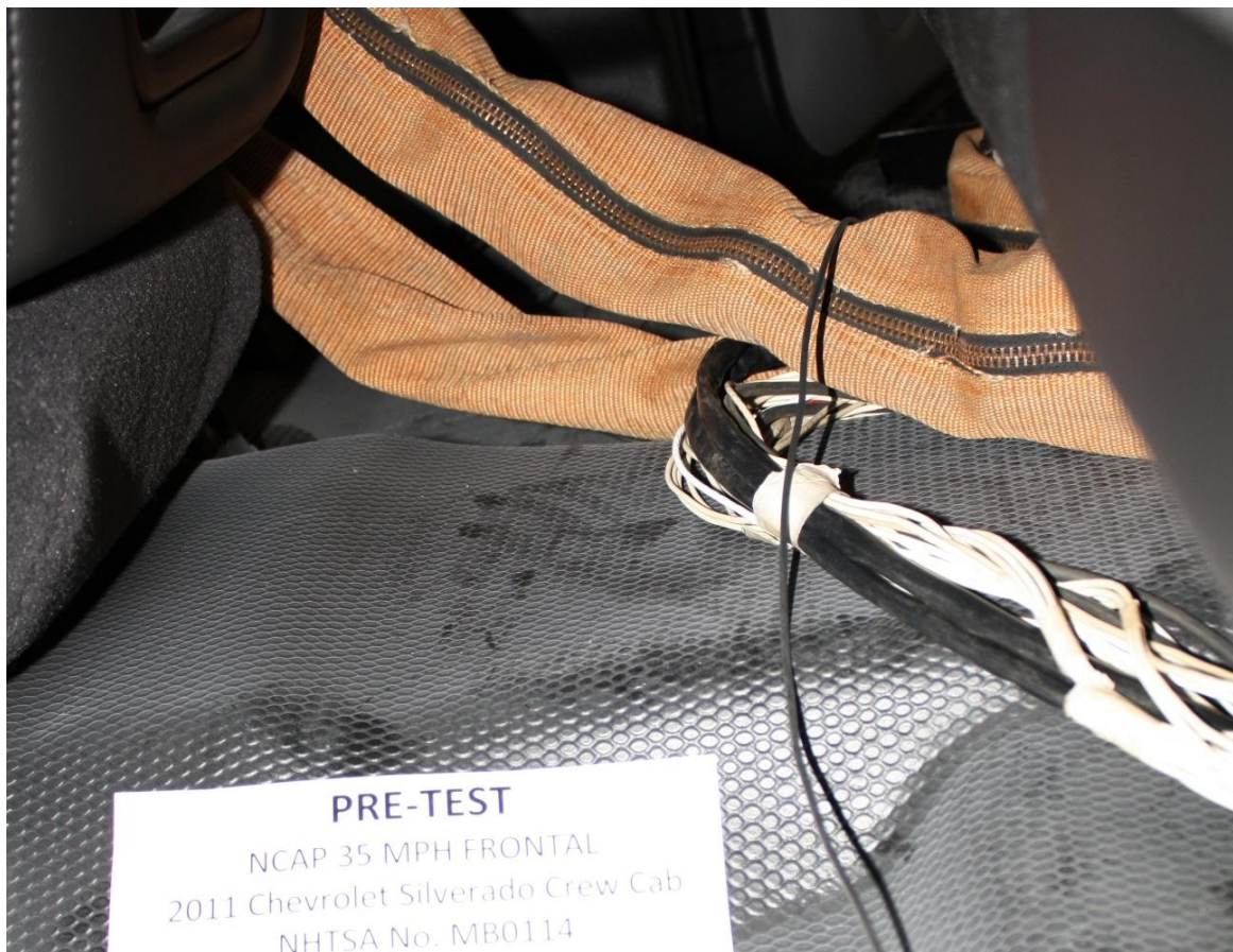
Figure A-27: Pre-Test Dummy Cable Routing
