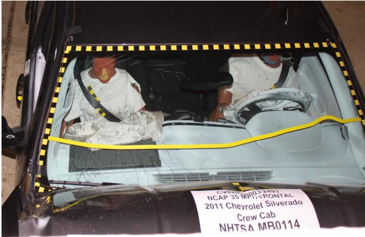
Figure A-18: Post-Test Windshield View
