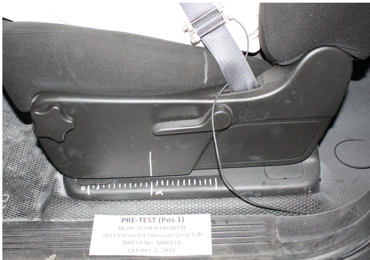
Figure A-35: Pre-Test Driver's Seat Fore-Aft Markings
