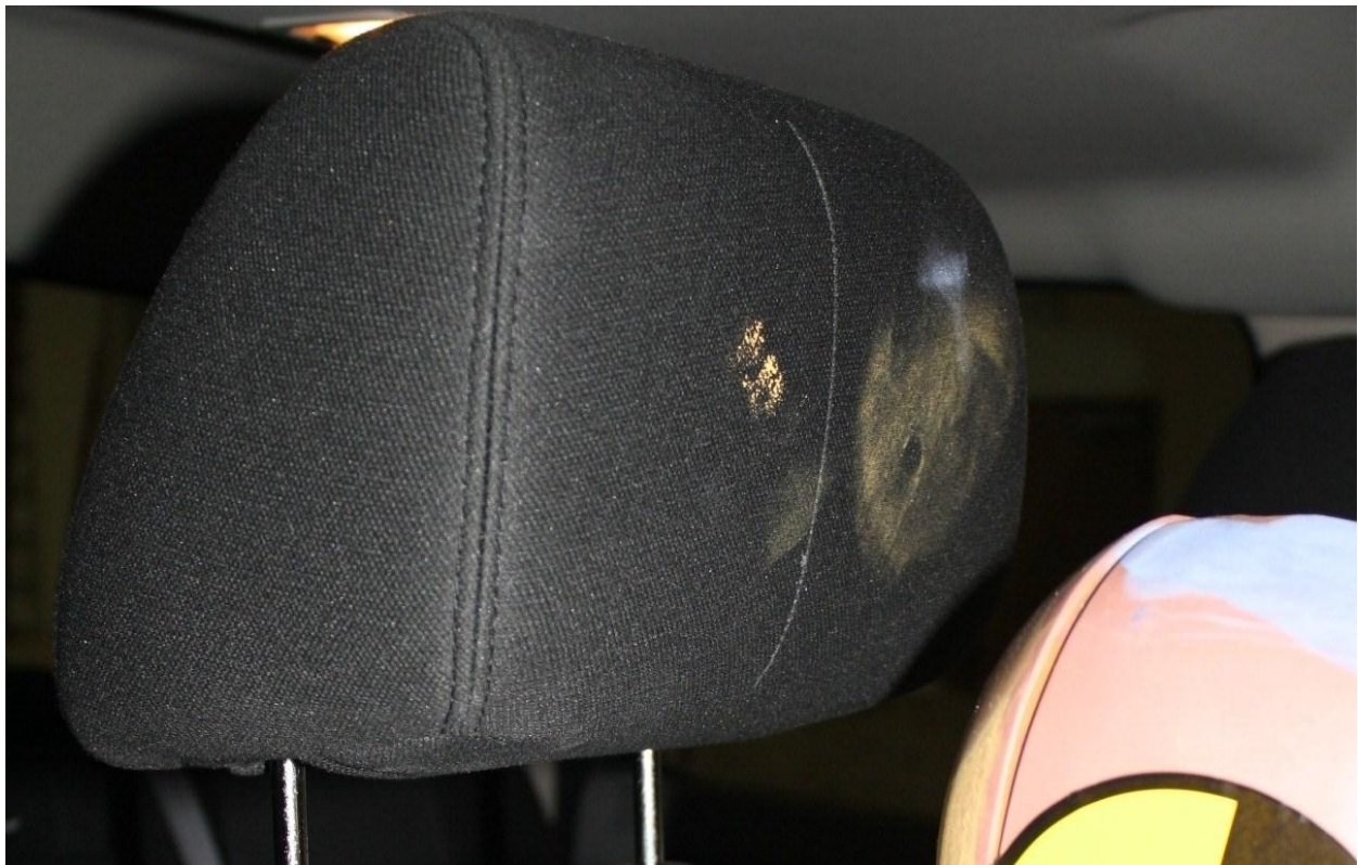
Figure A-60b: Post-Test Passenger Dummy Contact with Head Restraint
