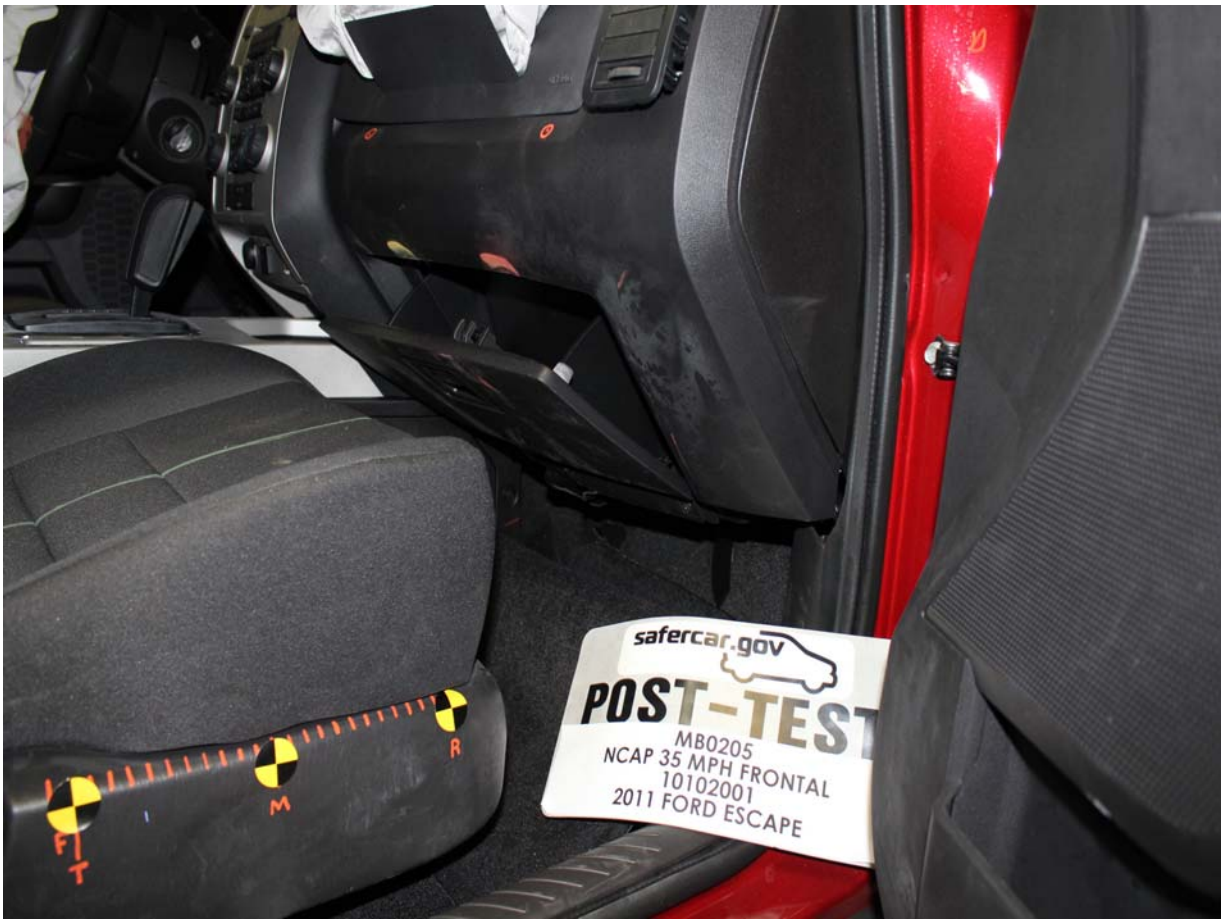
Post-Test Passenger Dummy Contact with Glovebox
