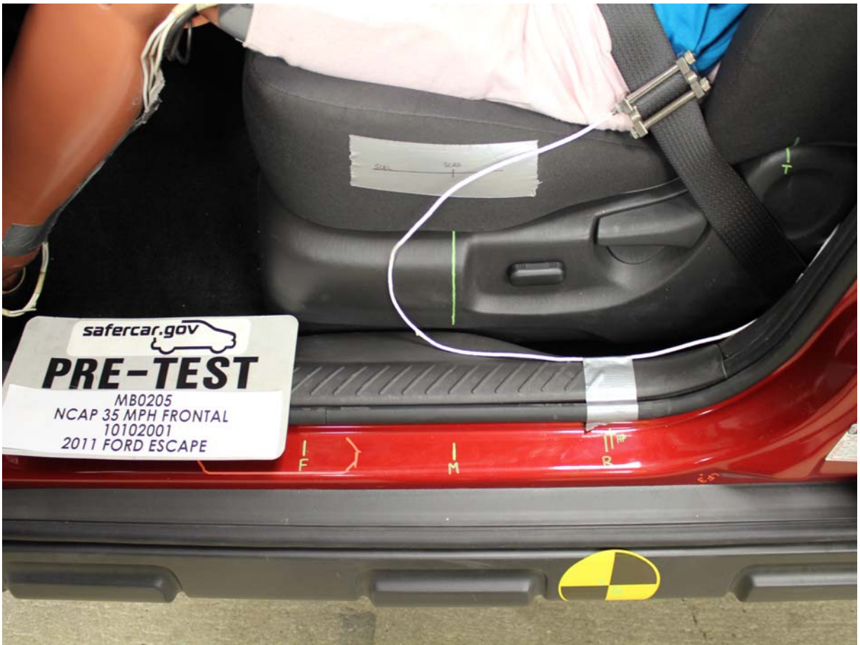
Pre-Test Driver's Seat Fore-Aft Markings
