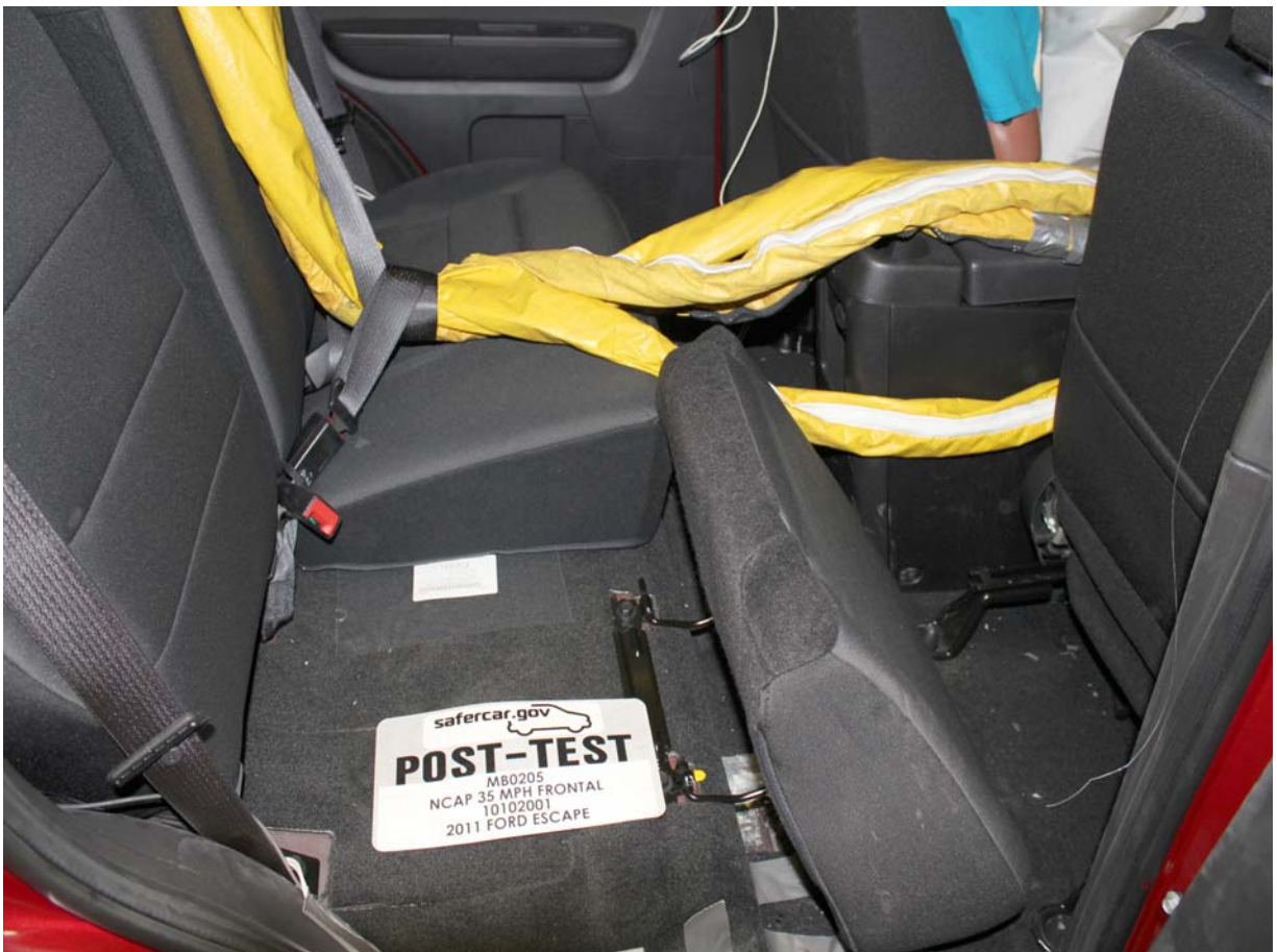
Post-Test Dummy Cable Routing
