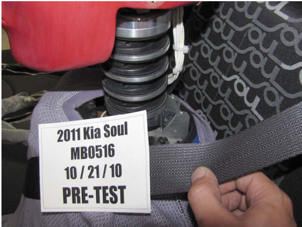
FIGURE 60. Pre-Test View of Rear Passenger Dummy's Neck Showing Position of Adjustable Neck Bracket
