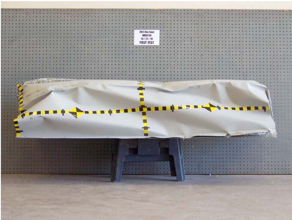
FIGURE 84. Post-Test Top View of MDB Impactor Face
