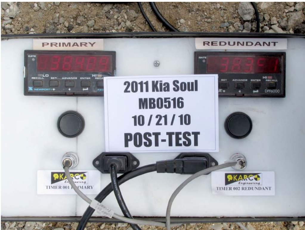
FIGURE 92. Post-Test Primary and Redundant Speed Trap Read-Out
