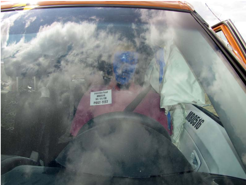
FIGURE 26. Post-Test Front Close-Up View of Driver Dummy
