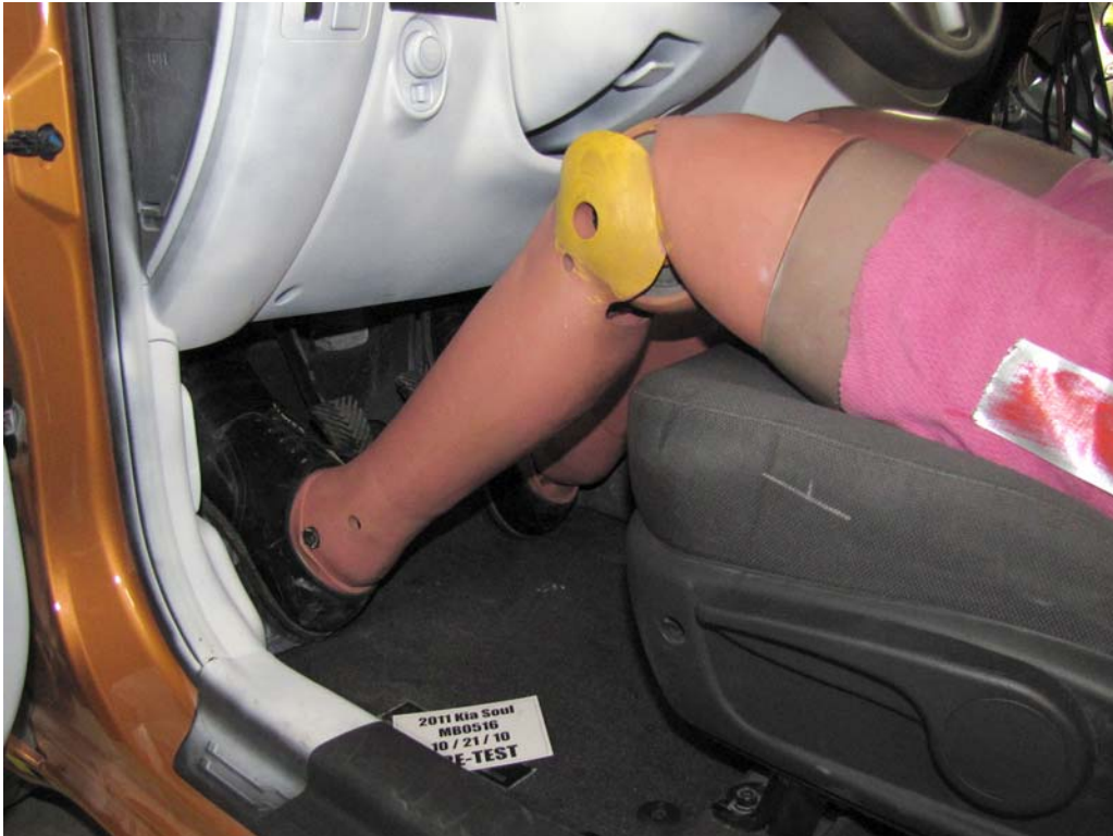
FIGURE 34. Pre-Test Placement of Driver Dummy's Feet
