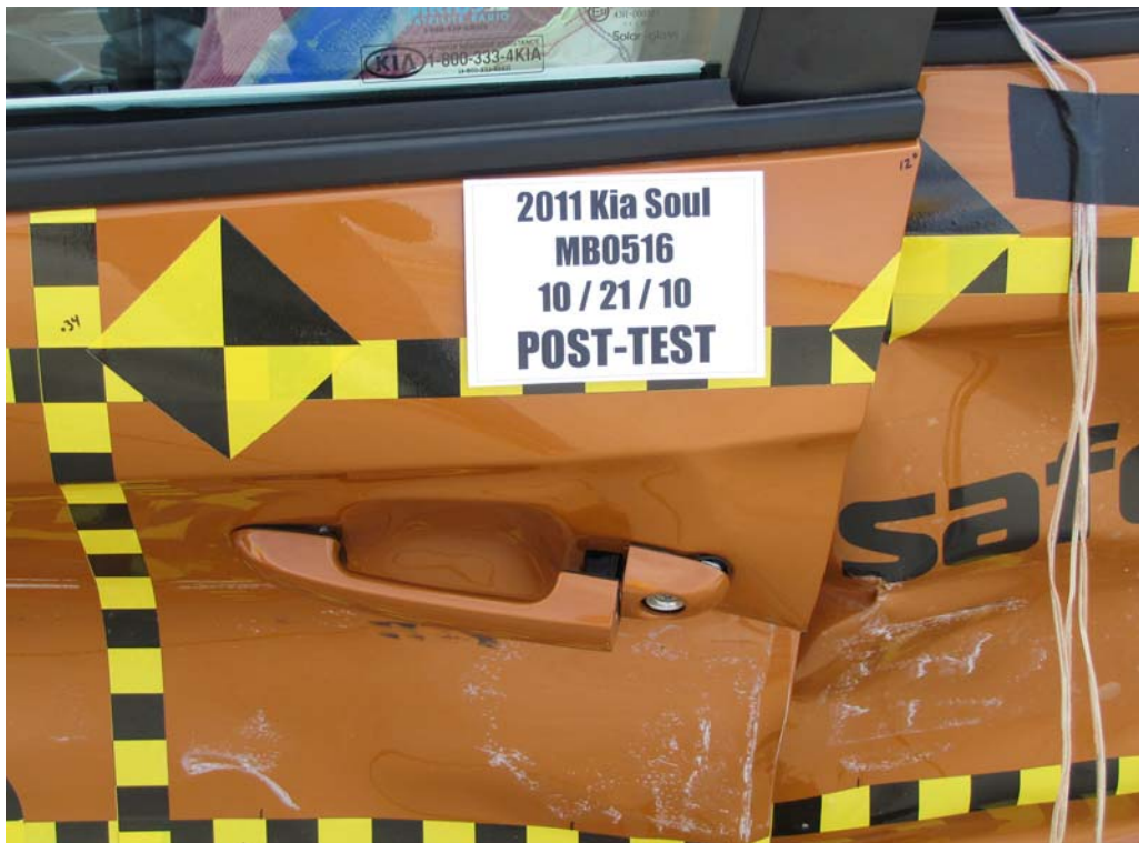
FIGURE 22. Post-Test Left Front Door Latch Close-Up
