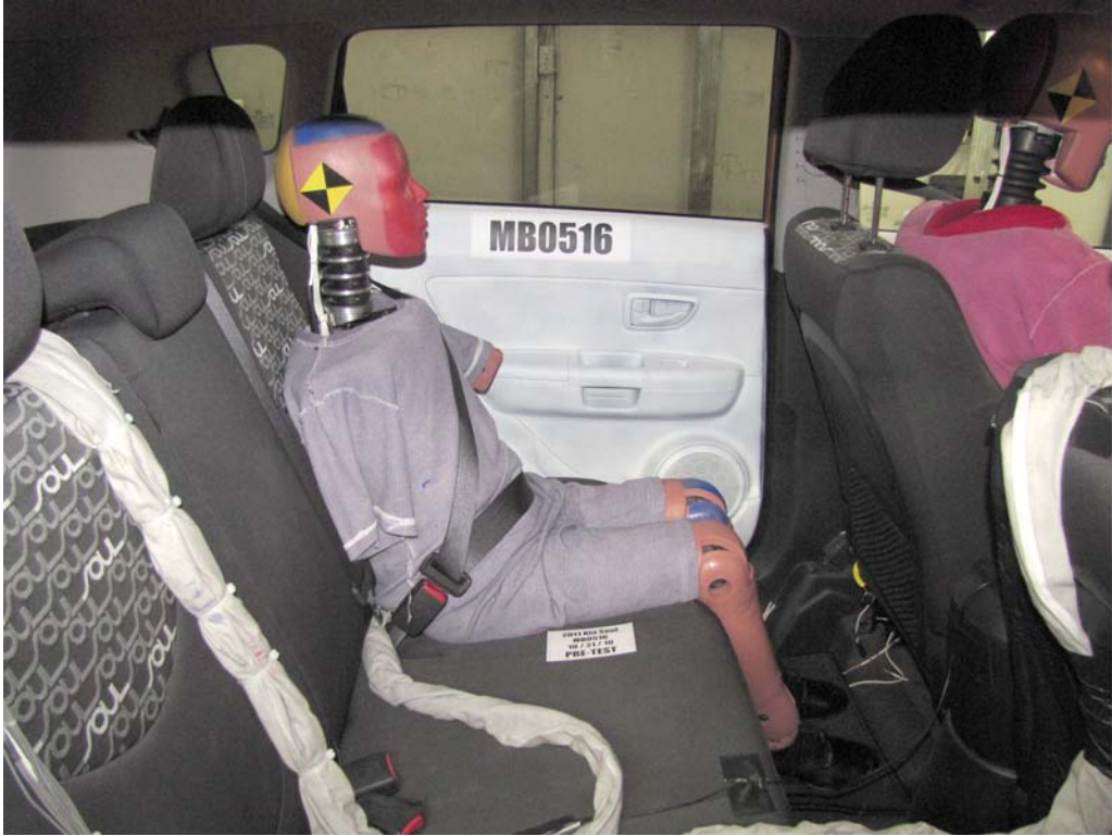
FIGURE 69. Pre-Test Right Side View of Rear Passenger Dummy and Rear Seat Occupant Compartment
