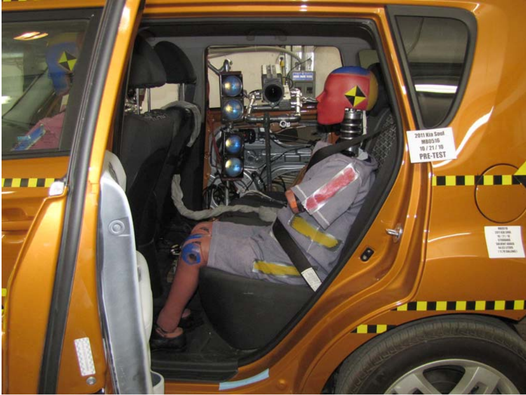
FIGURE 53. Pre-Test Left Side View of Rear Passenger Dummy Showing Belt, Chalking, and Contact Switches
