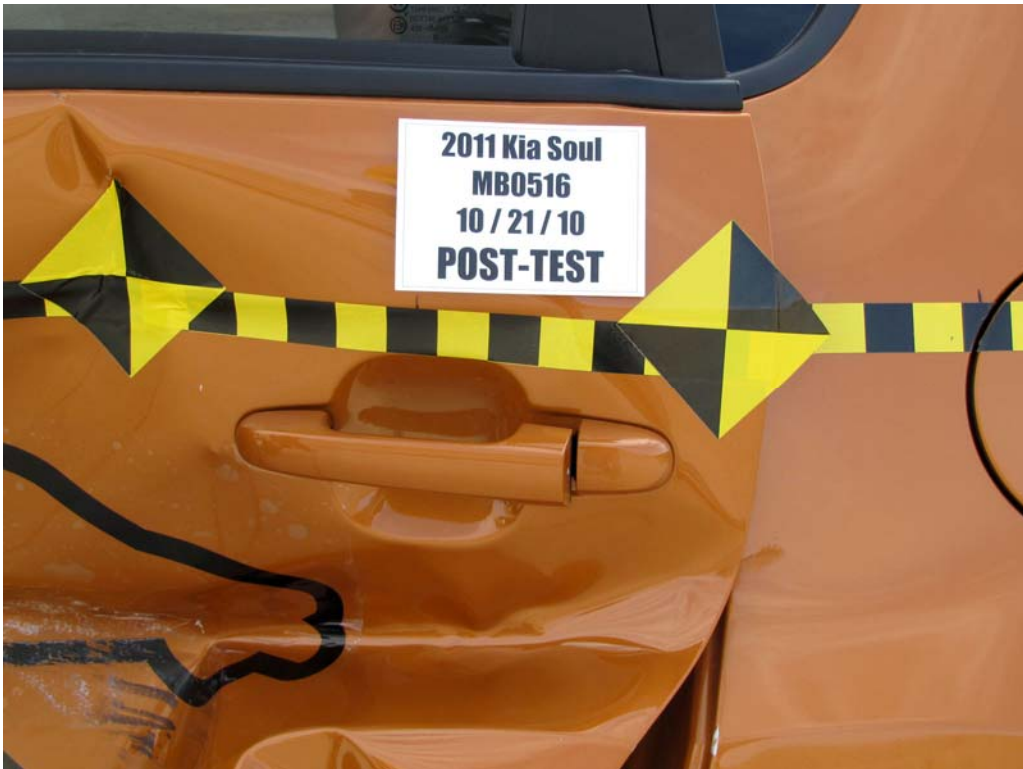
FIGURE 24. Post-Test Left Rear Door Latch Close-Up
