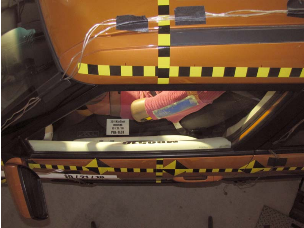
FIGURE 41. Pre-Test Driver Dummy and Door Clearance View
