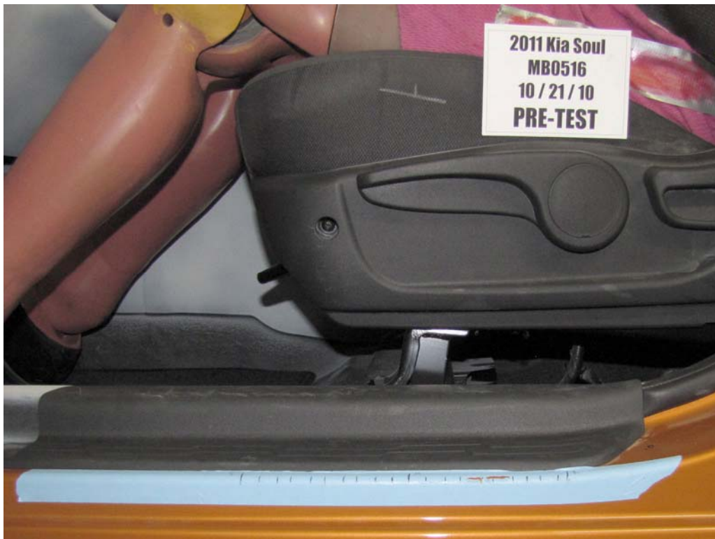
FIGURE 38. Pre-Test Close-Up Left Side View of Driver Seat Track
