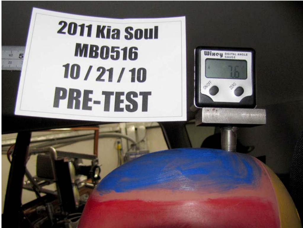
FIGURE 61. Pre-Test View of Rear Passenger Dummy's Head Showing Dummy's Head is Level
