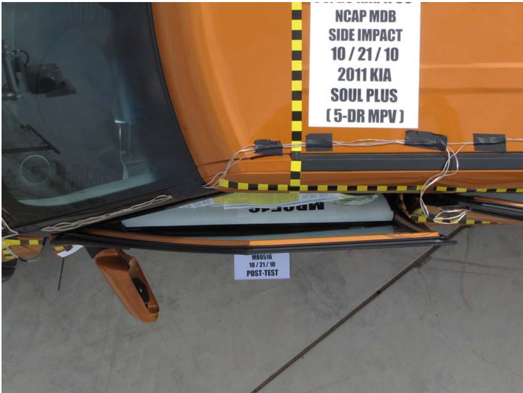
FIGURE 42. Post-Test Driver Dummy and Door Clearance View
