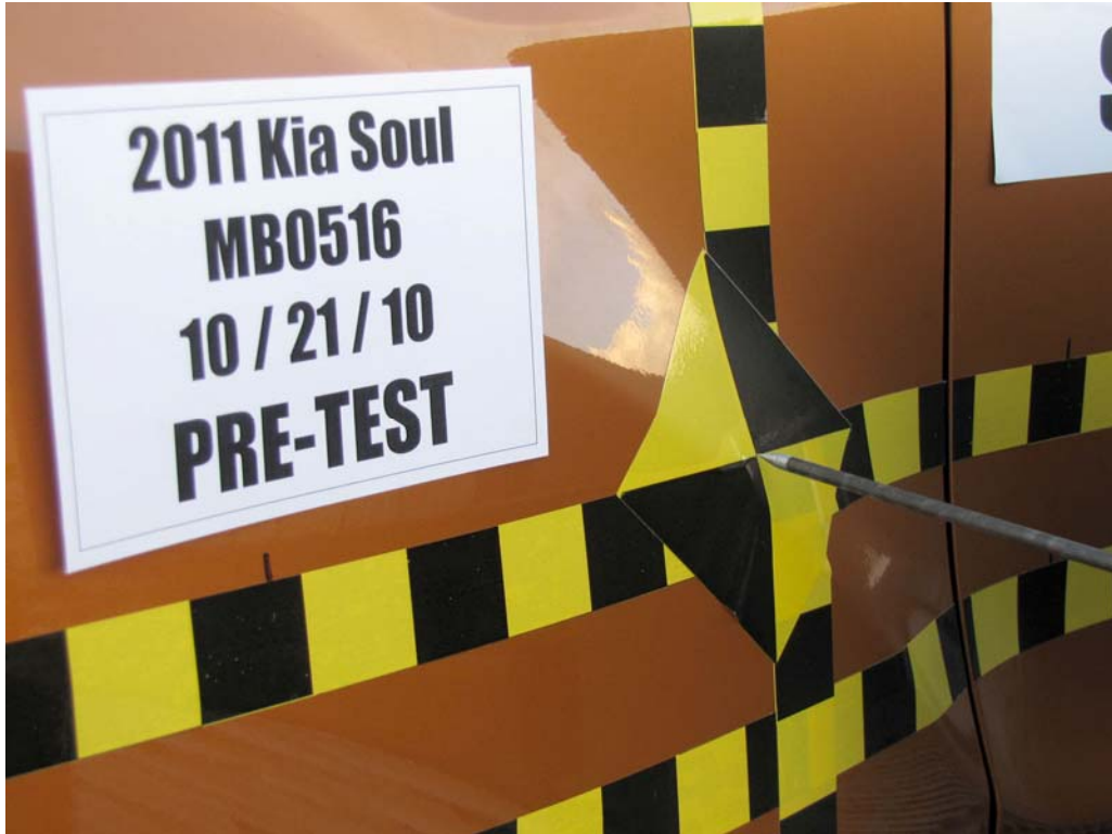
FIGURE 19. Pre-Test Close-Up View of Impact Point Target
