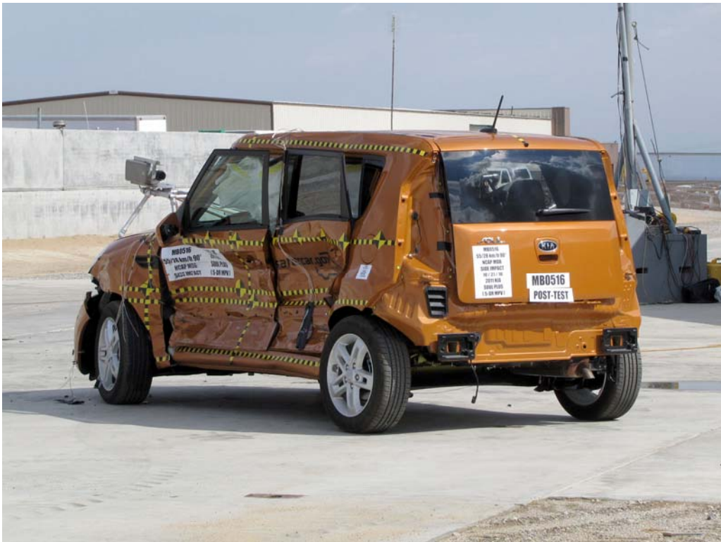
FIGURE 10. Post-Test Left Rear Three-Quarter View of Impact Zone
