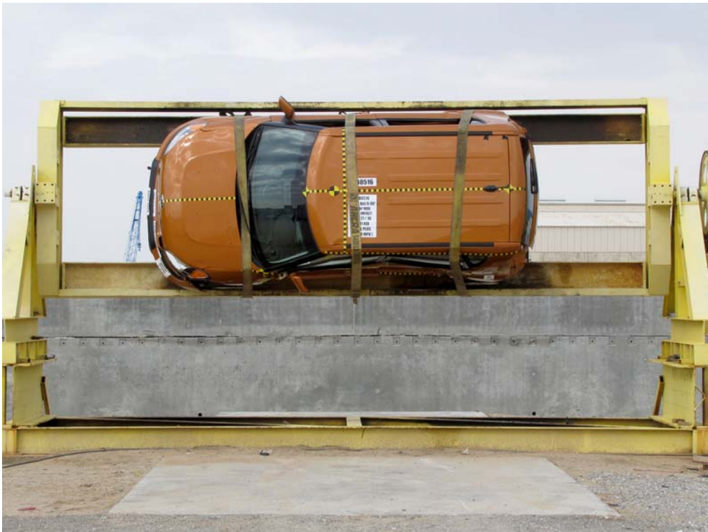
FIGURE 94. FMVSS No. 301/305 Rollover 90 Degrees
