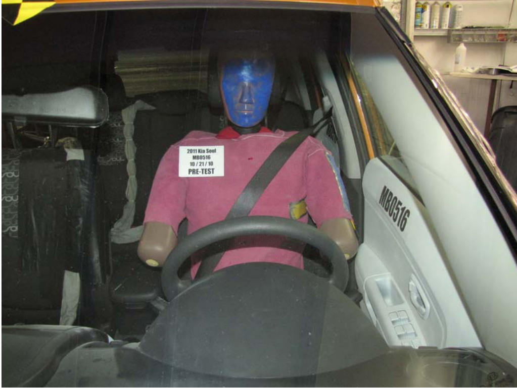
FIGURE 25. Pre-Test Front Close-Up View of Driver Dummy
