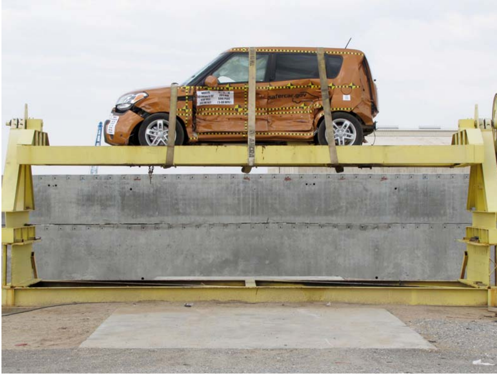
FIGURE 97. FMVSS No. 301/305 Rollover 360 Degrees
