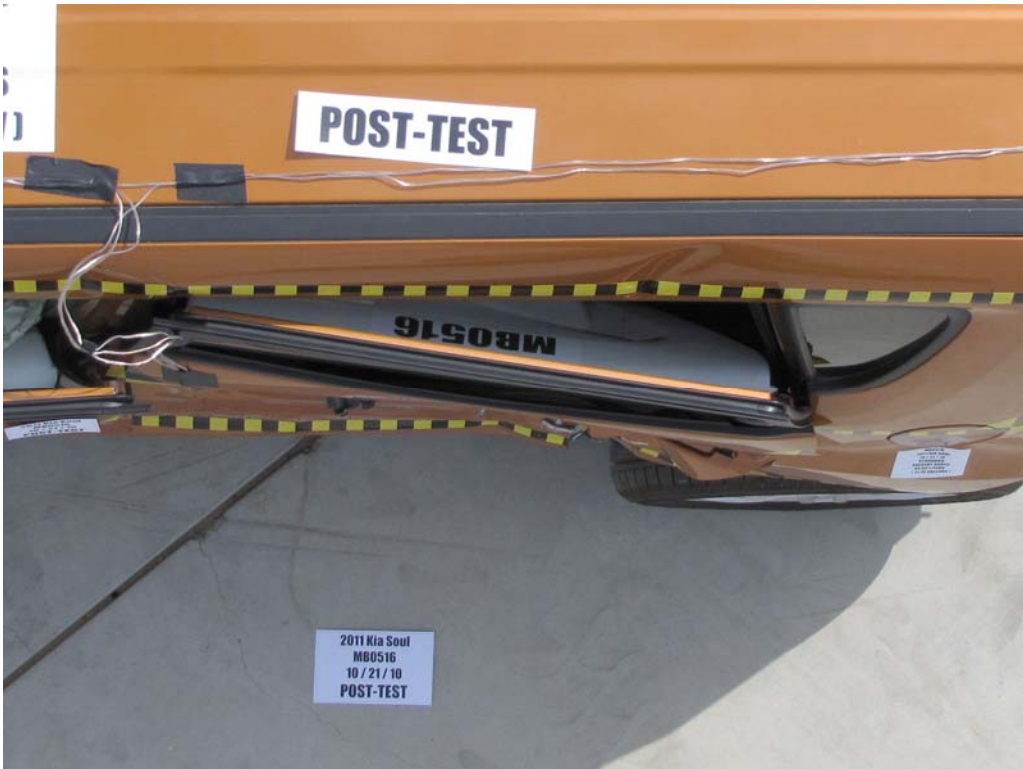
FIGURE 68. Post-Test Rear Passenger Dummy and Door Clearance View
