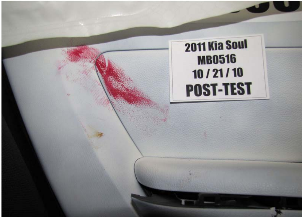
FIGURE 77. Post-Test Rear Passenger Dummy Close-Up Pelvis Contact with Vehicle Interior View
