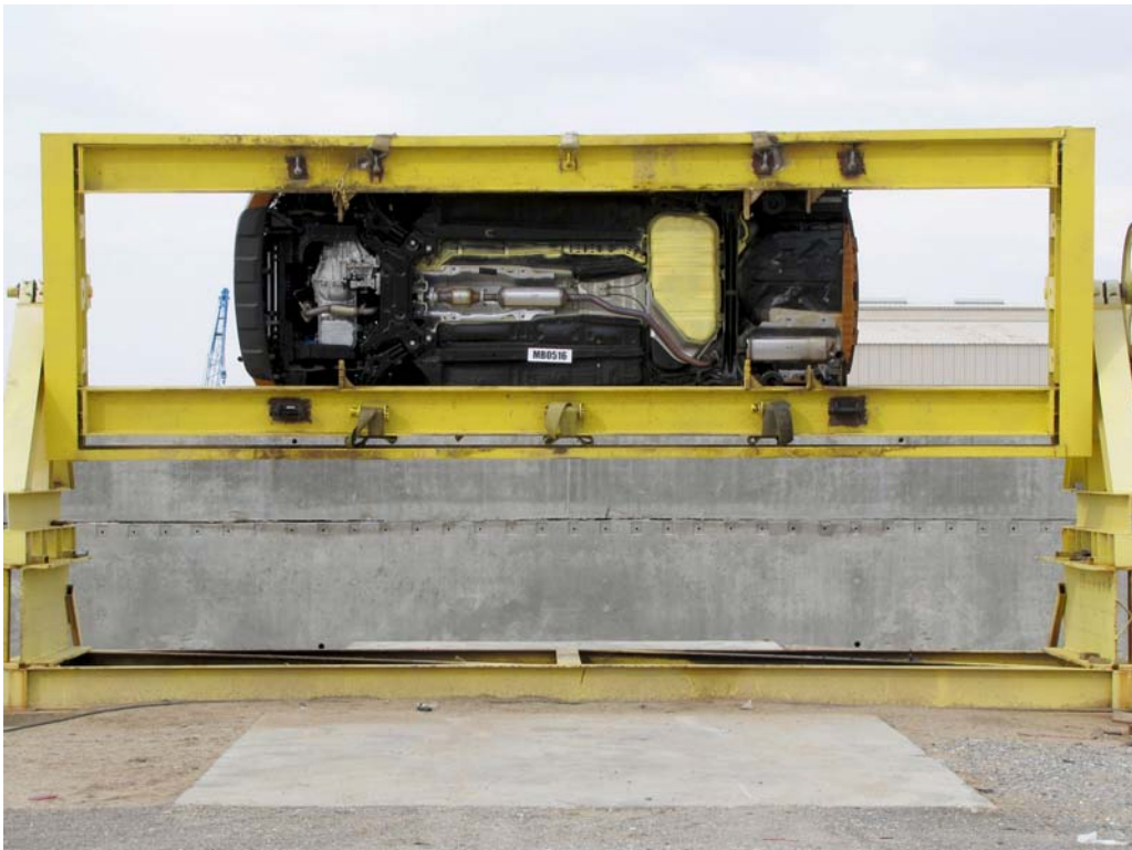
FIGURE 96. FMVSS No. 301/305 Rollover 270 Degrees
