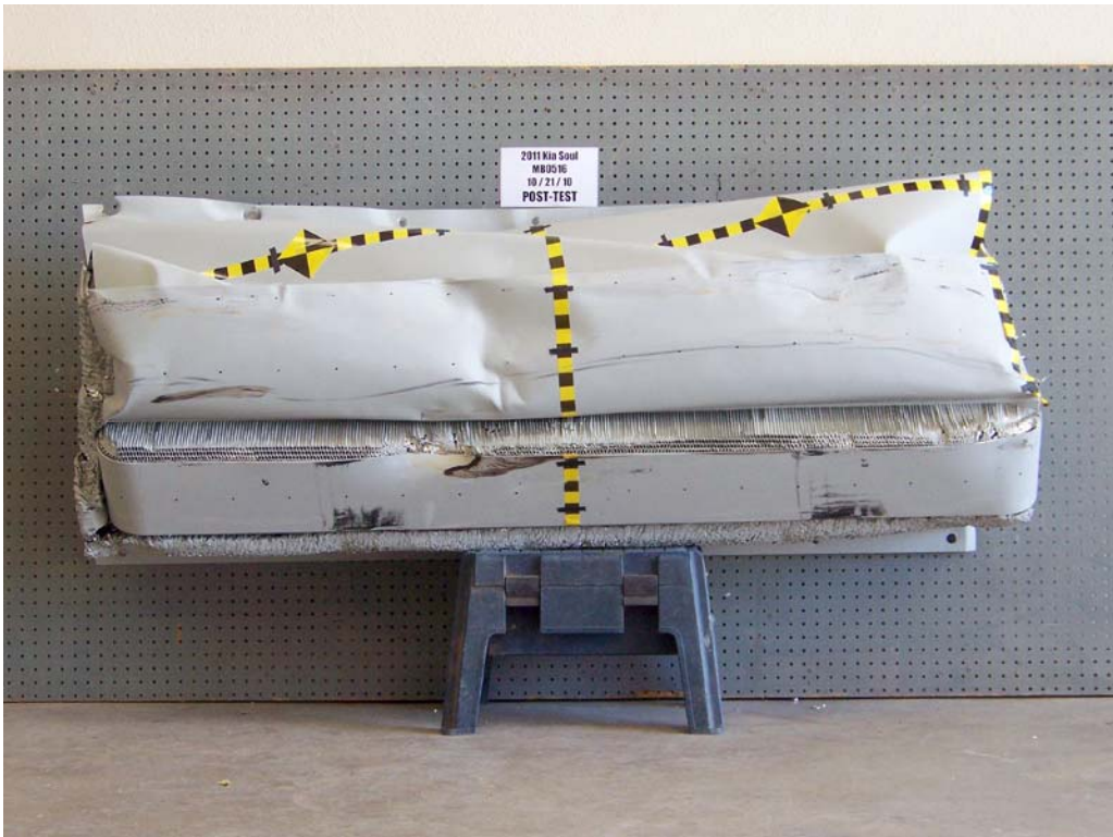
FIGURE 82. Post-Test Front View of MDB Impactor Face
