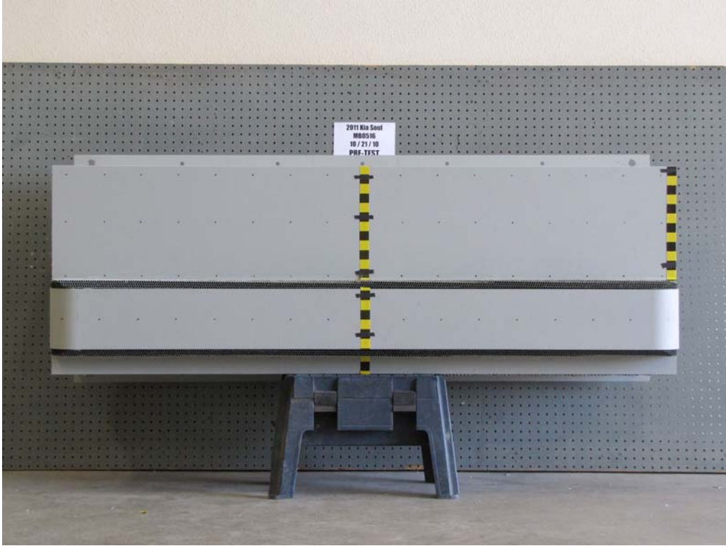
FIGURE 81. Pre-Test Front View of MDB Impactor Face
