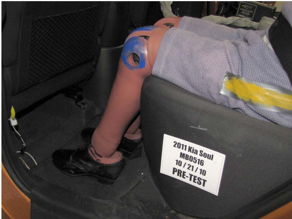
FIGURE 62. Pre-Test Placement of Rear Passenger Dummy's Feet
