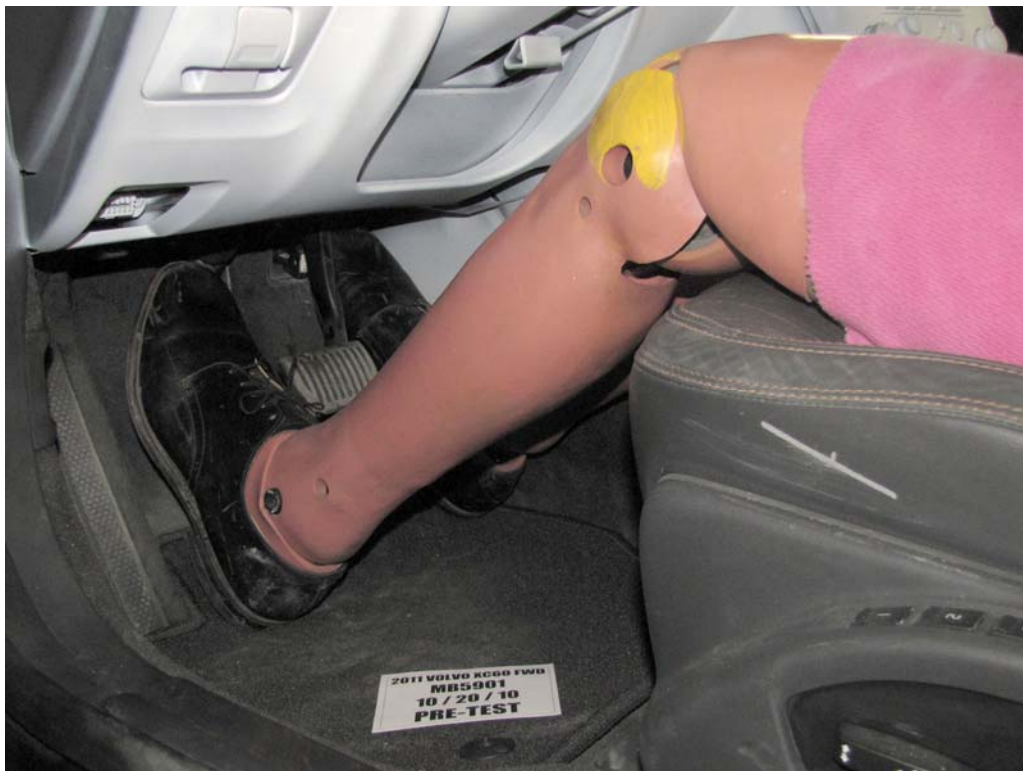
FIGURE 34. Pre-Test Placement of Driver Dummy's Feet
