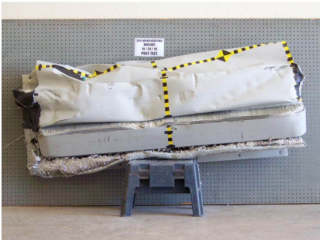
FIGURE 82. Post-Test Front View of MDB Impactor Face
