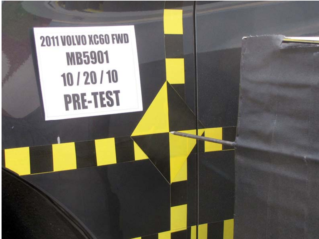
FIGURE 19. Pre-Test Close-Up View of Impact Point Target
