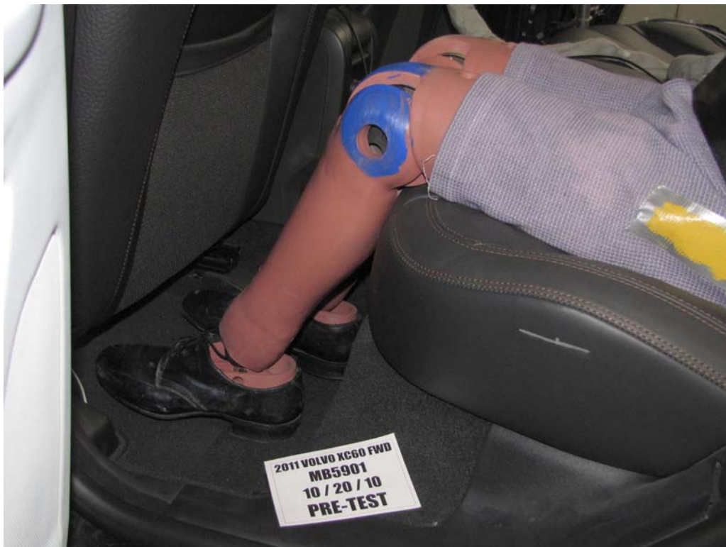
FIGURE 62. Pre-Test Placement of Rear Passenger Dummy's Feet
