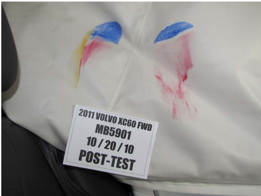
FIGURE 74. Post-Test Rear Passenger Dummy Close-Up Head Contact With Side Airbag View
