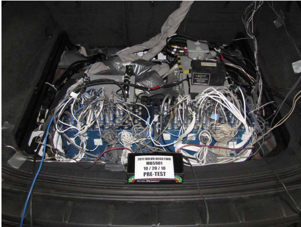
FIGURE 91. Pre-Test Ballast View
