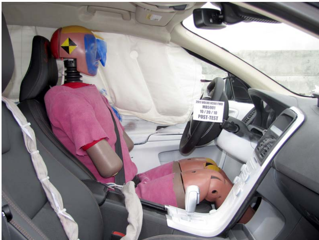
FIGURE 44. Post-Test Right Side View of Driver Dummy and Front Seat Occupant Compartment
