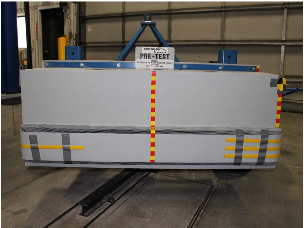
Pre-Test Front View of MDB Impactor Face
