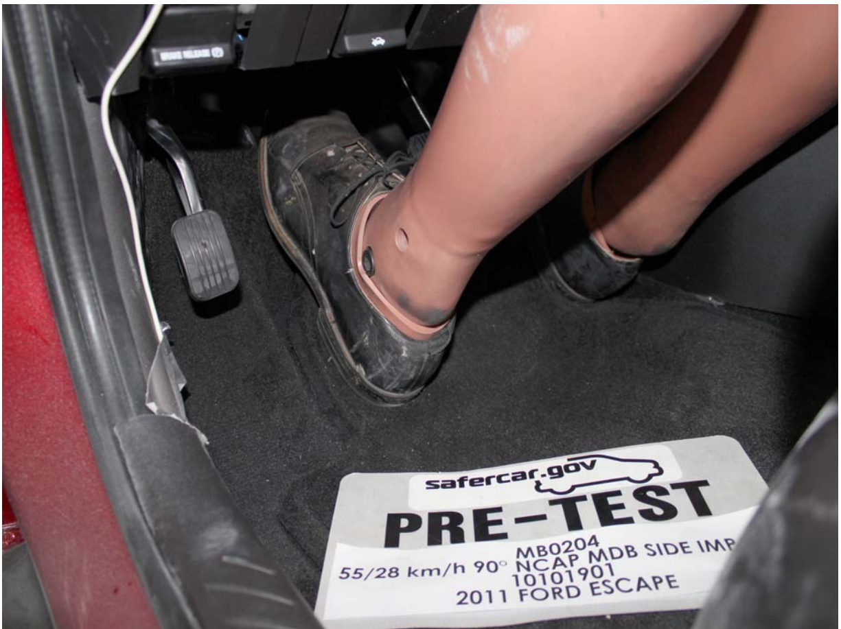
Pre-Test Placement of Driver Dummy's Feet
