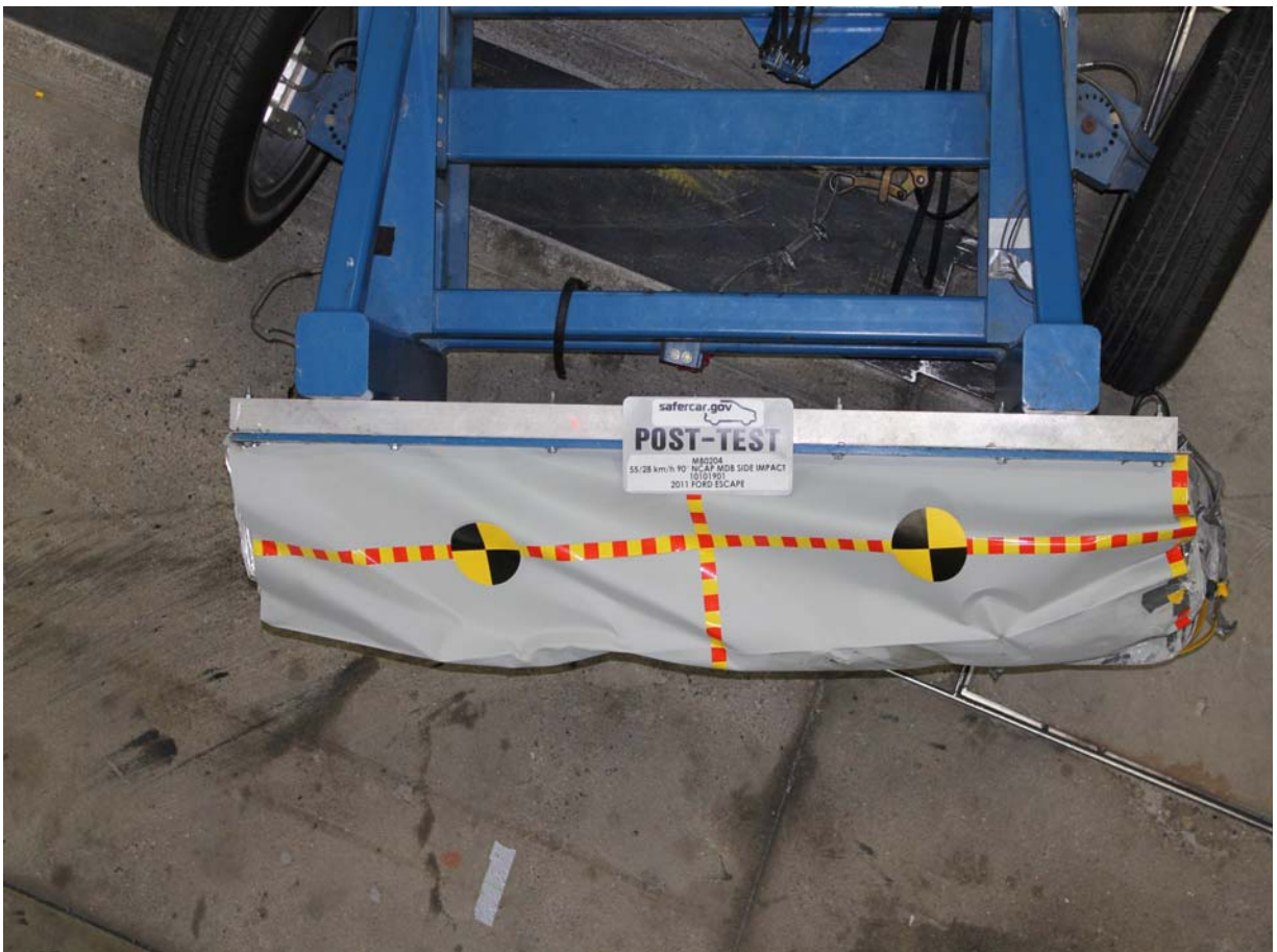
Post-Test Top View of MDB Impactor Face
