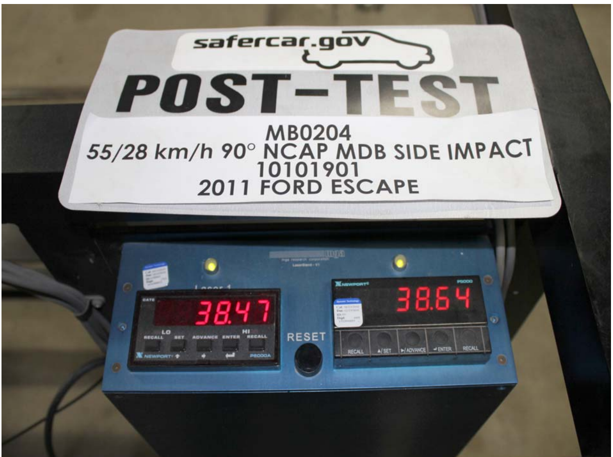
Post-Test Primary and Redundant Speed Trap Read-Out
