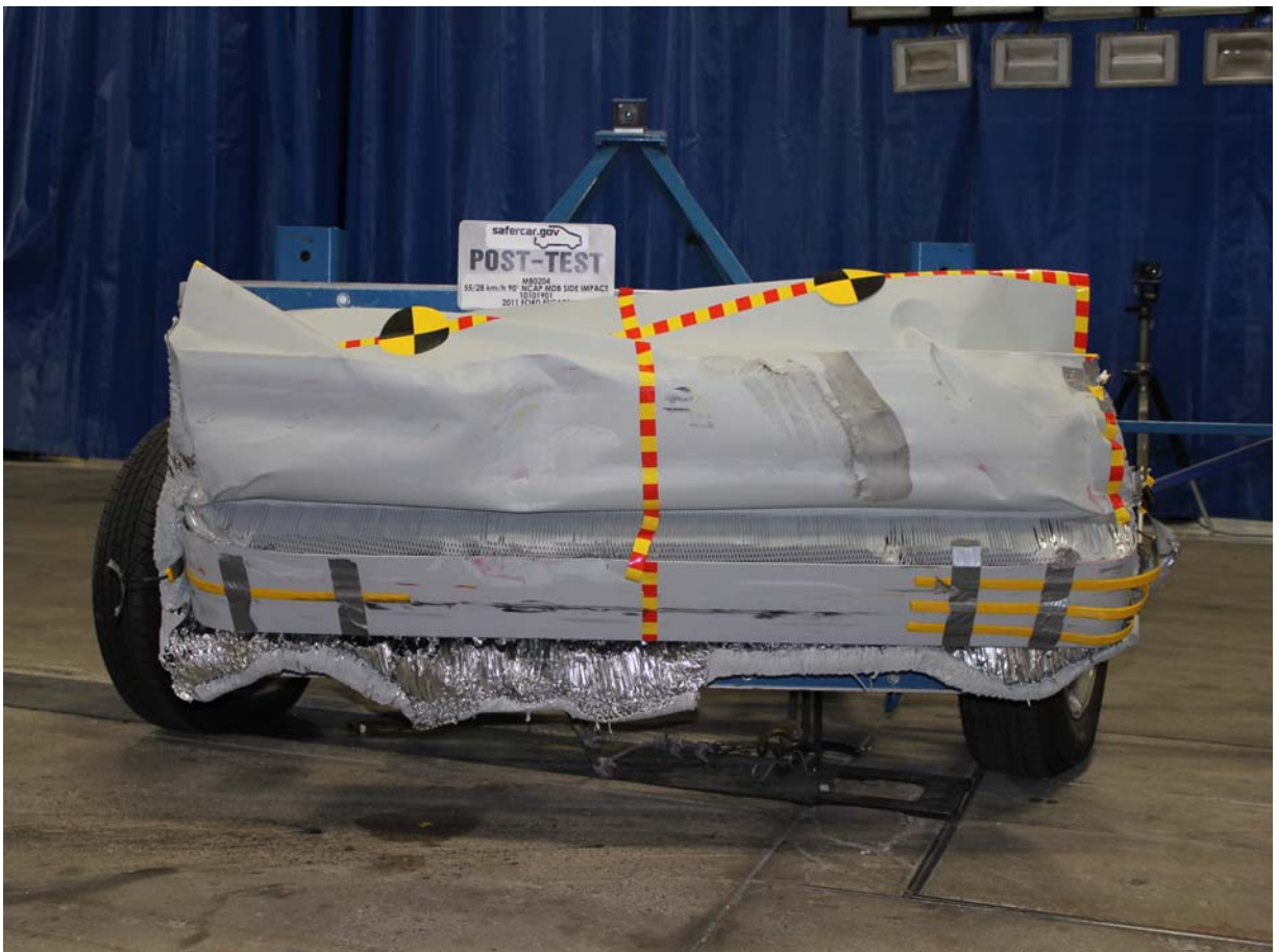
Post-Test Front View of MDB Impactor Face
