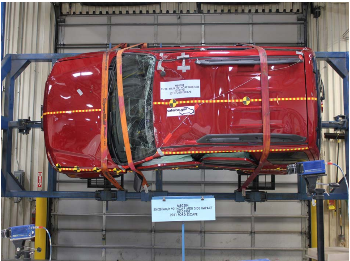
FMVSS No. 301/305 Rollover 90 Degrees
