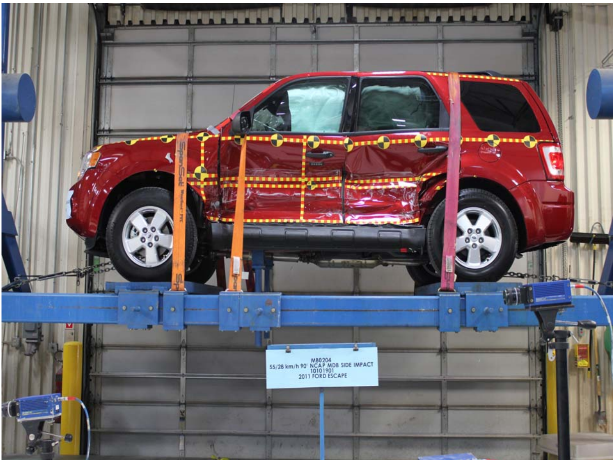
FMVSS No. 301/305 Rollover 0 Degrees
