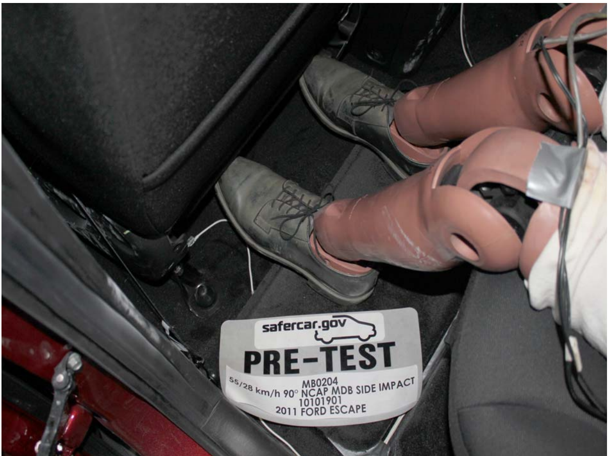
Pre-Test Placement of Rear Passenger Dummy's Feet
