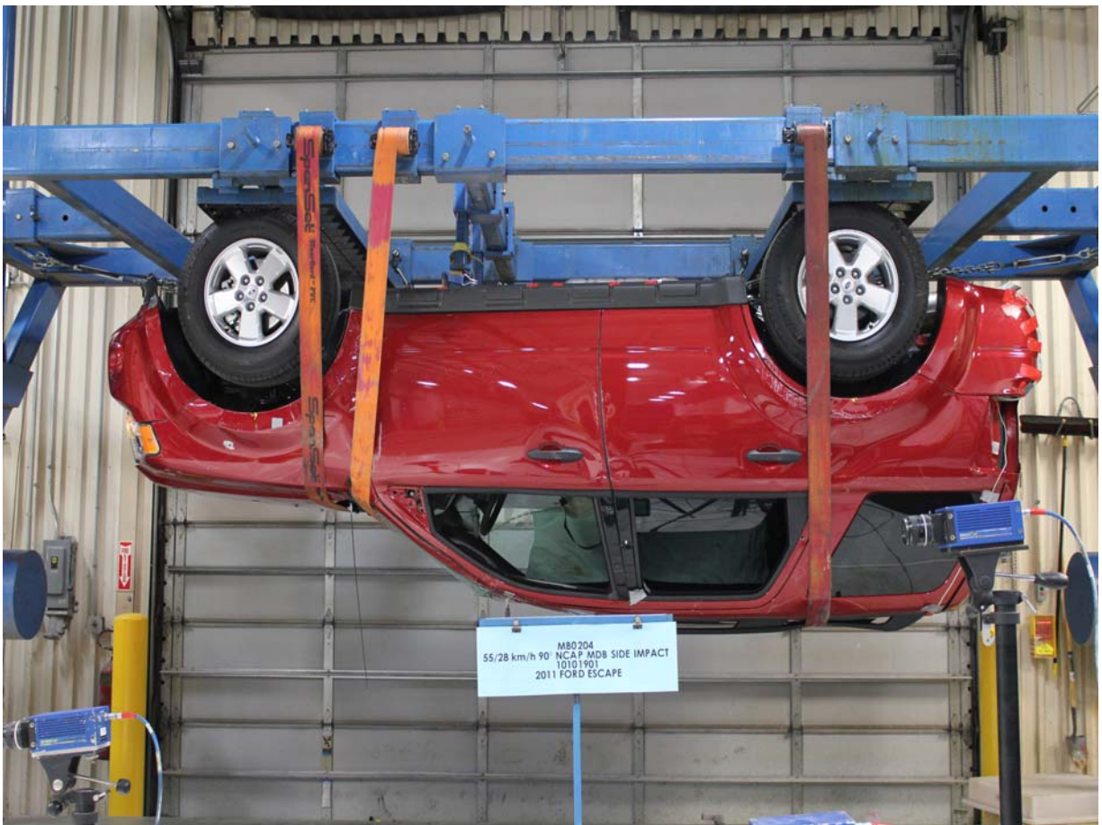
FMVSS No. 301/305 Rollover 180 Degrees
