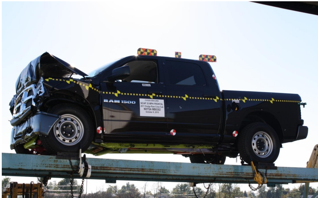
Figure A-64: Vehicle at 0° on Static Rollover Device
