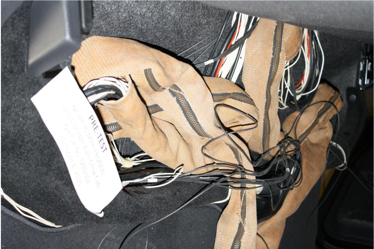
Figure A-27: Pre-Test Dummy Cable Routing
