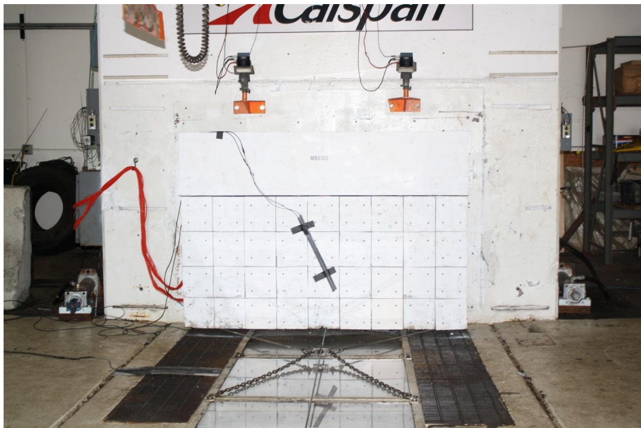
Figure A-2: Load Cell Wall
