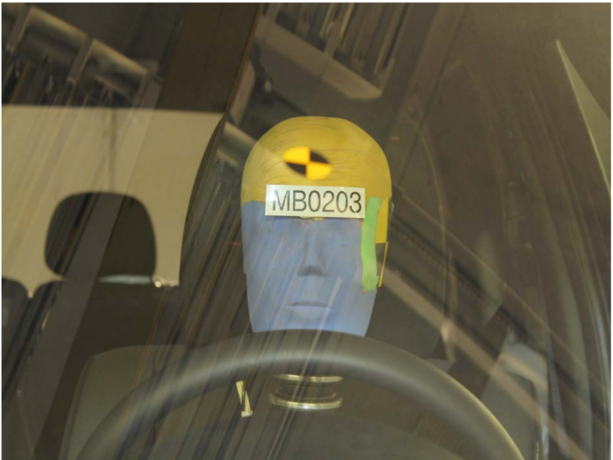
Pre-Test Frontal View of Dummy Head and Shoulders in Relation to Head Restraint
