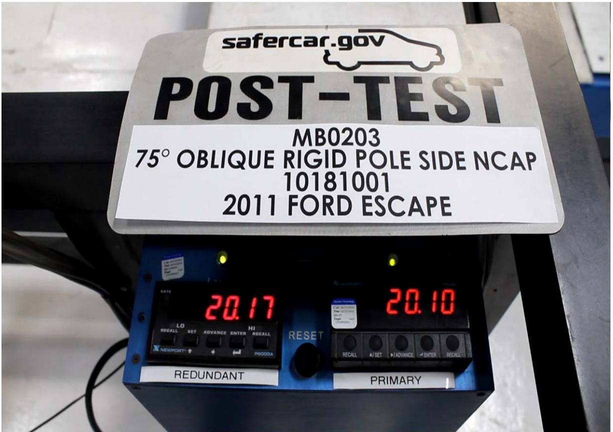
Post-Test Primary and Redundant Speed Trap Read-Out
