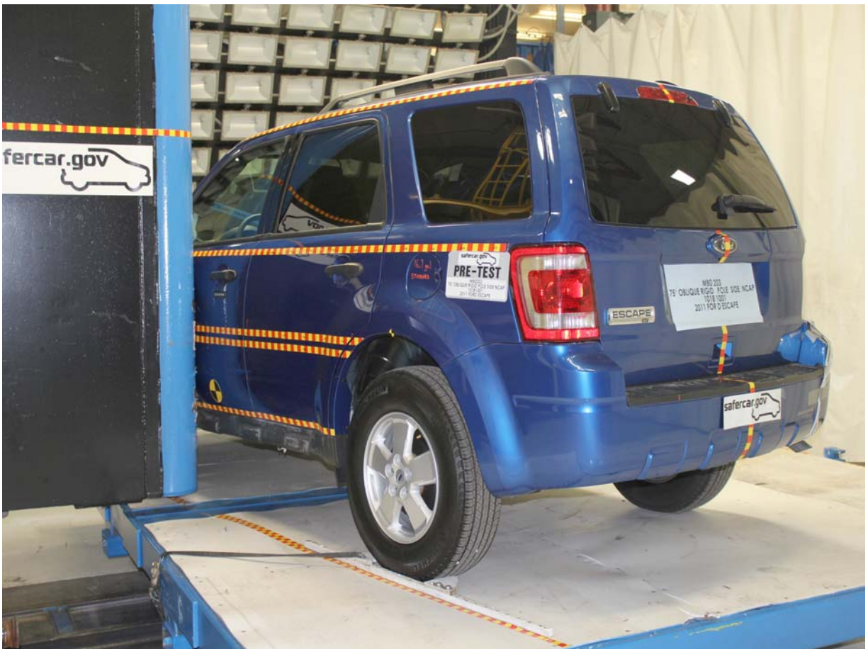
Pre-Test Right Side View of Pole Positioned Against Side of Vehicle at Ideal Impact Point
