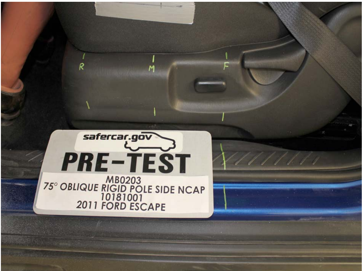
Pre-Test Close-Up Left Side View of Driver Seat Track Showing Test Position
