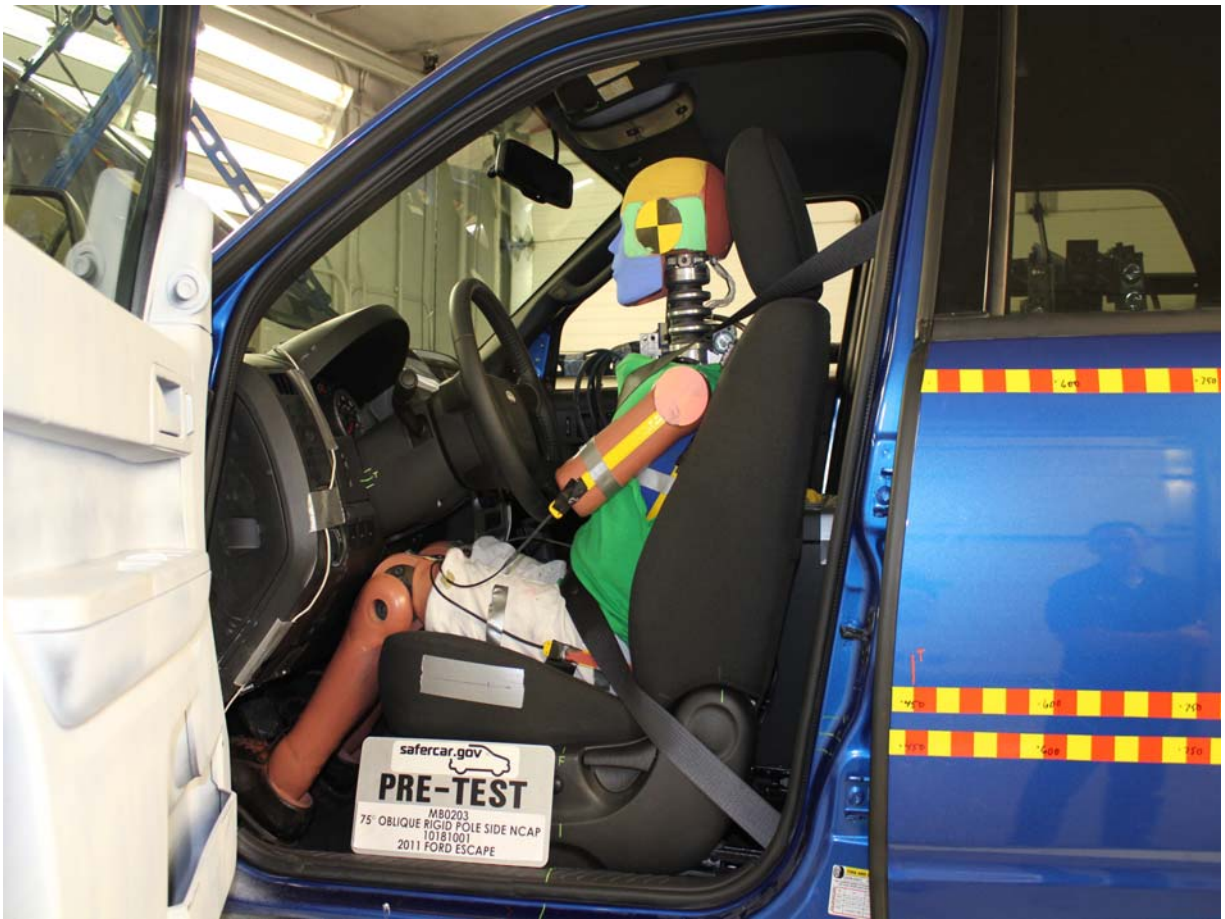
Pre-Test Left Side View of Dummy Showing Belts, Chalking, and Contact Switches
