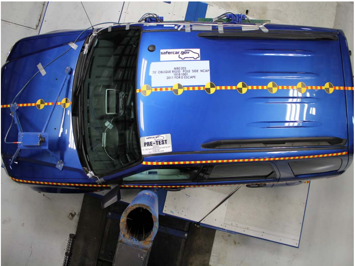
Pre-Test Overhead View of Test Vehicle and Pole
