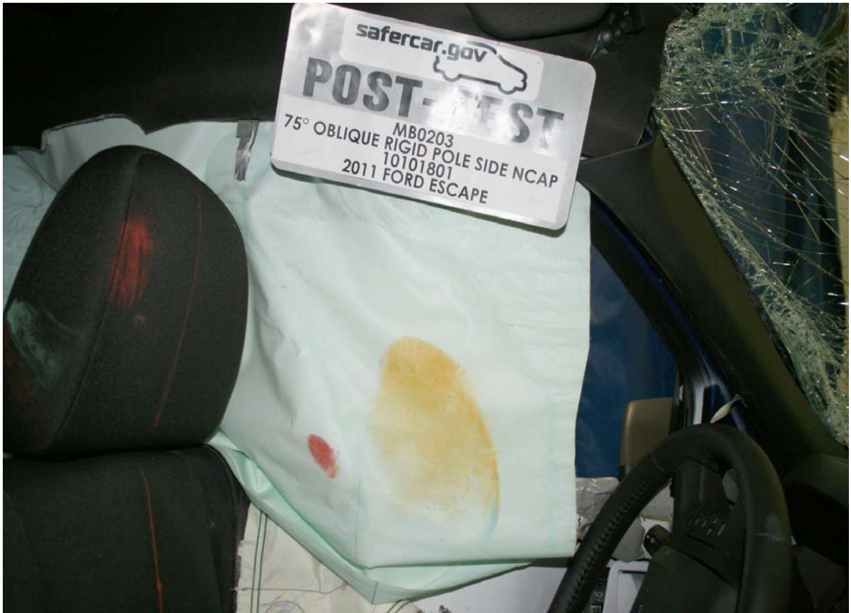
Post-Test Dummy Close-Up Head Contact with Side Airbag View
