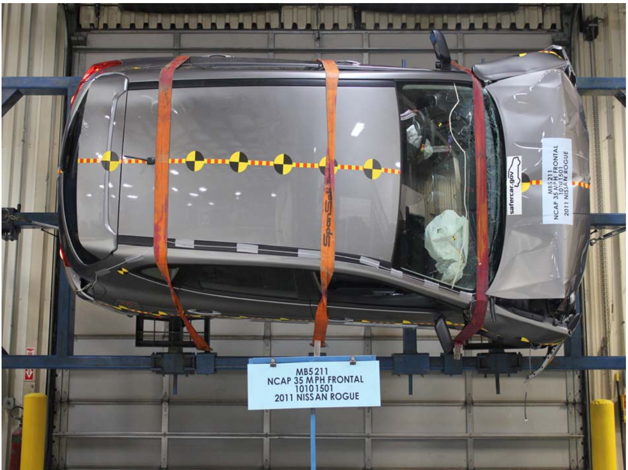
Vehicle at 90 Degrees on Static Rollover Device
