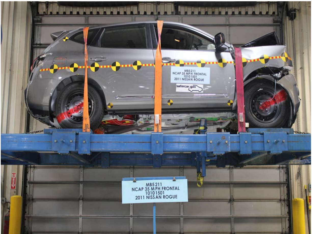
Vehicle at 360 Degrees on Static Rollover Device
