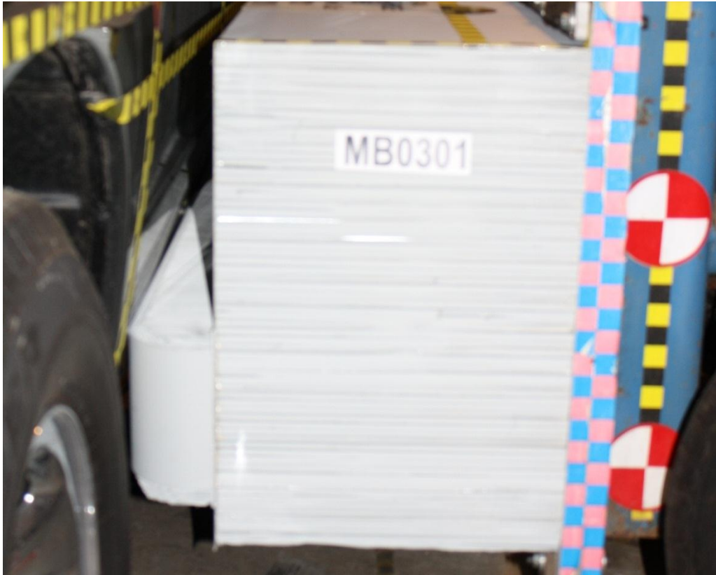
Figure A-17: Pre-Test Left Side View of MDB Positioned Against Side of Test Vehicle
