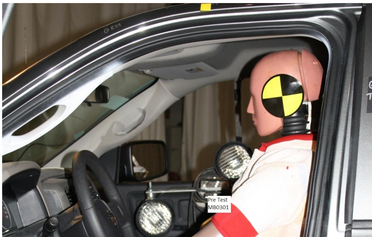
Figure A-27: Pre-Test Left Side View of Driver Dummy Showing Belt, Chalking, and Contact Switches
