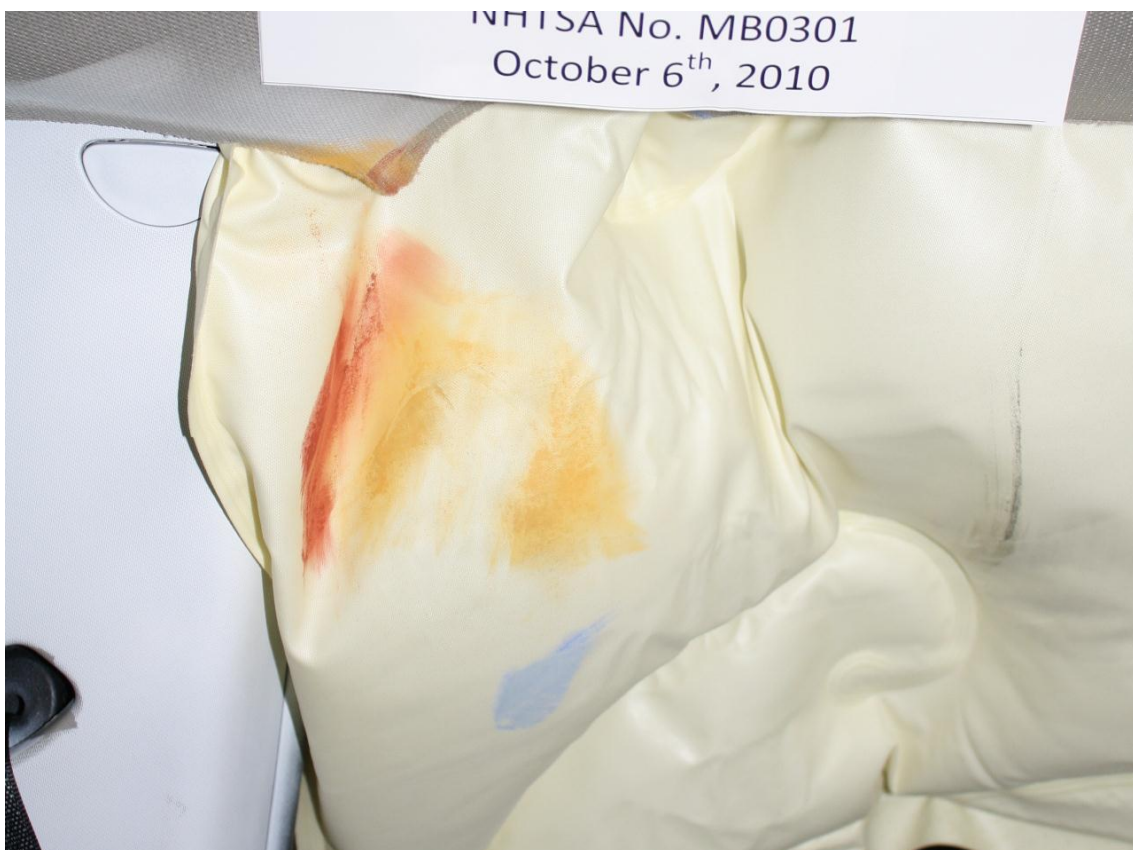
Figure A-74: Post-test Rear Passenger Dummy Close-Up Head Contact with Side Airbag View
