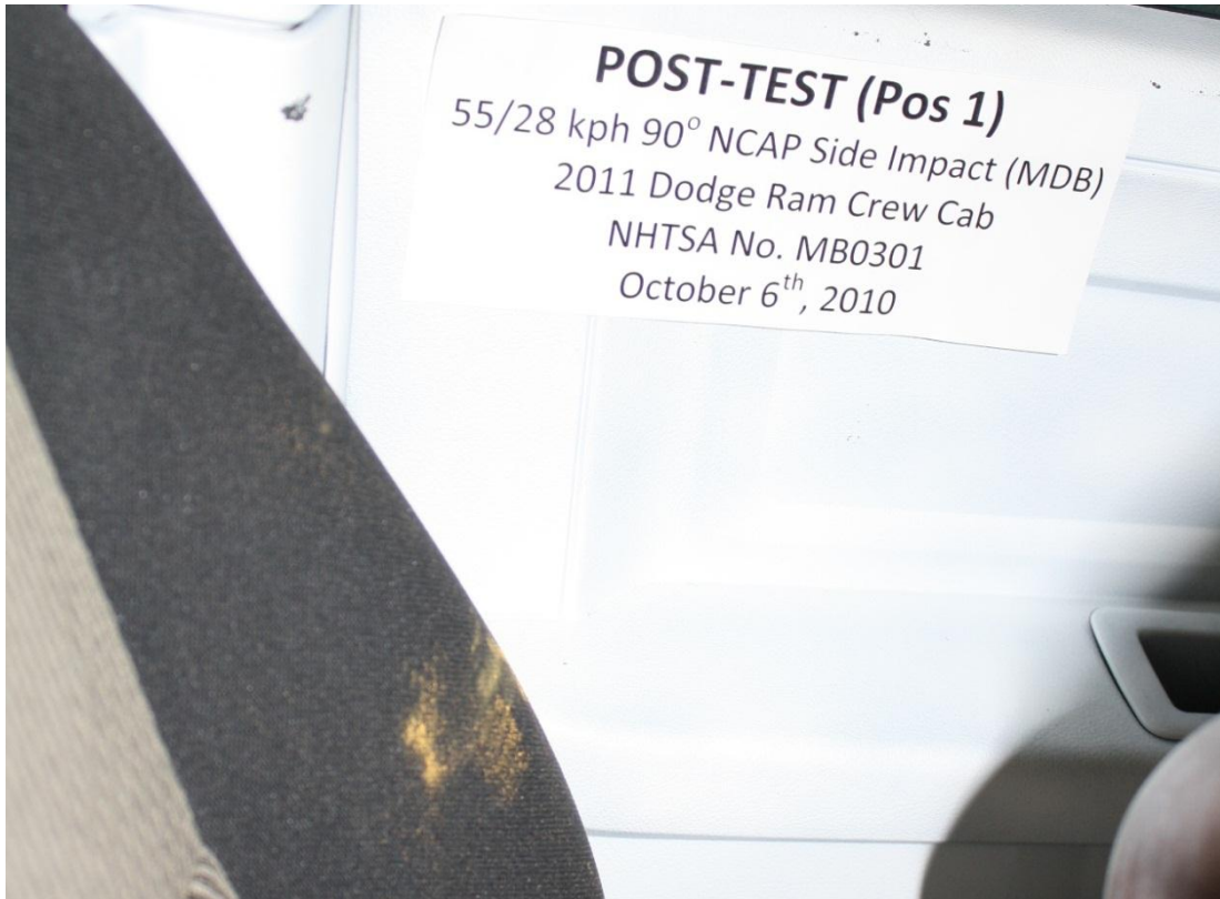
Figure A-49: Post-Test Driver Dummy Close-Up Torso Contact with Vehicle Interior View
