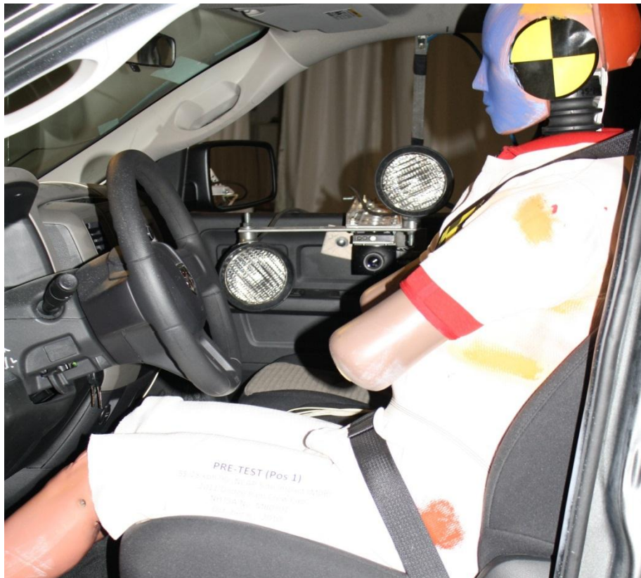
Figure A-27: Pre-Test Left Side View of Driver Dummy Showing Belt, Chalking, and Contact Switches
