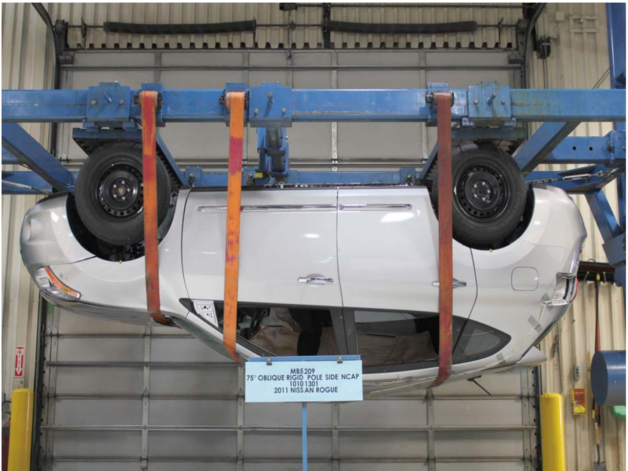
FMVSS No. 301/305 Rollover 180 Degrees
