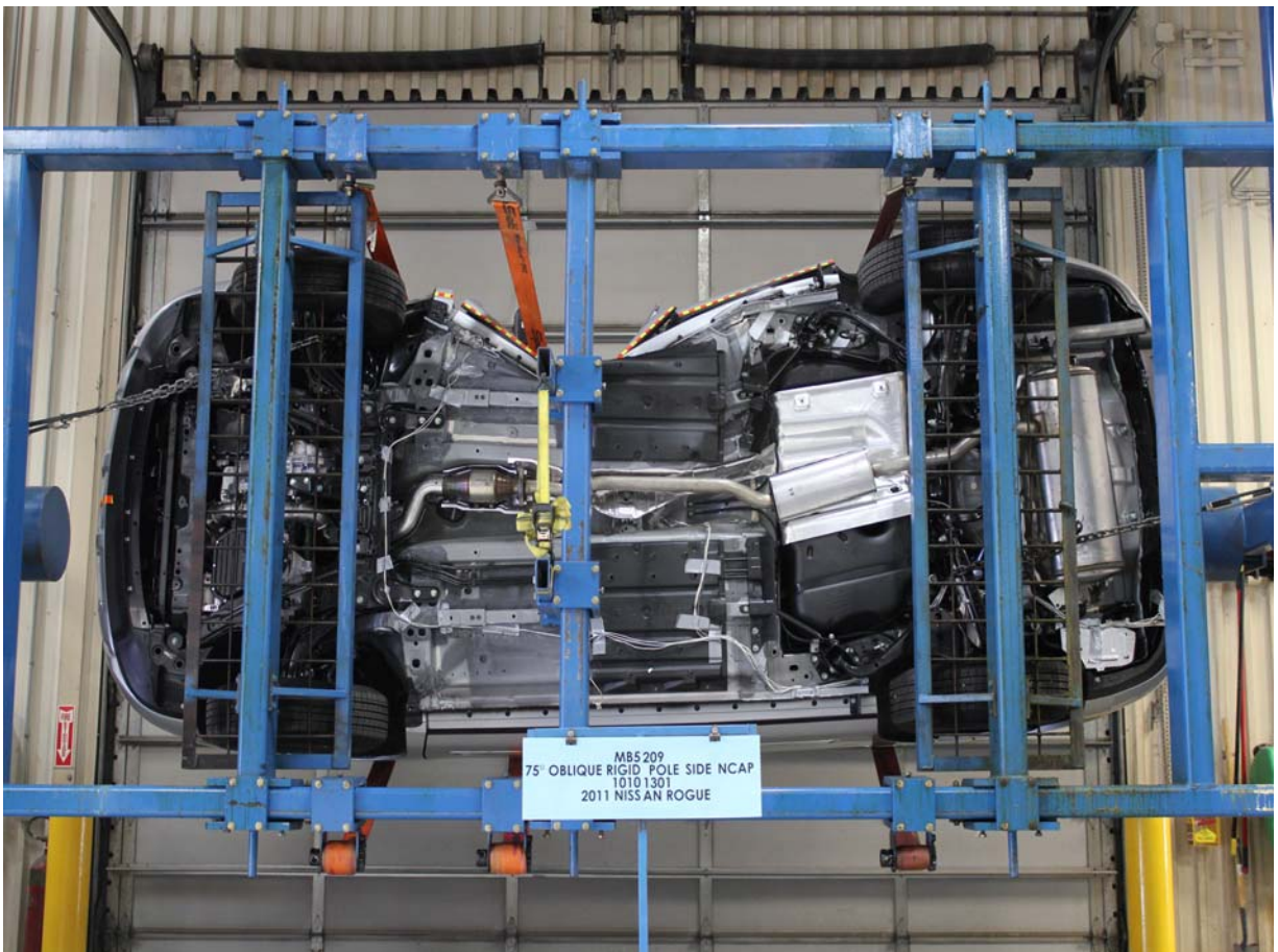
FMVSS No. 301/305 Rollover 90 Degrees
