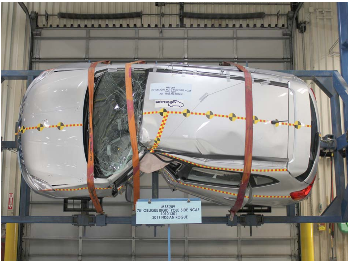
FMVSS No. 301/305 Rollover 270 Degrees
