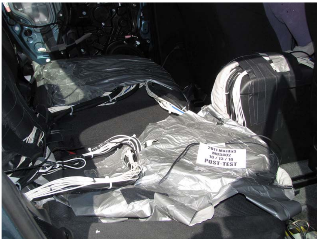
FIGURE 28. Post-Test Dummy Cable Routing
