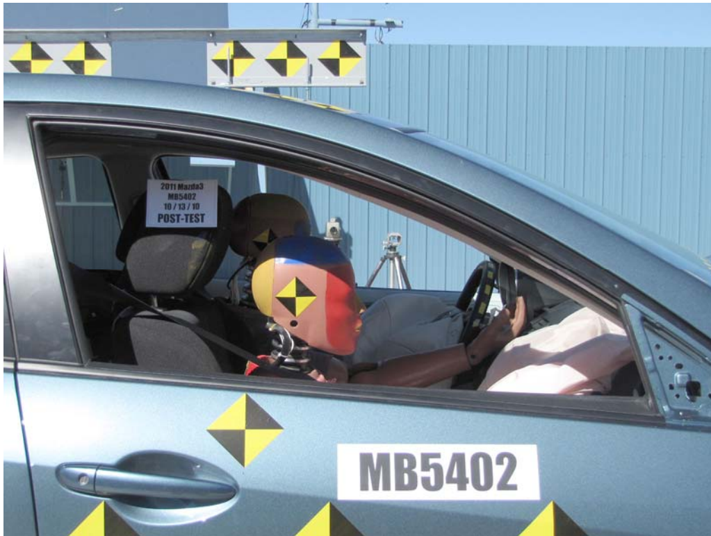
FIGURE 49. Post-Test Passenger Dummy Window View
