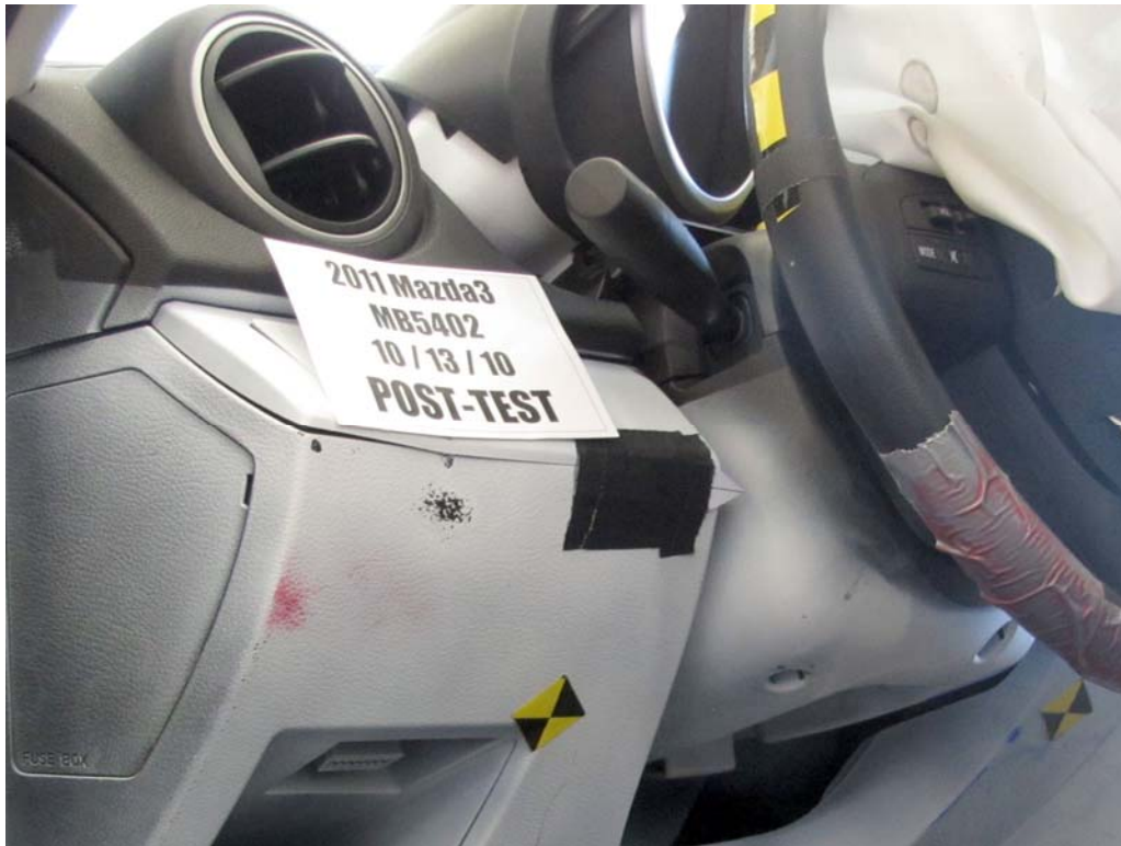
FIGURE 45. Post-Test View of Steering Column Shear Capsule
