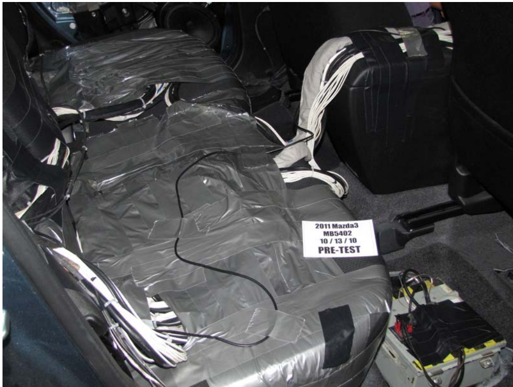
FIGURE 27. Pre-Test Dummy Cable Routing
