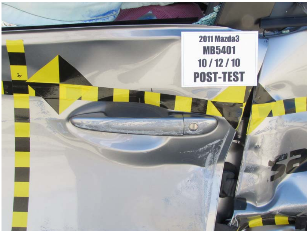
FIGURE 22. Post-Test Left Front Door Latch Close-Up
