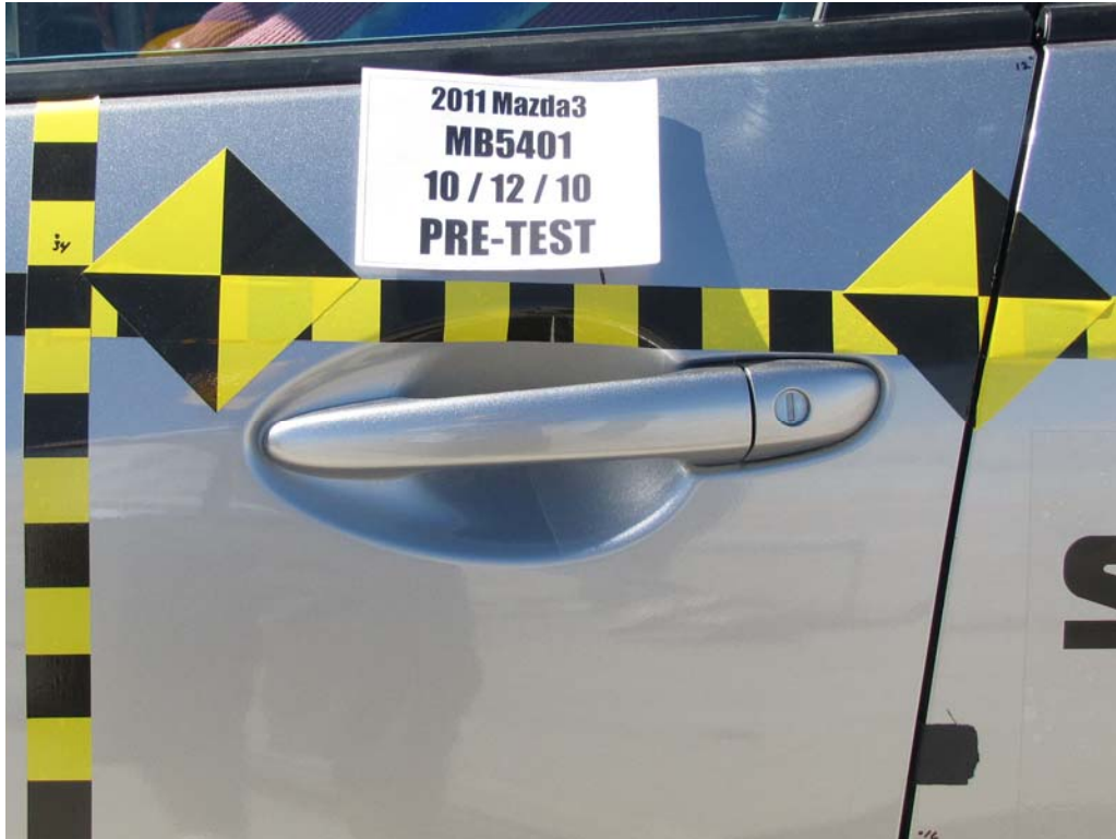
FIGURE 21. Pre-Test Left Front Door Latch Close-Up
