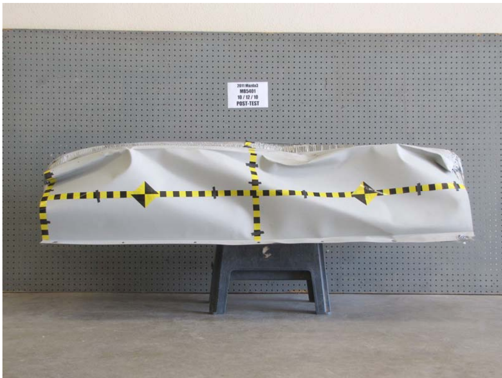
FIGURE 84. Post-Test Top View of MDB Impactor Face
