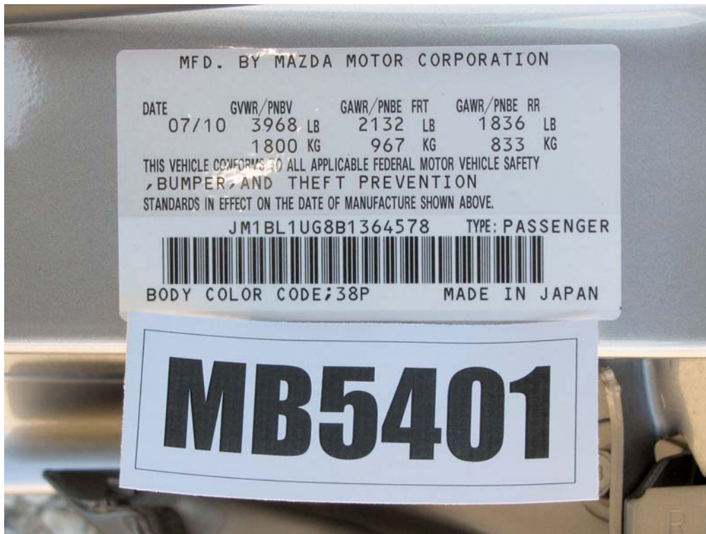
FIGURE 89. Close-Up View of Vehicle's Certification Label
