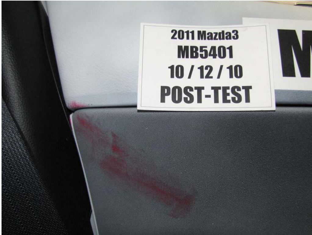
FIGURE 75. Post-Test Rear Passenger Dummy Close-Up Torso Contact with Vehicle Interior View
