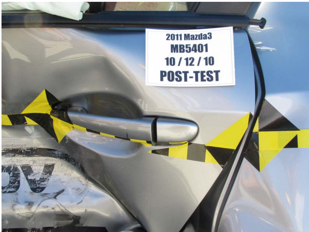
FIGURE 24. Post-Test Left Rear Door Latch Close-Up
