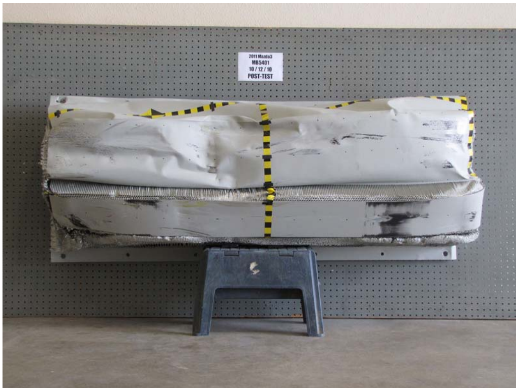
FIGURE 82. Post-Test Front View of MDB Impactor Face
