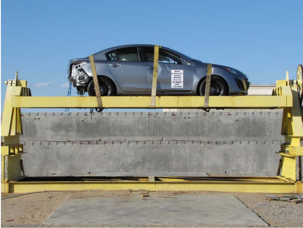
FIGURE 97. FMVSS No. 301/305 Rollover 360 Degrees
