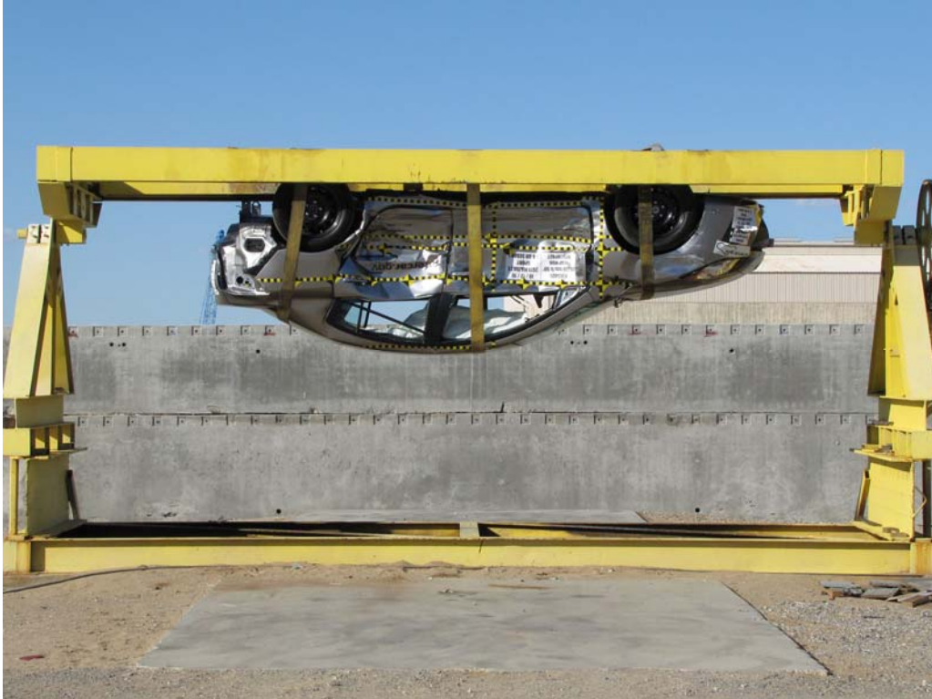
FIGURE 95. FMVSS No. 301/305 Rollover 180 Degrees
