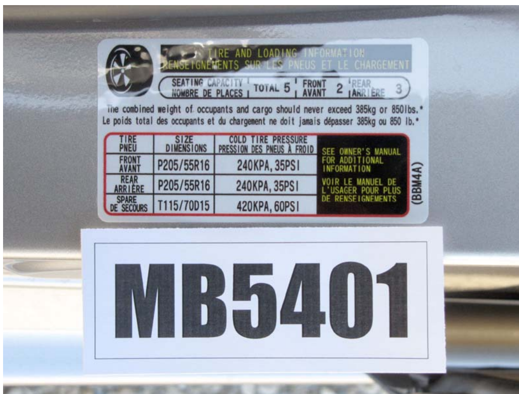
FIGURE 90. Close-Up View of Vehicle's Tire Information Placard
