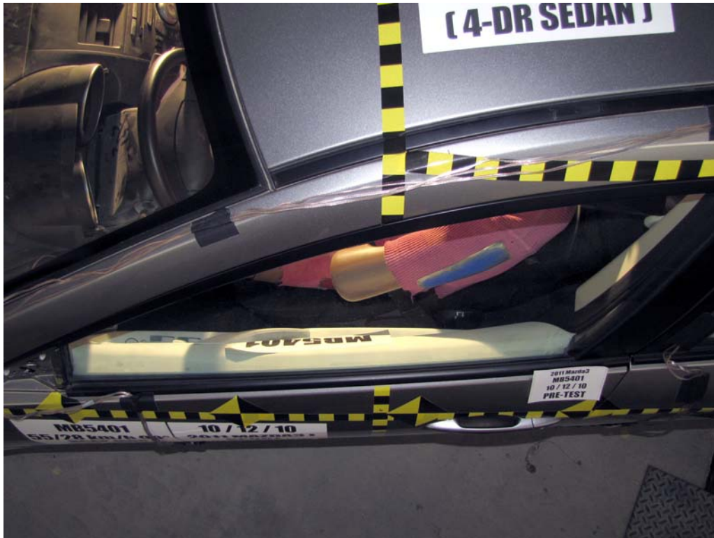
FIGURE 41. Pre-Test Driver Dummy and Door Clearance View
