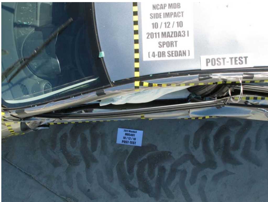
FIGURE 42. Post-Test Driver Dummy and Door Clearance View
