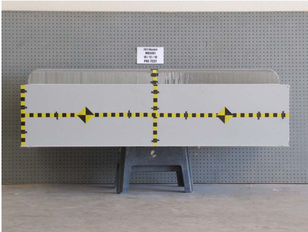
FIGURE 83. Pre-Test Top View of MDB Impactor Face
