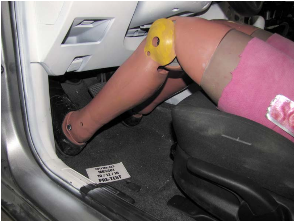
FIGURE 34. Pre-Test Placement of Driver Dummy's Feet
