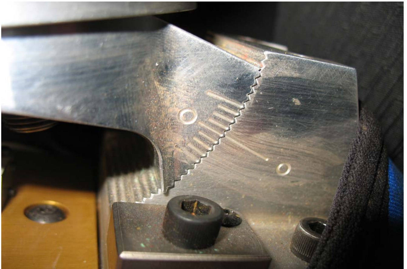
No. 030 – Pre-Test View of Dummy's Neck Showing Position of Adjustable Neck Bracket
