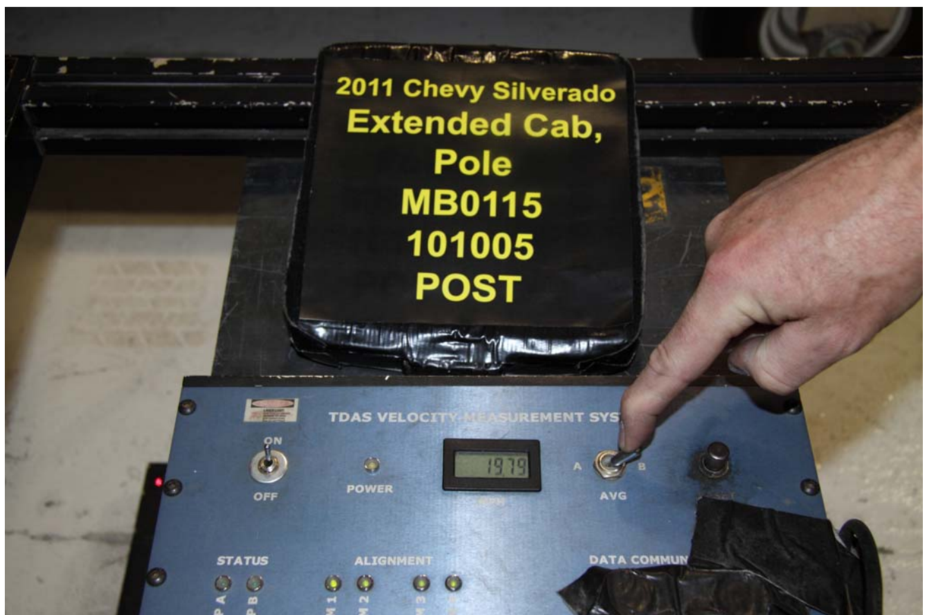
No. 060a – Post-Test Redundant Speed Trap Read-Out
