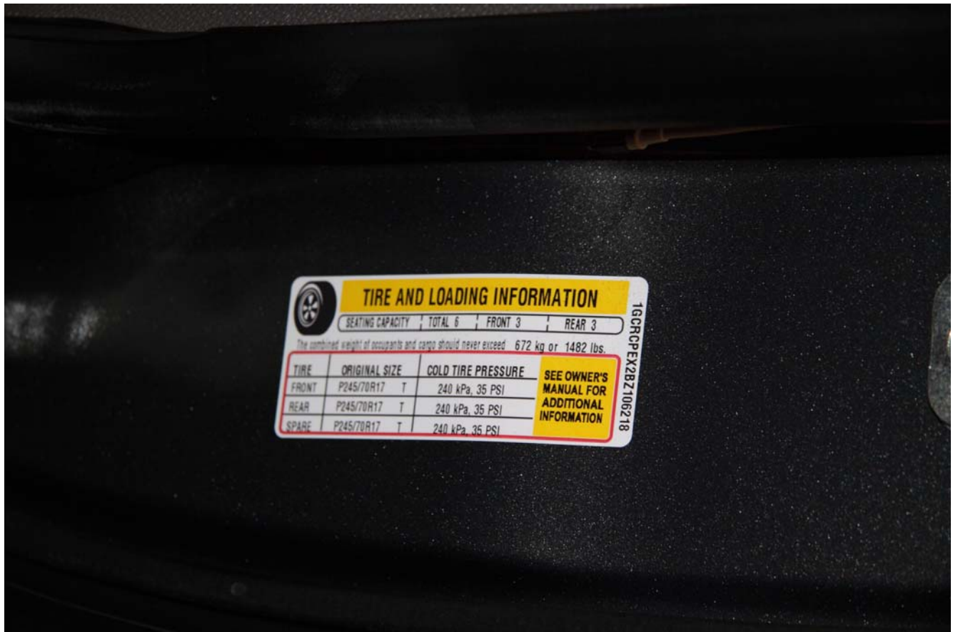
No. 054 – Close-Up View of Vehicle's Tire Information Label
