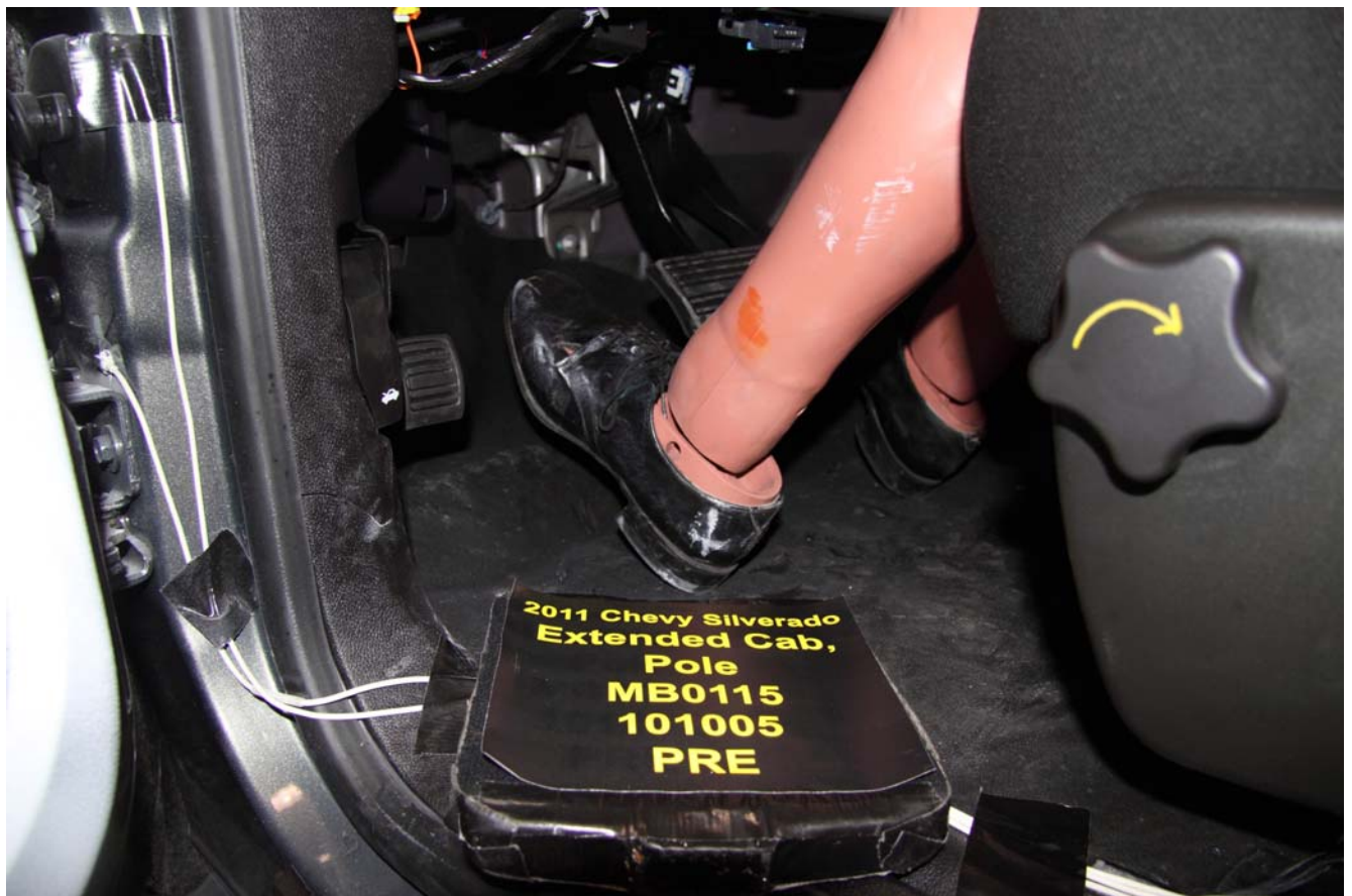
No. 032 – Pre-Test Placement of Dummy's Feet
