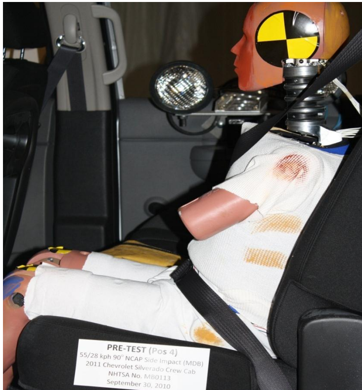
Figure A-53: Pre-test Left Side View of Passenger Dummy Showing Belt, Chalking, and Contact Switches
