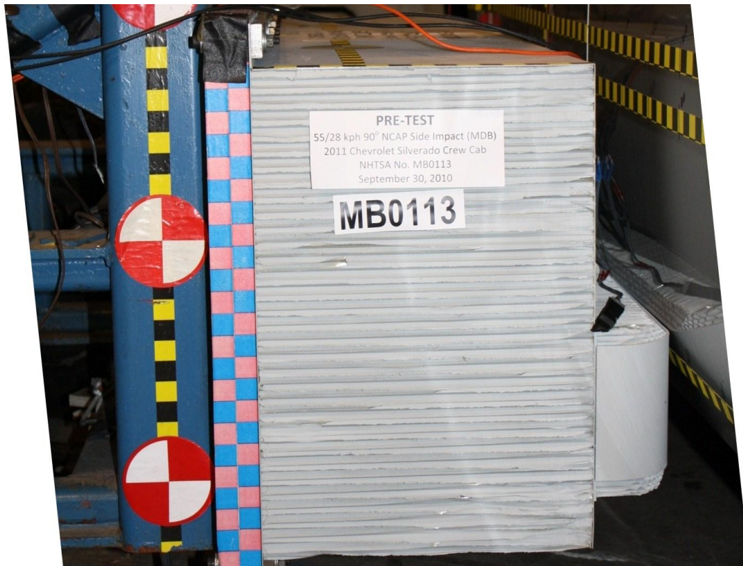
Figure A-18: Pre-Test Right Side View of MDB Positioned Against Side of Test Vehicle
