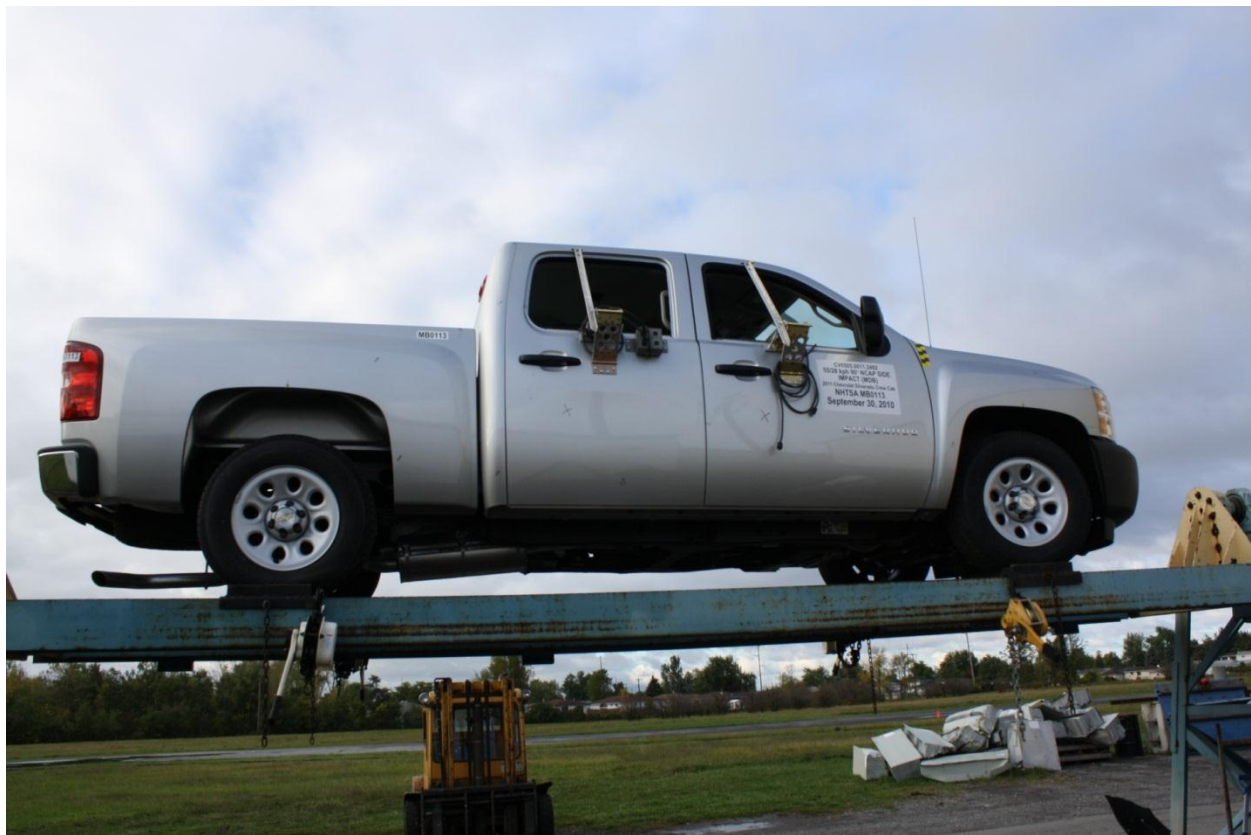
Figure A-93: FMVSS No. 301 Rollover 0°
