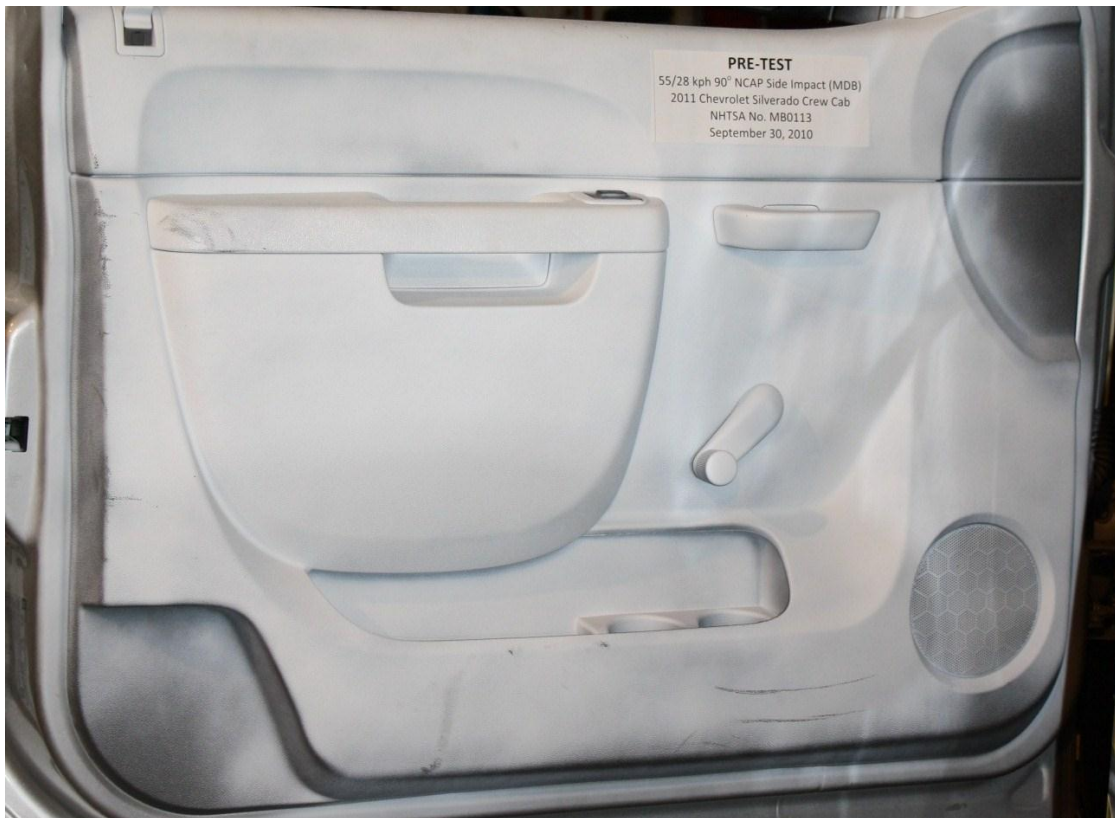
Figure A-45: Pre-test Driver Inner Door Panel View
