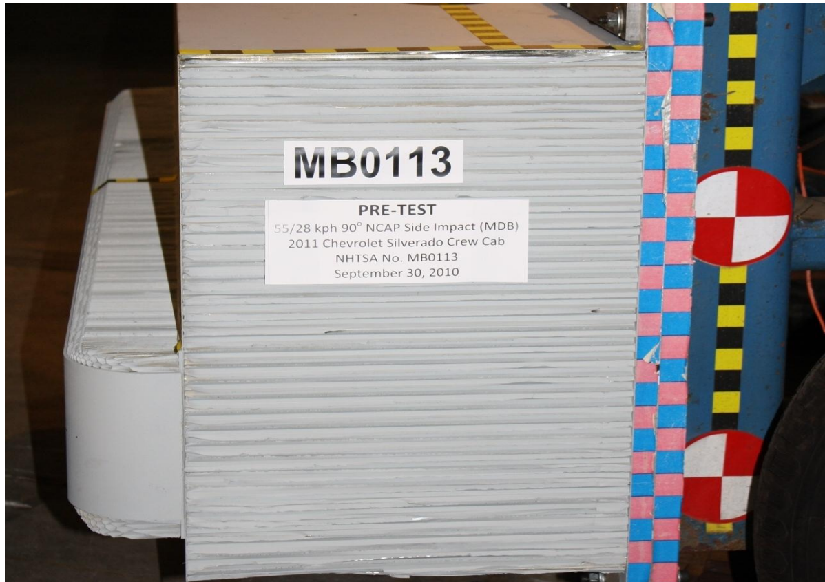
Figure A-85: Pre-Test Left Side View of MDB Impactor Face
