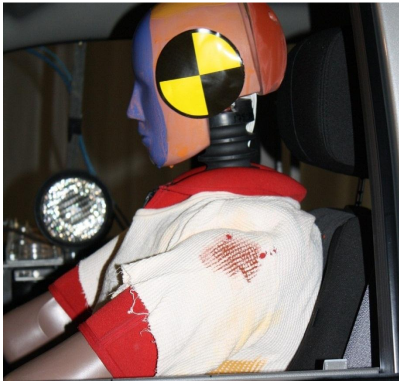
Figure A-27: Pre-Test Left Side View of Driver Dummy Showing Belt, Chalking, and Contact Switches
