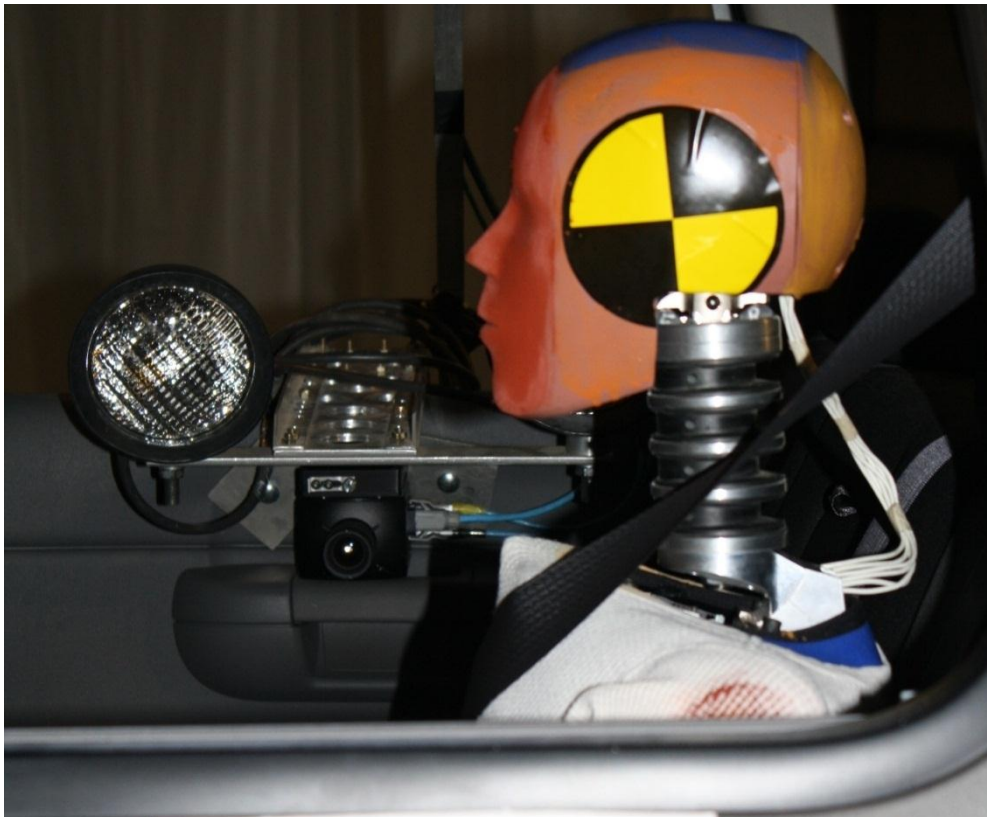
Figure A-53: Pre-test Left Side View of Passenger Dummy Showing Belt, Chalking, and Contact Switches
