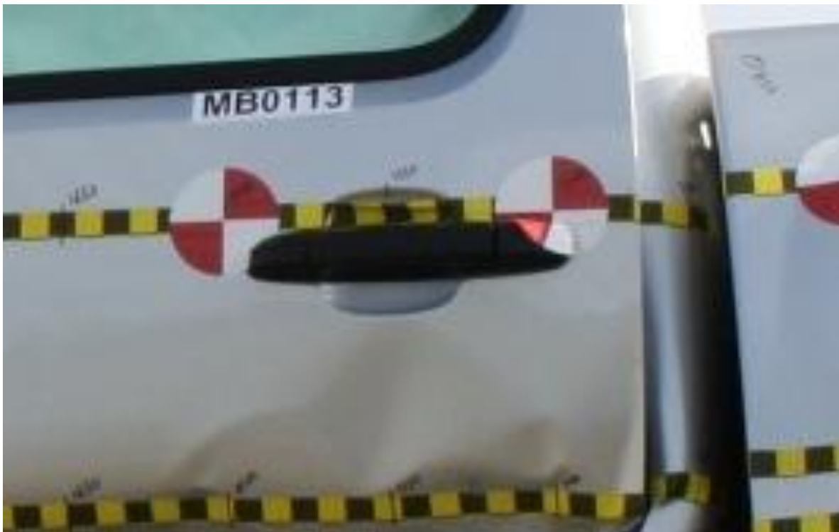
Figure A-23: Pre-Test Left Rear Door Latch Close-up
