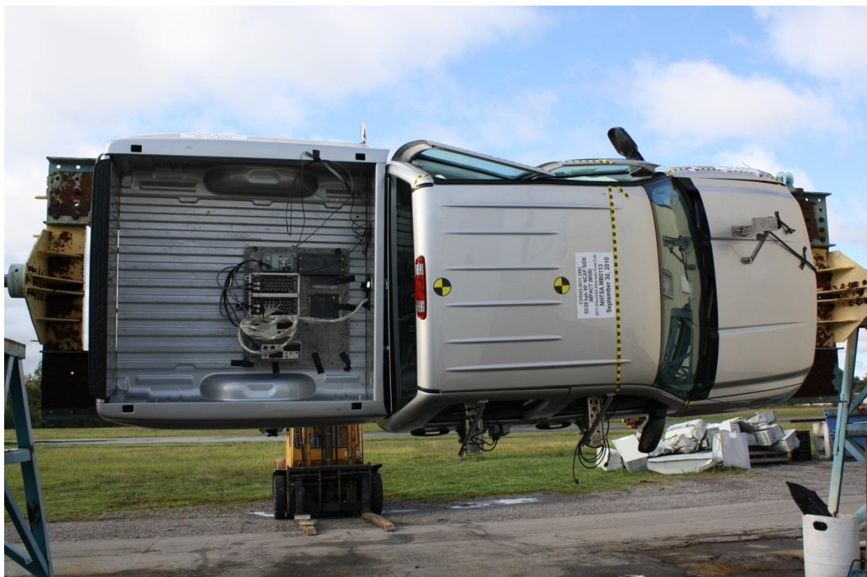
Figure A-96: FMVSS No. 301 Rollover 270°
