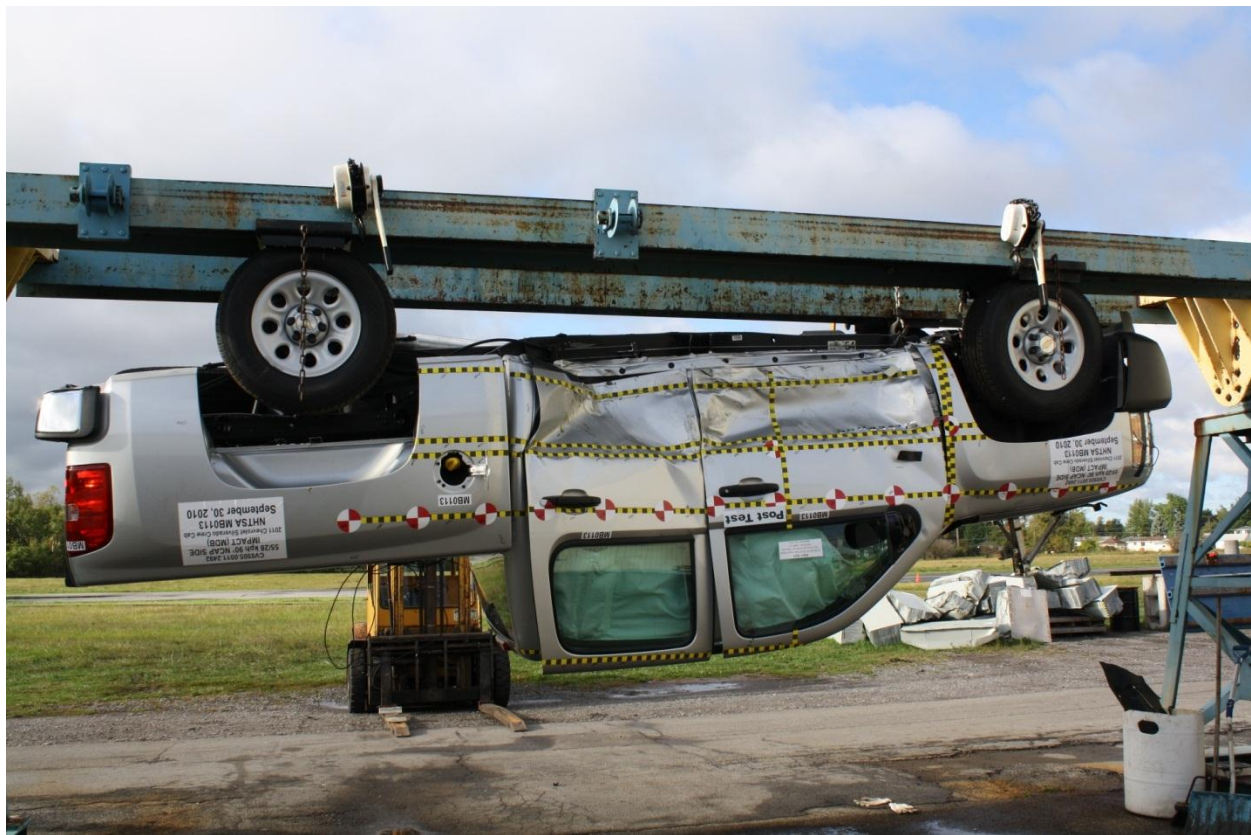
Figure A-95: FMVSS No. 301 Rollover 180°
