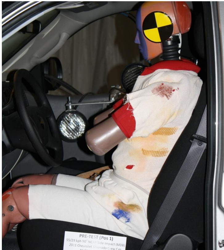
Figure A-27: Pre-Test Left Side View of Driver Dummy Showing Belt, Chalking, and Contact Switches
