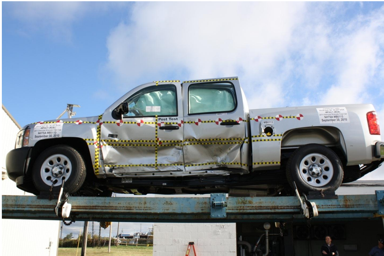
Figure A-97: FMVSS No. 301 Rollover 360°
