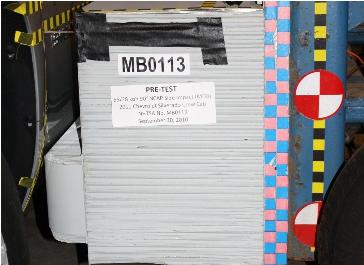
Figure A-17: Pre-Test Left Side View of MDB Positioned Against Side of Test Vehicle
