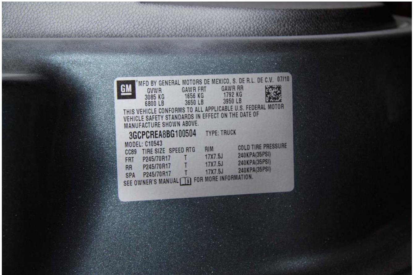
No. 053 – Close-Up View of Vehicle's Certification Label
