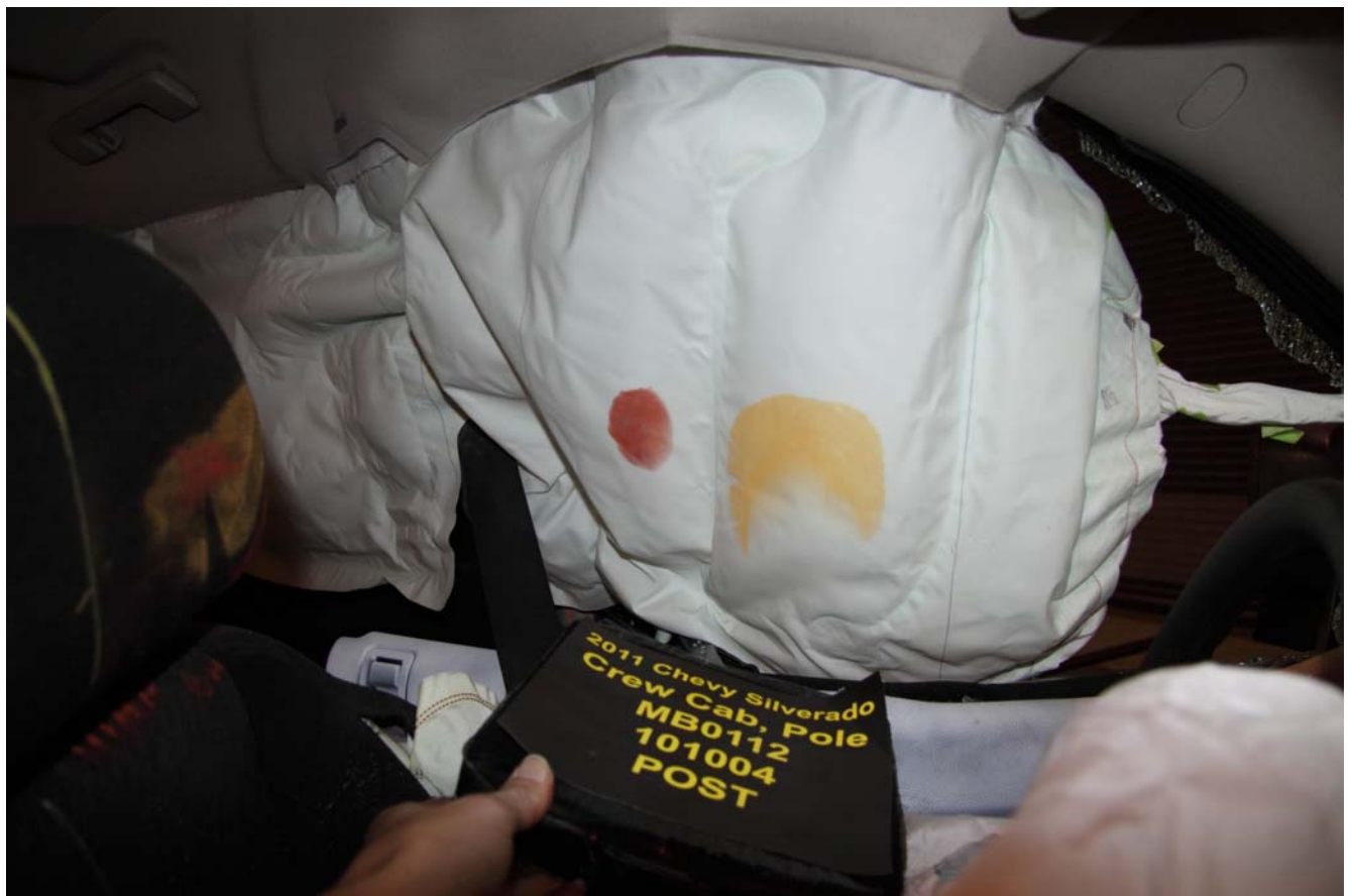
No. 046 – Post-Test Dummy Close-Up Head Contact with Side Airbag View
