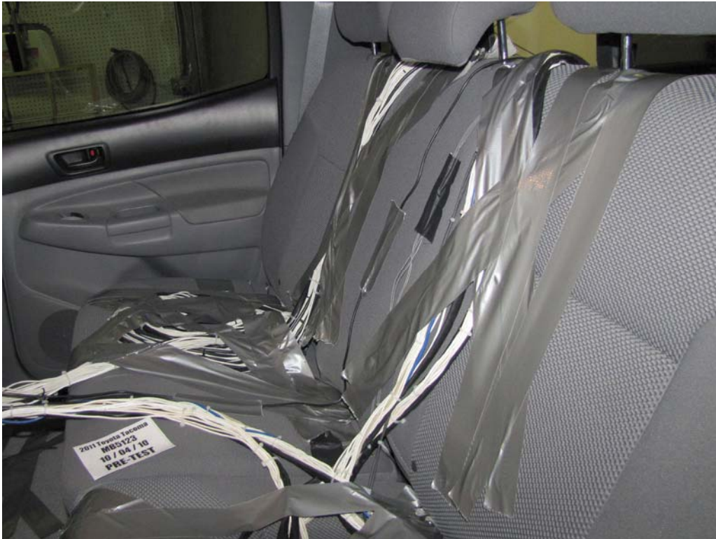
FIGURE 27. Pre-Test Dummy Cable Routing
