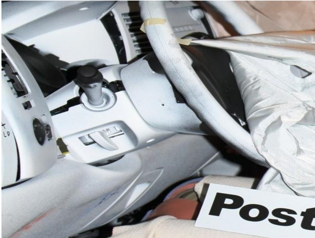
Figure A-45: Post-Test View of the Steering Column Shear Capsule
