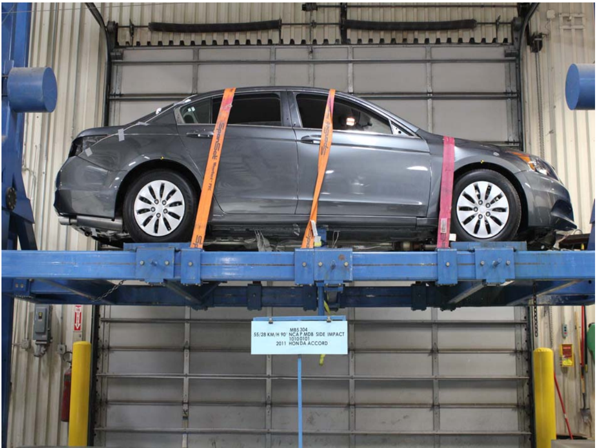
FMVSS No. 301/305 Rollover 0 Degrees
