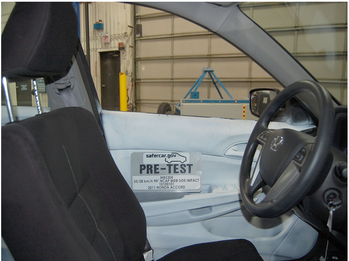
Pre-Test Driver Inner Door Panel View
