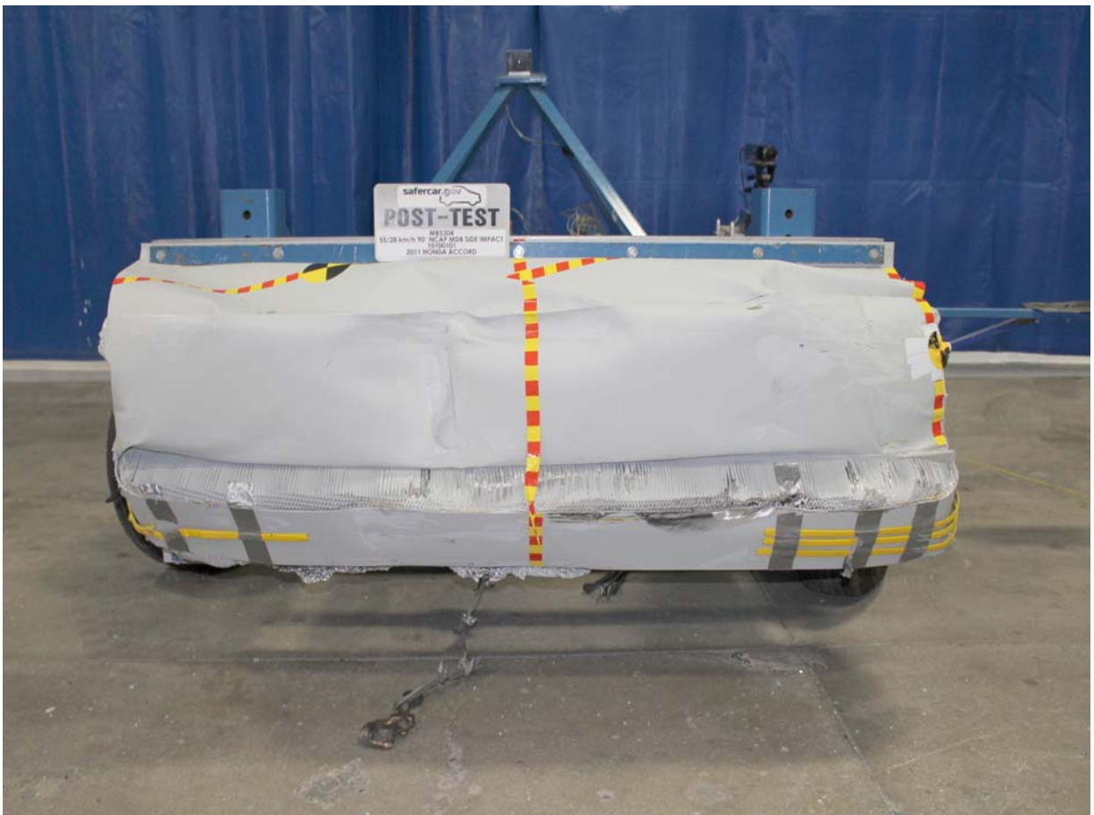
Post-Test Front View of MDB Impactor Face
