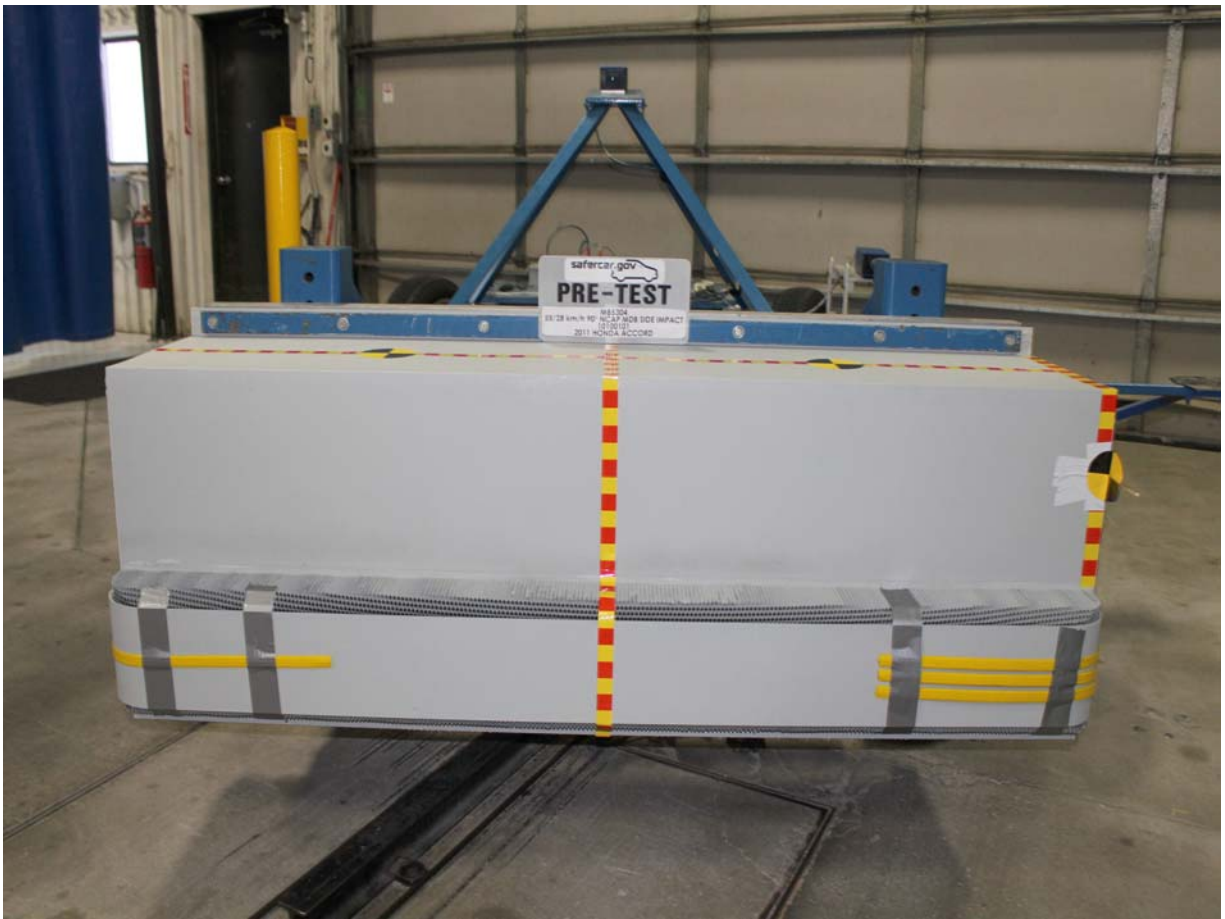
Pre-Test Front View of MDB Impactor Face
