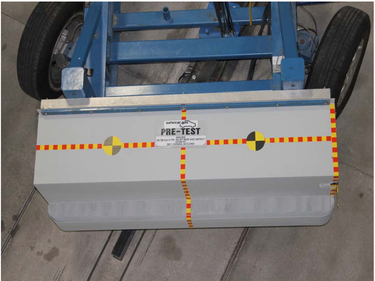
Pre-Test Top View of MDB Impactor Face
