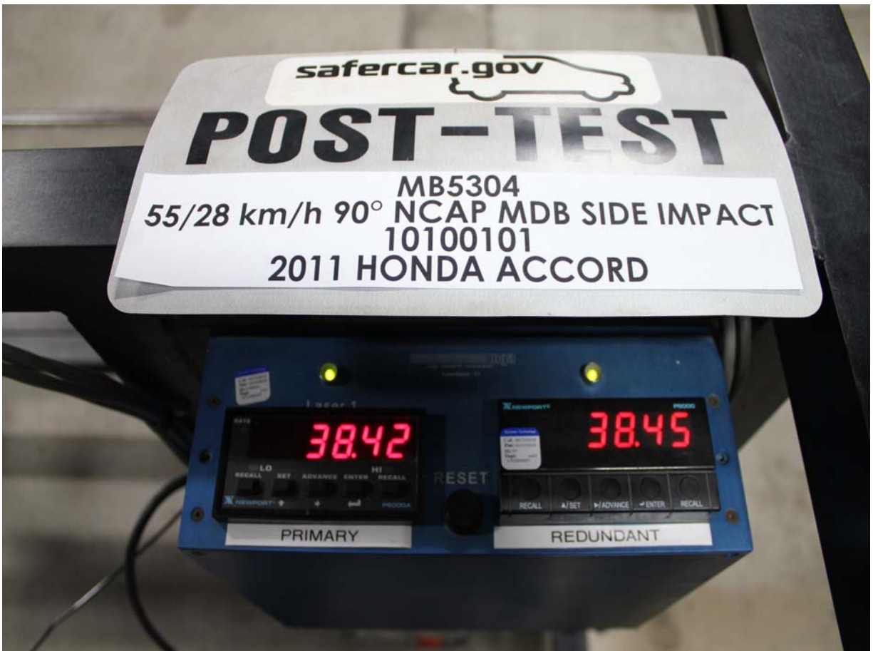
Post-Test Primary and Redundant Speed Trap Read-Out
