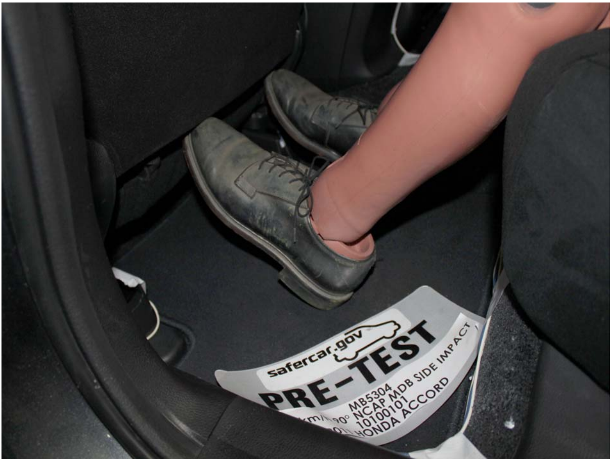
Pre-Test Placement of Rear Passenger Dummy's Feet
