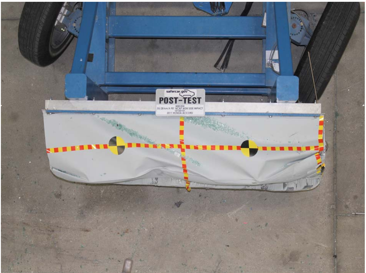
Post-Test Top View of MDB Impactor Face
