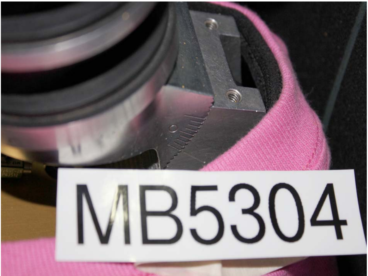
Pre-Test View of Rear Passenger Dummy's Neck Showing Position of Adjustable Neck Bracket
