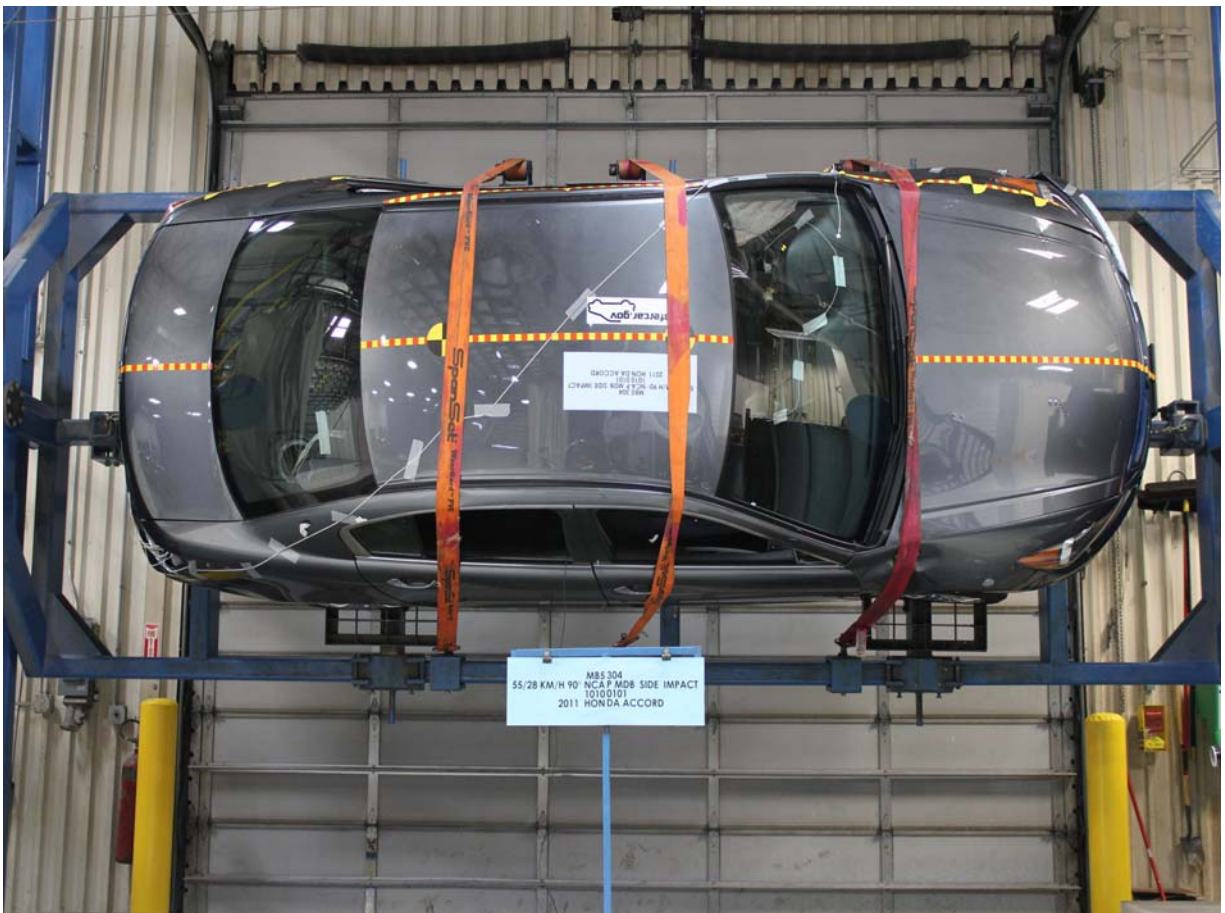
FMVSS No. 301/305 Rollover 270 Degrees
