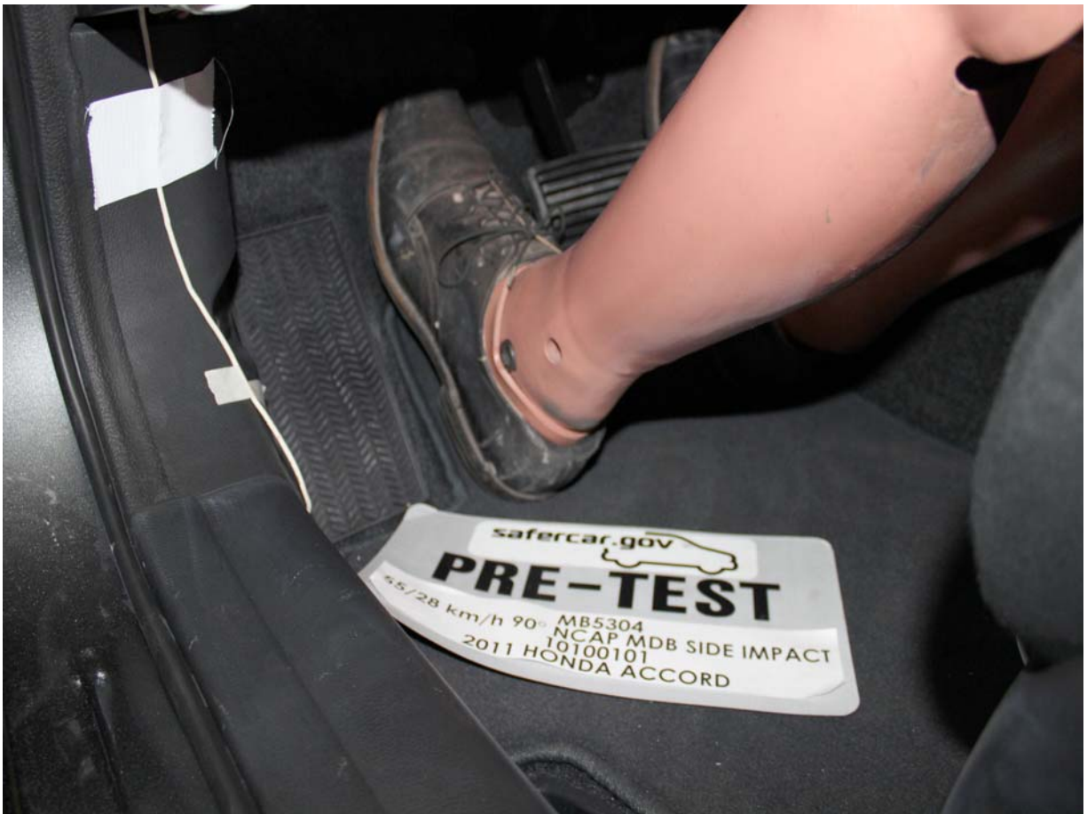
Pre-Test Placement of Driver Dummy's Feet
