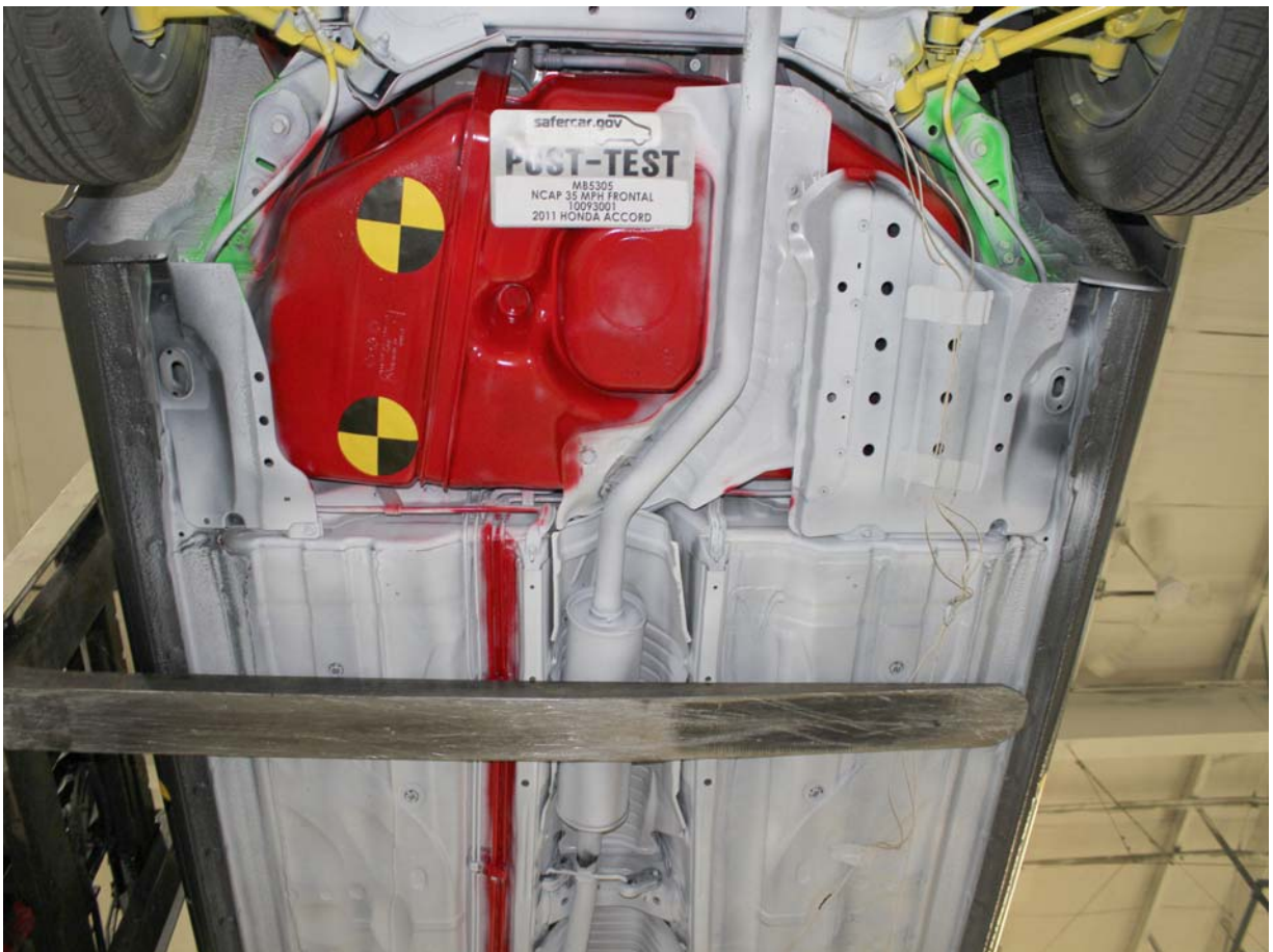
Post-Test Mid Rear Underbody View
