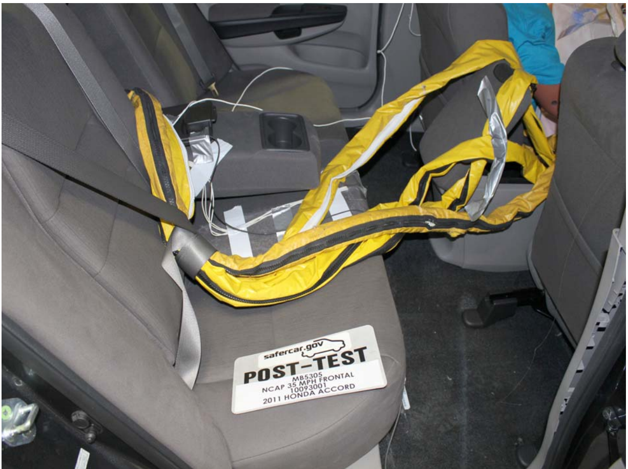
Post-Test Dummy Cable Routing
