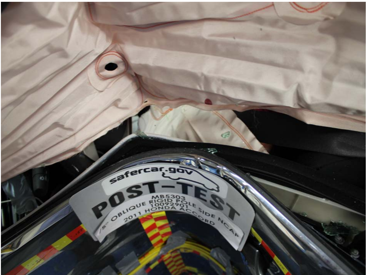
Post-Test Dummy and Door Clearance View
