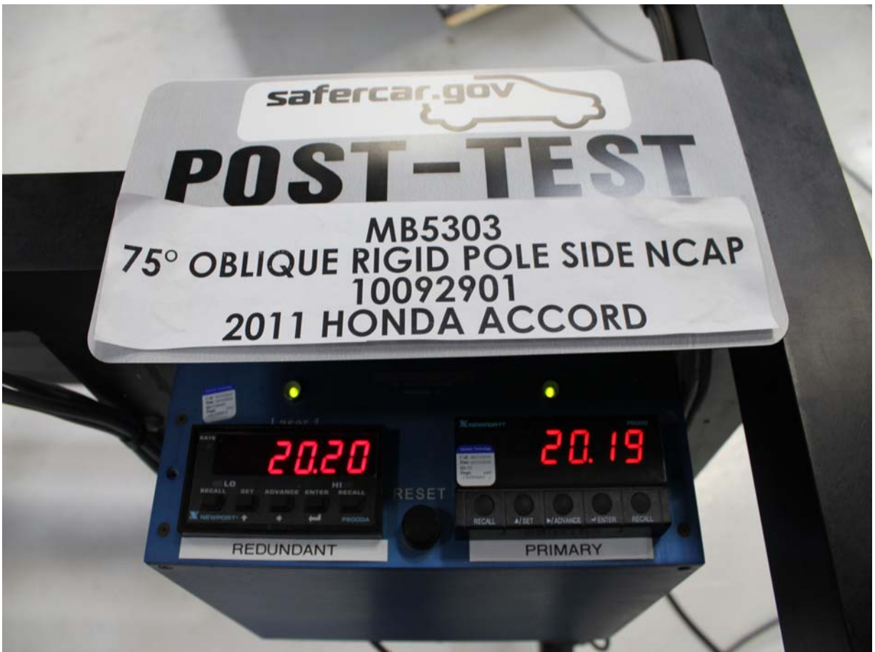
Post-Test Primary and Redundant Speed Trap Read-Out
