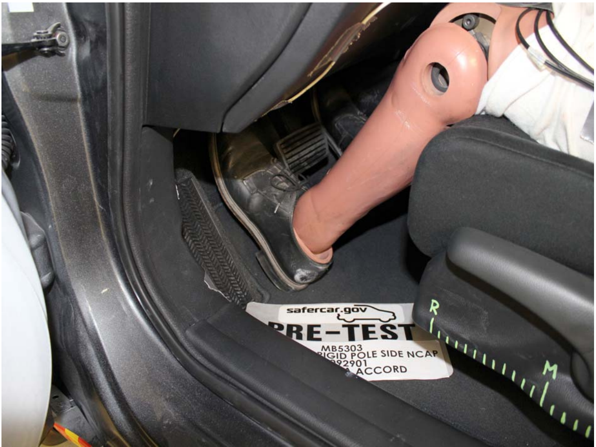
Pre-Test Placement of Dummy's Feet
