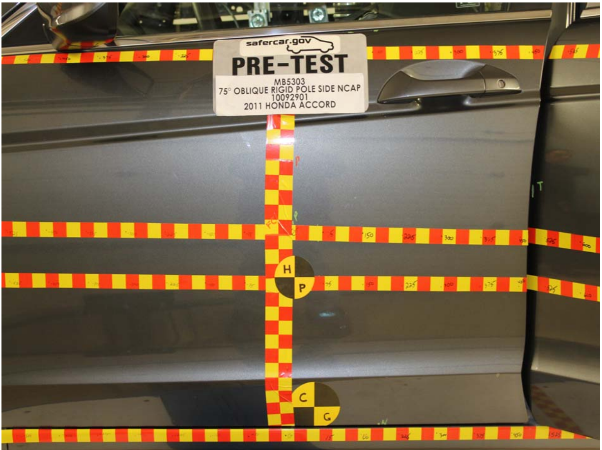
Pre-Test Close-Up View of Impact Point Target
