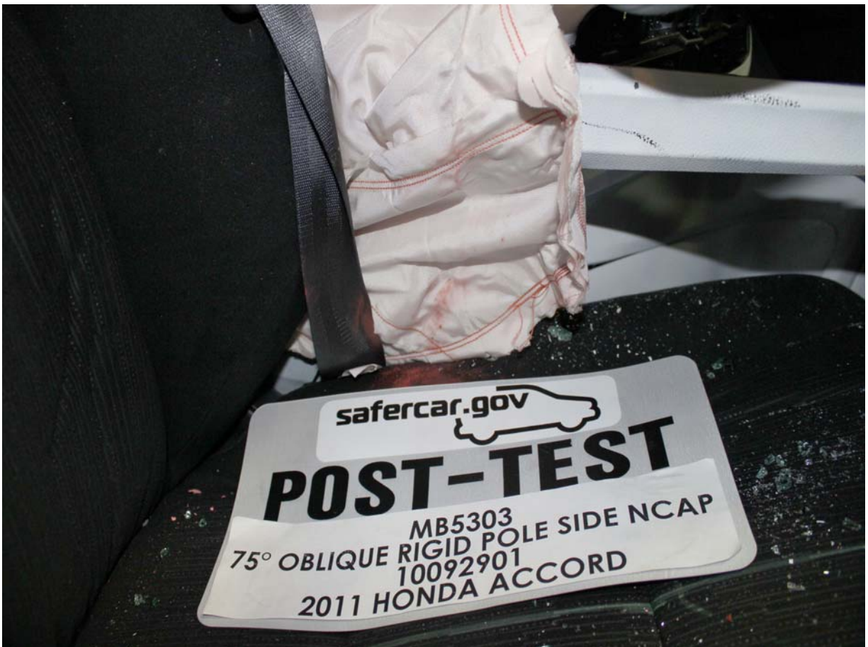
Post-Test Dummy Close-Up Pelvis Contact with Side Airbag View
