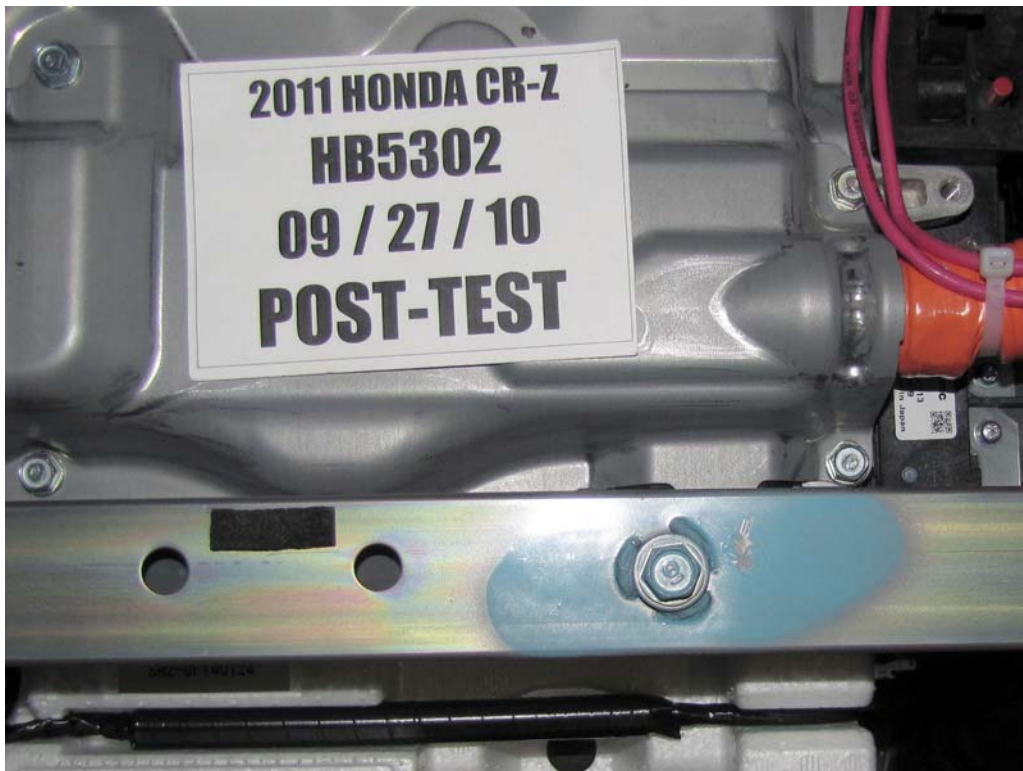
FIGURE 106. Post-Test Battery Mounting Hardware
