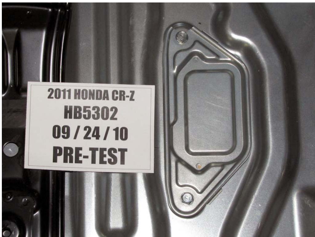
FIGURE 84. Pre-Test Propulsion Battery Disconnect
