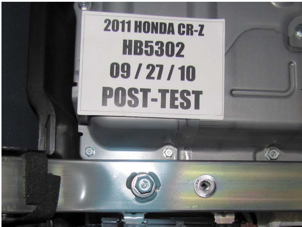
FIGURE 108. Post-Test Battery Mounting Hardware
