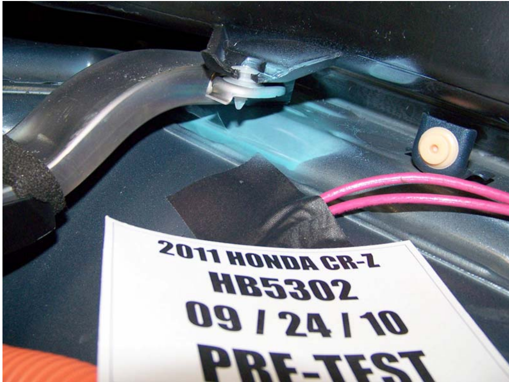
FIGURE 95. Pre-Test Battery Mounting Hardware
