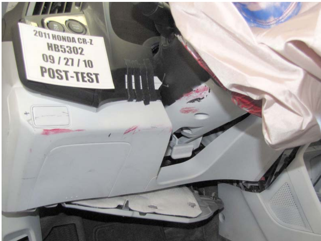
FIGURE 45. Post-Test View of Steering Column Shear Capsule
