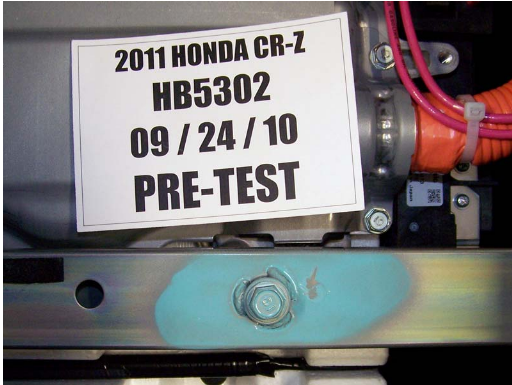
FIGURE 105. Pre-Test Battery Mounting Hardware
