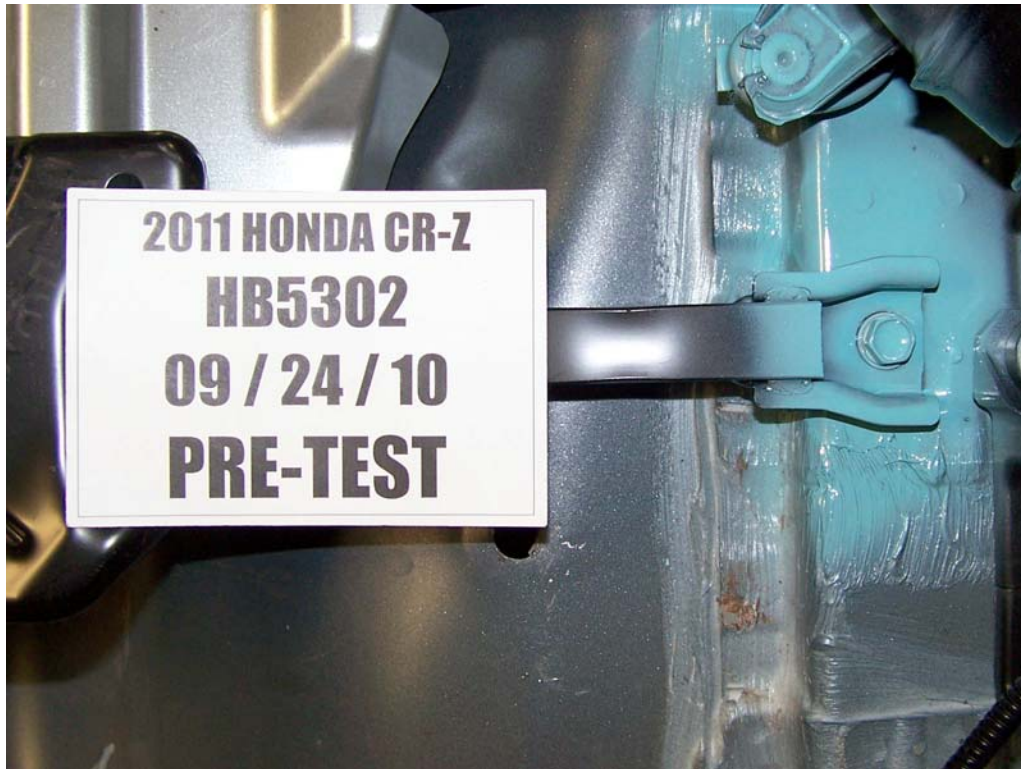
FIGURE 91. Pre-Test Battery Mounting Hardware
