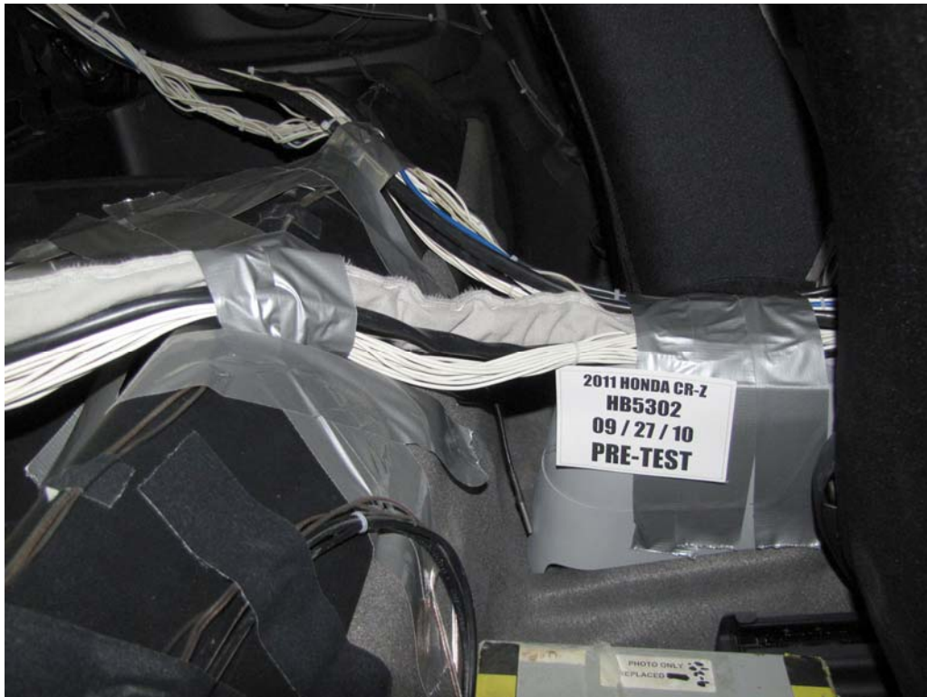
FIGURE 27. Pre-Test Dummy Cable Routing
