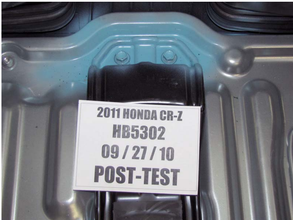
FIGURE 88. Post-Test Battery Mounting Hardware
