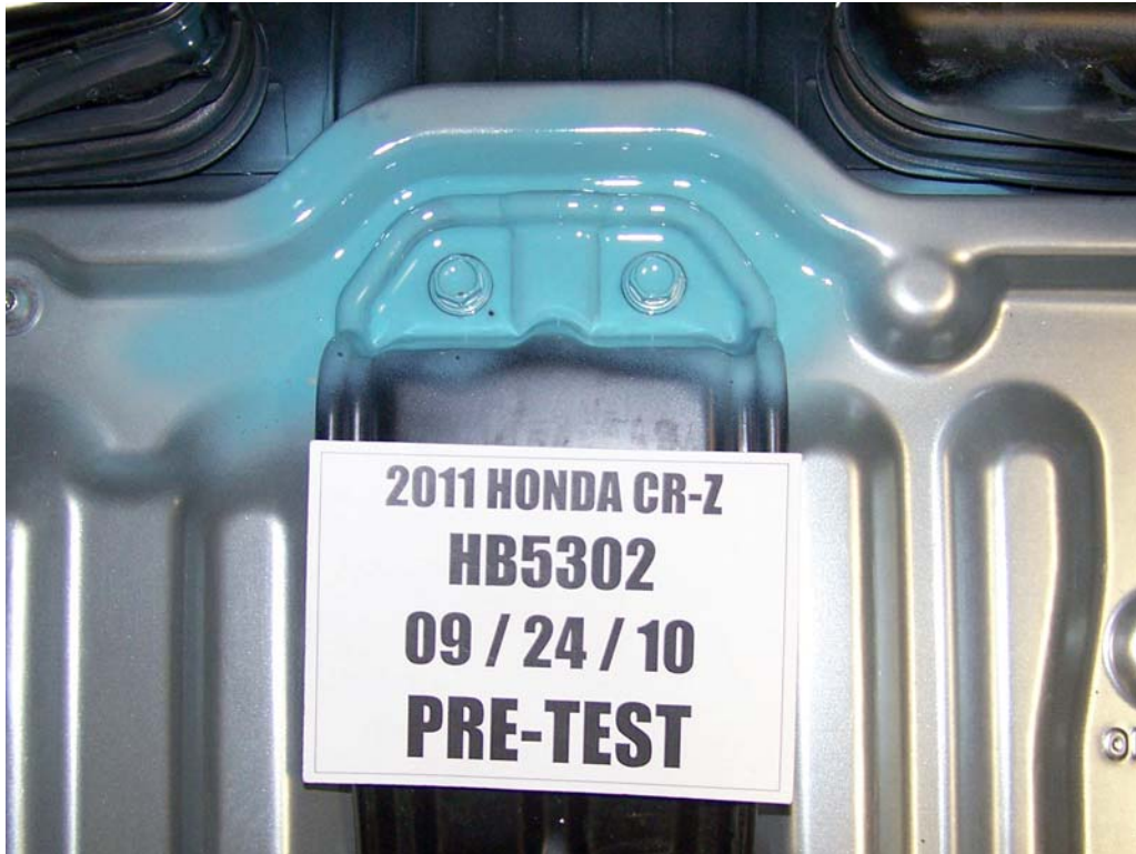
FIGURE 87. Pre-Test Battery Mounting Hardware
