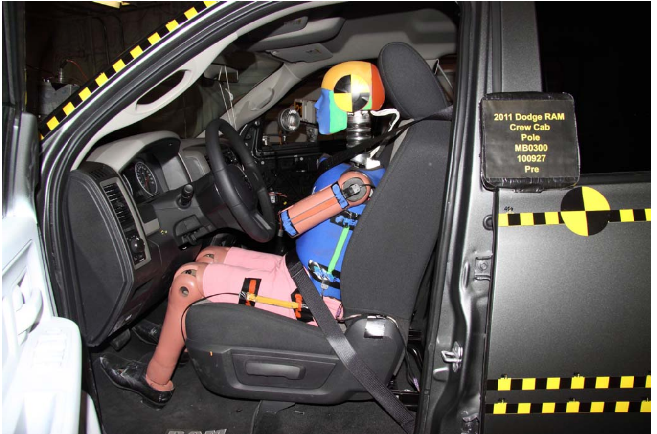
No. 023 – Pre-Test Left Side View of Dummy Showing Belt, Chalking, and Contact Switches
