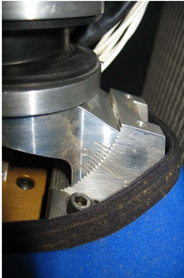
No. 030 – Pre-Test View of Dummy’s Neck Showing Position of Adjustable Neck Bracket
