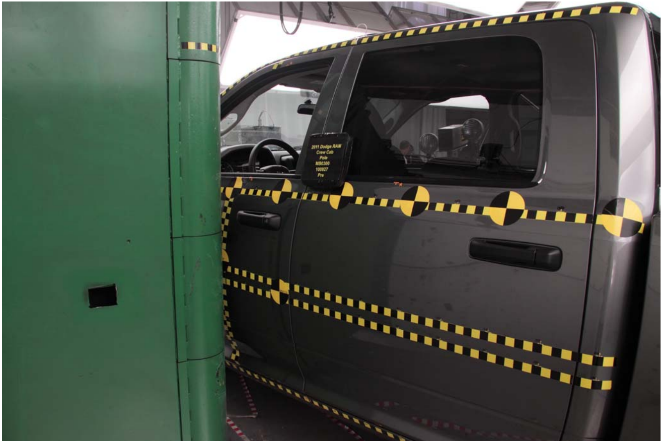
No. 017 – Pre-Test Left Side View of Pole Positioned Against Side of Vehicle at Impact Point
