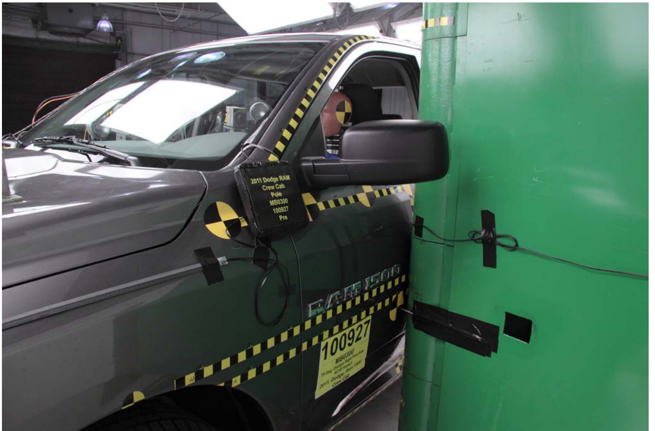
No. 018 – Pre-Test Right Side View of Pole Positioned Against Side of Vehicle at Impact Point
