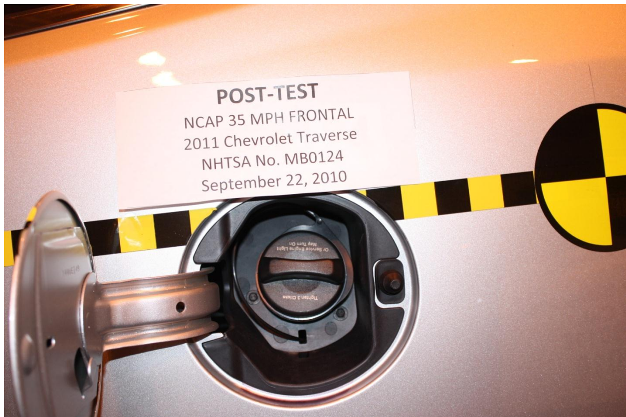
Figure A-22: Post-Test Fuel Filler Cap View
