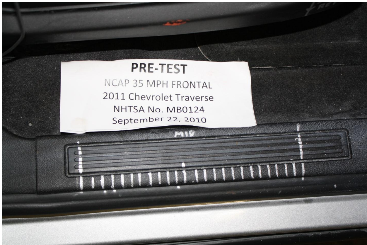
Figure A-52: Pre-Test Passenger's Seat Fore-Aft Markings
