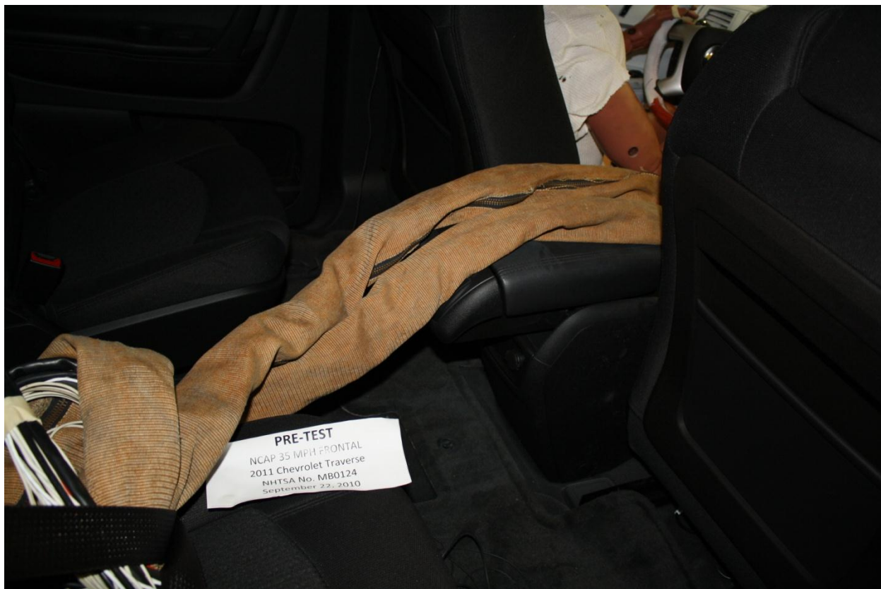
Figure A-27: Pre-Test Dummy Cable Routing
