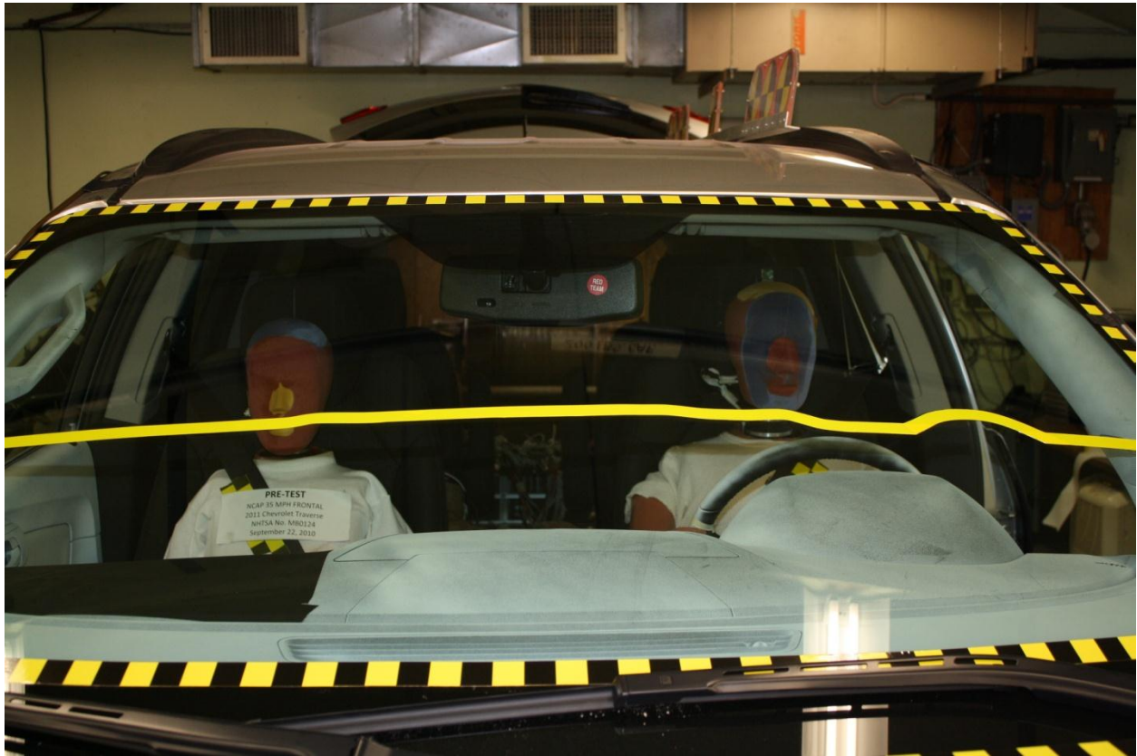
Figure A-17: Pre-Test Windshield View
