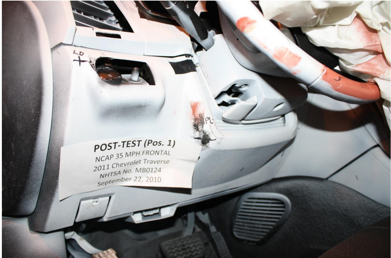
Figure A-40: Post-Test Driver's Side Knee Bolster
