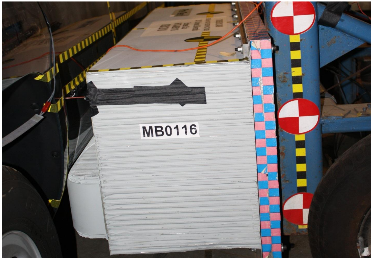
Figure A-17: Pre-Test Left Side View of MDB Positioned Against Side of Test Vehicle
