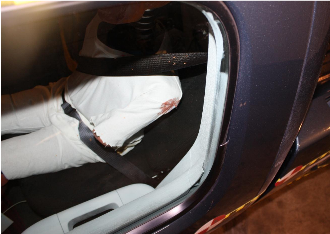
Figure A-67: Pre-Test Passenger Dummy and Door Clearance View
