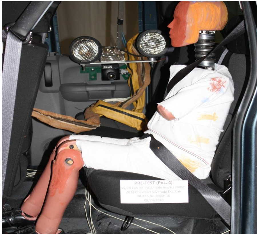
Figure A-53: Pre-test Left Side View of Passenger Dummy Showing Belt, Chalking, and Contact Switches
