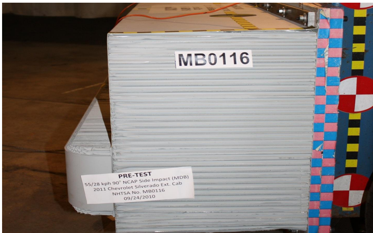
Figure A-85: Pre-Test Left Side View of MDB Impactor Face
