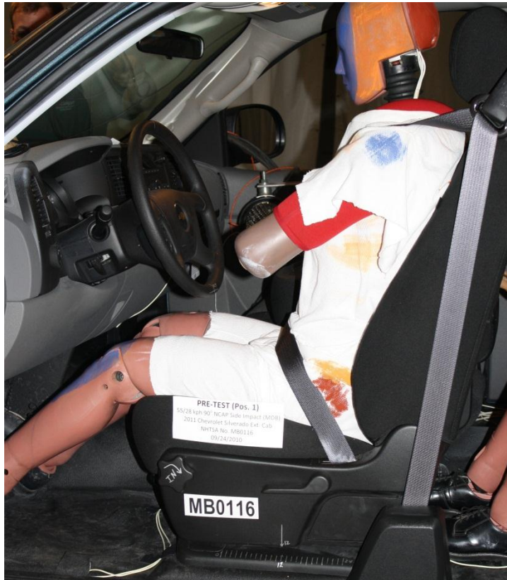
Figure A-27: Pre-Test Left Side View of Driver Dummy Showing Belt, Chalking, and Contact Switches
