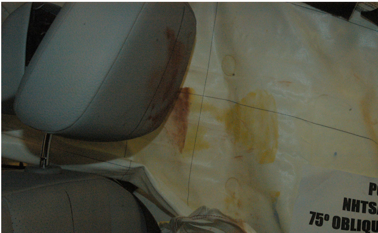
Figure 046 Post-test dummy close-up head contact with side airbag view
