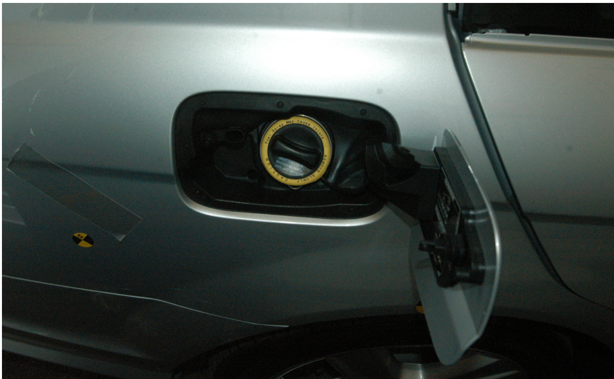
Figure 052: Post-test view of fuel filler cap/neck
