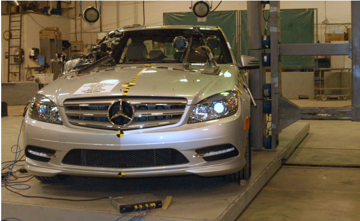
Figure 017: Pre-test left side view of pole positioned against side of vehicle at impact point
