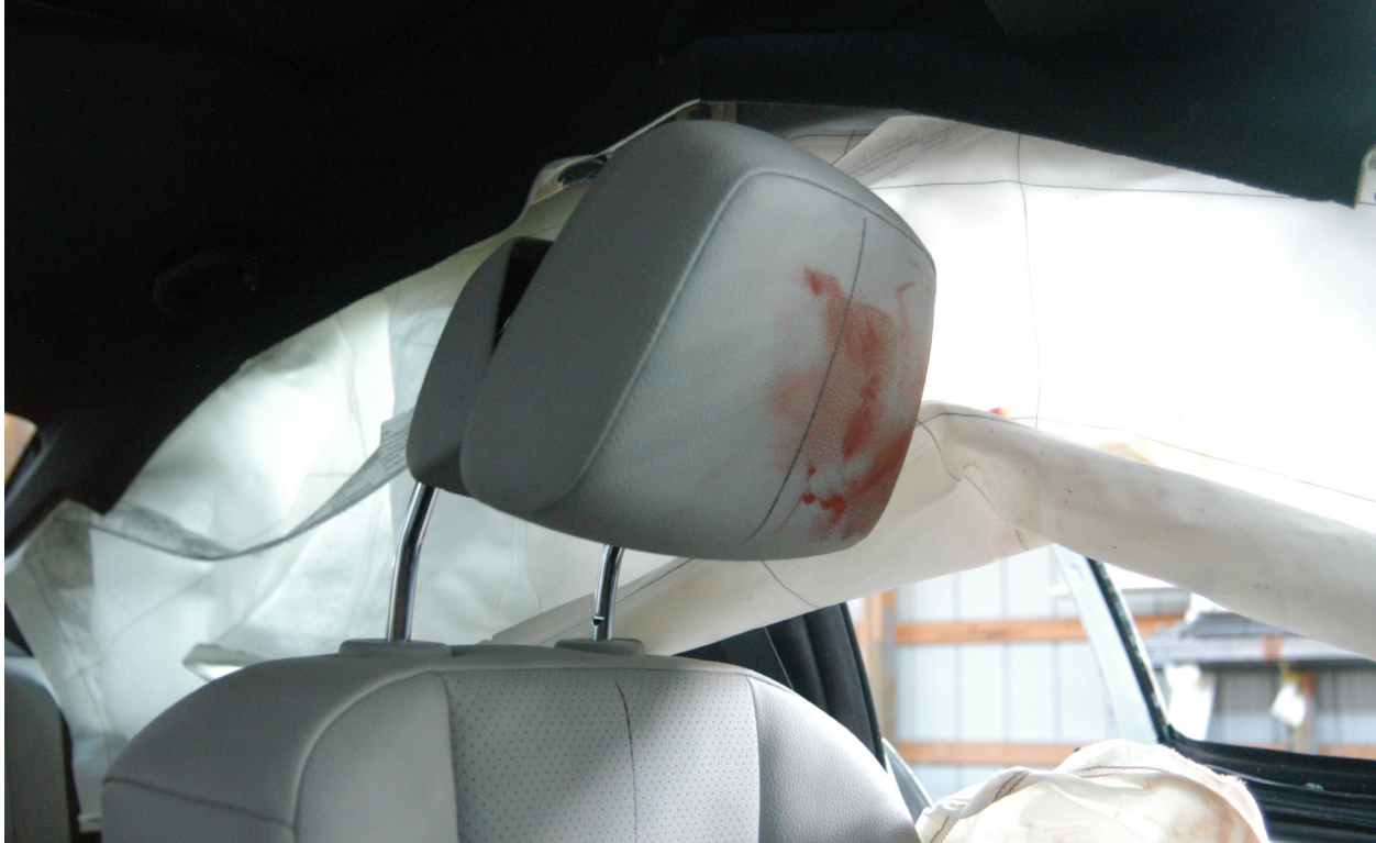
Figure 045: Post-test dummy close-up head contact with vehicle view
