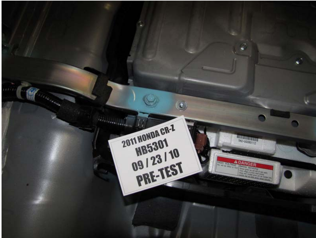
FIGURE 136. Pre-Test Battery Mounting Hardware
