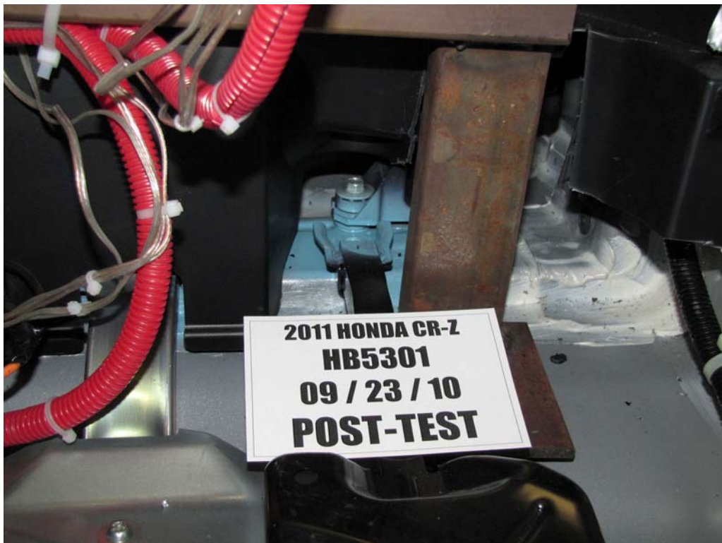
FIGURE 123. Post-Test Battery Mounting Hardware
