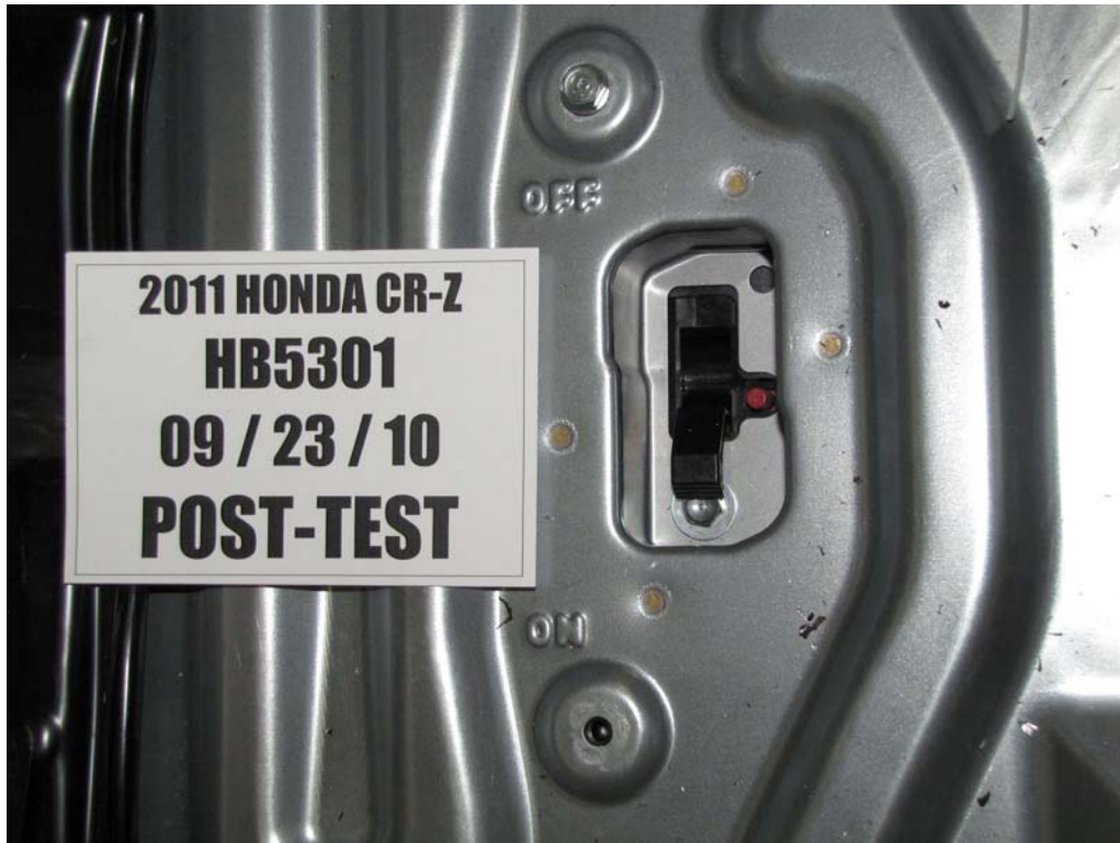
FIGURE 116. Post-Test Propulsion Battery Disconnect
