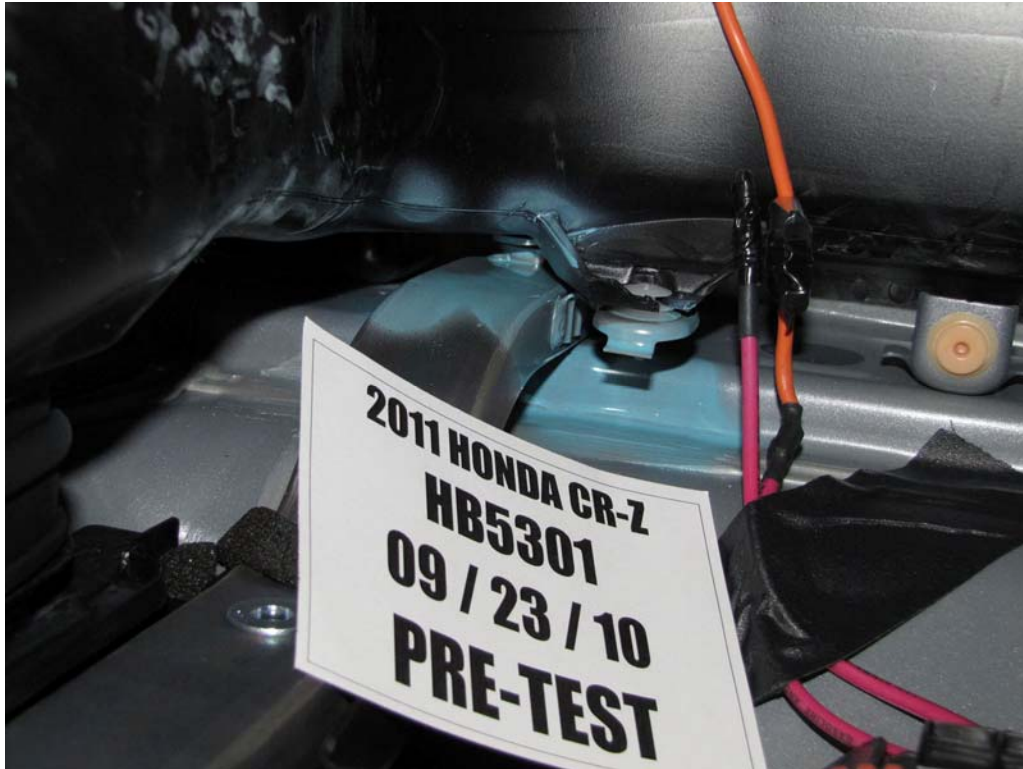
FIGURE 126. Pre-Test Battery Mounting Hardware
