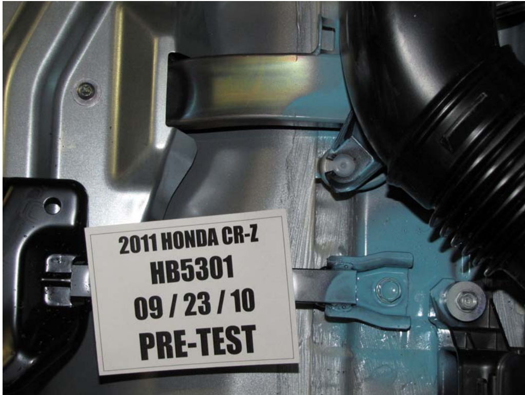
FIGURE 122. Pre-Test Battery Mounting Hardware
