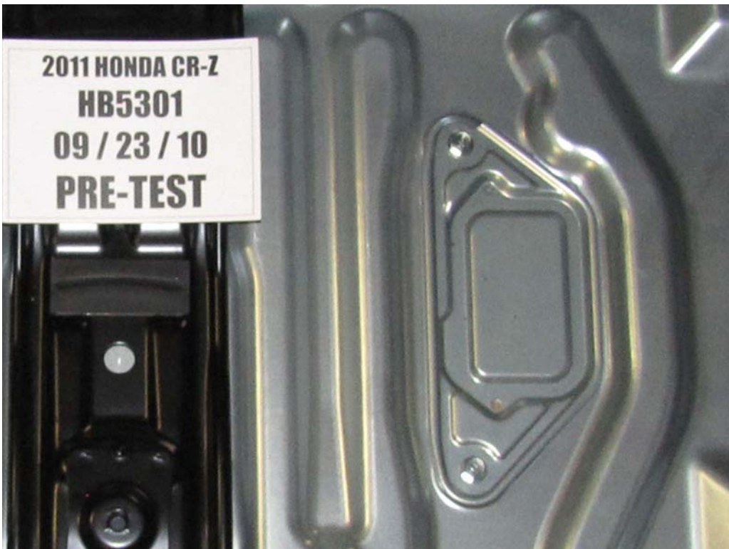
FIGURE 113. Pre-Test Propulsion Battery Disconnect
