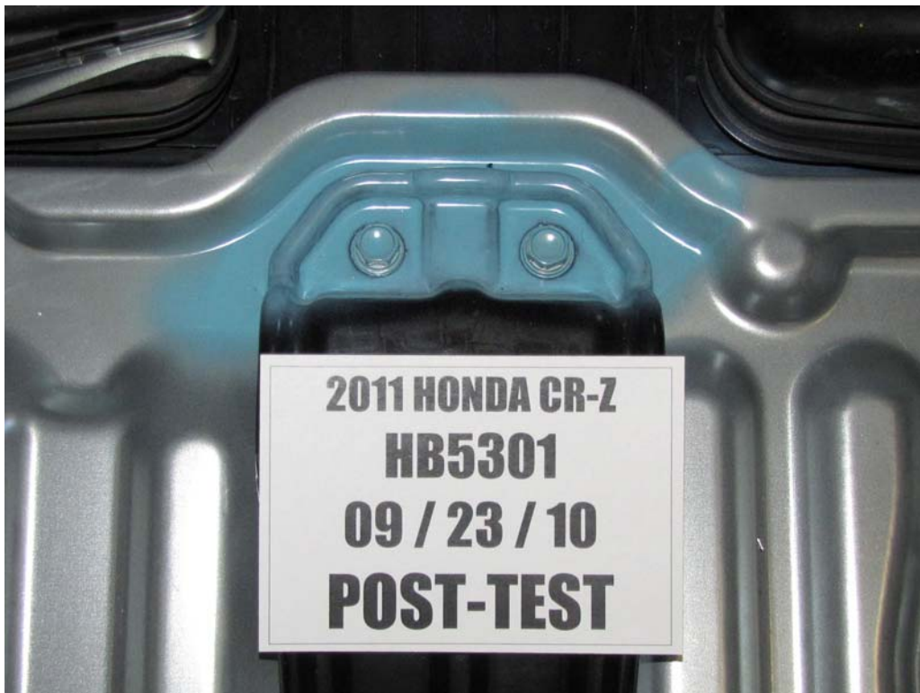
FIGURE 119. Post-Test Battery Mounting Hardware
