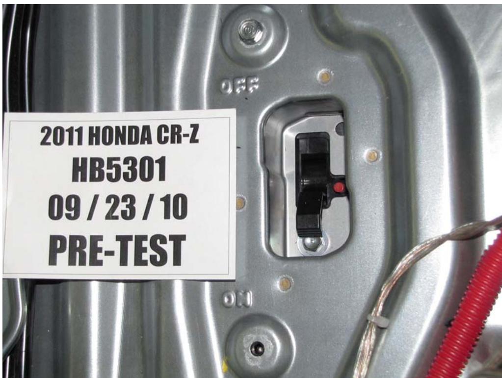
FIGURE 115. Pre-Test Propulsion Battery Disconnect
