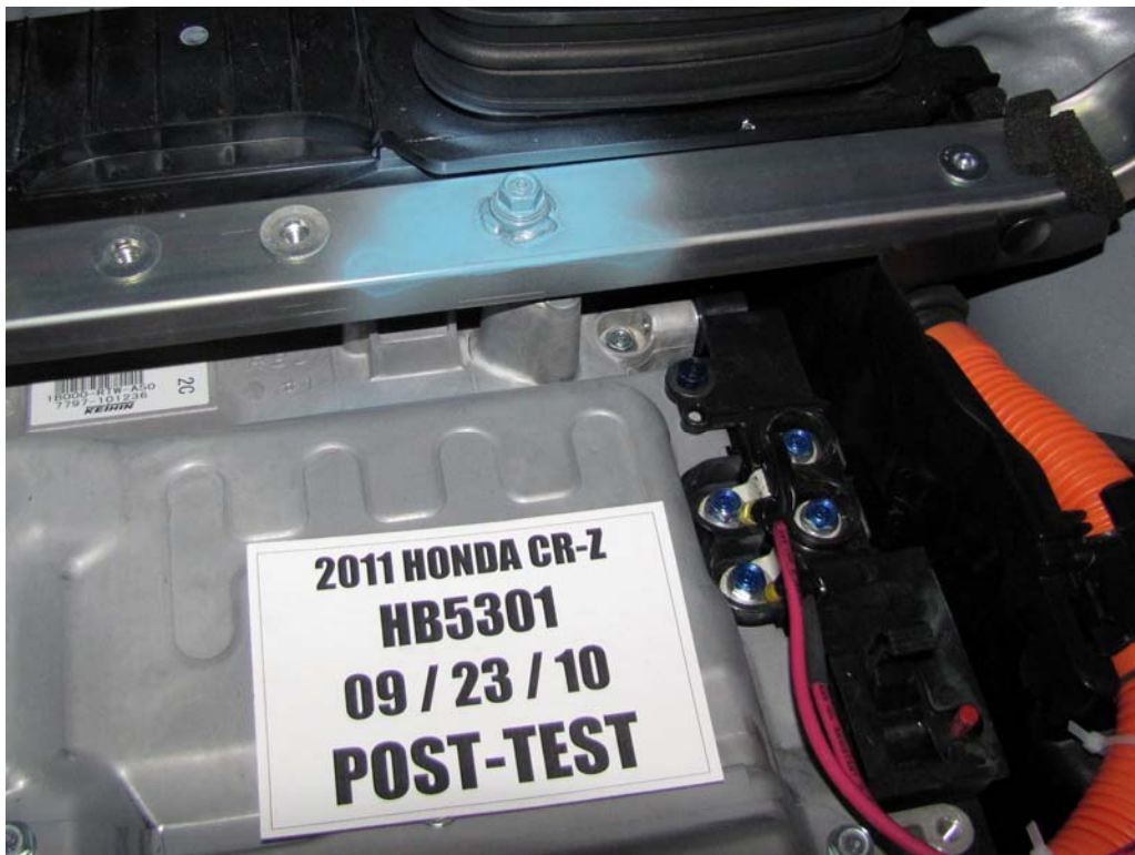
FIGURE 135. Post-Test Battery Mounting Hardware
