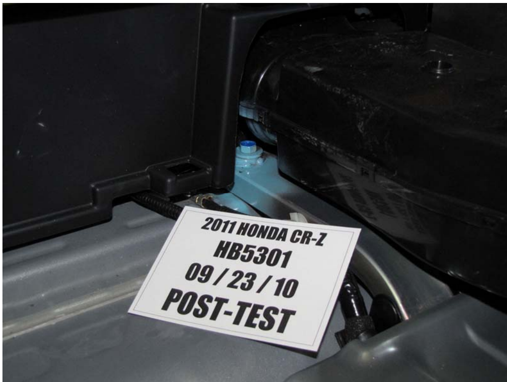
FIGURE 125. Post-Test Battery Mounting Hardware
