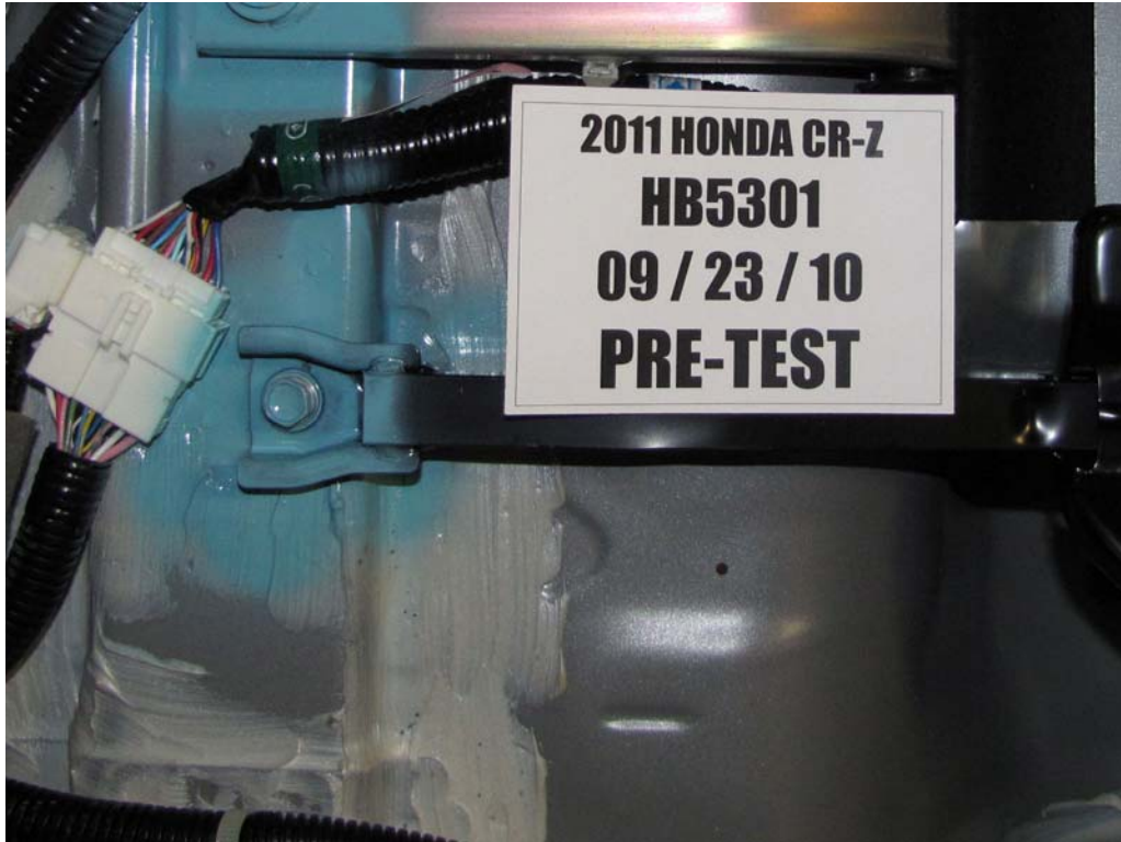
FIGURE 120. Pre-Test Battery Mounting Hardware
