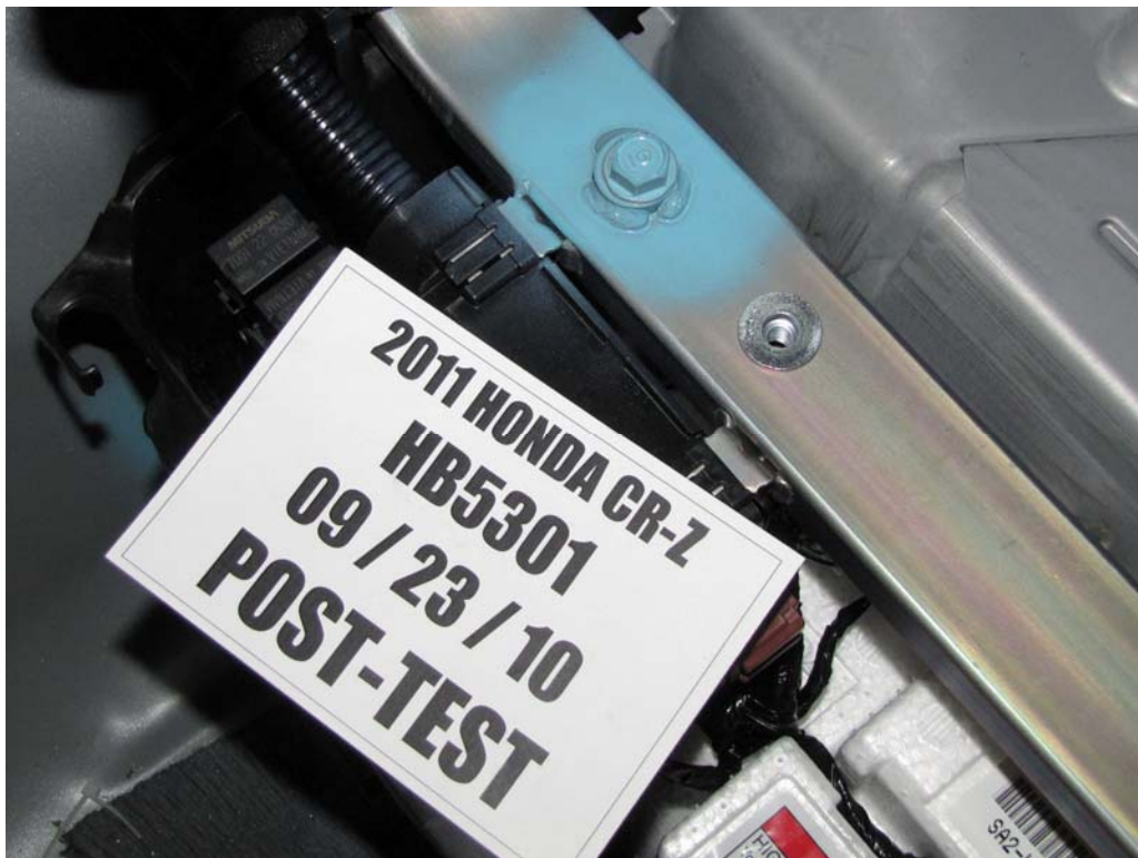
FIGURE 137. Post-Test Battery Mounting Hardware
