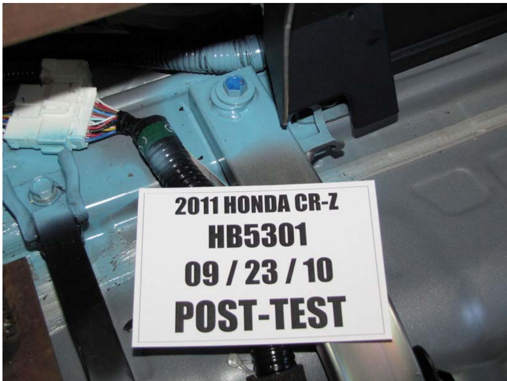
FIGURE 129. Post-Test Battery Mounting Hardware
