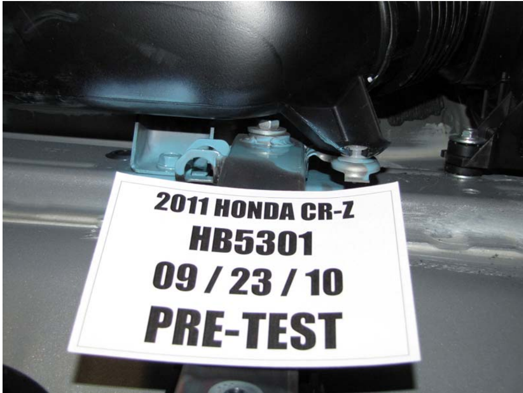
FIGURE 130. Pre-Test Battery Mounting Hardware
