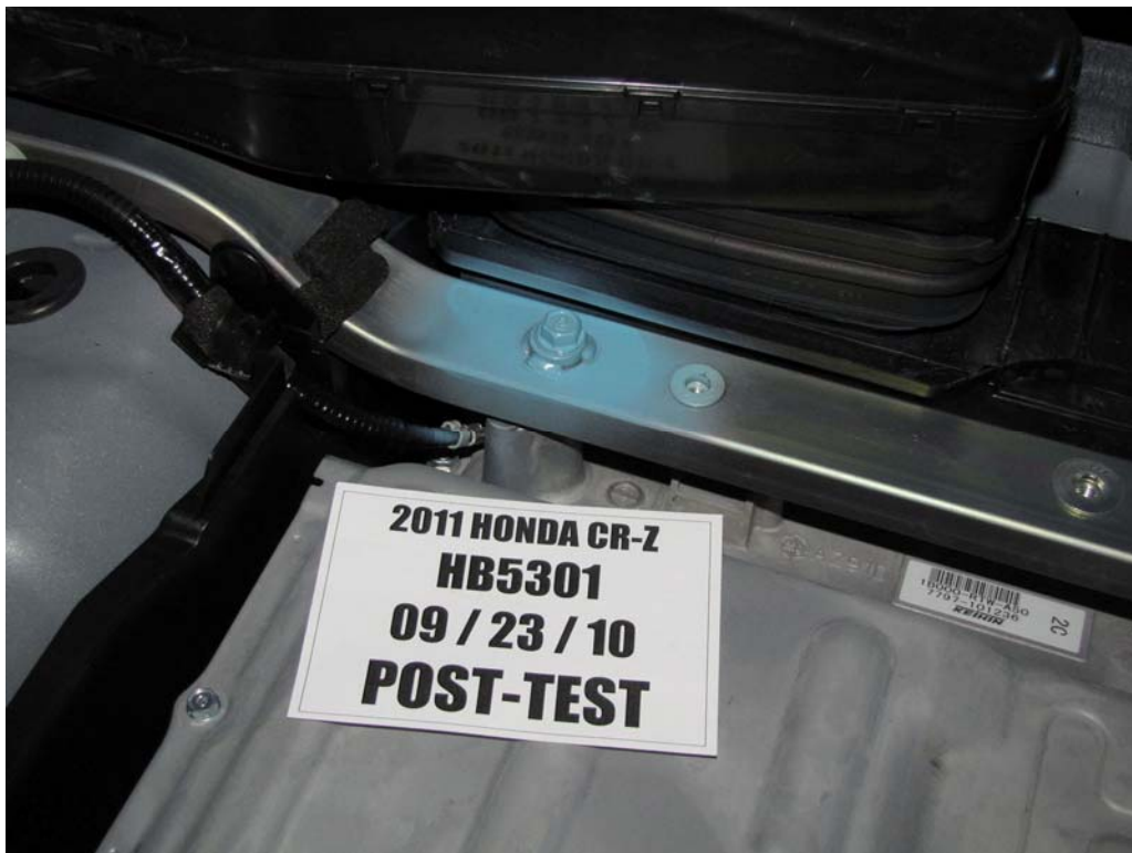
FIGURE 133. Post-Test Battery Mounting Hardware
