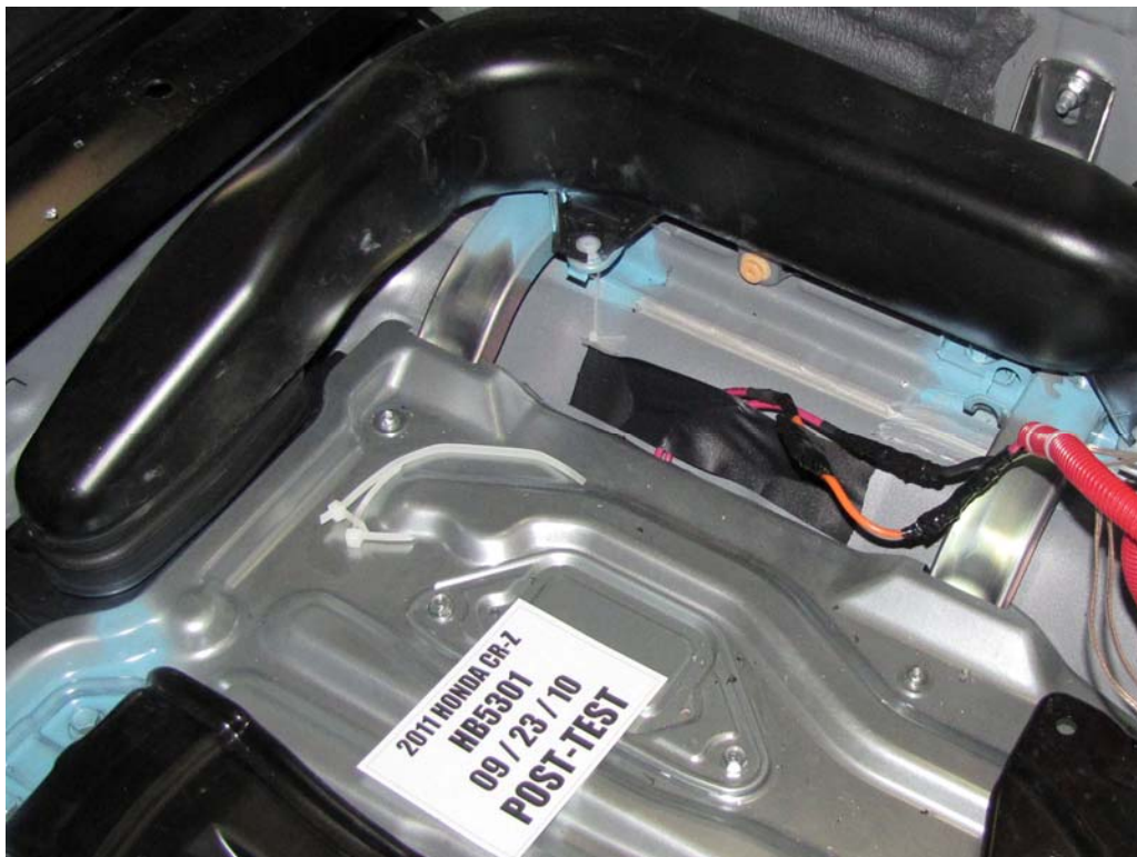
FIGURE 127. Post-Test Battery Mounting Hardware
