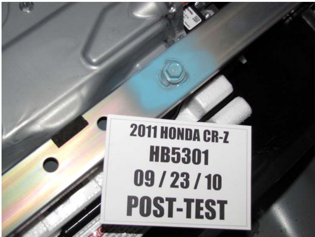
FIGURE 139. Post-Test Battery Mounting Hardware
