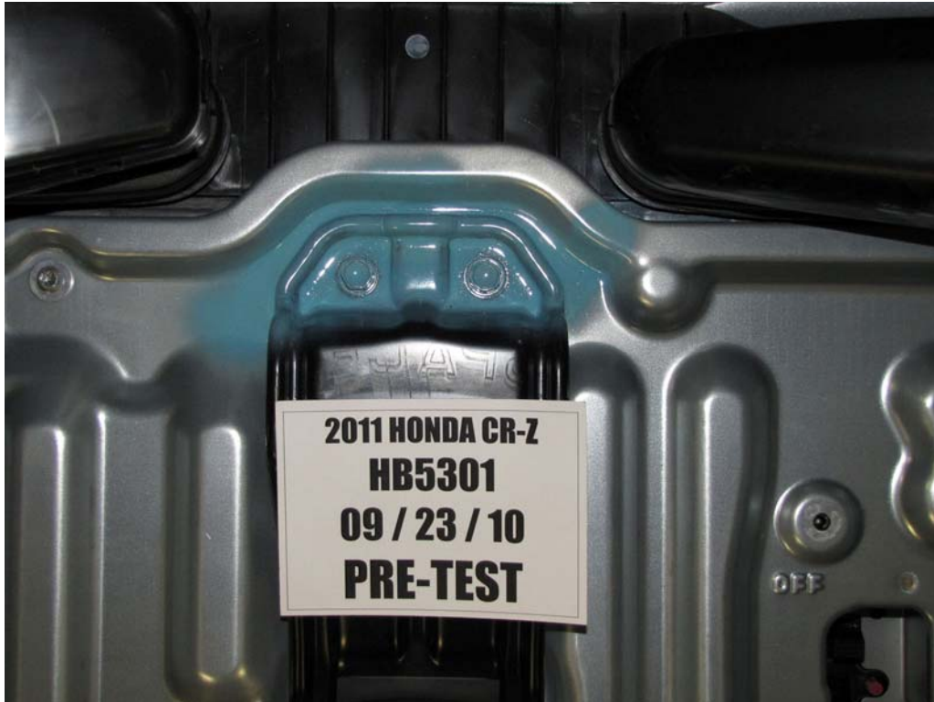
FIGURE 118. Pre-Test Battery Mounting Hardware
