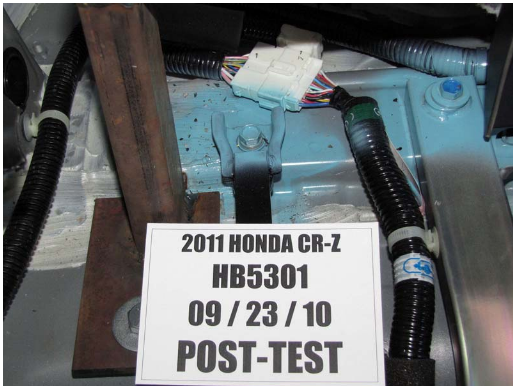
FIGURE 121. Post-Test Battery Mounting Hardware
