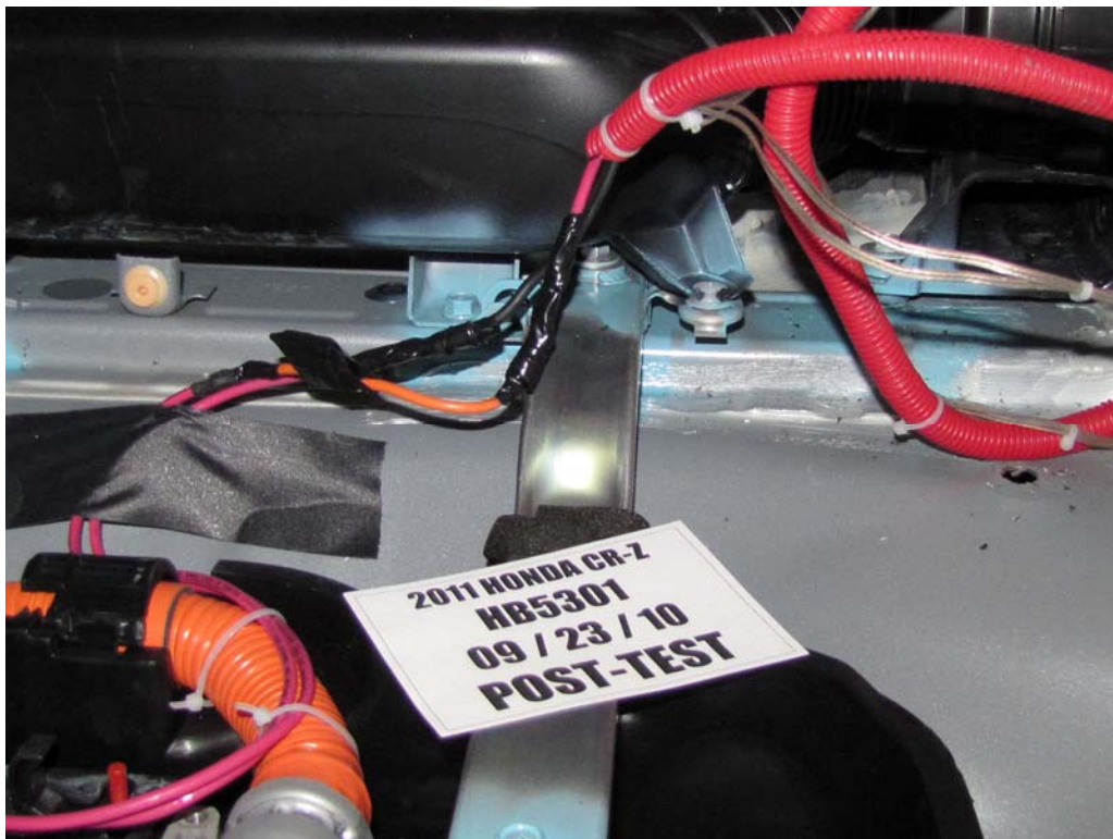
FIGURE 131. Post-Test Battery Mounting Hardware
