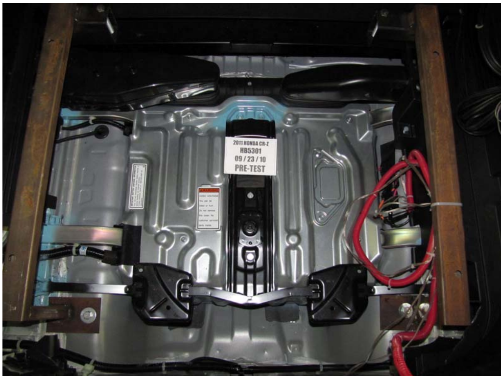
FIGURE 109. Pre-Test Battery Compartment
