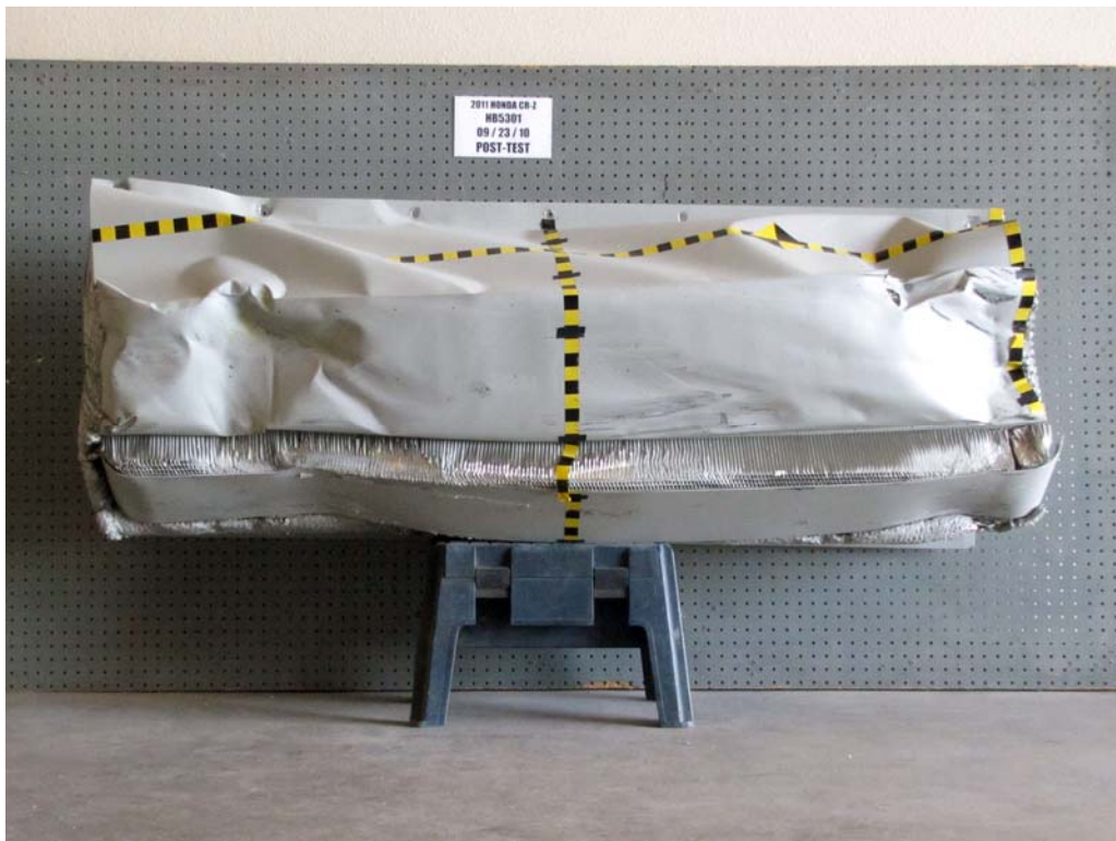
FIGURE 82. Post-Test Front View of MDB Impactor Face
