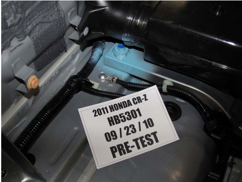
FIGURE 124. Pre-Test Battery Mounting Hardware
