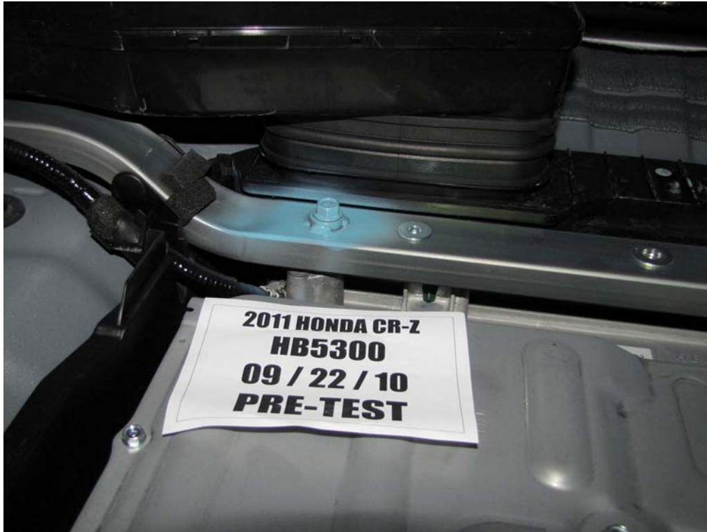
FIGURE 99. Pre-Test Battery Mounting Hardware
