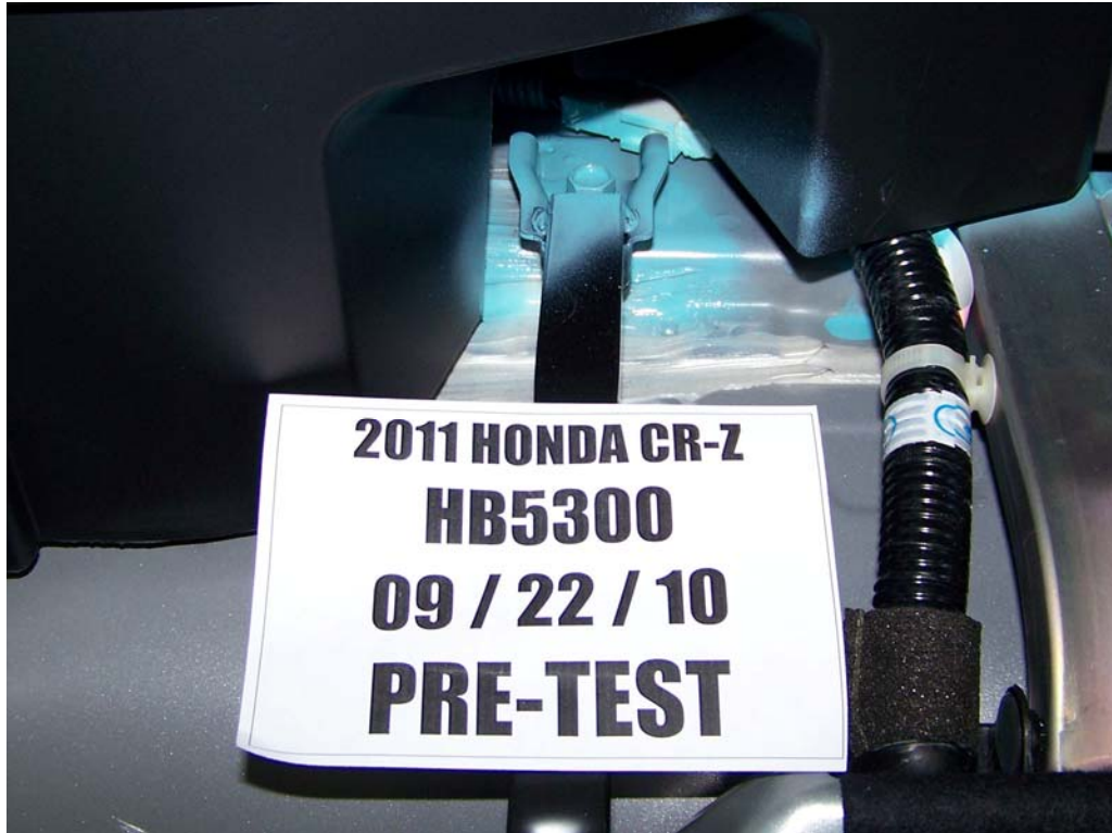
FIGURE 87. Pre-Test Battery Mounting Hardware
