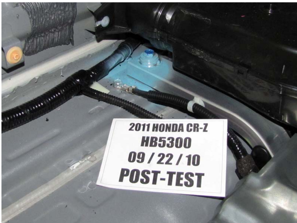
FIGURE 92. Post-Test Battery Mounting Hardware
