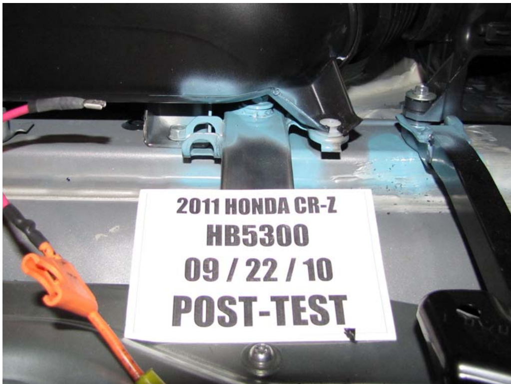
FIGURE 98. Post-Test Battery Mounting Hardware
