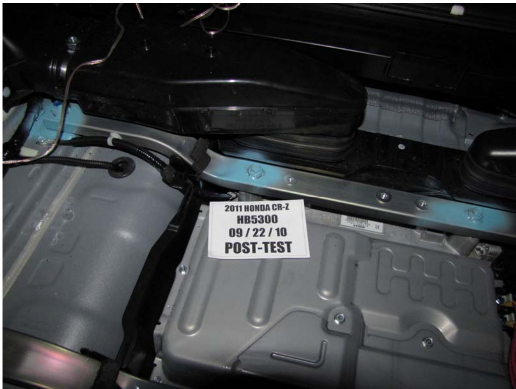
FIGURE 100. Post-Test Battery Mounting Hardware
