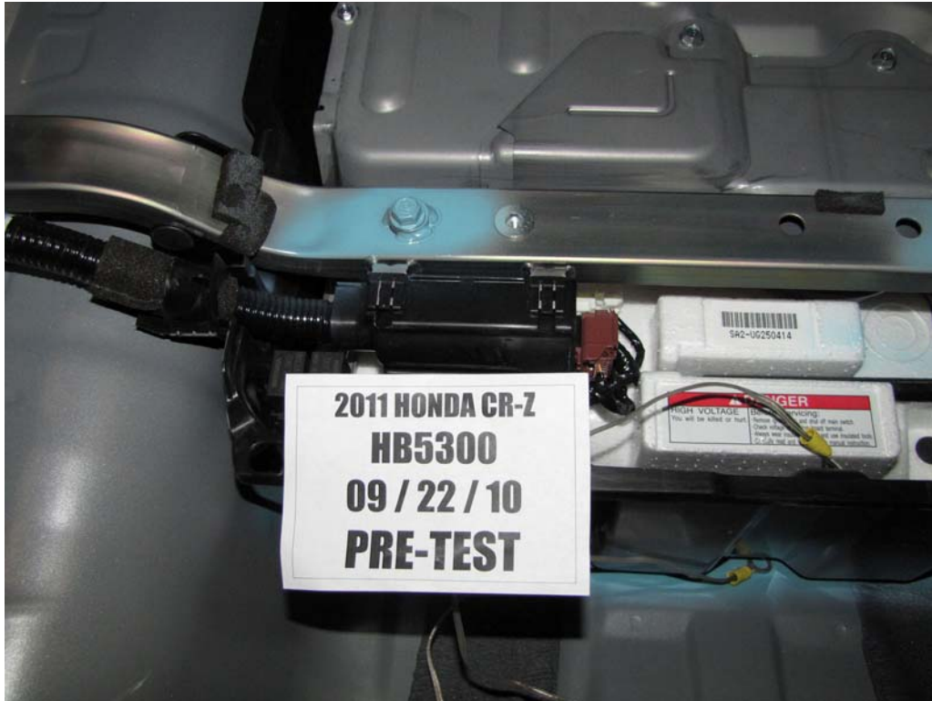
FIGURE 103. Pre-Test Battery Mounting Hardware
