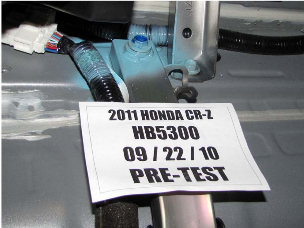
FIGURE 95. Pre-Test Battery Mounting Hardware
