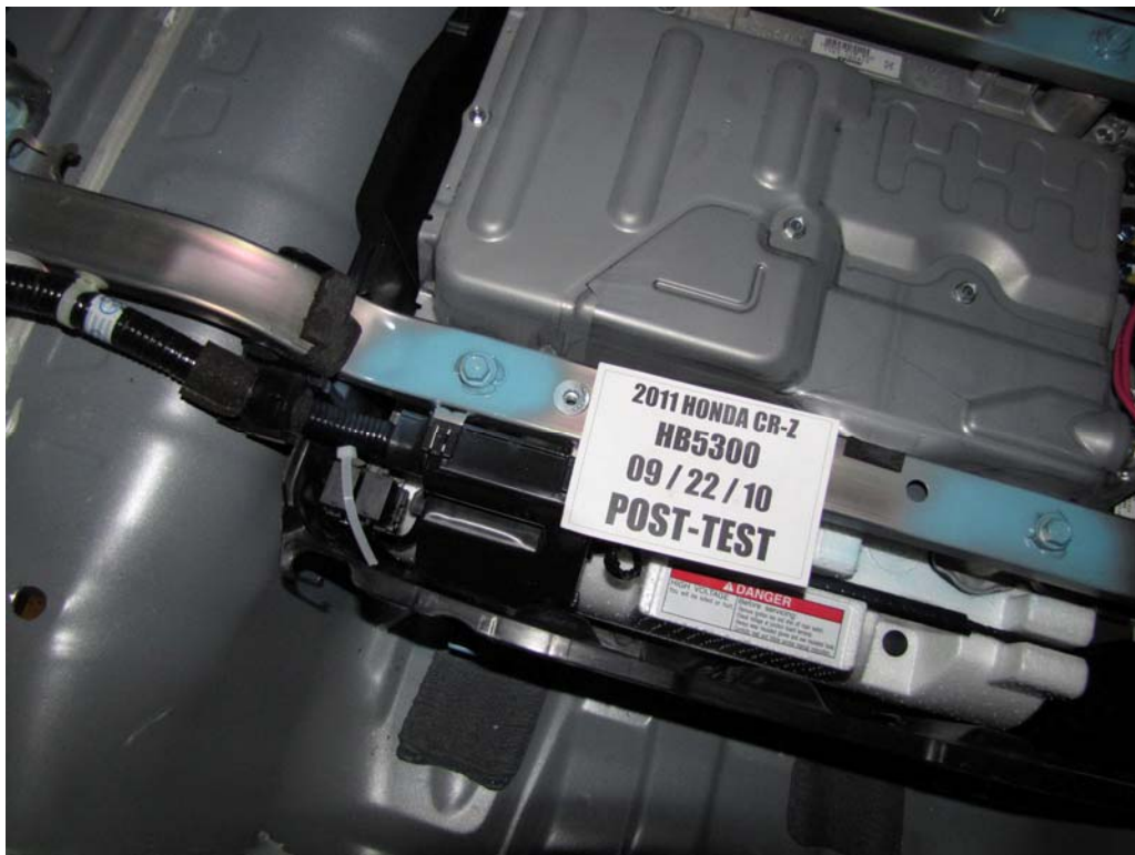
FIGURE 104. Post-Test Battery Mounting Hardware
