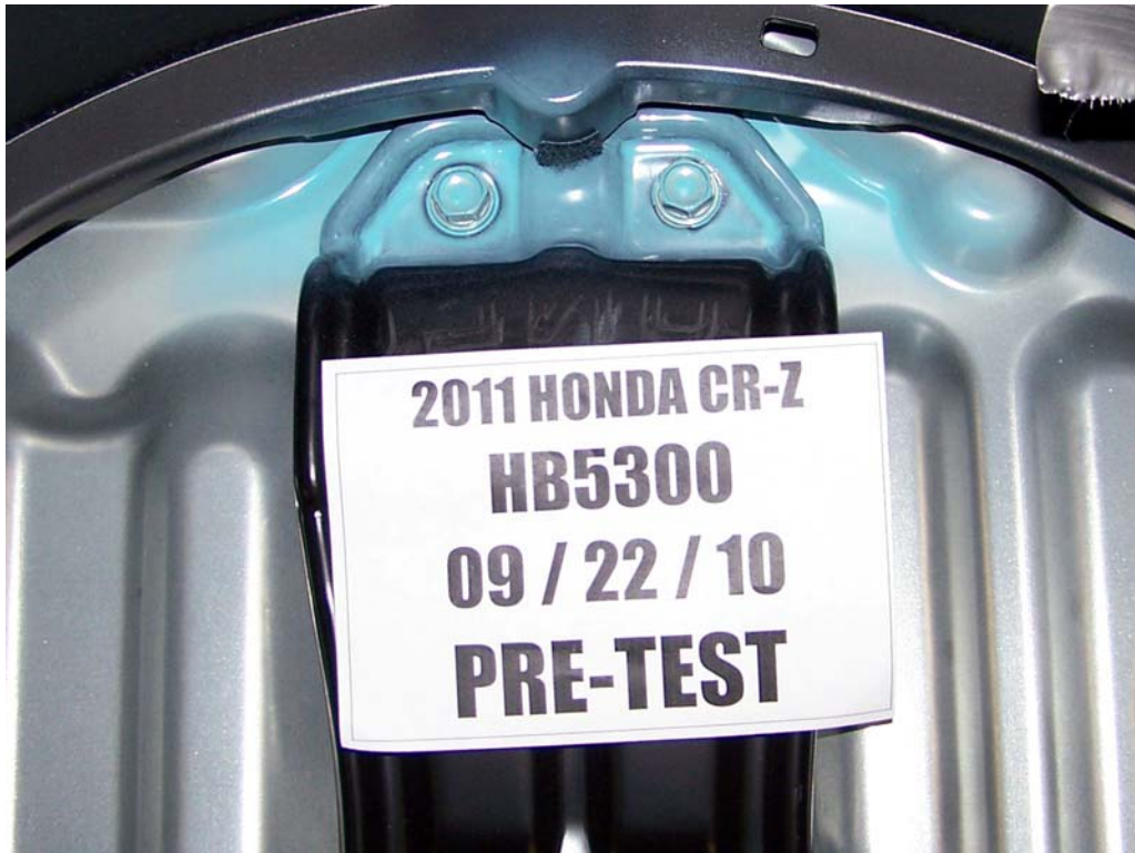
FIGURE 85. Pre-Test Battery Mounting Hardware
