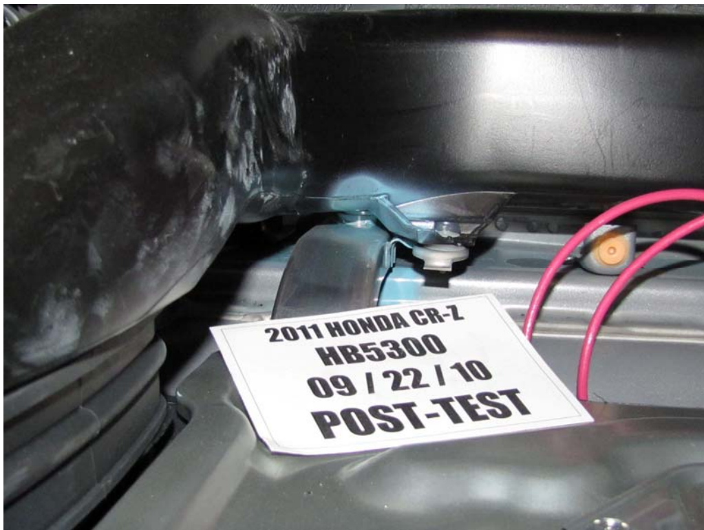
FIGURE 94. Post-Test Battery Mounting Hardware
