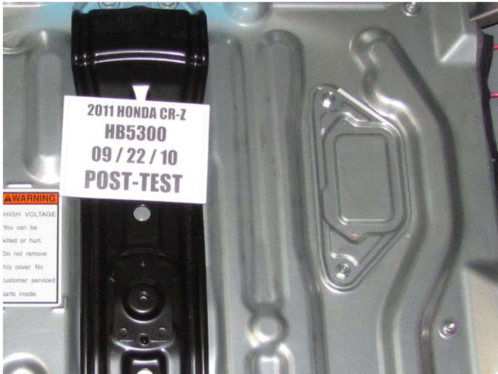
FIGURE 81. Post-Test Propulsion Battery Disconnect
