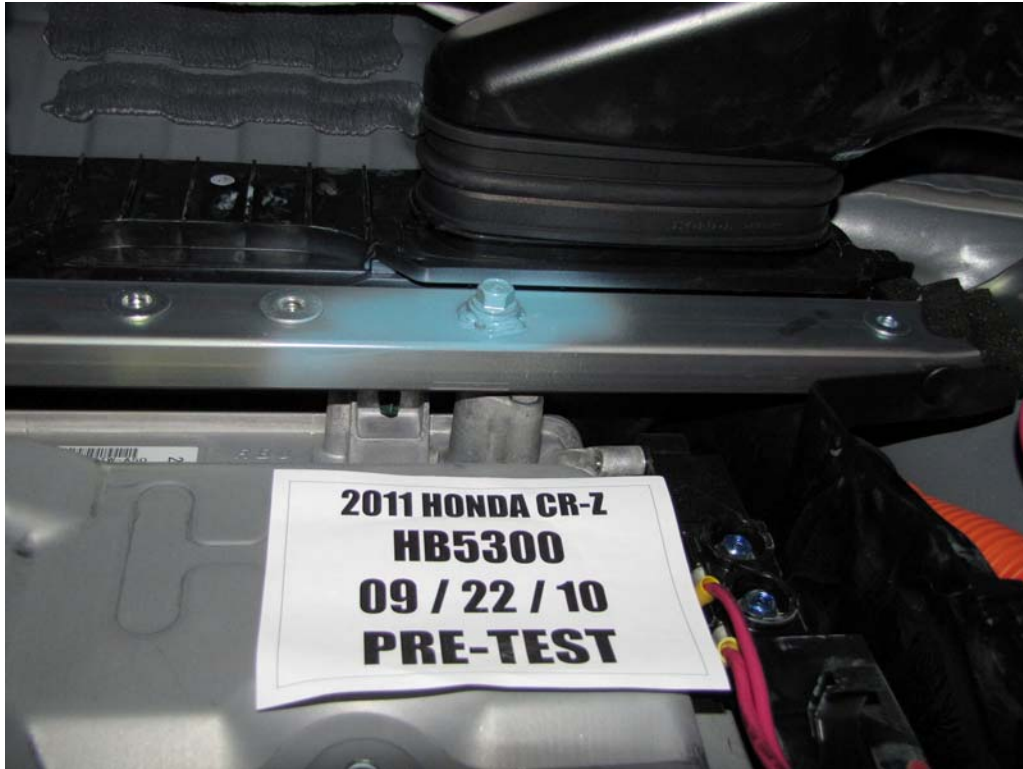
FIGURE 101. Pre-Test Battery Mounting Hardware
