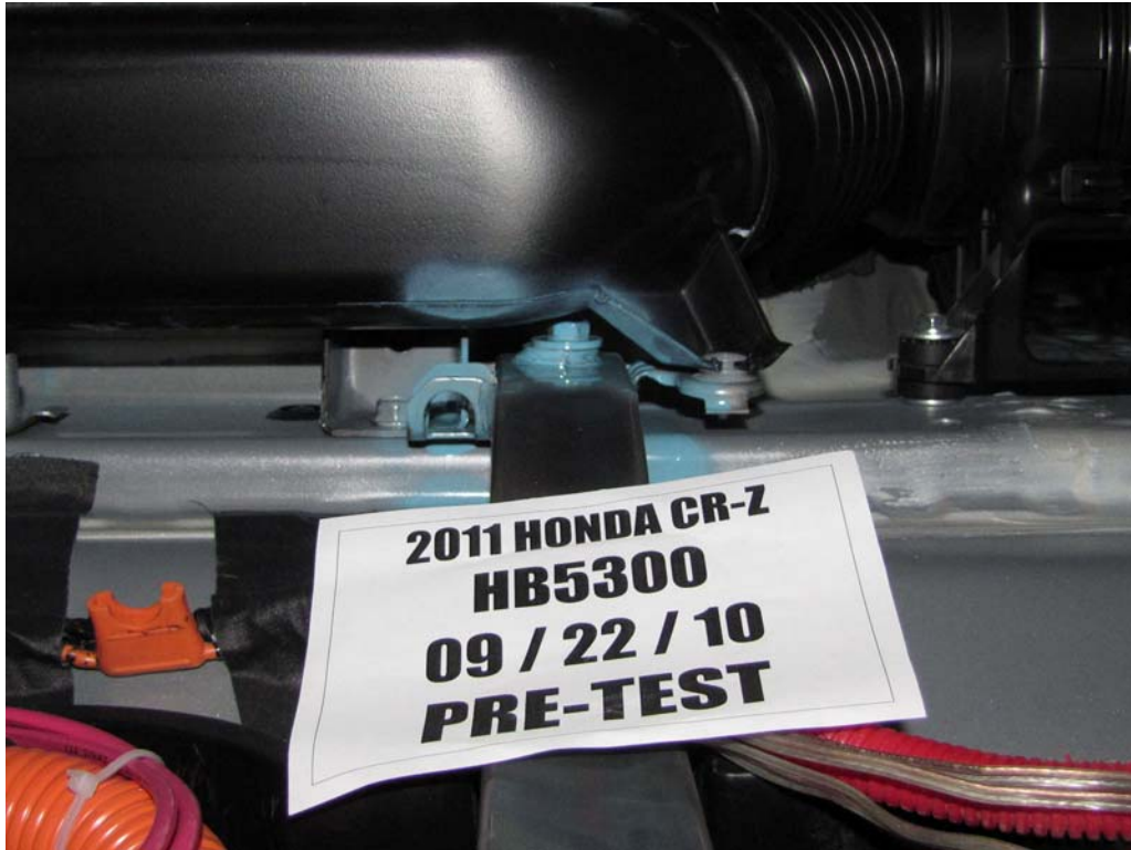
FIGURE 97. Pre-Test Battery Mounting Hardware
