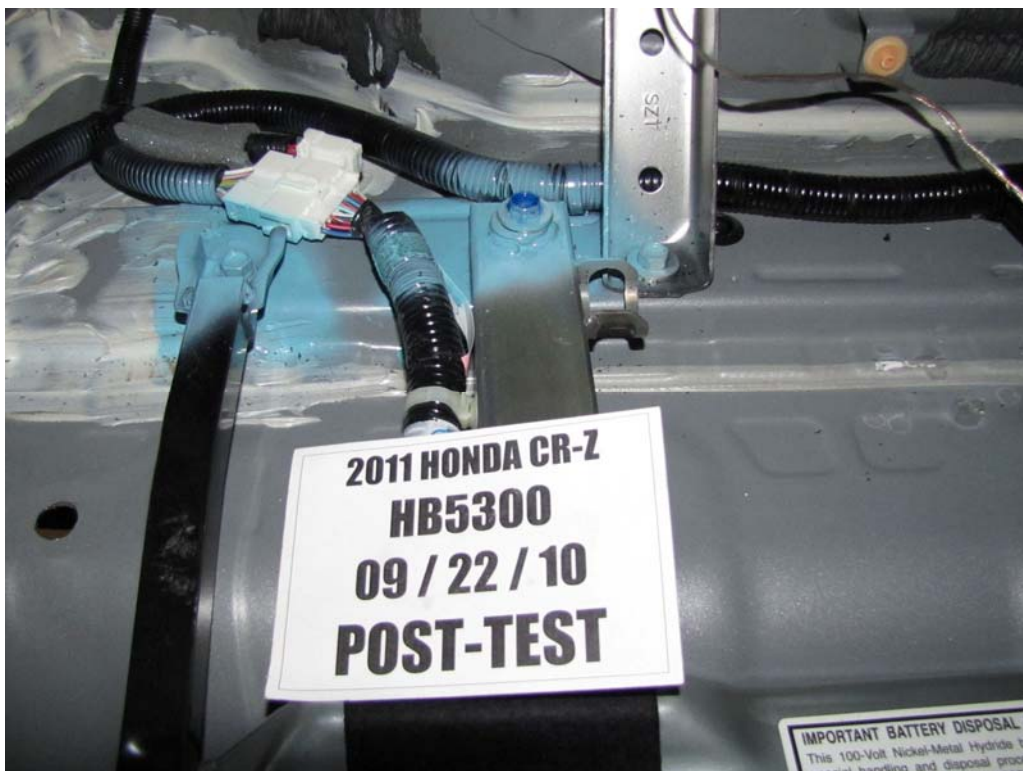
FIGURE 96. Post-Test Battery Mounting Hardware
