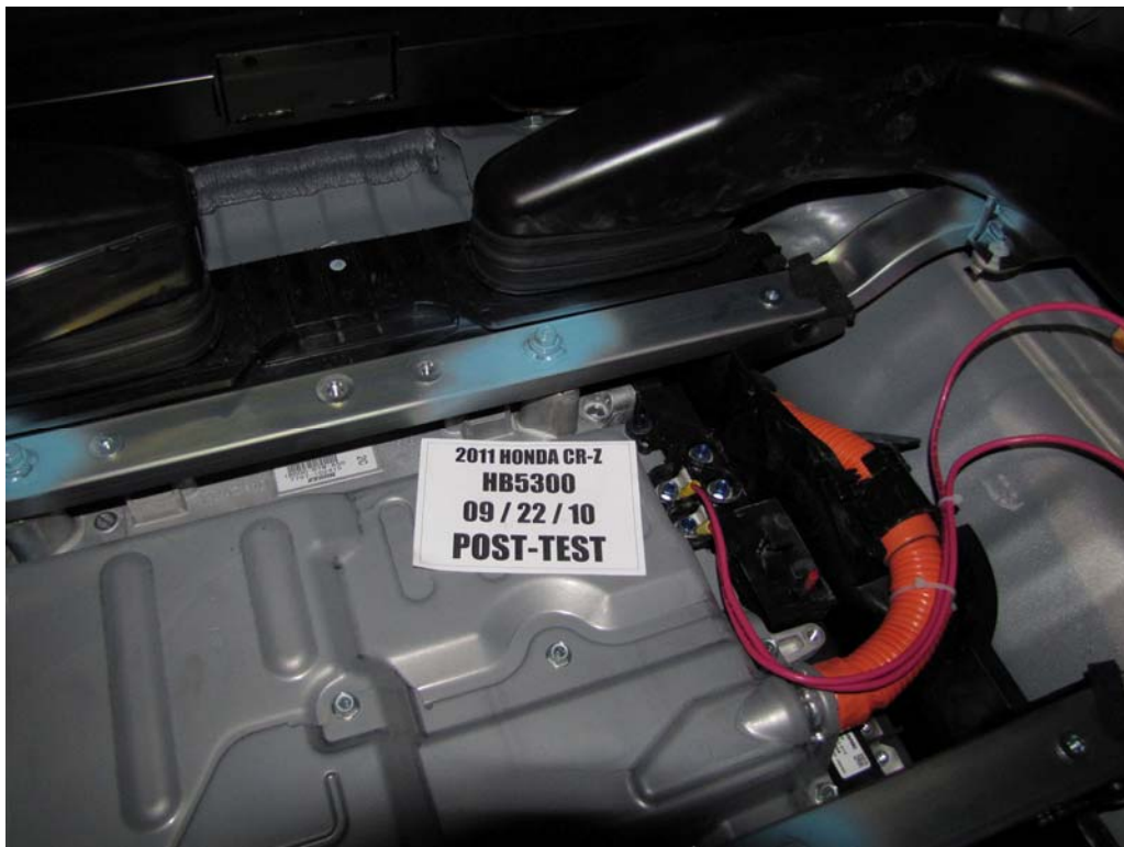
FIGURE 102. Post-Test Battery Mounting Hardware
