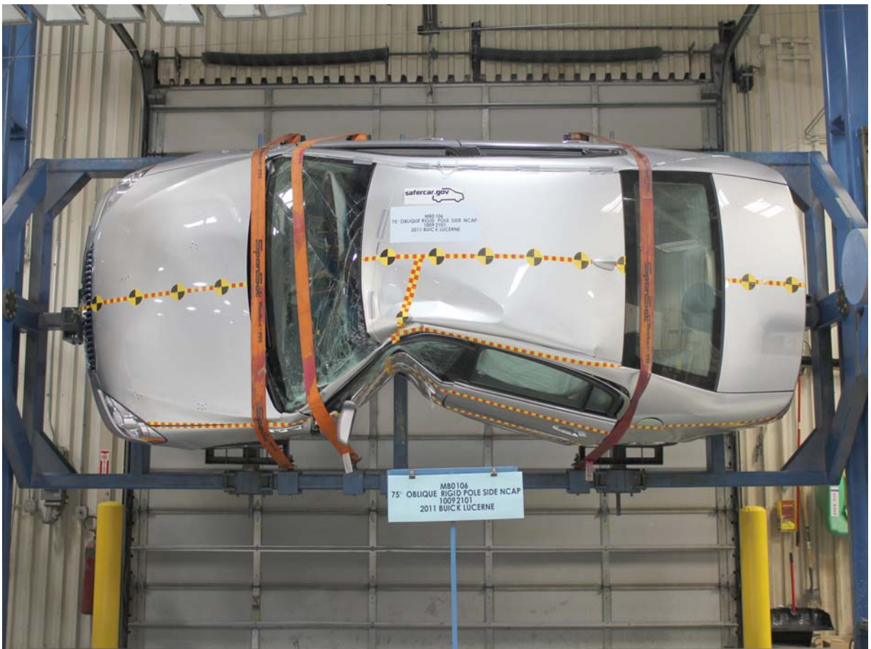
FMVSS No. 301/305 Rollover 90 Degrees
