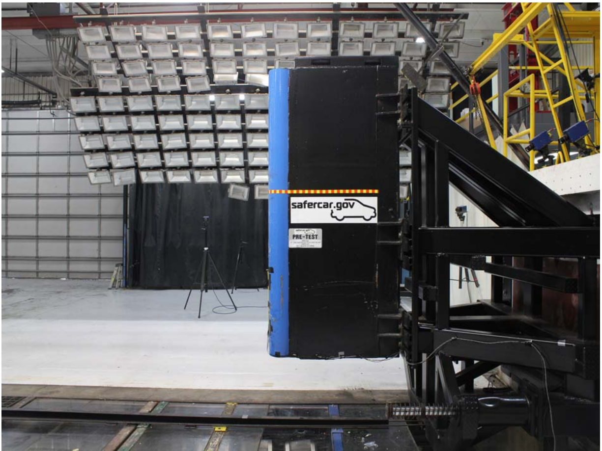
Pre-Test Pole Barrier Side View
