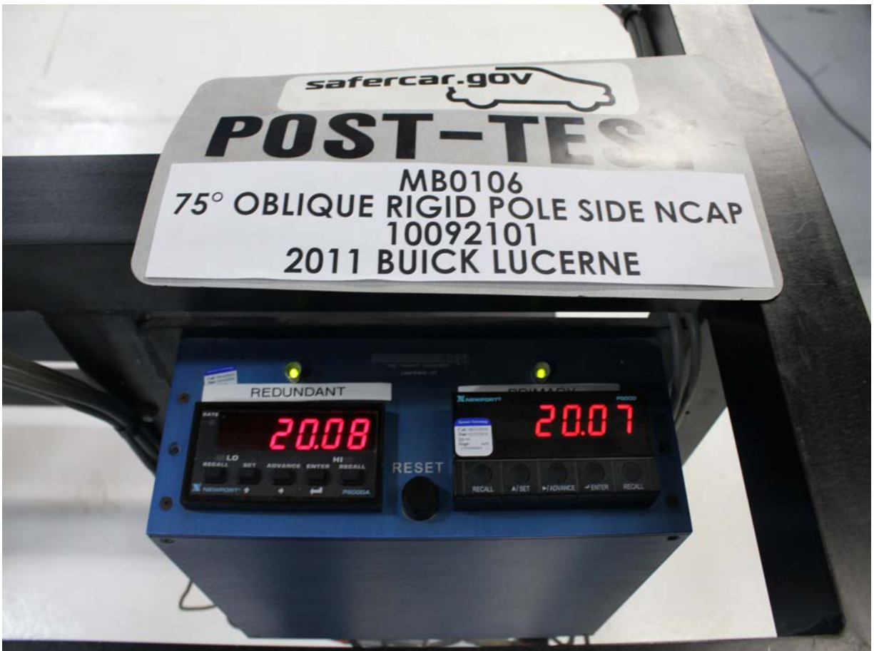
Post-Test Primary and Redundant Speed Trap Read-Out
