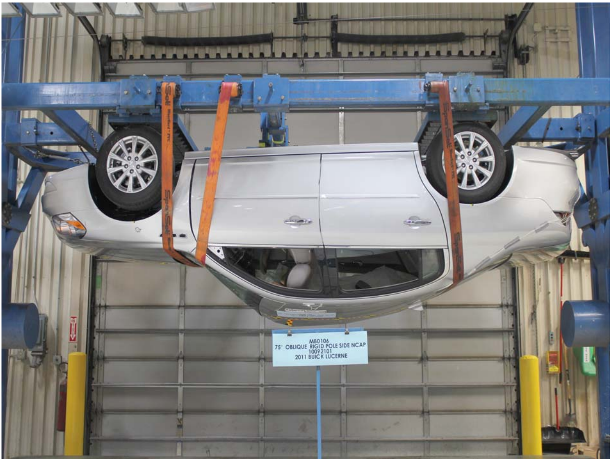
FMVSS No. 301/305 Rollover 180 Degrees
