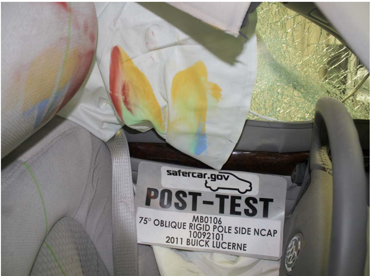
Post-Test Dummy Close-Up Head Contact with Side Airbag View
