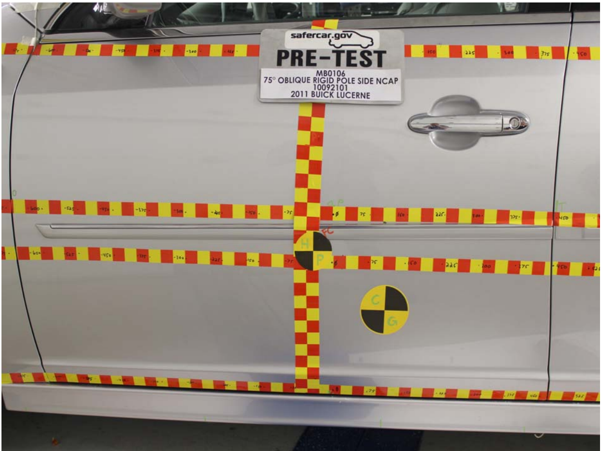
Pre-Test Close-Up View of Impact Point Target
