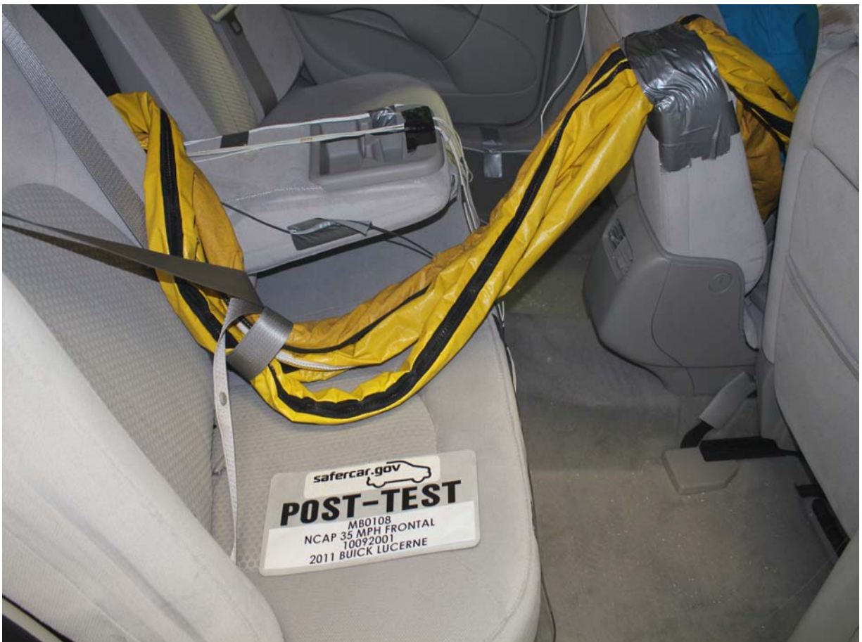
Post-Test Dummy Cable Routing
