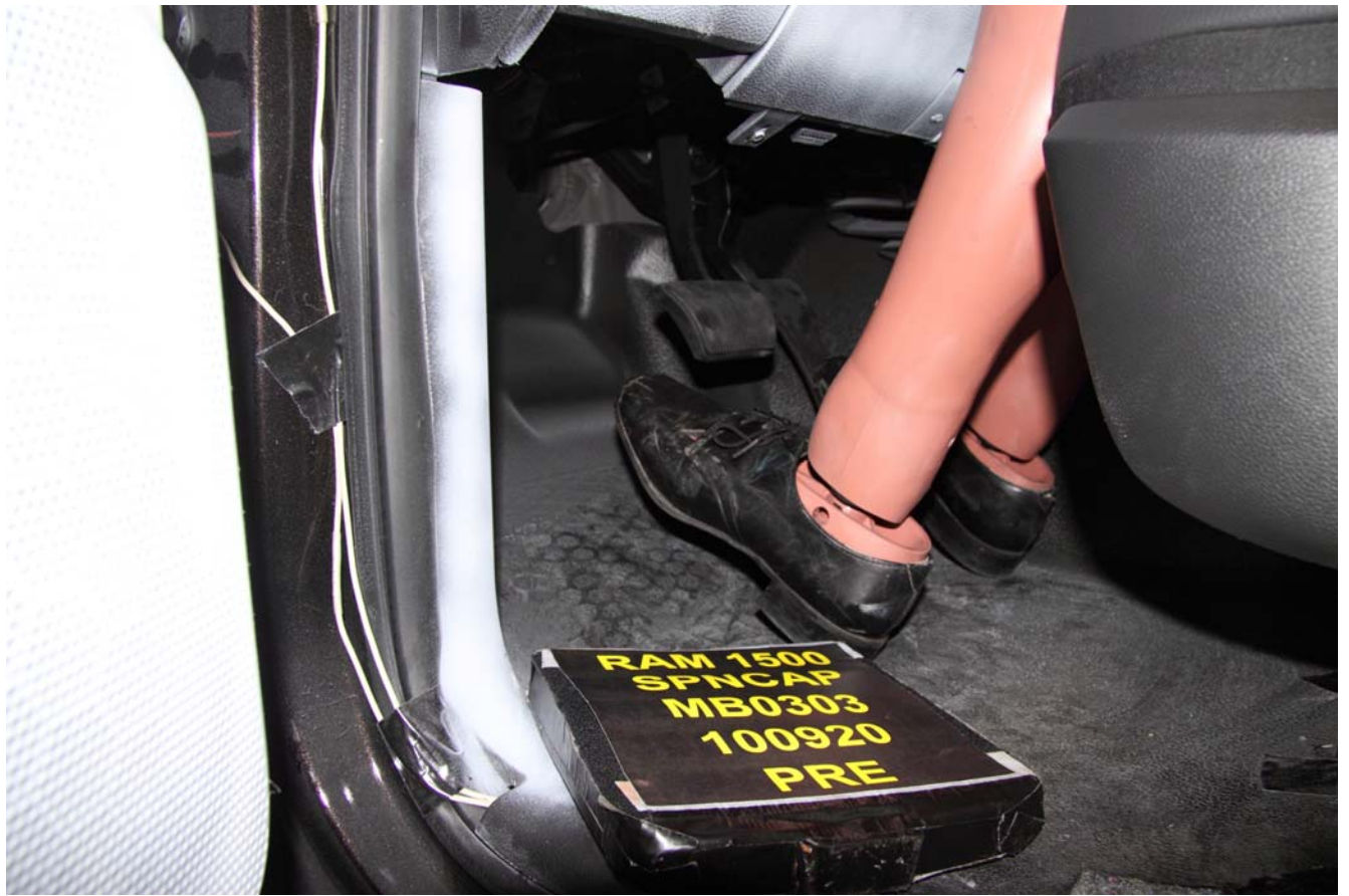
No. 032 – Pre-Test Placement of Dummy's Feet
