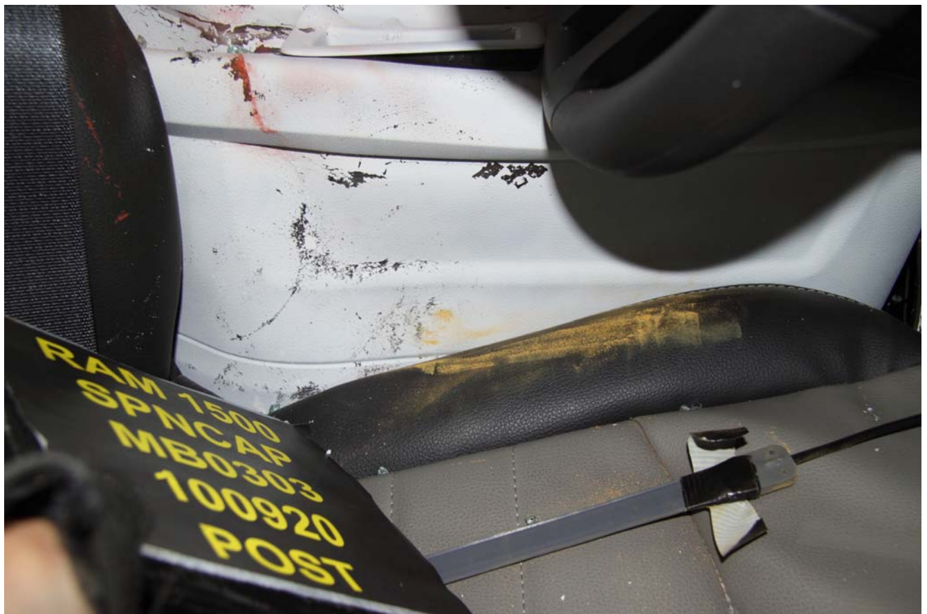
No. 050 – Post-Test Dummy Close-Up Pelvis Contact with Side Airbag View
