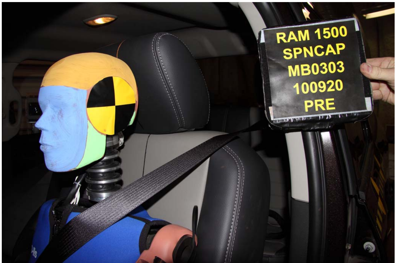
No. 027 – Pre-Test Frontal View of Dummy Head and Shoulders in Relation to Head Restraint
