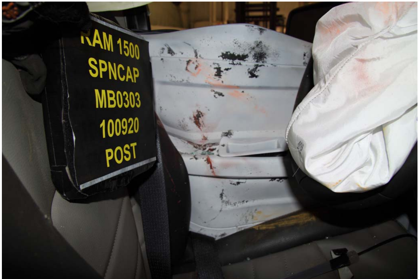
No. 047 – Post-Test Dummy Close-Up Torso Contact with Vehicle Interior View
