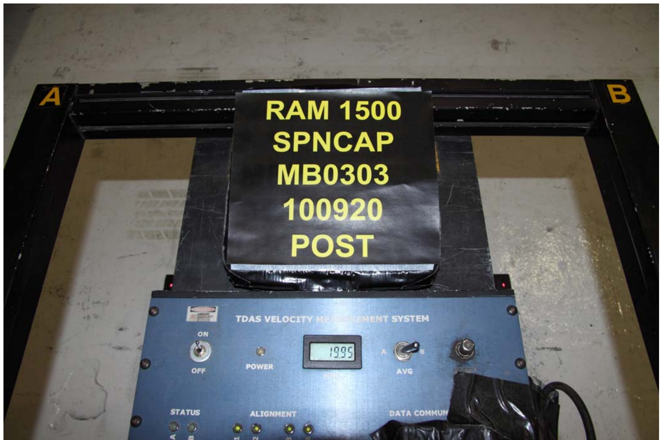
No. 060 – Post-Test Primary Speed Trap Read-Out
