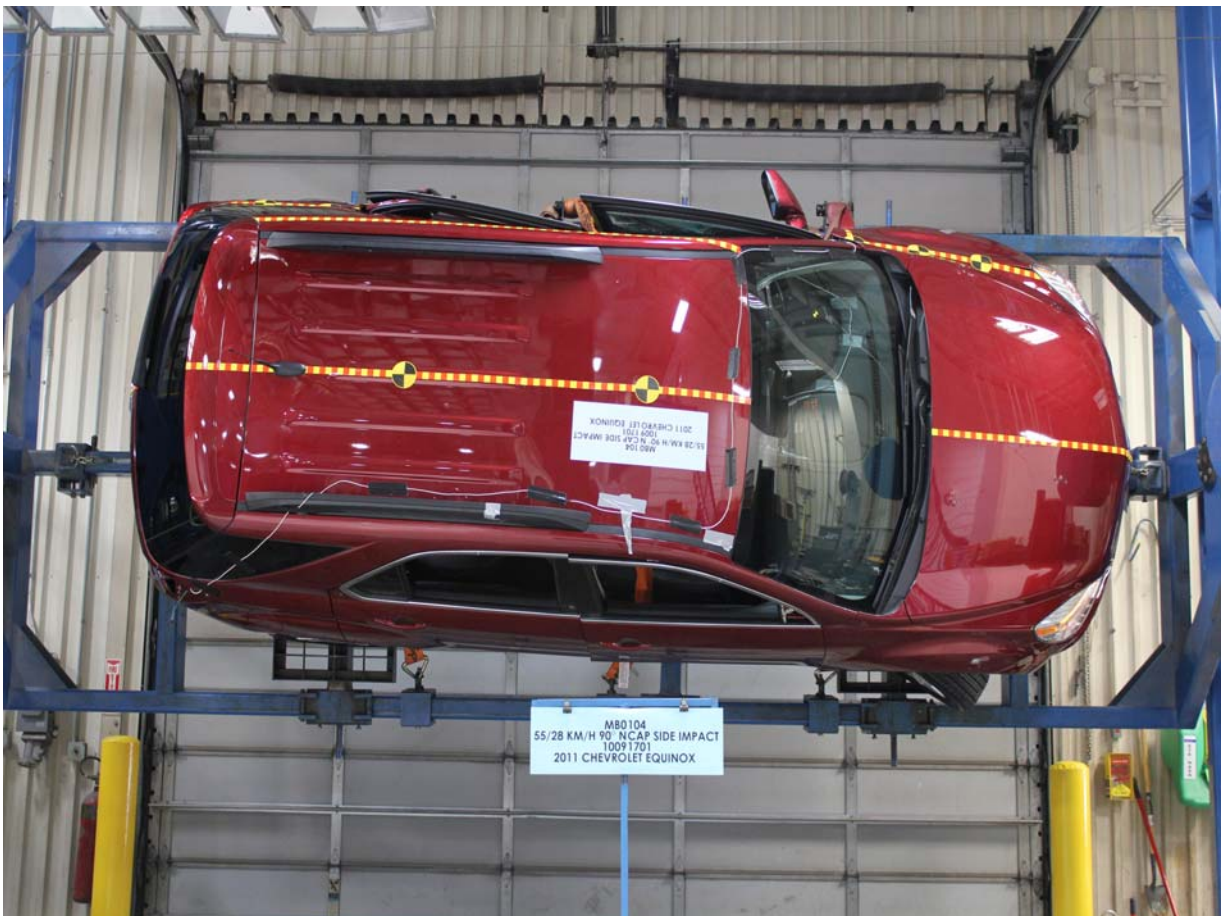
FMVSS No. 301/305 Rollover 90 Degrees
