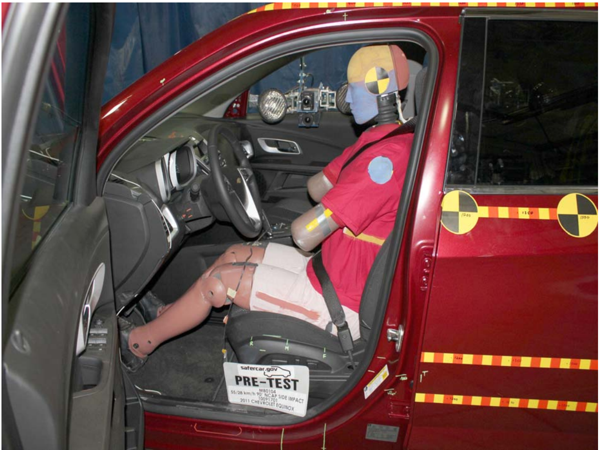
Pre-Test Left Side View of Driver Dummy Showing Belt, Chalking, and Contact Switches
