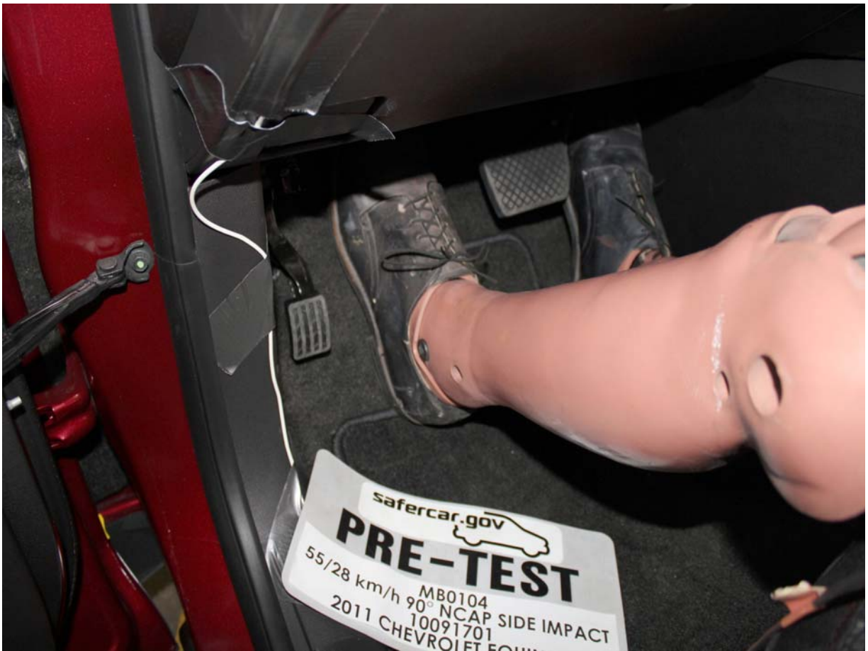
Pre-Test Placement of Driver Dummy's Feet
