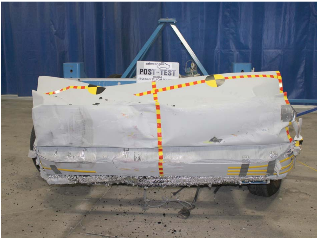
Post-Test Front View of MDB Impactor Face
