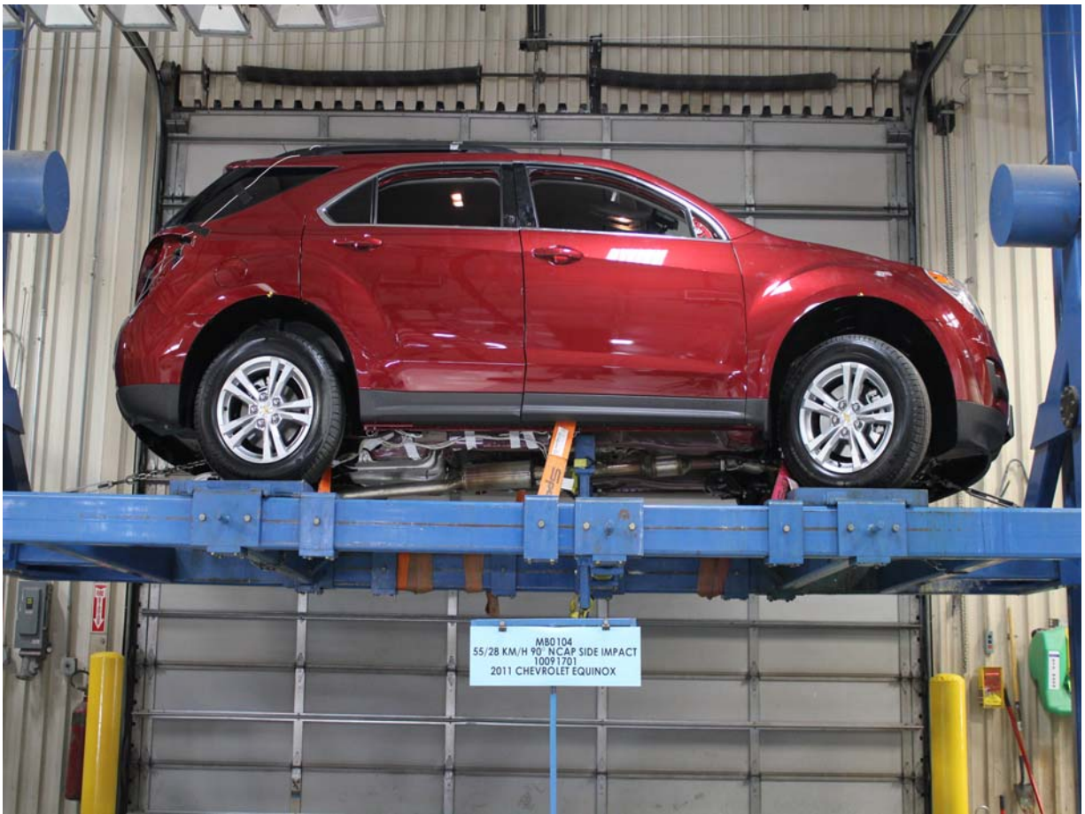
FMVSS No. 301/305 Rollover 360 Degrees
