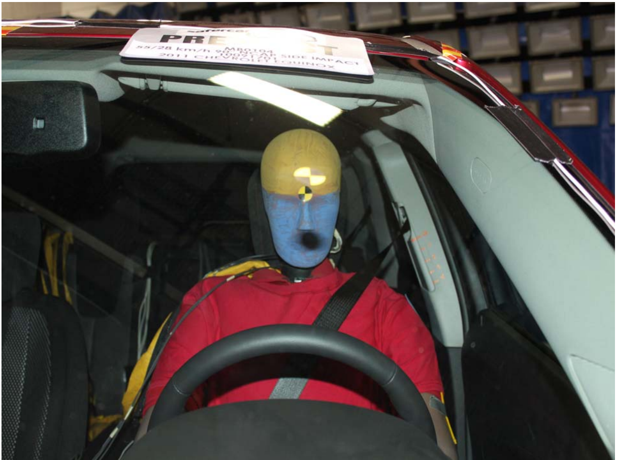
Pre-Test Frontal View of Driver Dummy Head and Shoulders in Relation to Head Restraint
