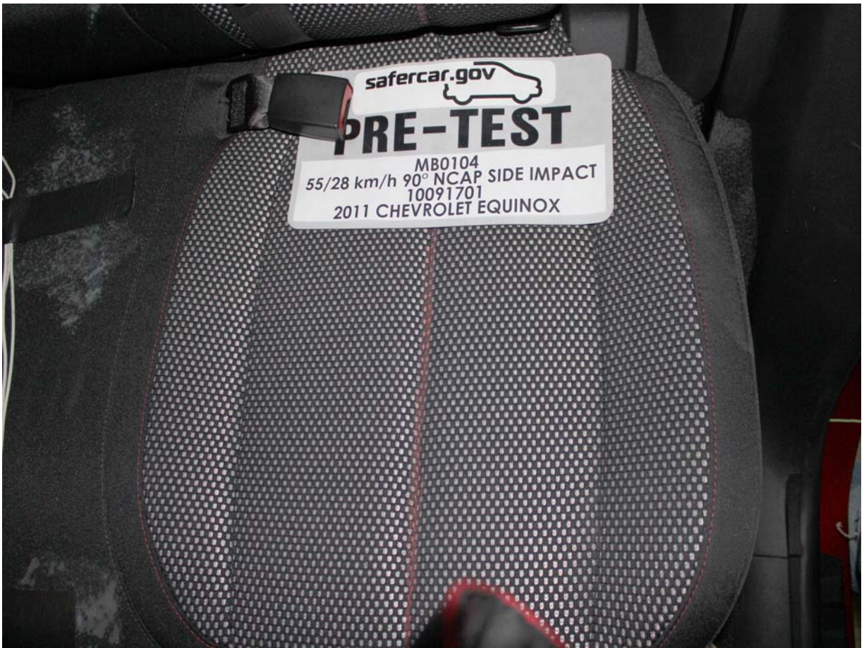
Pre-Test Overhead View of Rear Passenger Seat Pan Prior to Dummy Positioning
