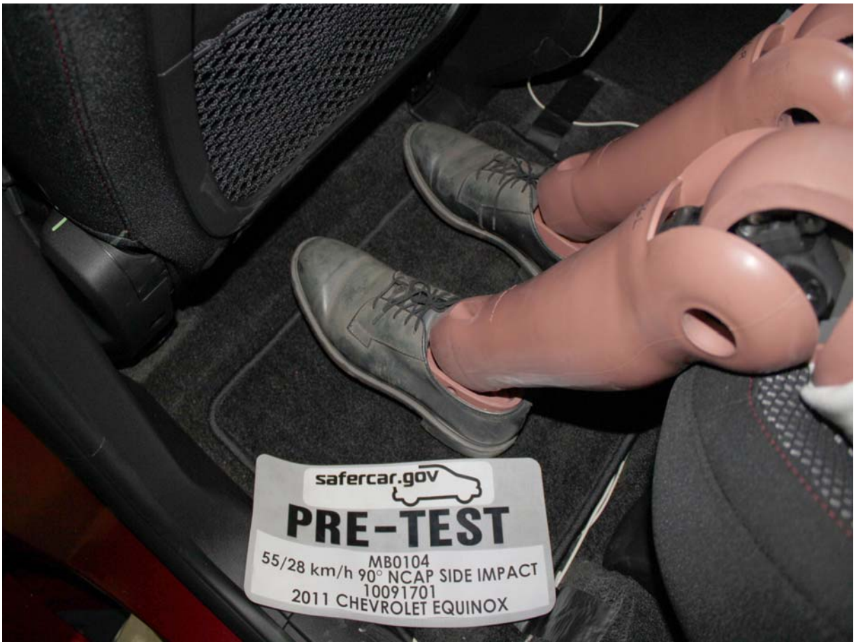
Pre-Test Placement of Rear Passenger Dummy's Feet
