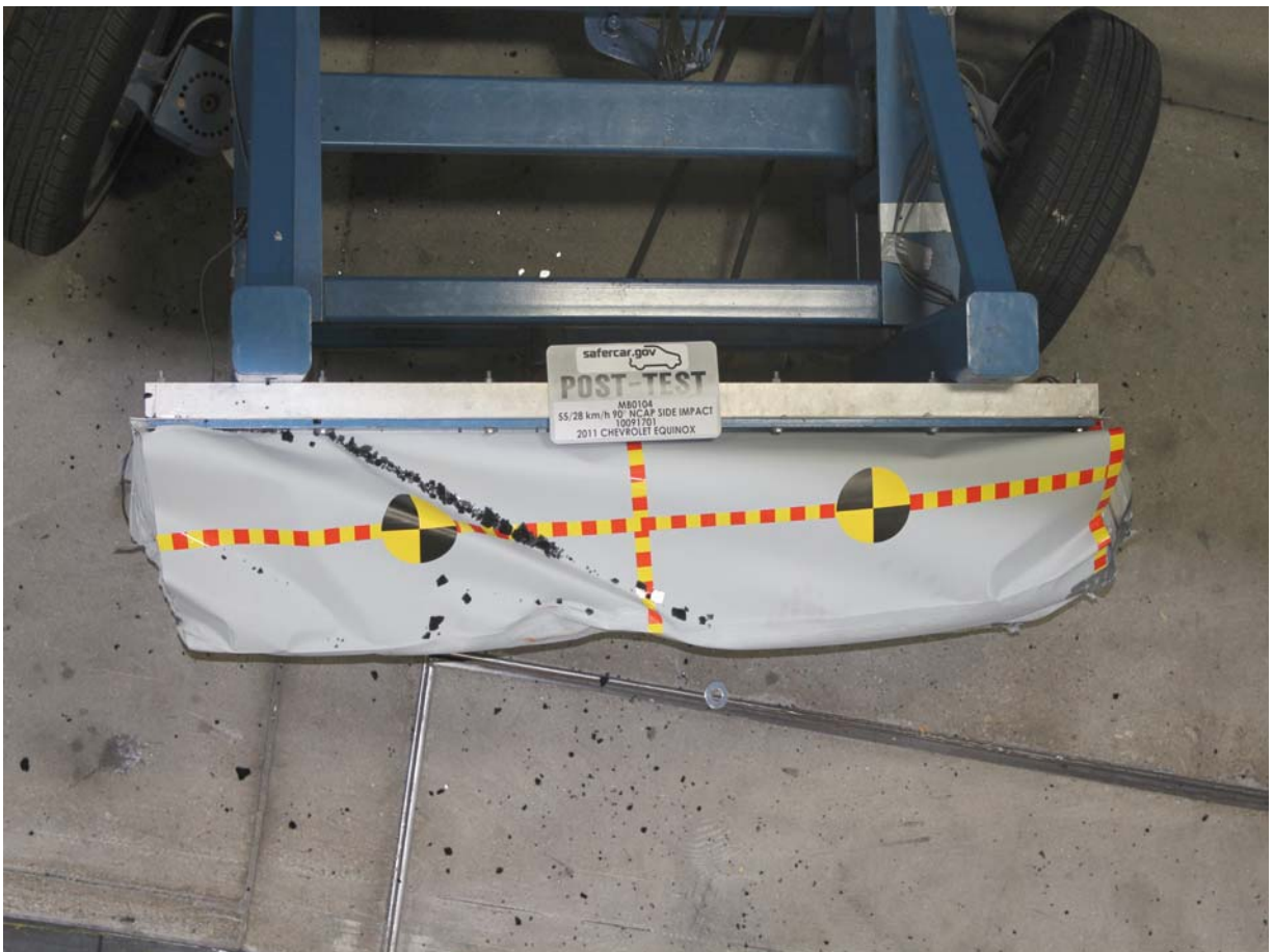
Post-Test Top View of MDB Impactor Face
