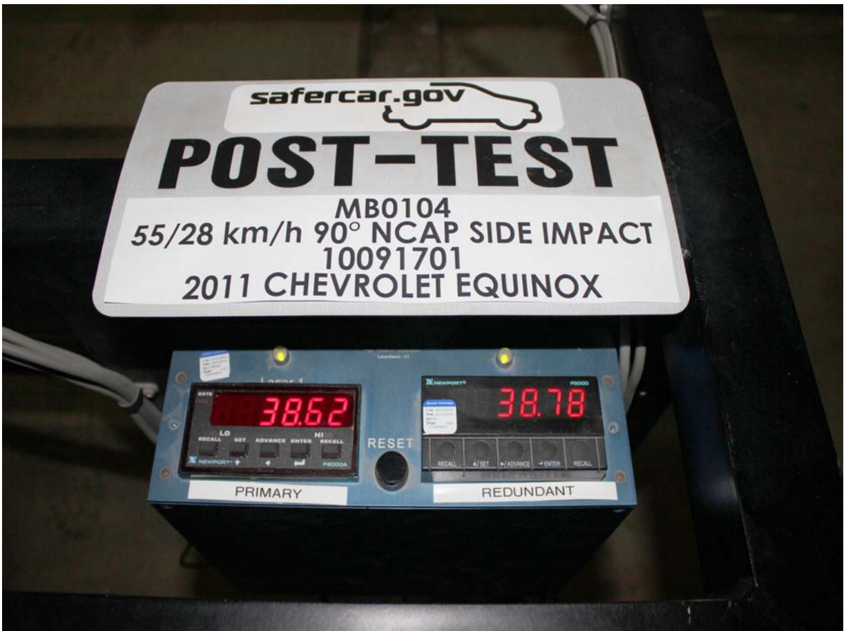
Post-Test Primary and Redundant Speed Trap Read-Out
