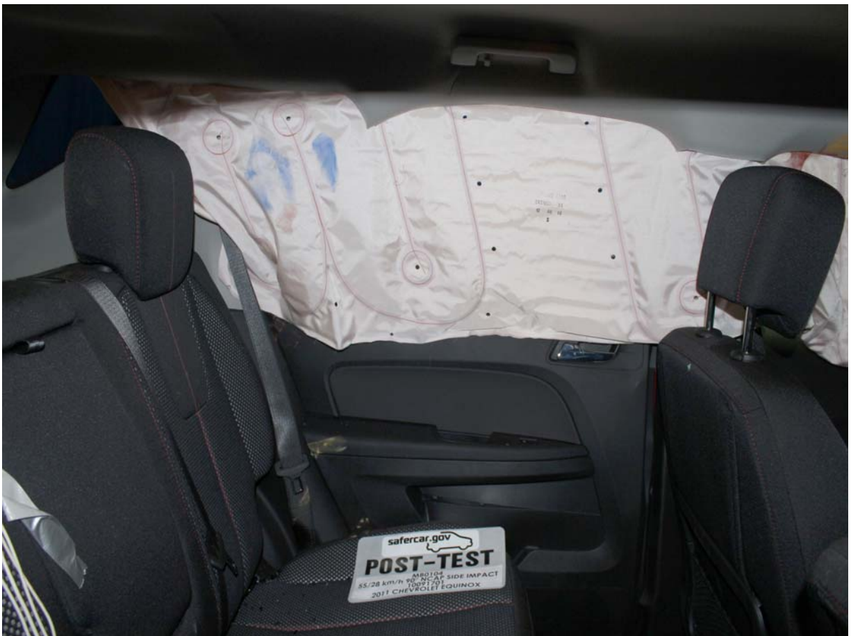
Post-Test Rear Passenger Inner Door Panel View Showing Dummy Contact Locations
