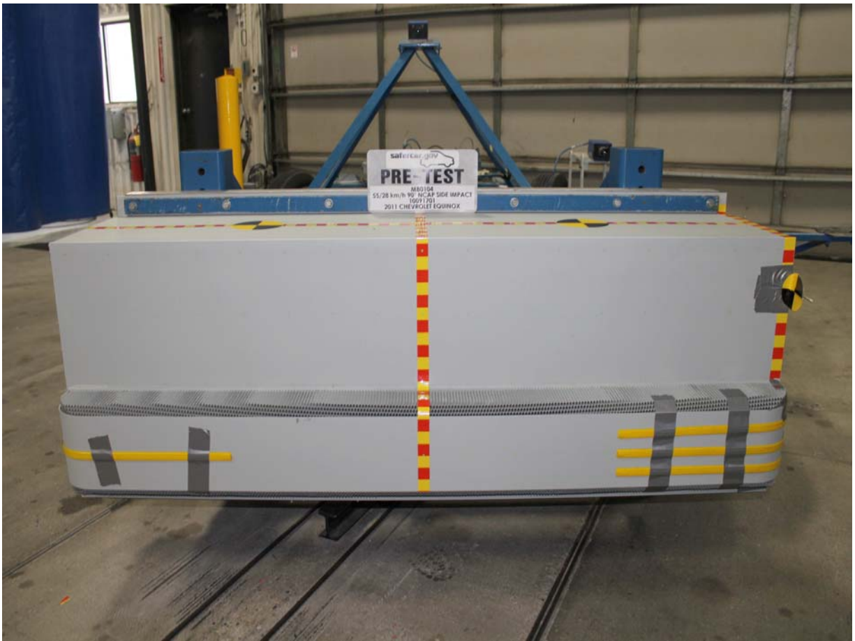
Pre-Test Front View of MDB Impactor Face
