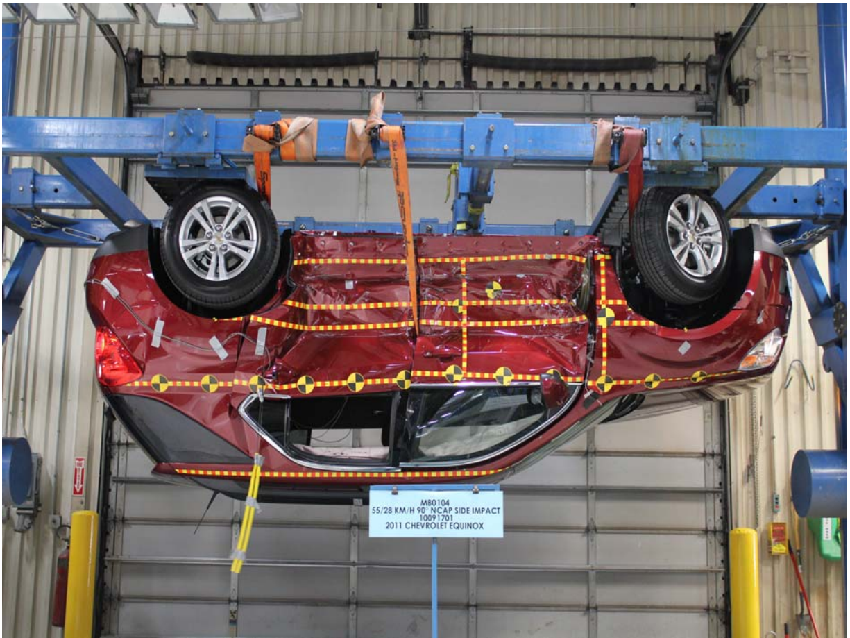
FMVSS No. 301/305 Rollover 180 Degrees
