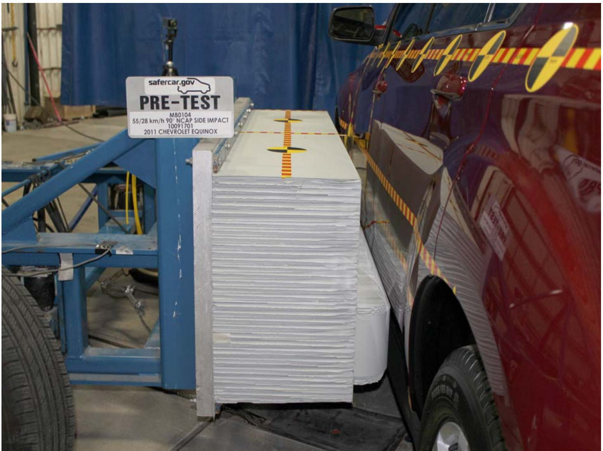
Pre-Test Right Side View of MDB Positioned Against Side of Test Vehicle
