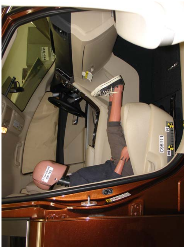
6-Year-Old Unbelted, Rearward Seat Track, Position 1
