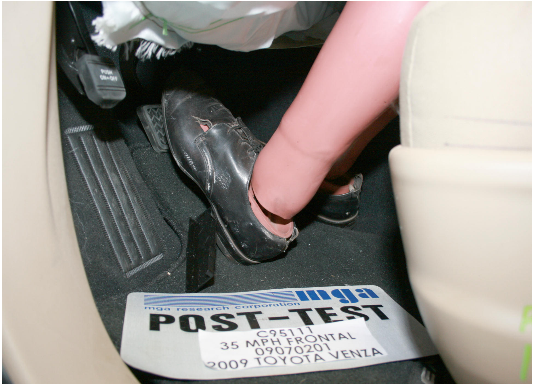
Post-Test Driver Dummy Feet Position
