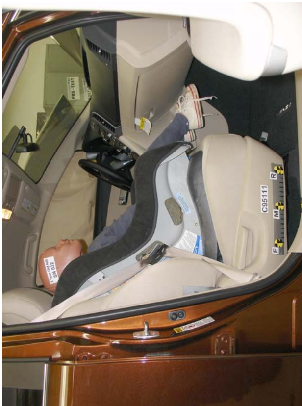
3-Year-Old Forward Facing Century Encore Buckled, Middle Seat Track
