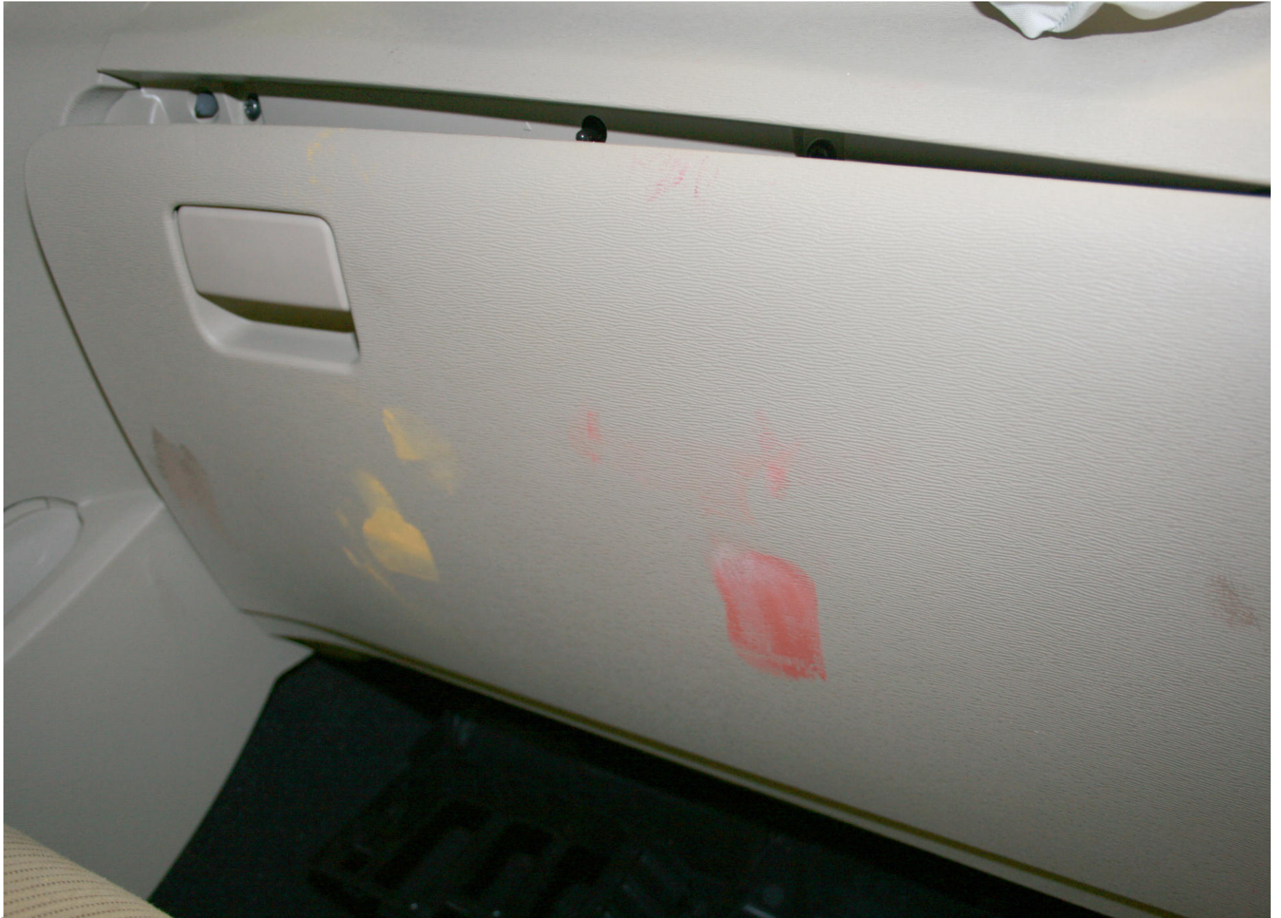
Post-Test Passenger Dummy Knee Contact
