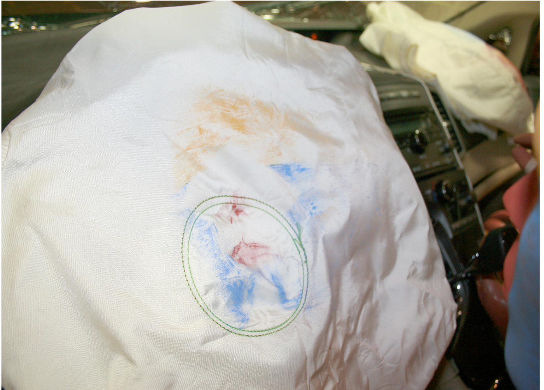
Post-Test Driver Dummy Airbag Contact
