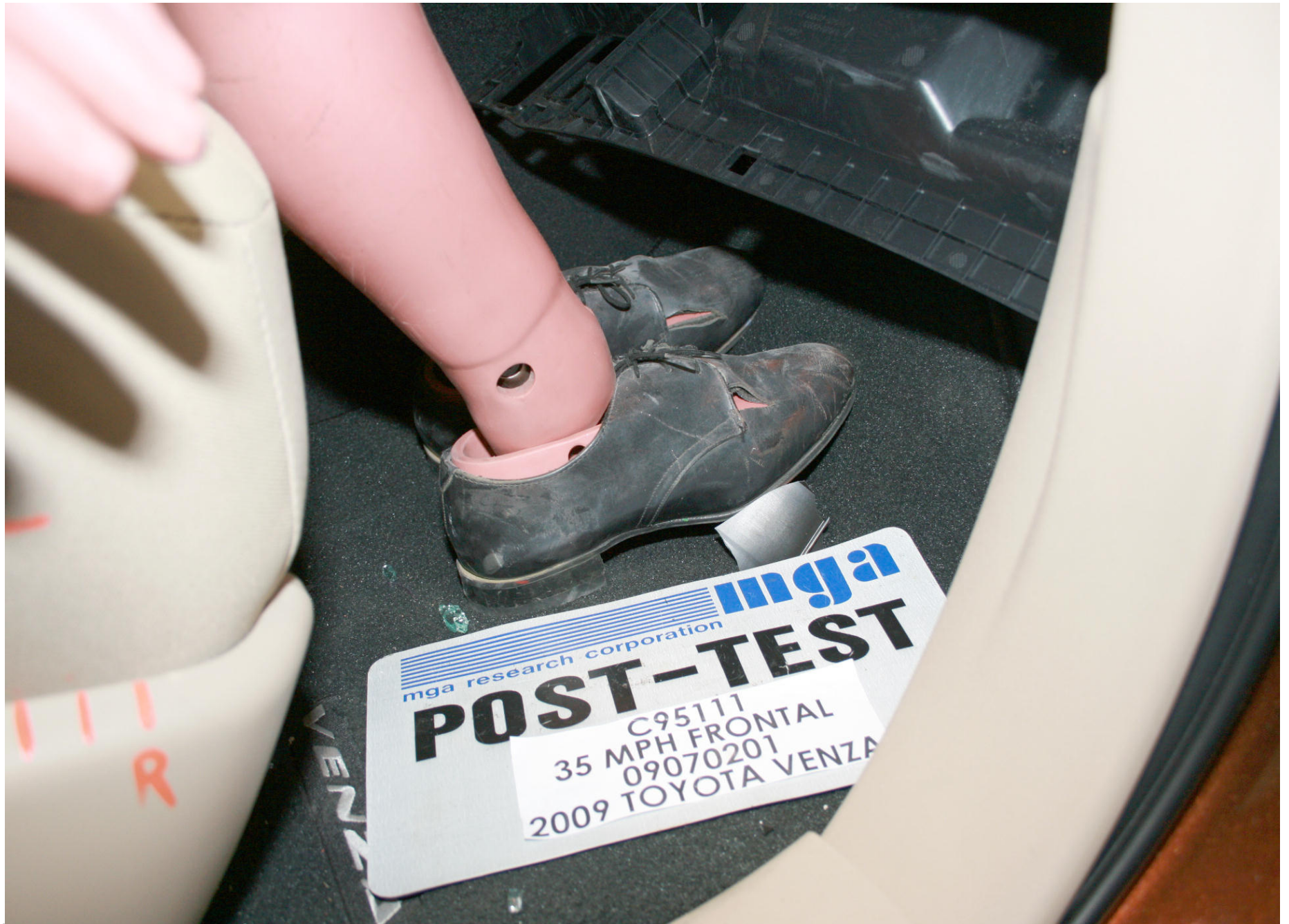
Post-Test Passenger Dummy Feet Position
