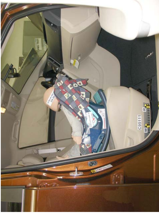
Britax Handle With Care 191 Unbelted, Rearward Seat Track
