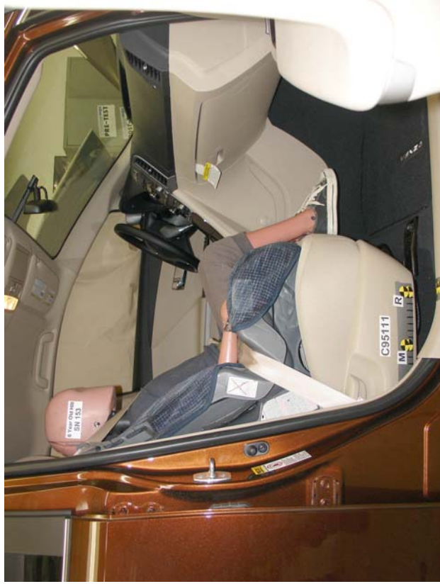
6-Year-Old Cosco High Back Booster Belted, Rearward Seat Track
