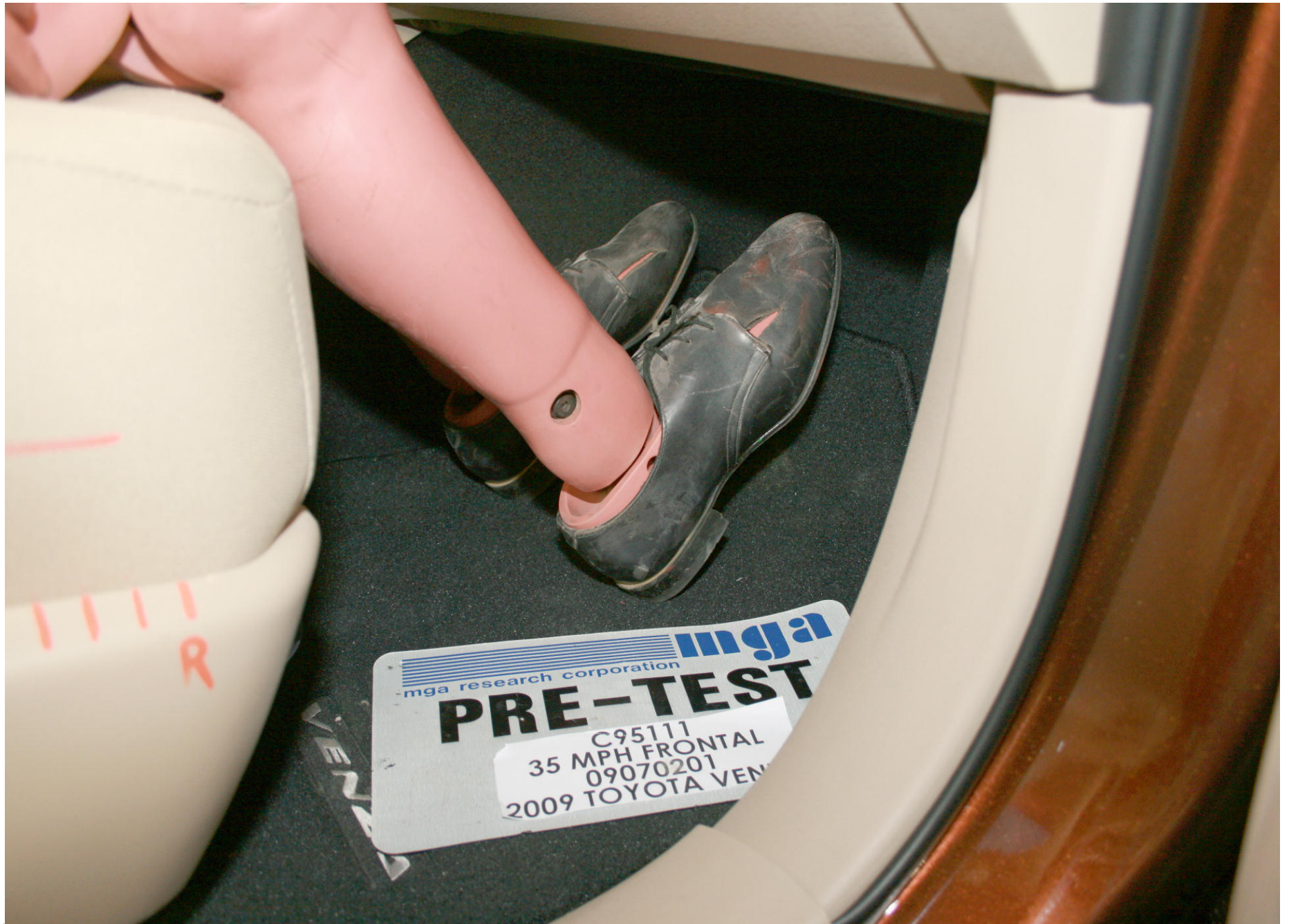
Pre-Test Passenger Dummy Feet Position
