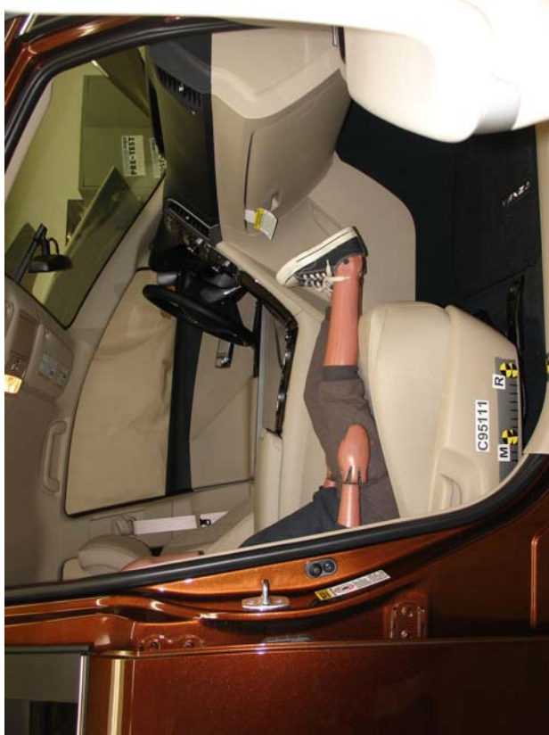
6-Year-Old Unbelted, Rearward Seat Track, Position 2
