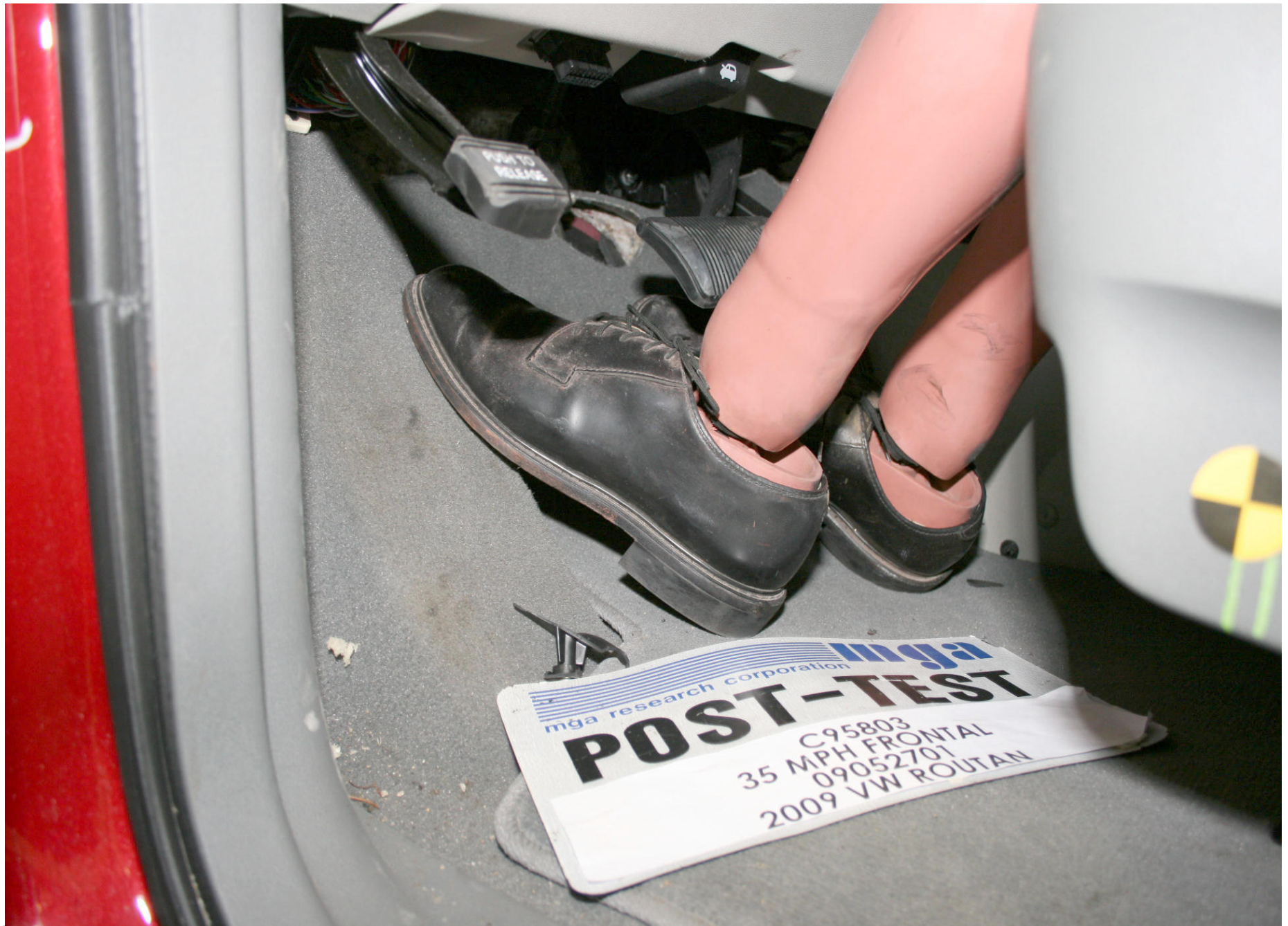
Post-Test Driver Dummy Feet Position
