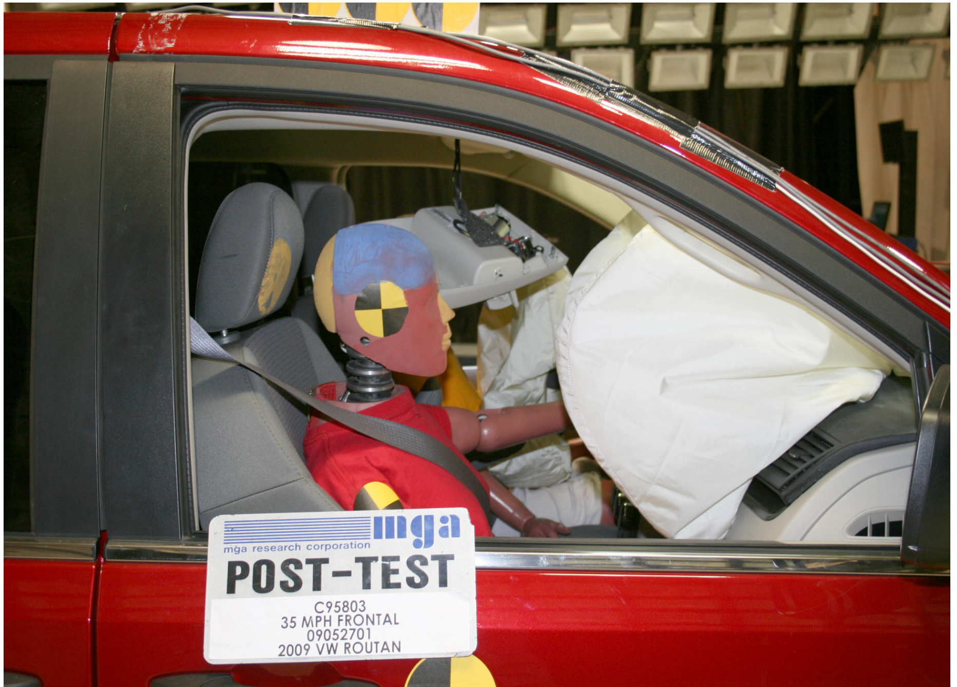
Post-Test Passenger Dummy Position Right Side View
