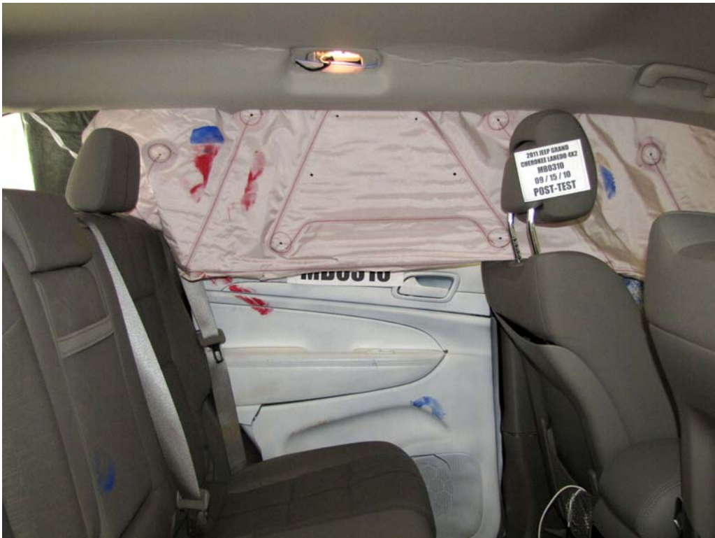
FIGURE 72. Post-Test Rear Passenger Inner Door Panel View Showing Dummy Contact Locations
