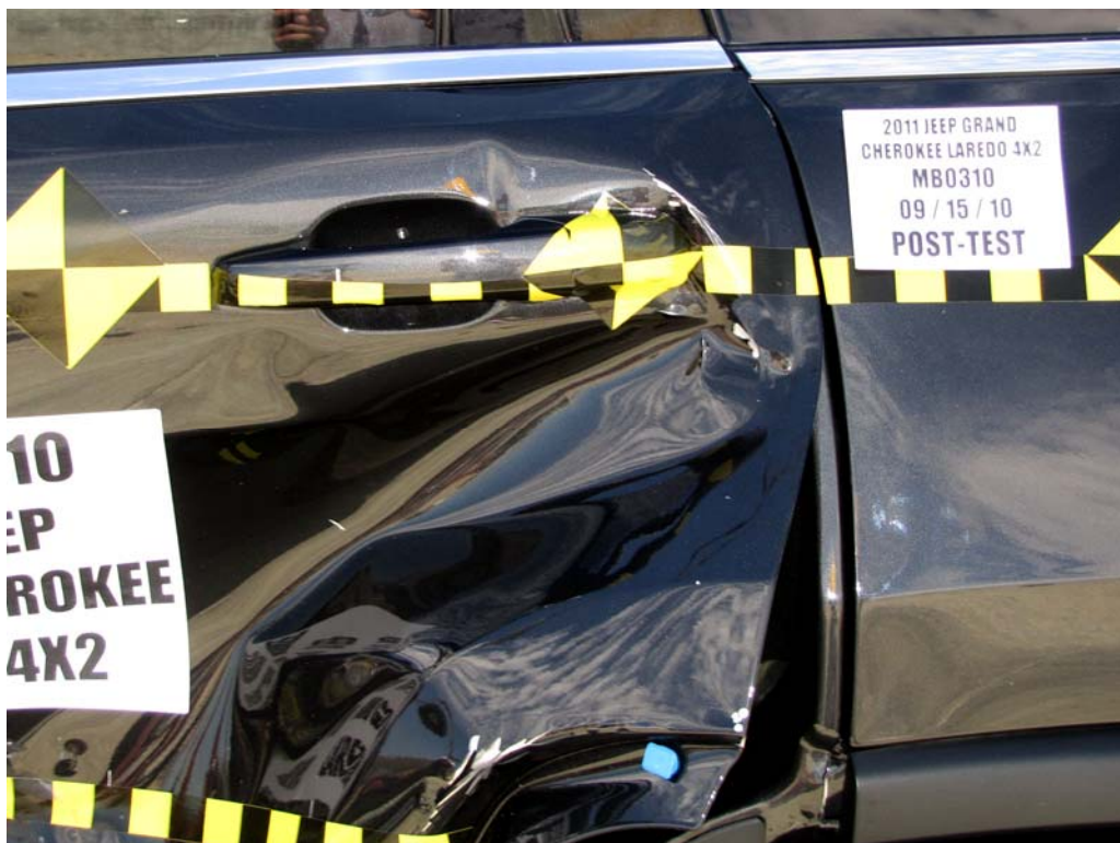
FIGURE 24. Post-Test Left Rear Door Latch Close-Up
