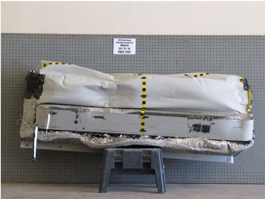
FIGURE 82. Post-Test Front View of MDB Impactor Face
