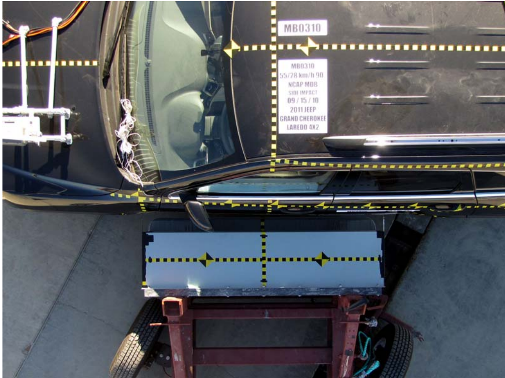
FIGURE 15. Pre-Test Overhead View of Test Vehicle with MDB Positioned Against Side of Test Vehicle
