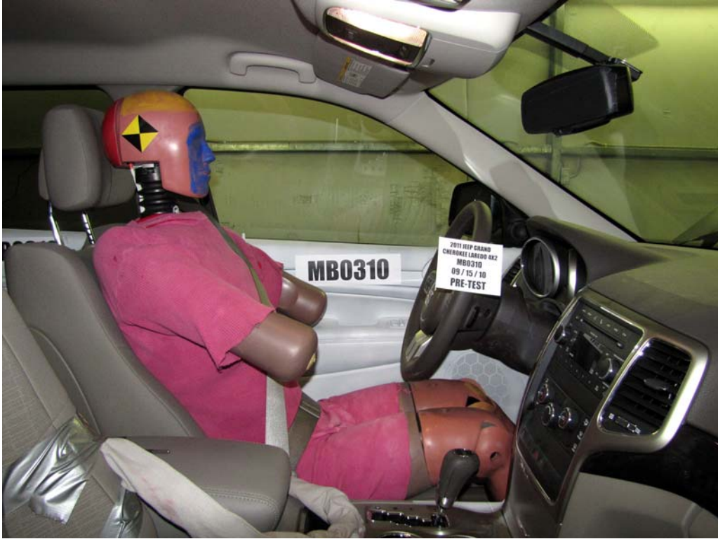
FIGURE 43. Pre-Test Right Side View of Driver Dummy and Front Seat Occupant Compartment
