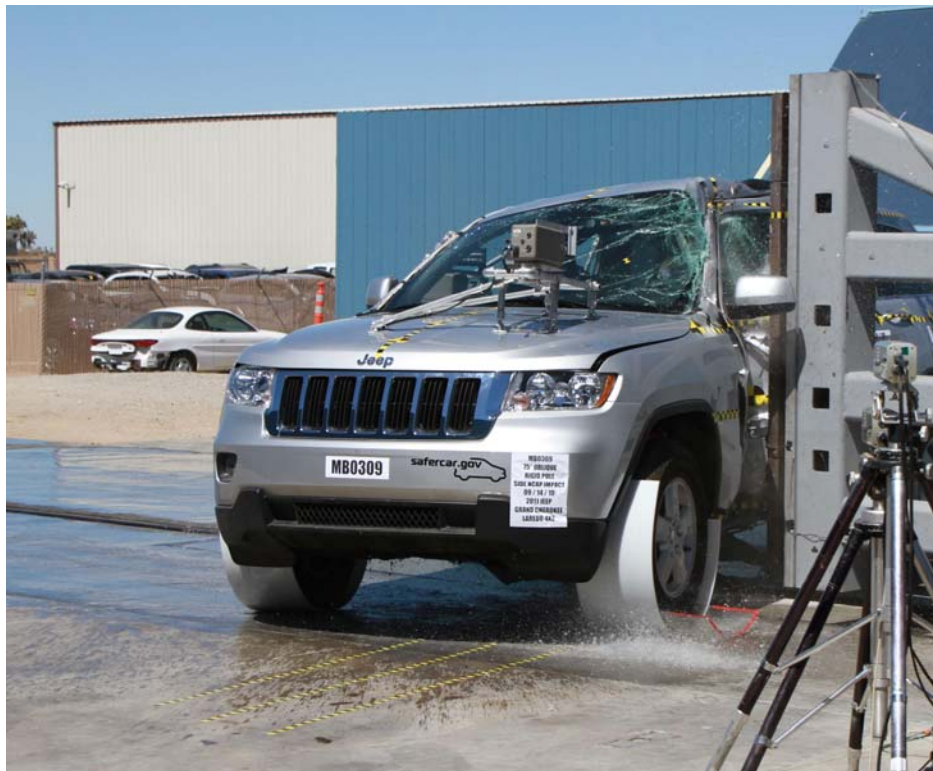
FIGURE 66. 2011 Jeep Grand Cherokee Laredo 4x2 Side Pole Impact Event
