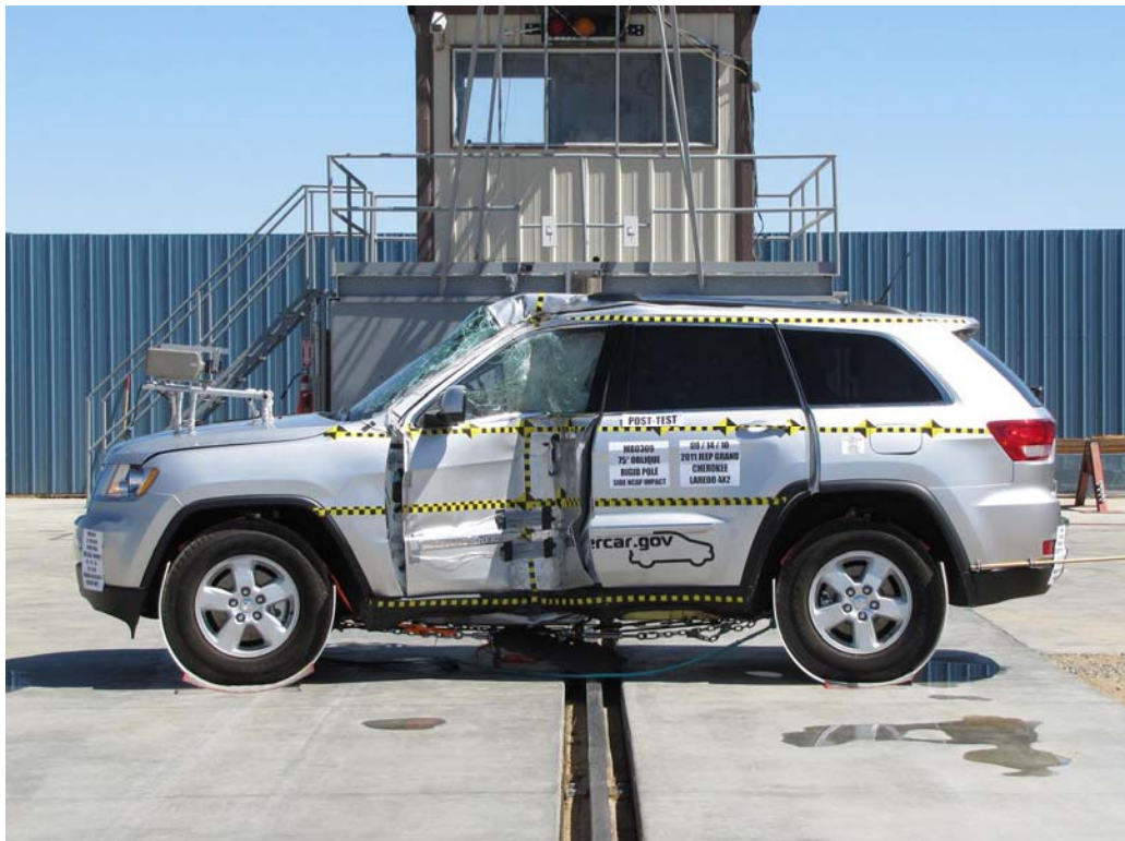
FIGURE 8. Post-Test Left Side View of Vehicle
