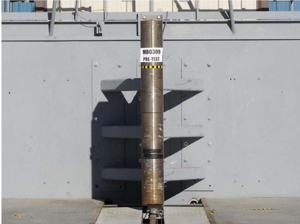
FIGURE 55. Pre-Test Pole Barrier Front View
