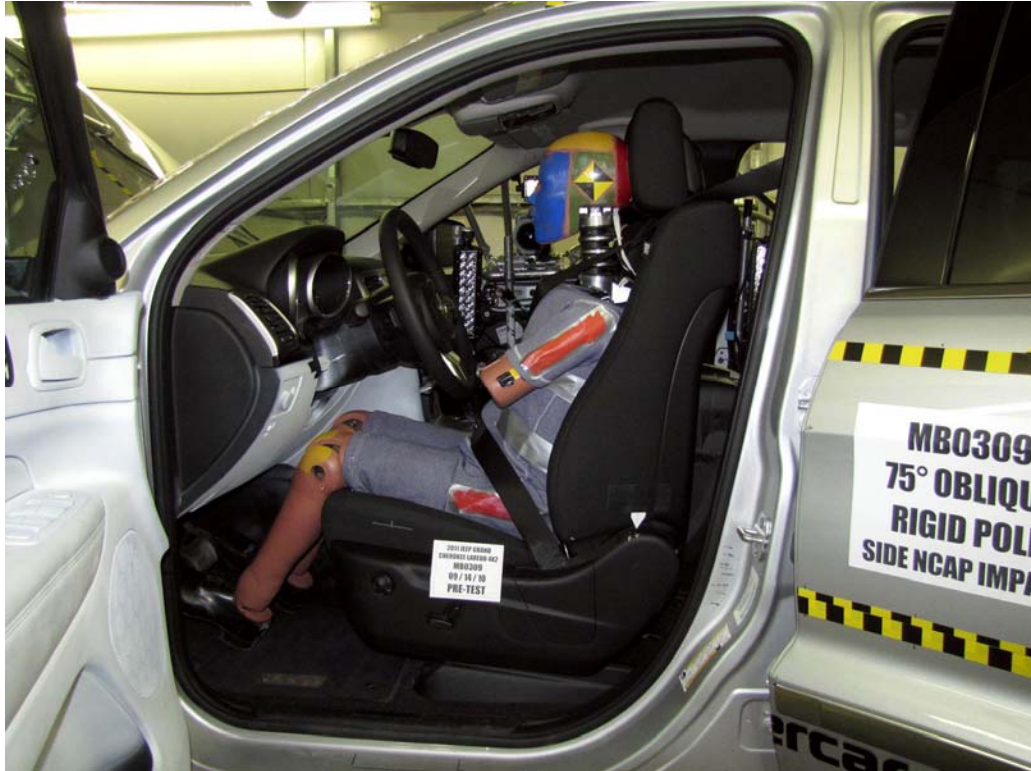
FIGURE 23. Pre-Test Left Side View of Dummy Showing Belt, Chalking, and Contact Switches
