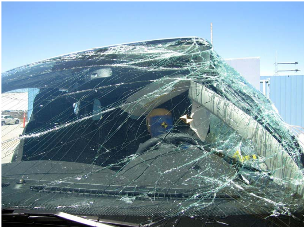
FIGURE 22. Post-Test Front Close-Up View of Dummy
