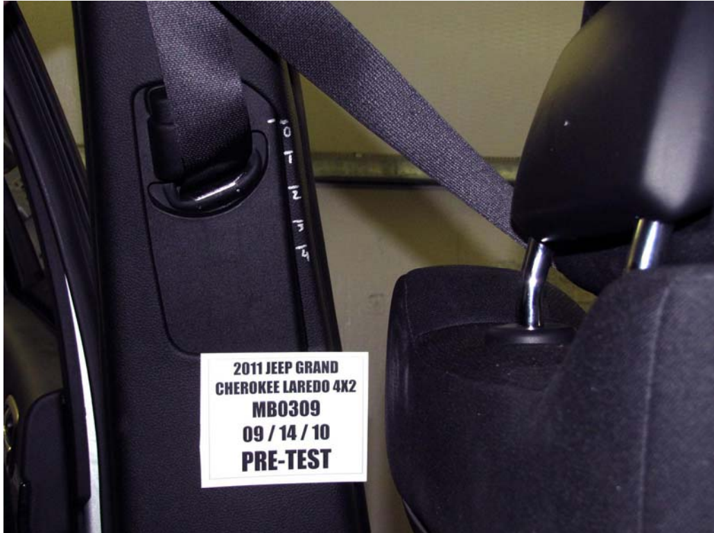
FIGURE 33. Pre-Test View of Belt Anchorage for Dummy
