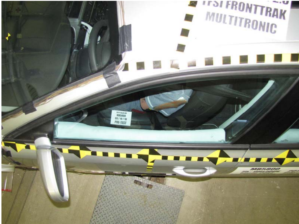
FIGURE 39. Pre-Test Dummy and Driver Door Clearance
