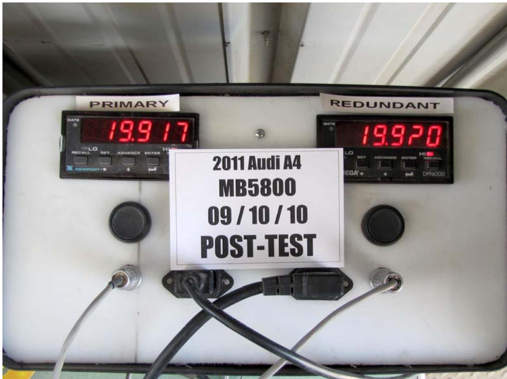
FIGURE 60. Post-Test Primary and Redundant Speed Trap Read-Out
