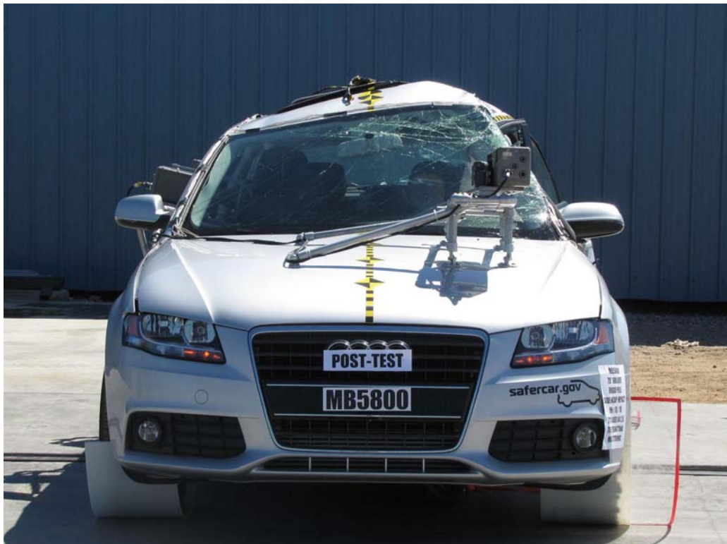
FIGURE 4. Post-Test Frontal View of Test Vehicle
