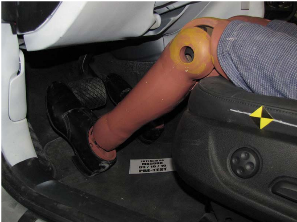
FIGURE 32. Pre-Test Placement of Dummy's Feet
