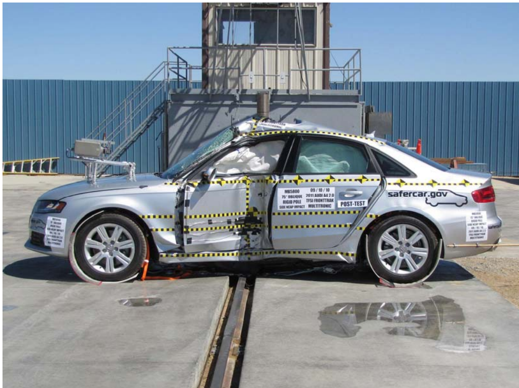
FIGURE 8. Post-Test Left Side View of Vehicle
