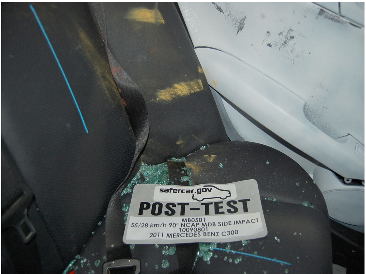
Post-Test Rear Passenger Dummy Close-up Pelvis Contact View
