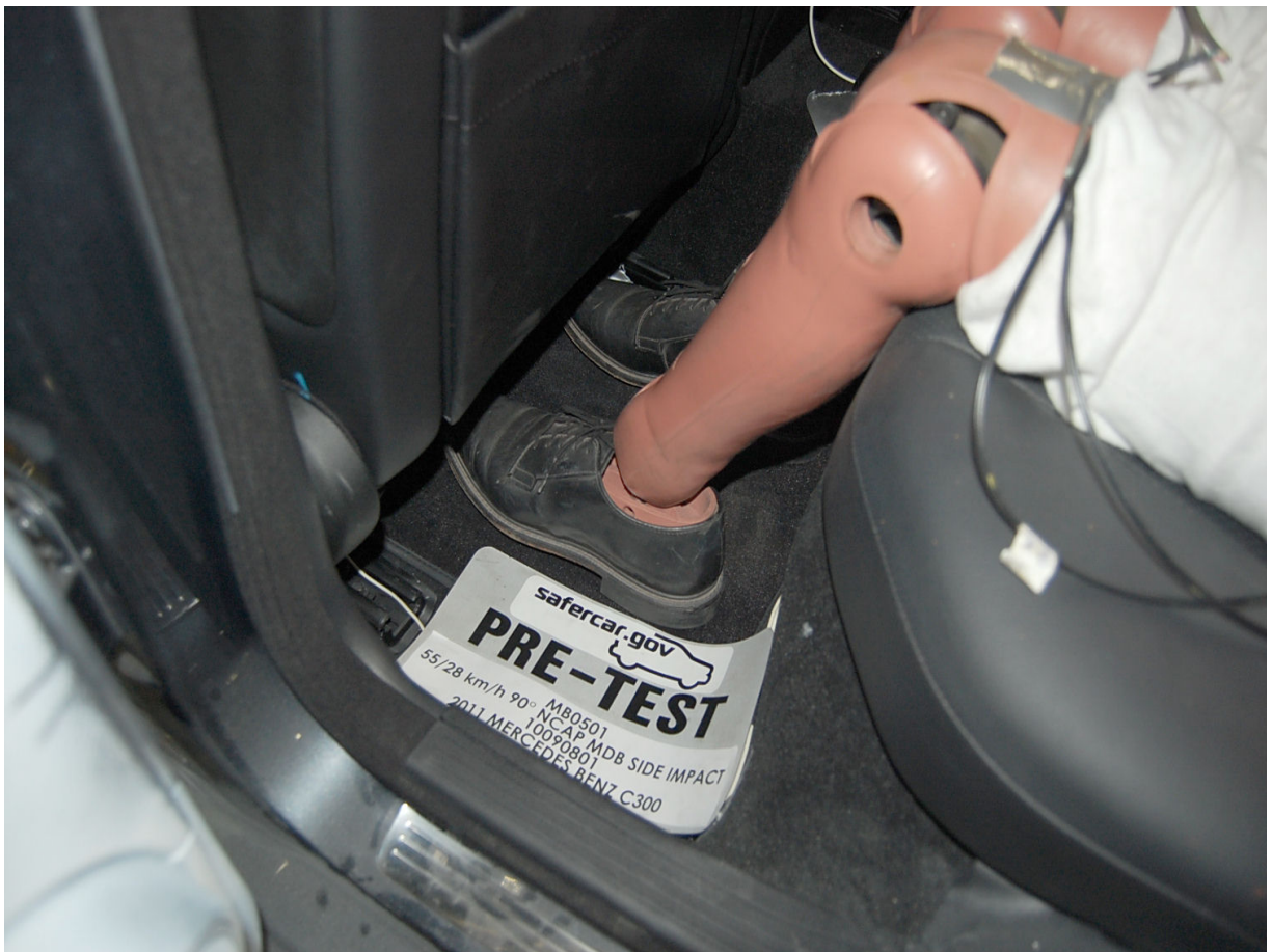
Pre-Test Placement of Rear Passenger Dummy's Feet
