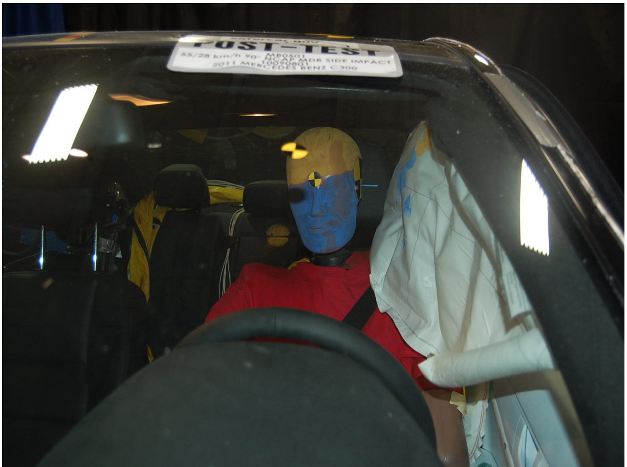
Post-Test Front Close-Up View of Driver Dummy
