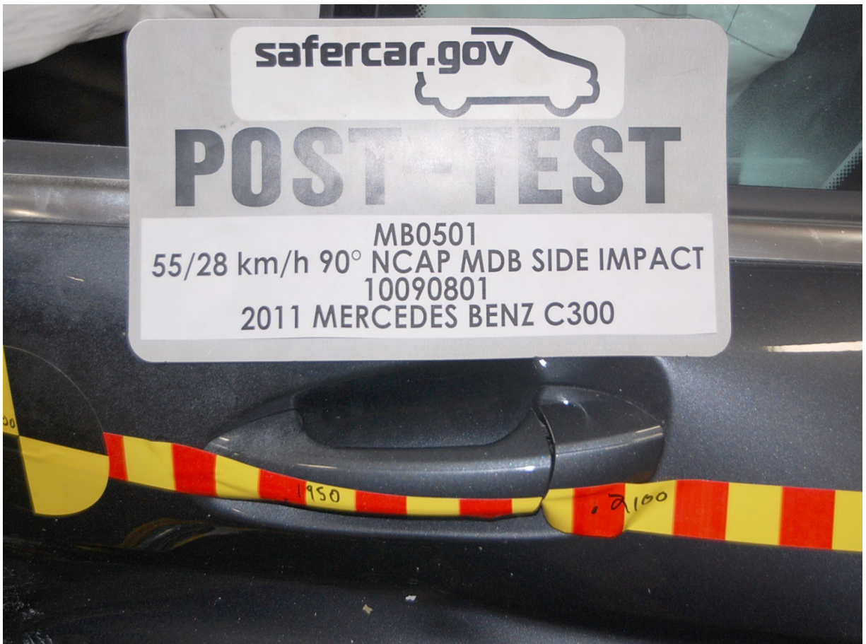
Post-Test Left Rear Door Latch Close-Up
