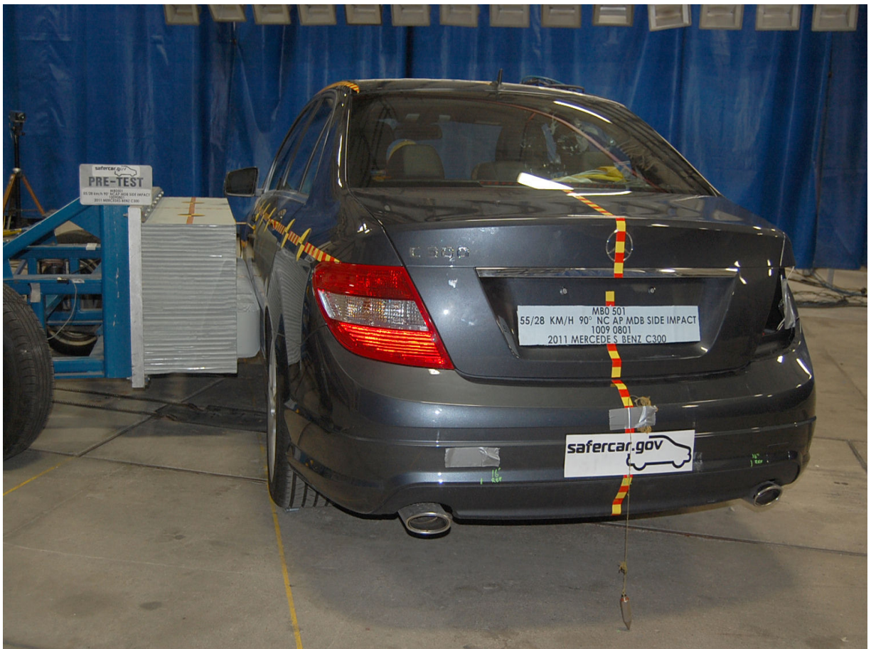
Pre-Test Right Side View of MDB Positioned Against Side of Target Vehicle
