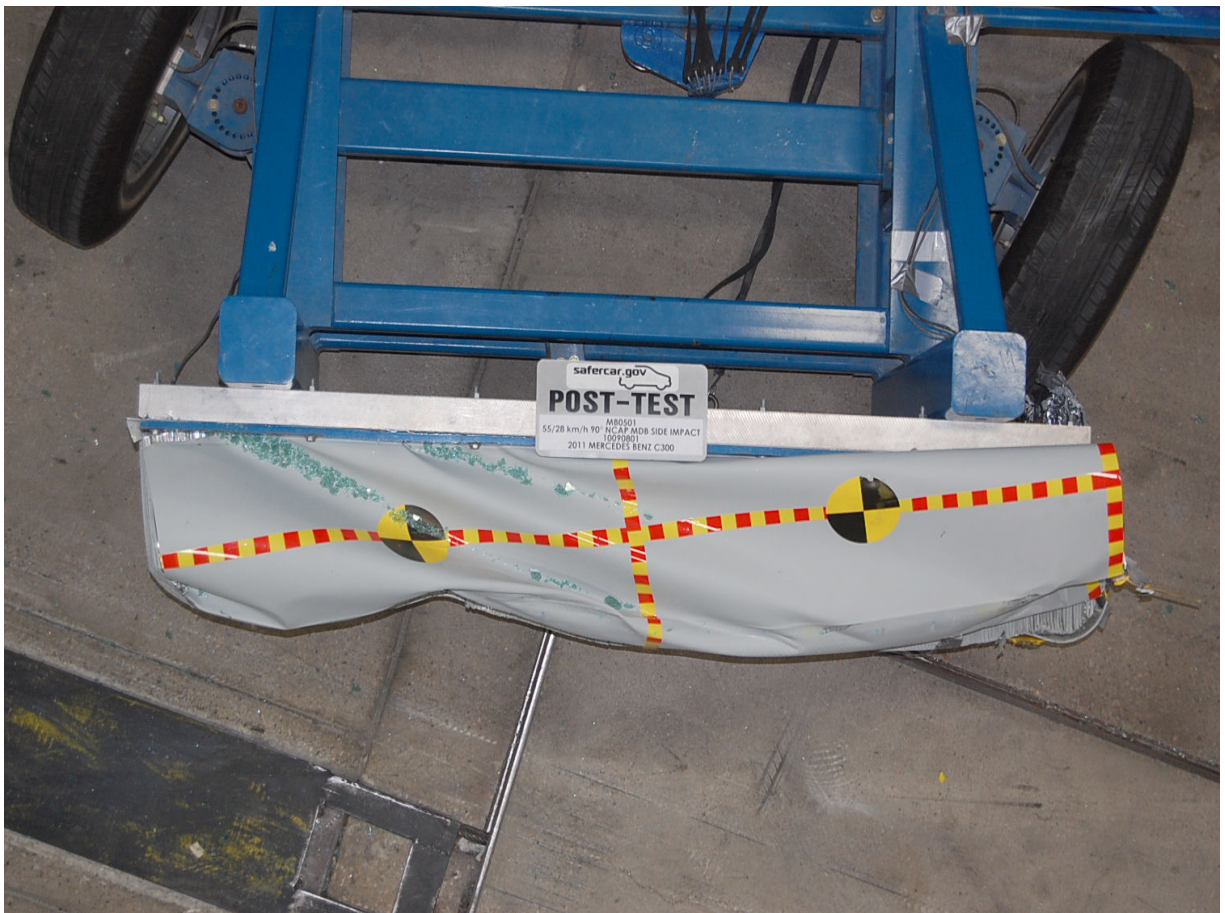
Post-Test Top View of MDB Impactor Face
