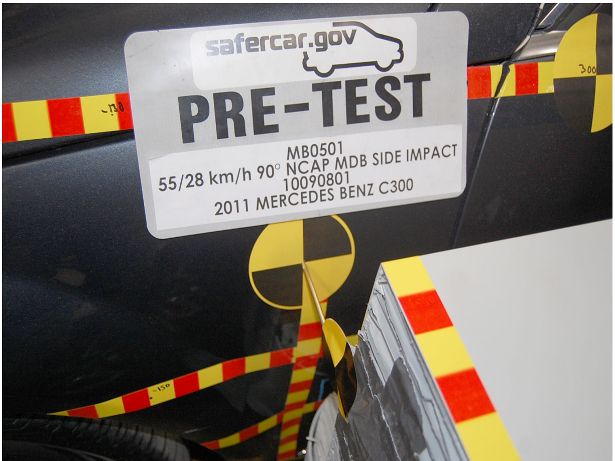
Pre-Test Close-Up View of Impact Point Target
