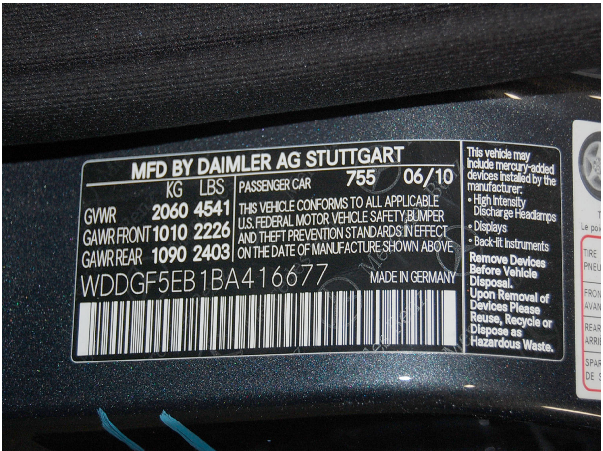
Close-Up View of Vehicle's Certification Label
