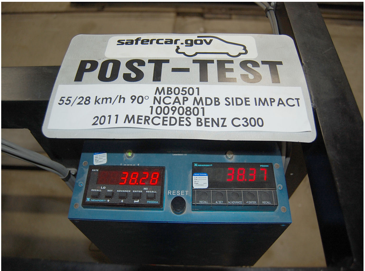
Post-Test Primary and Redundant Speed Trap Read-Out
