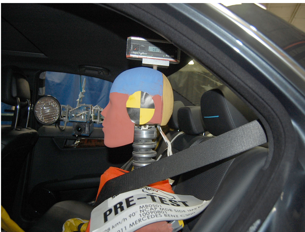
Pre-Test View of Rear Passenger Dummy's Head Showing Dummy's Head is Level
