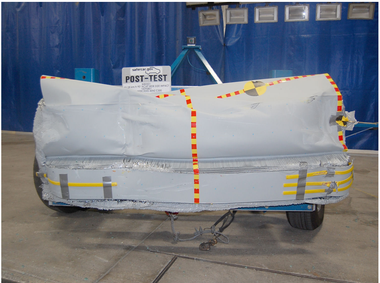
Post-Test Front View of MDB Impactor Face
