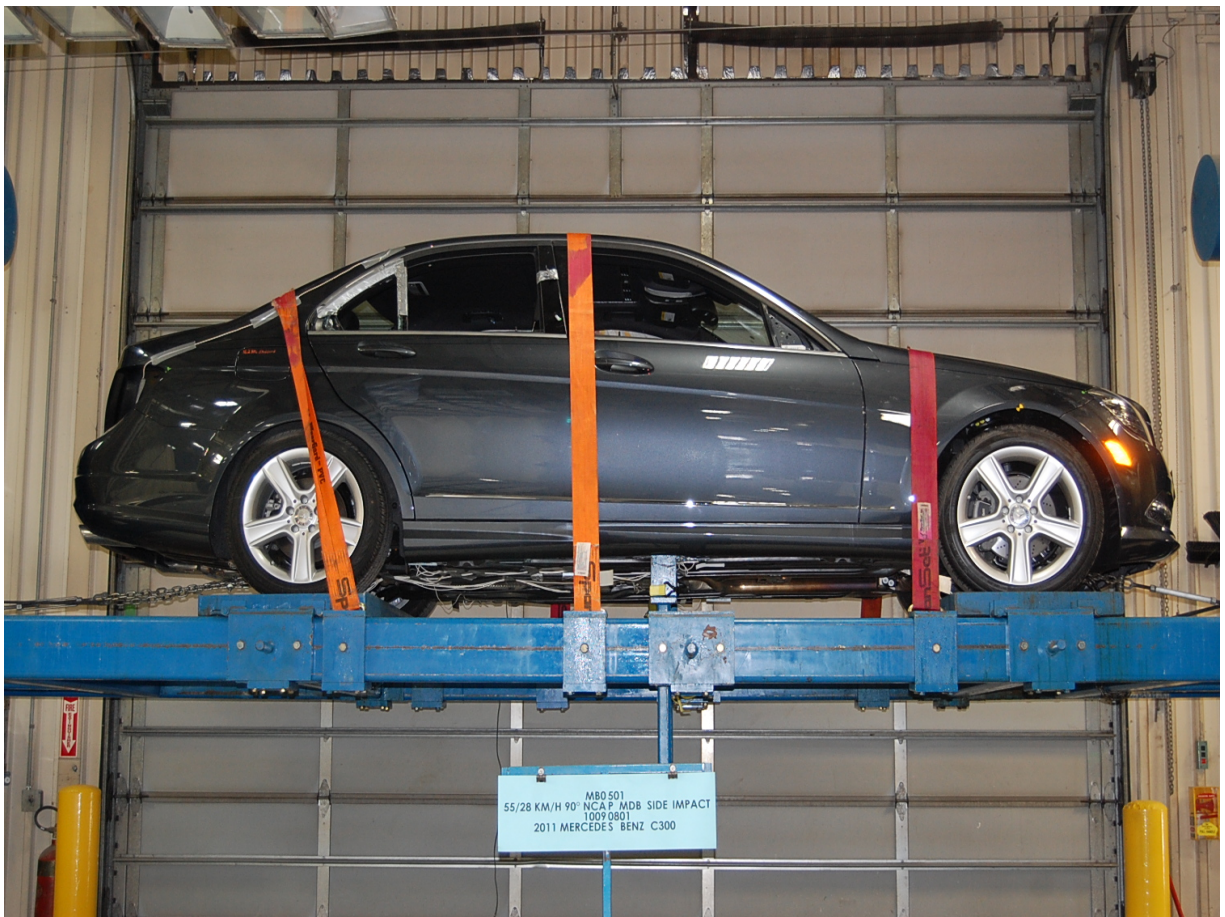
FMVSS No. 301/305 Rollover 360 Degrees
