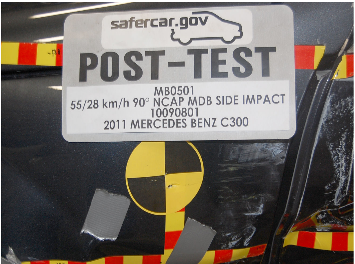
Post-Test Close-Up View of Impact Point Target
