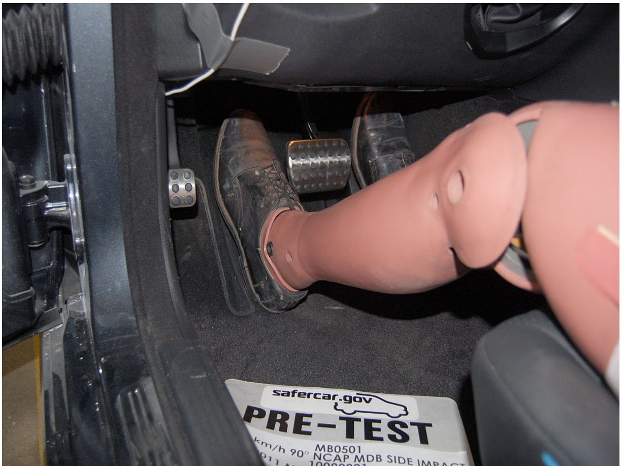
Pre-Test Placement of Driver Dummy's Feet
