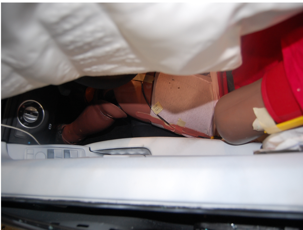
Post-Test Driver Dummy and Door Clearance View
