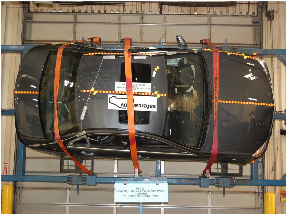
FMVSS No. 301/305 Rollover 90 Degrees
