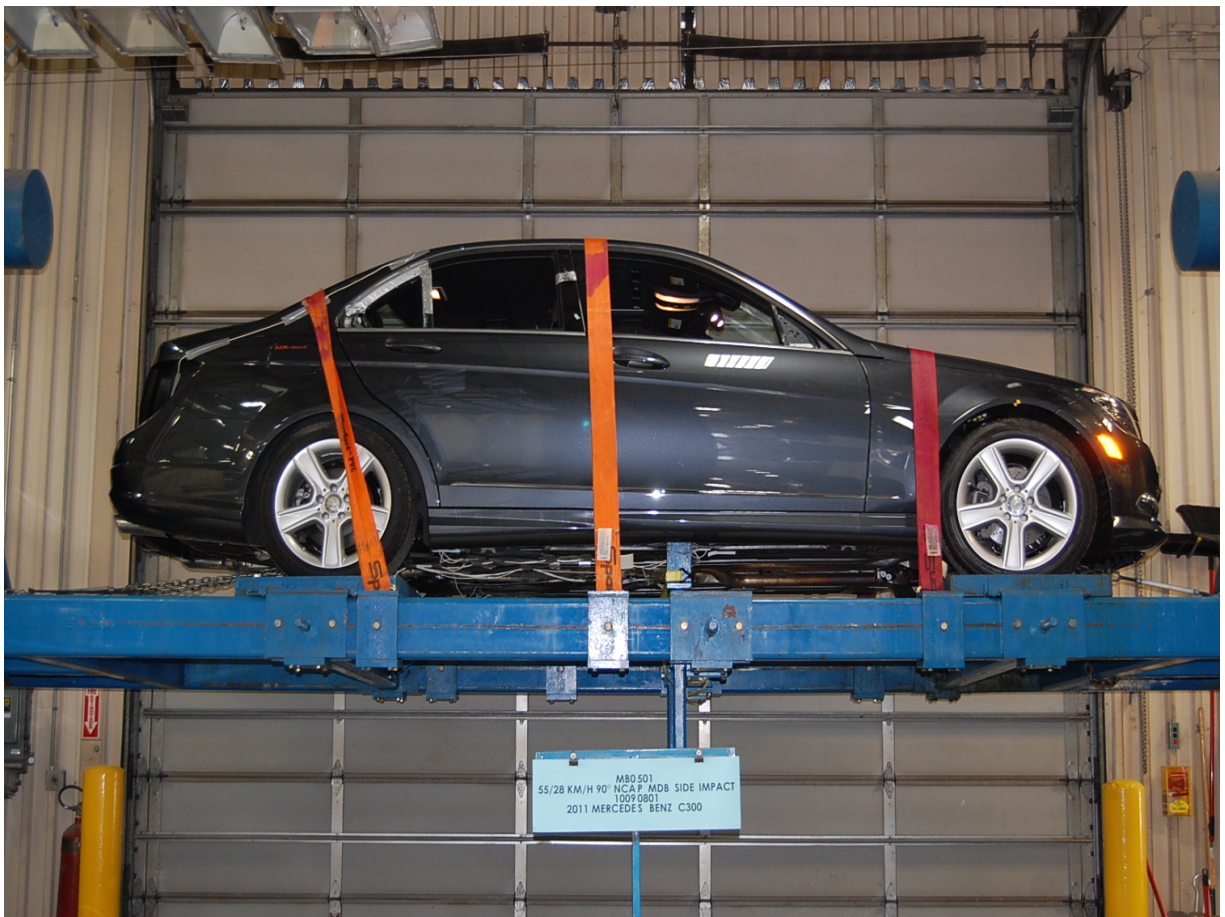
FMVSS No. 301/305 Rollover 0 Degrees
