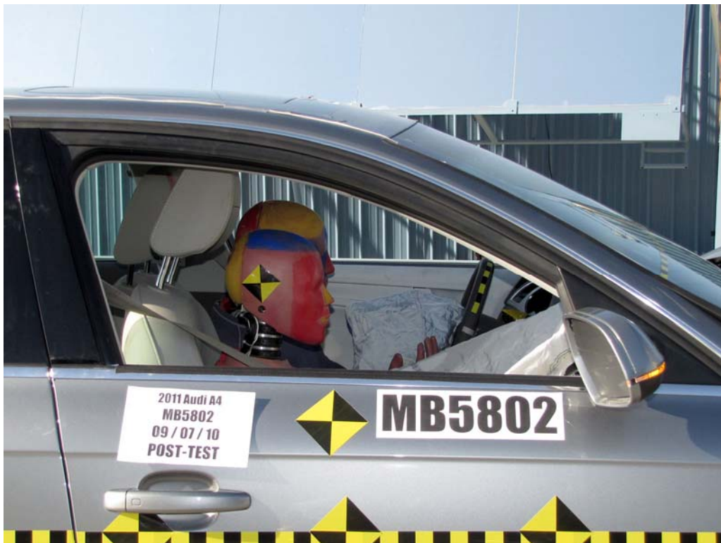
FIGURE 49. Post-Test Passenger Dummy Window View
