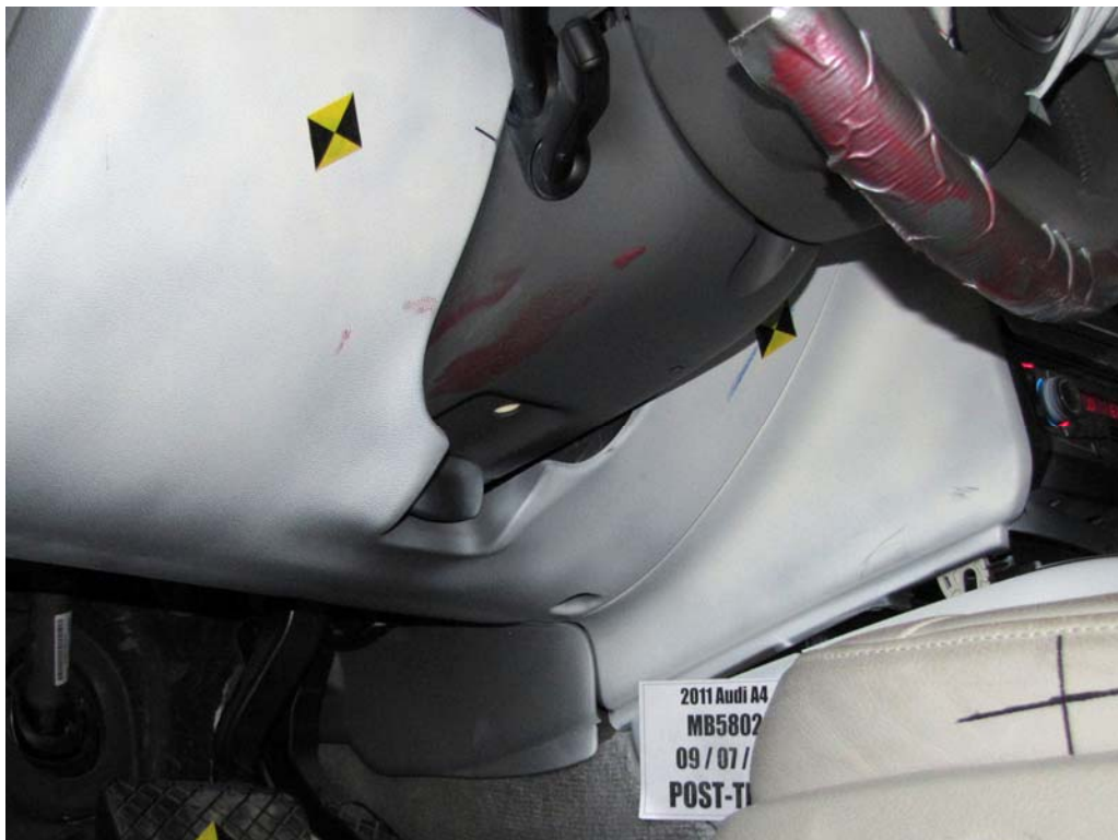
FIGURE 45. Post-Test View of Steering Column Shear Capsule
