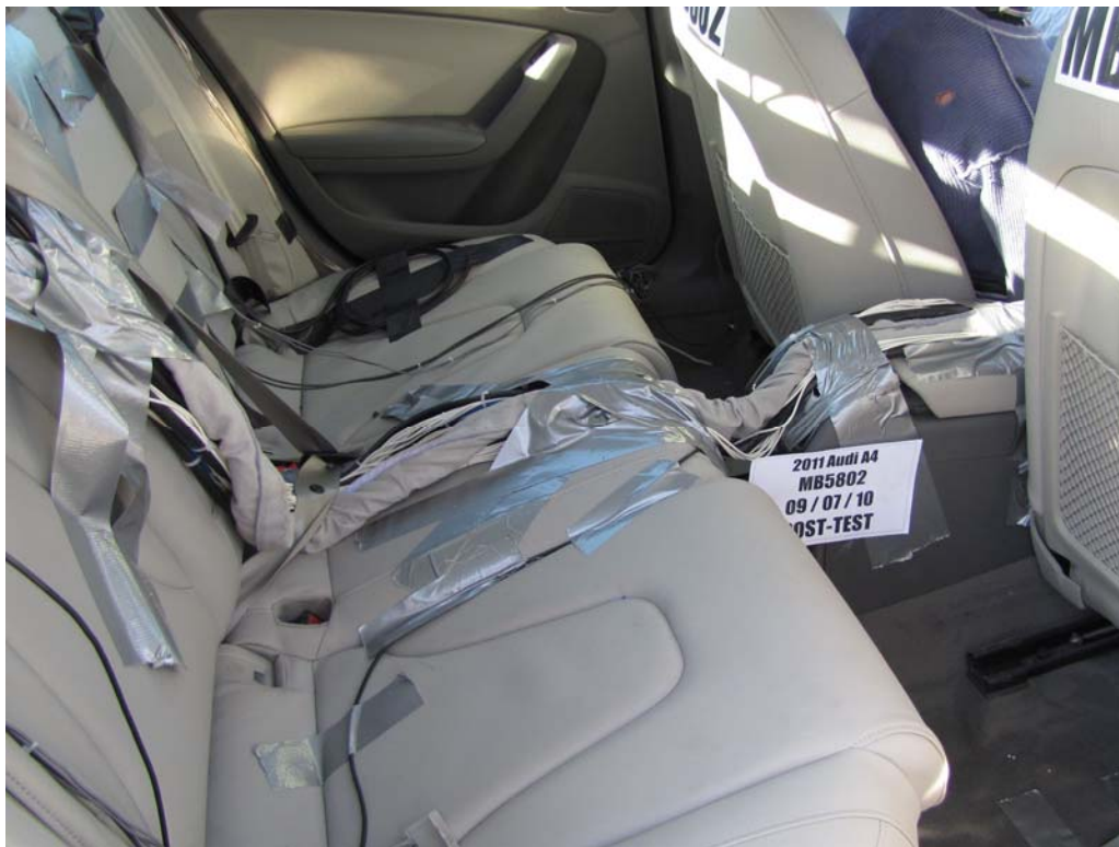
FIGURE 28. Post-Test Dummy Cable Routing
