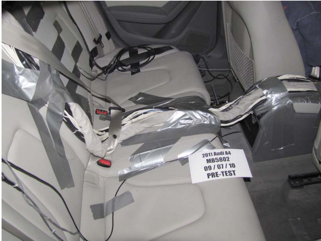
FIGURE 27. Pre-Test Dummy Cable Routing
