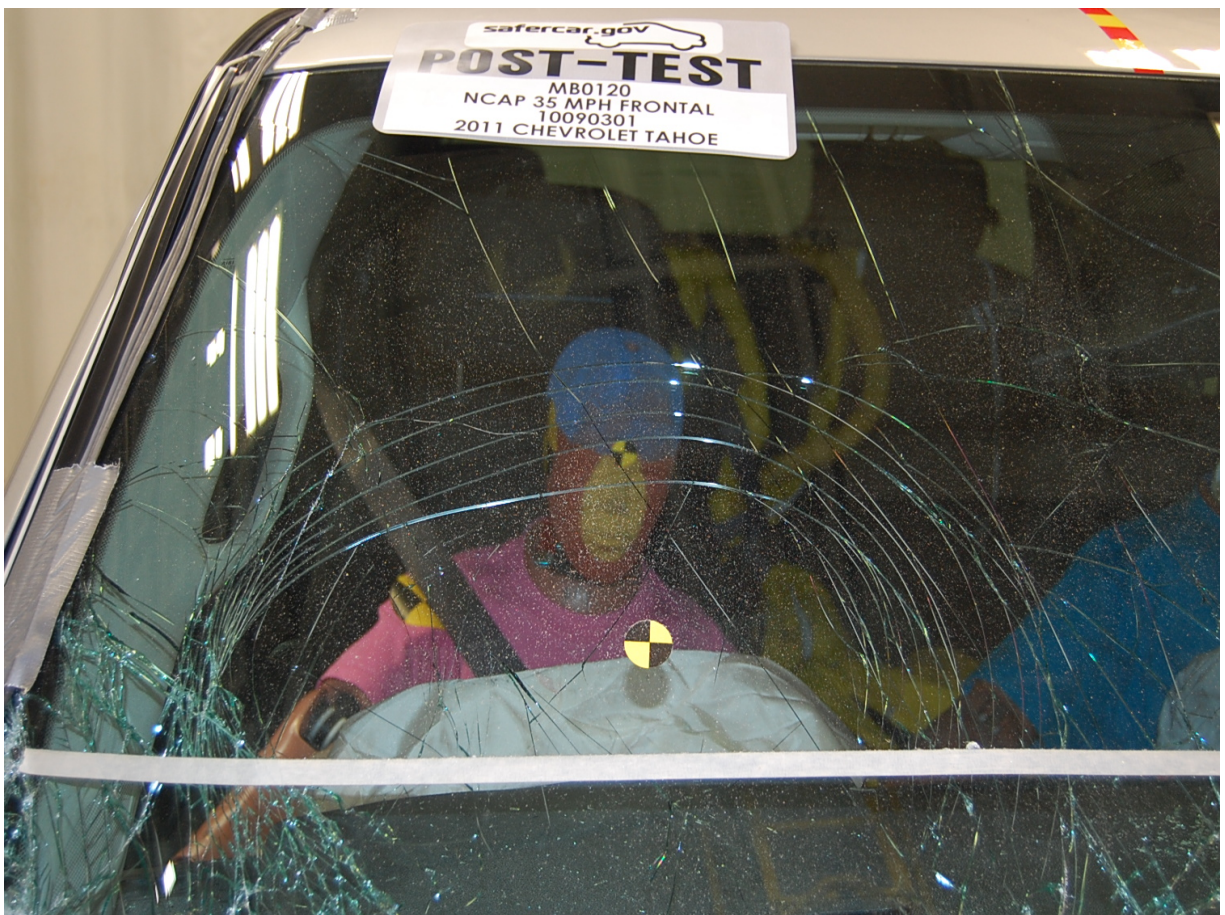
Post-Test Passenger Dummy Front View
