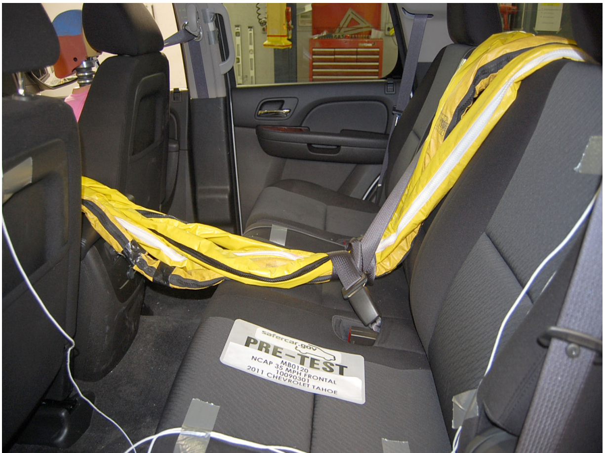
Pre-Test Dummy Cable Routing
