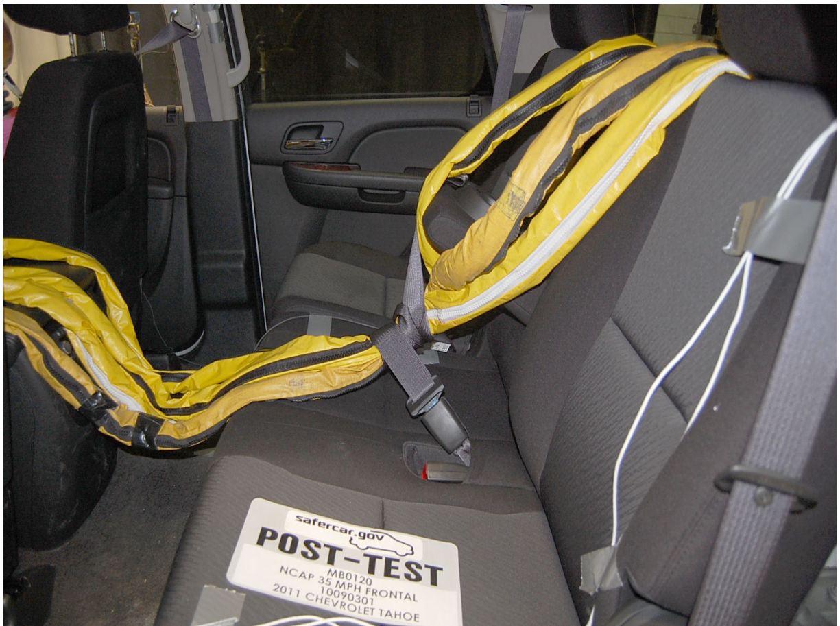
Post-Test Dummy Cable Routing
