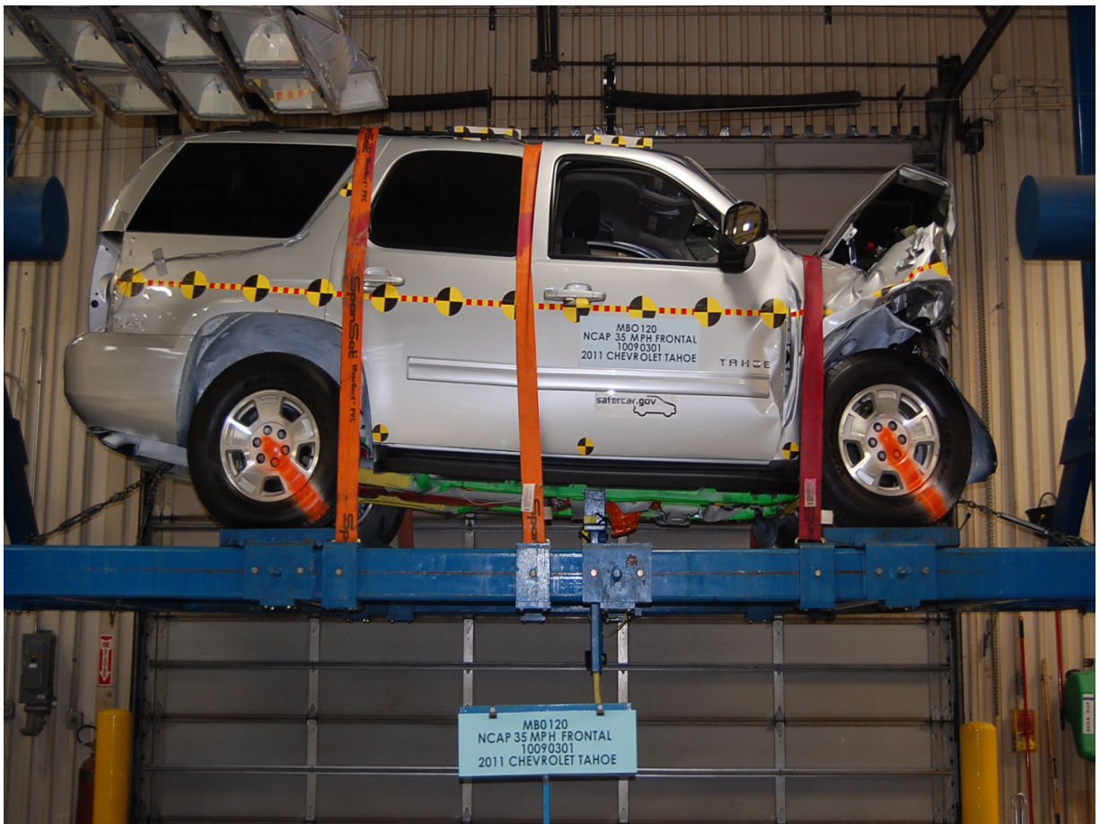
Vehicle at 0 Degrees on Static Rollover Device
