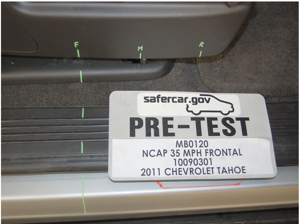
Pre-Test Passenger's Seat Fore-Aft Markings
