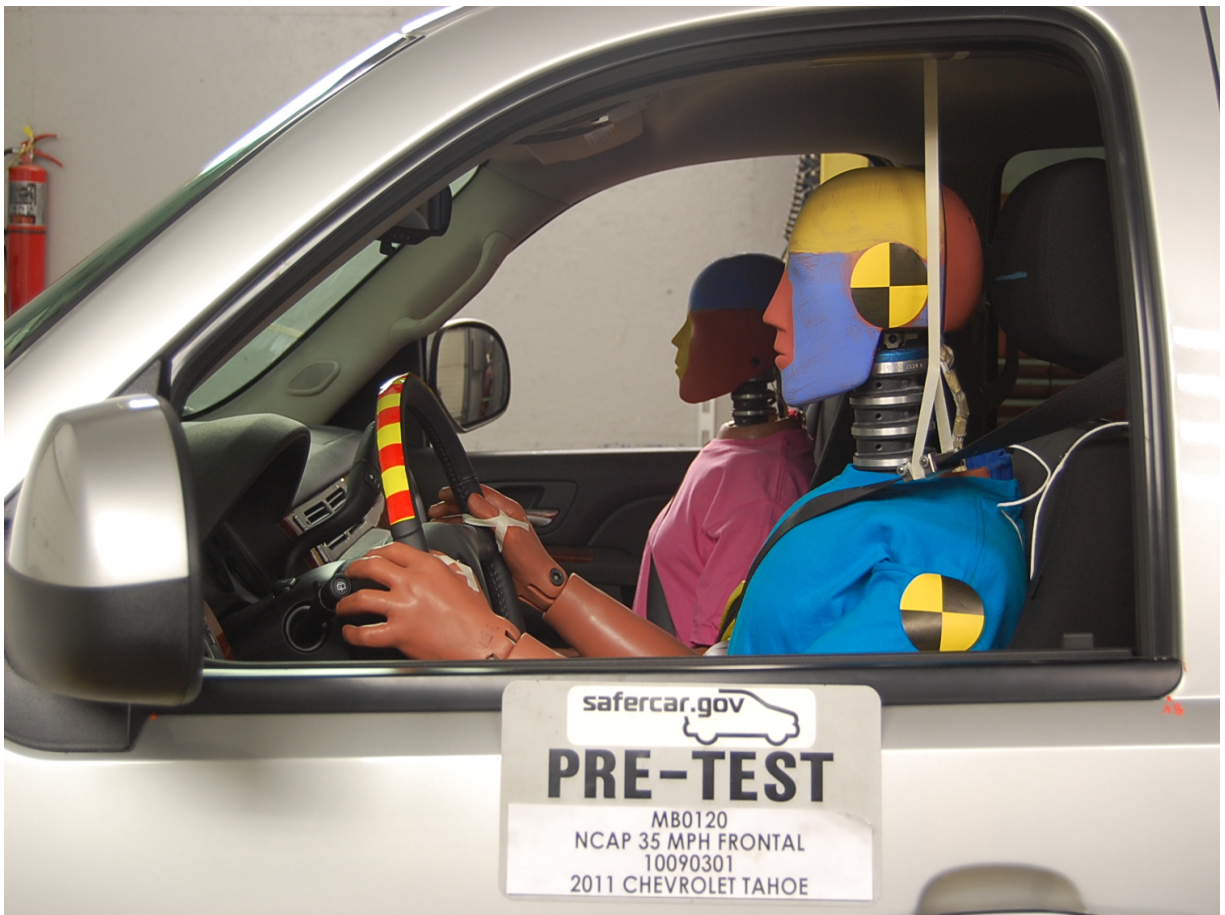
Pre-Test Driver Dummy Window View
