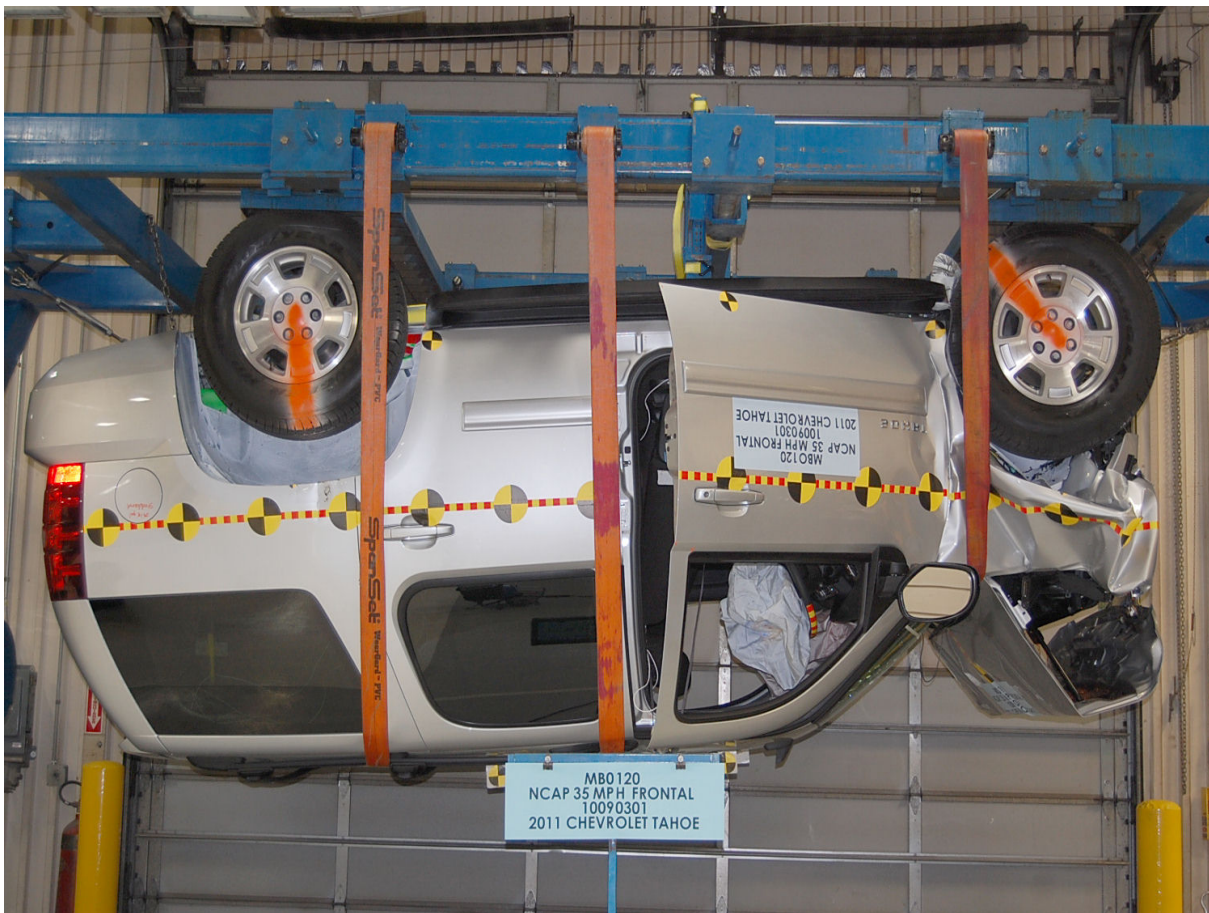
Vehicle at 180 Degrees on Static Rollover Device
