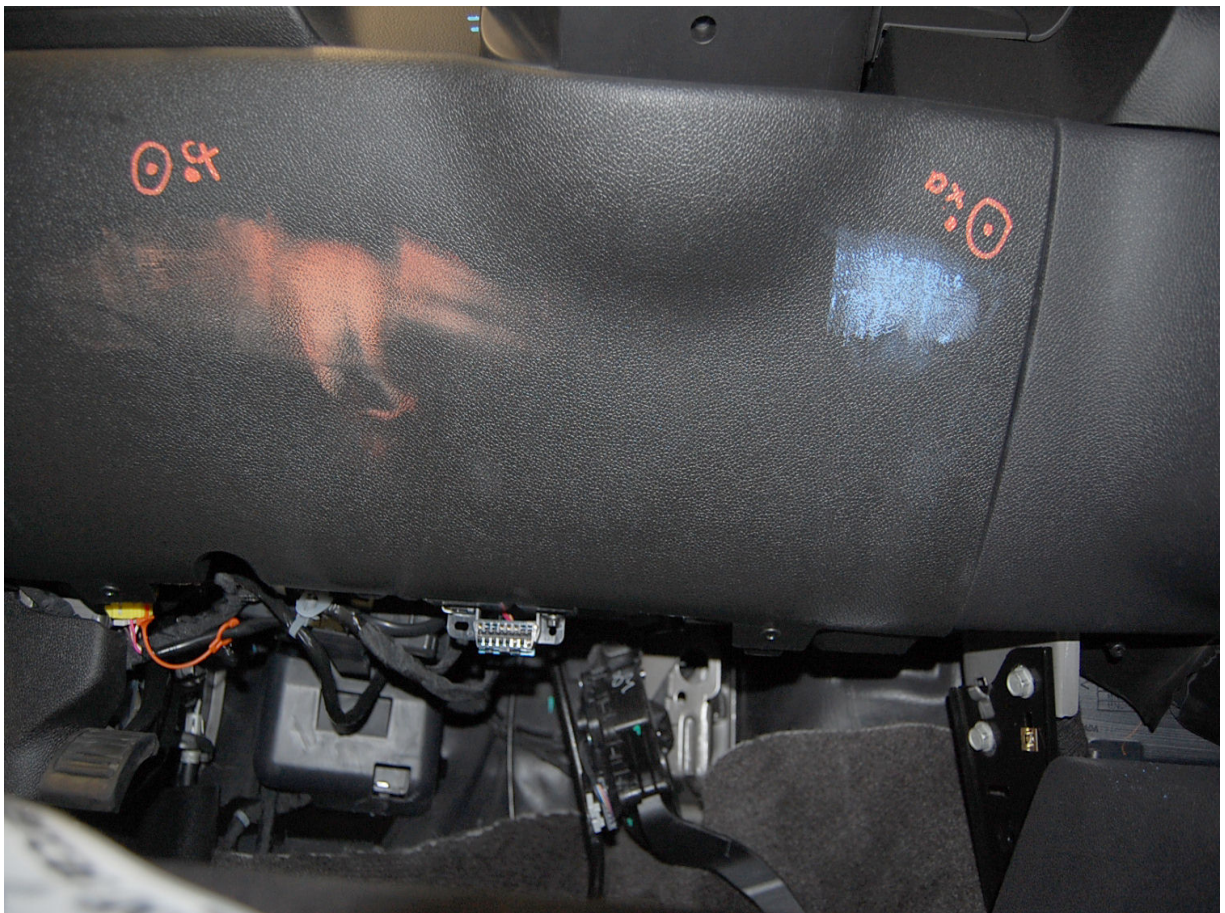
Post-Test Driver Dummy Contact with Knee Bolster
