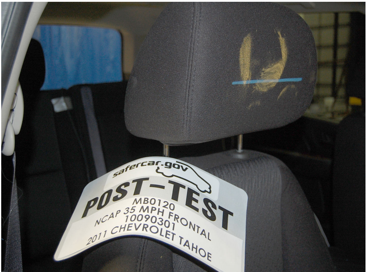
Post-Test Passenger Dummy Contact with Headrest
