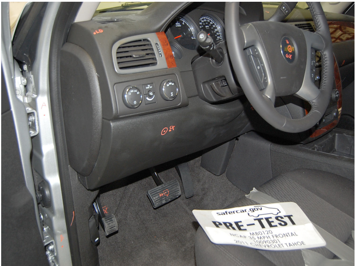
Pre-Test Driver's Side Knee Bolster (without dummy)
