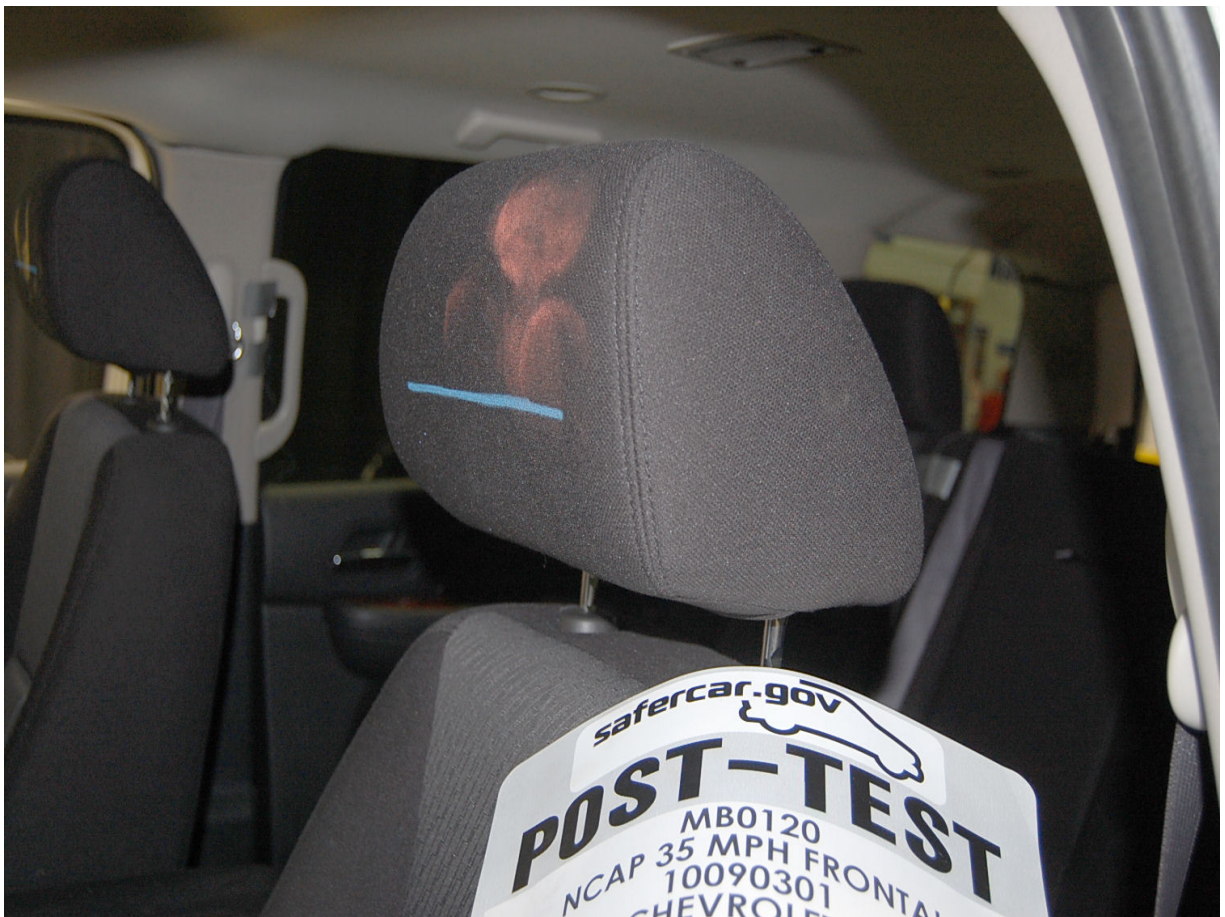
Post-Test Driver Dummy Contact with Headrest
