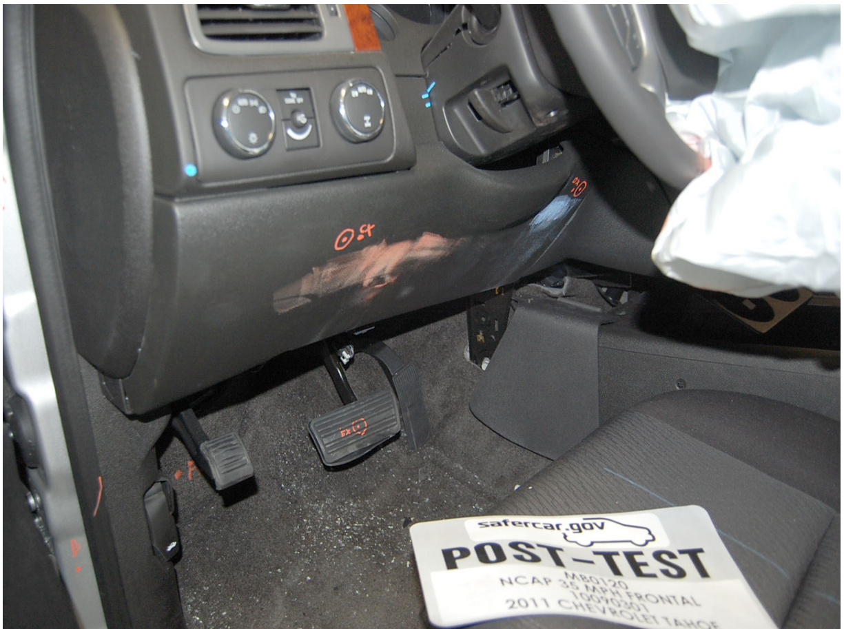
Post-Test Driver's Side Knee Bolster (without dummy)
