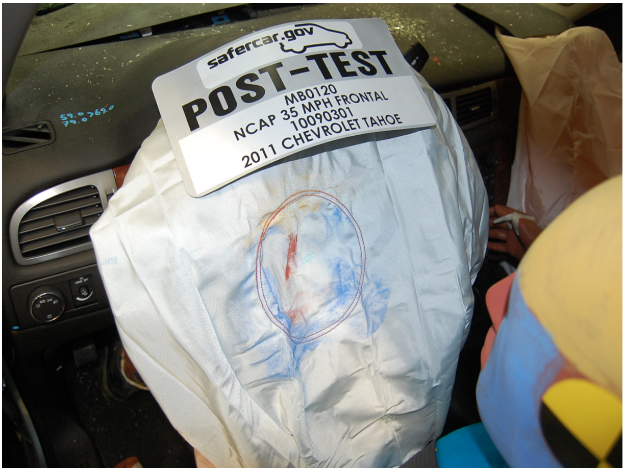
Post-Test Driver Dummy Contact with Airbag
