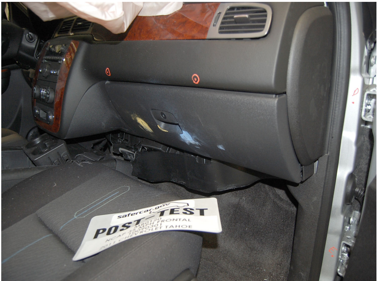
Post-Test Passenger's Side Knee Bolster (without dummy)
