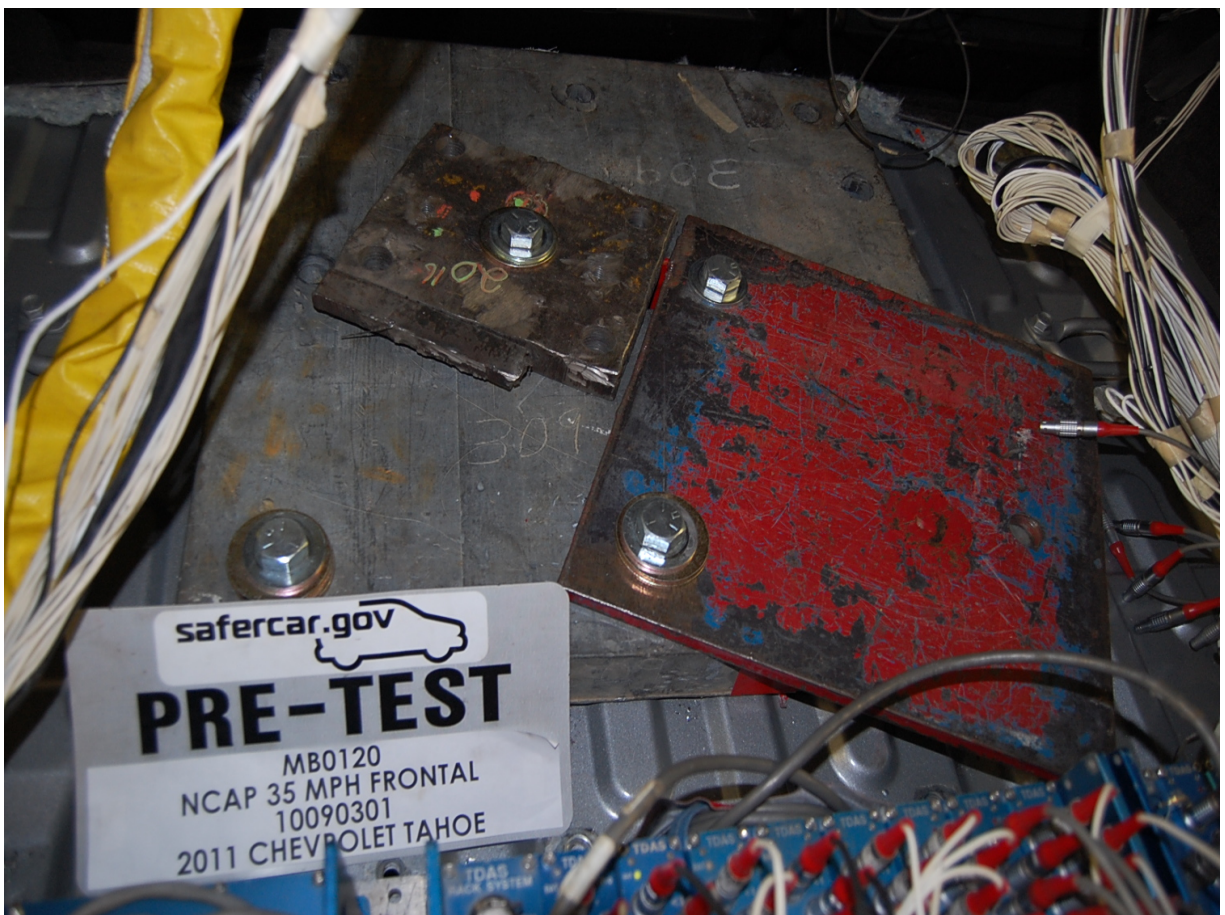
Ballast Installed in Vehicle
