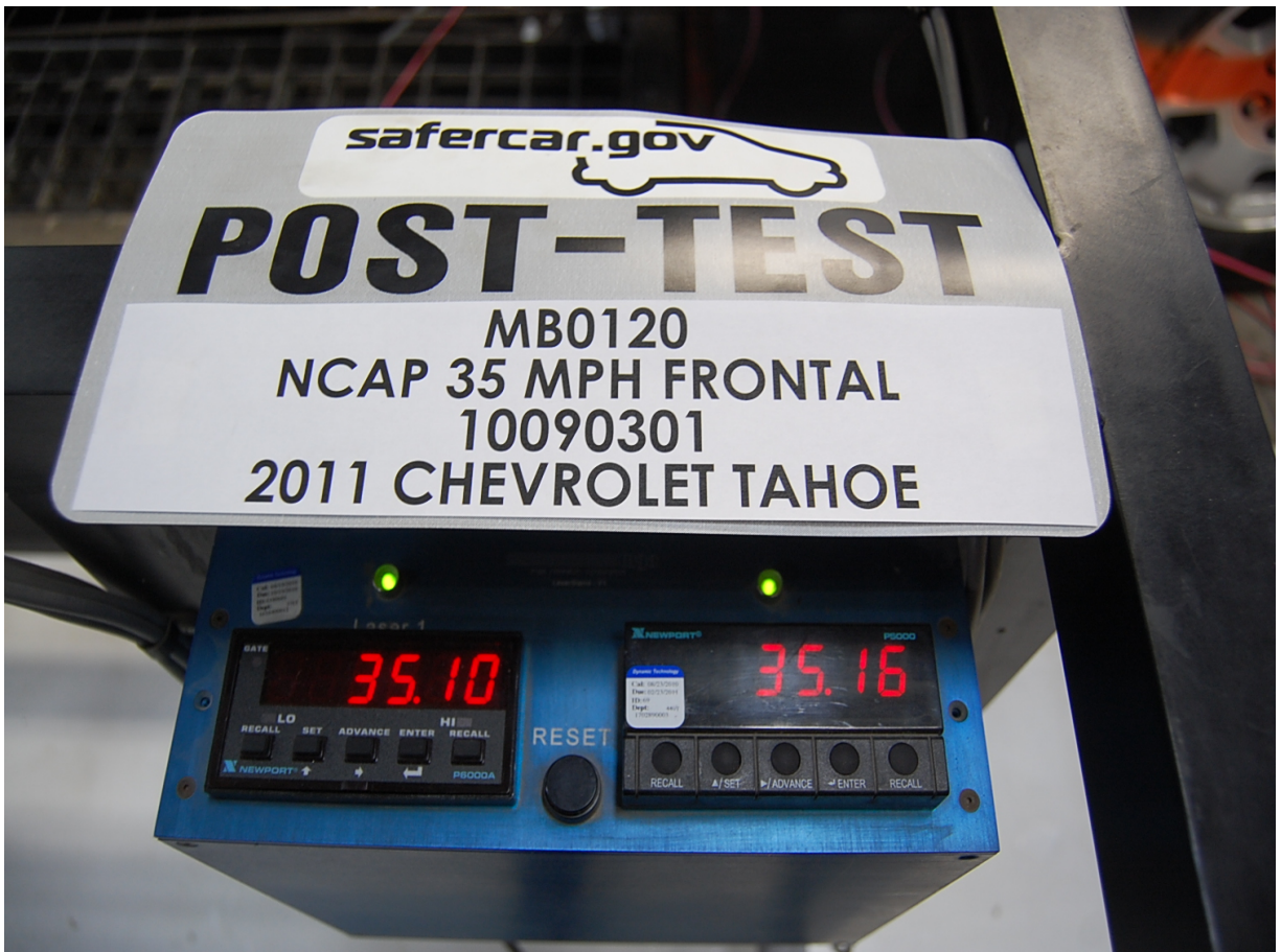
Post-Test Speed Trap Read-Out
