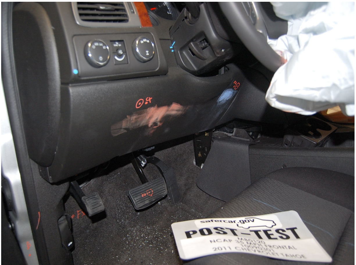
Post-Test View of Steering Column Shear Capsule
