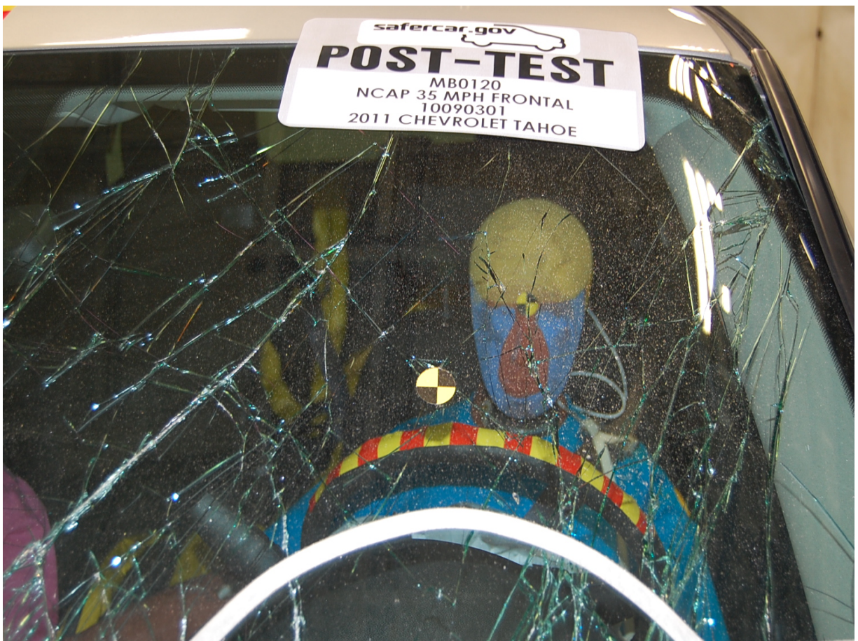
Post-Test Driver Dummy Front View
