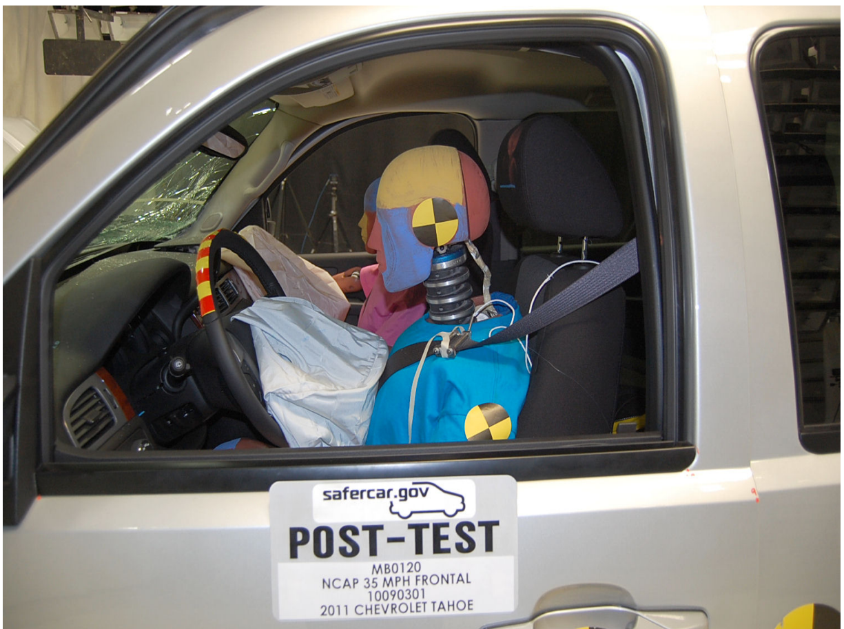
Post-Test Driver Dummy Window View
