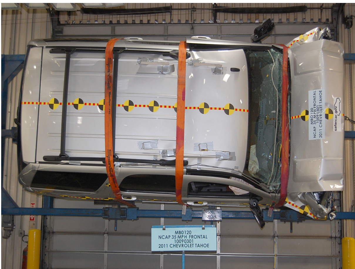
Vehicle at 270 Degrees on Static Rollover Device
