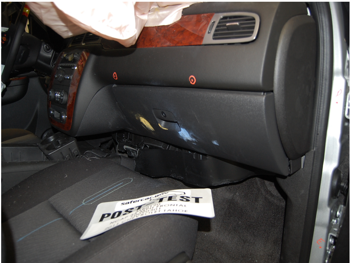
Post-Test Passenger Dummy Contact with Glovebox
