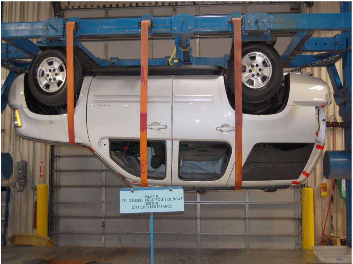
FMVSS No. 301/305 Rollover 180 Degrees
