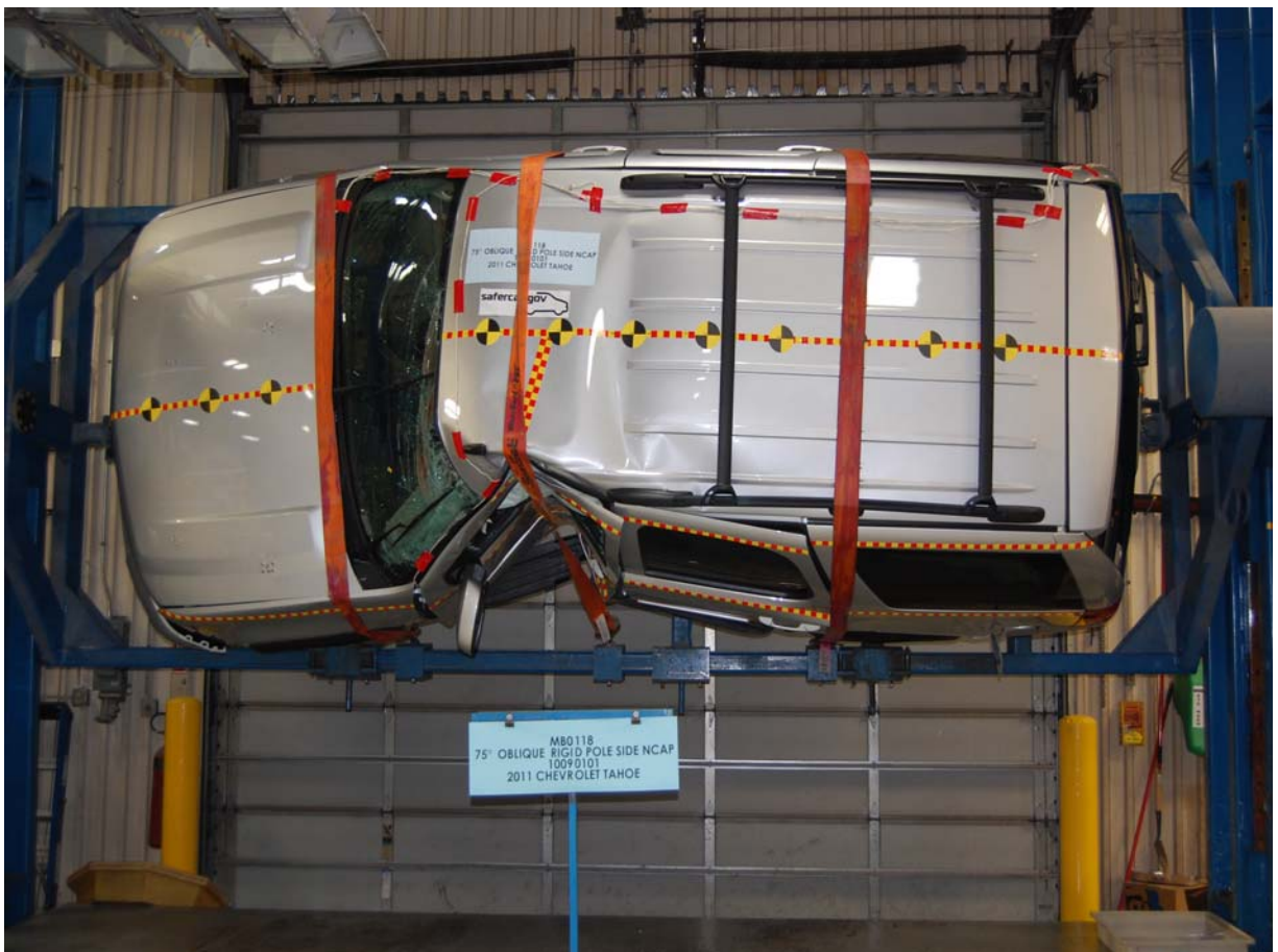
FMVSS No. 301/305 Rollover 90 Degrees
