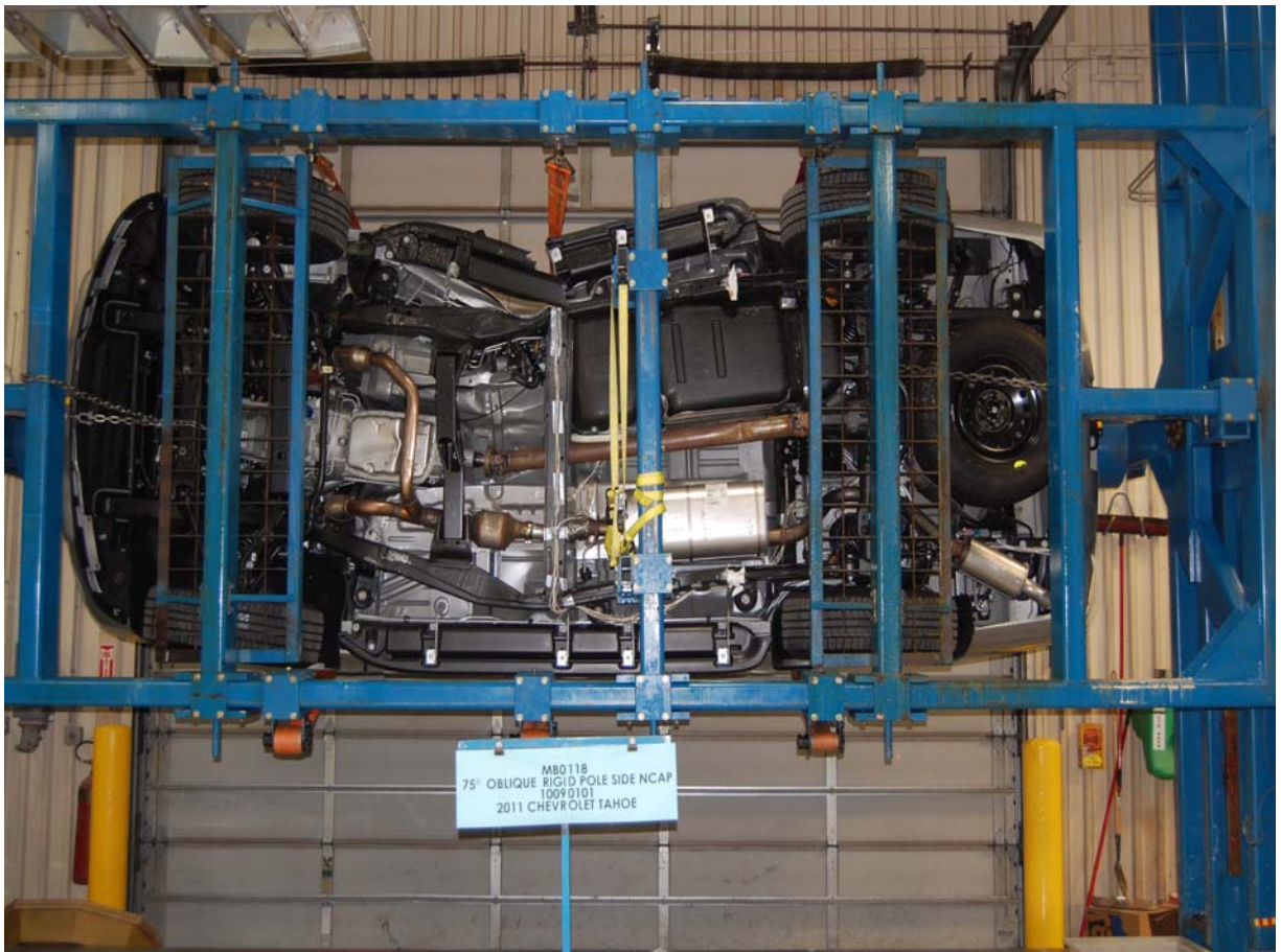
FMVSS No. 301/305 Rollover 270 Degrees
