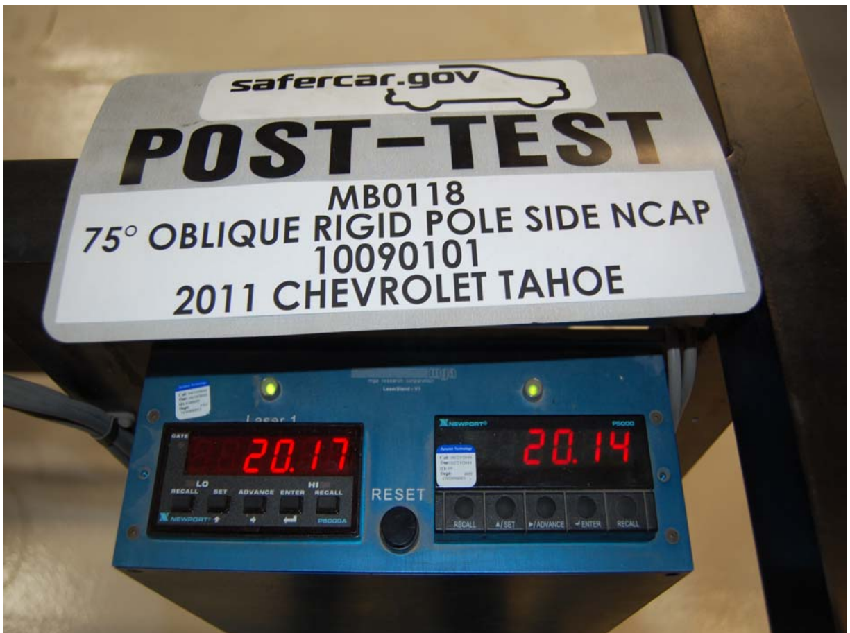
Post-Test Primary and Redundant Speed Trap Read-Out
