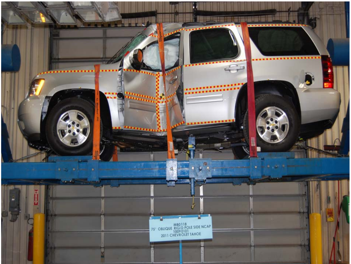
FMVSS No. 301/305 Rollover 0 Degrees
