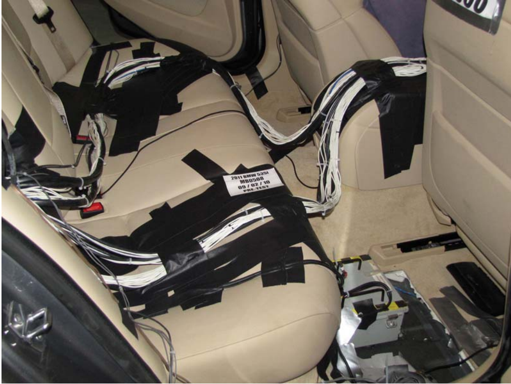
FIGURE 27. Pre-Test Dummy Cable Routing
