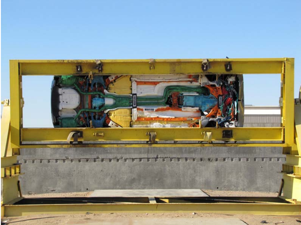
FIGURE 67. Vehicle at 270 Degrees on Static Rollover Device
