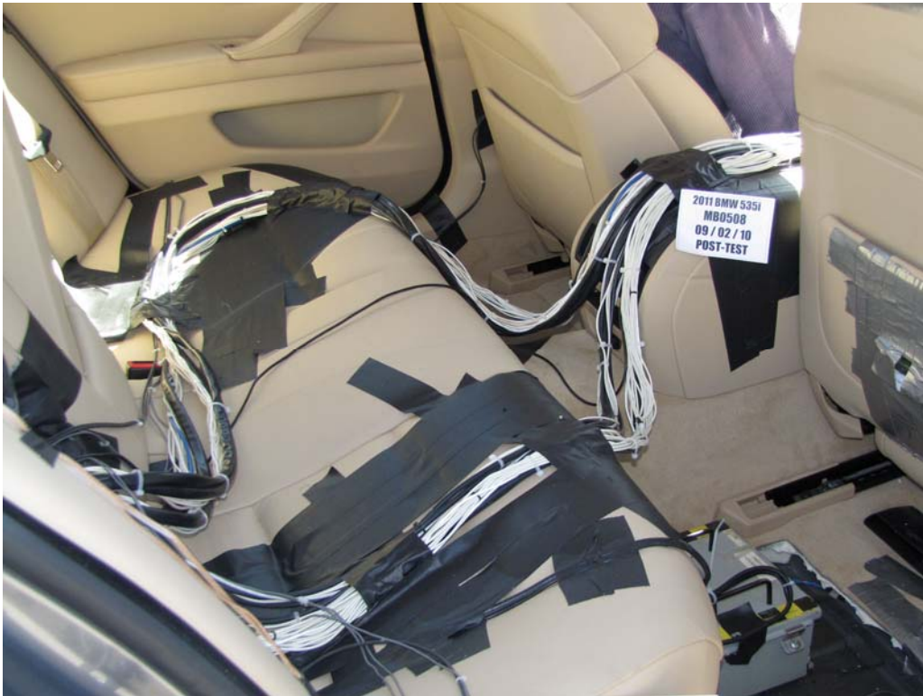
FIGURE 28. Post-Test Dummy Cable Routing
