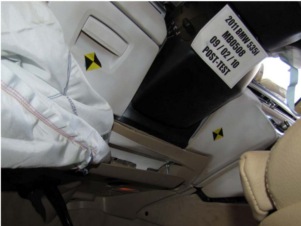
FIGURE 45. Post-Test View of Steering Column Shear Capsule
