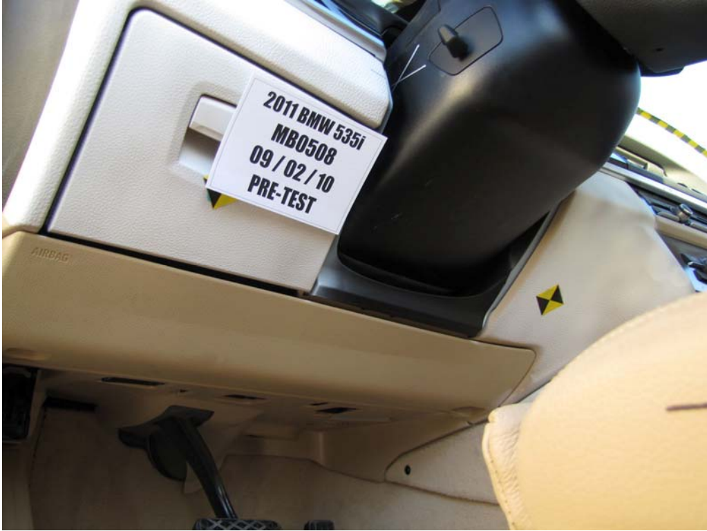
FIGURE 44. Pre-Test View of Steering Column Shear Capsule
