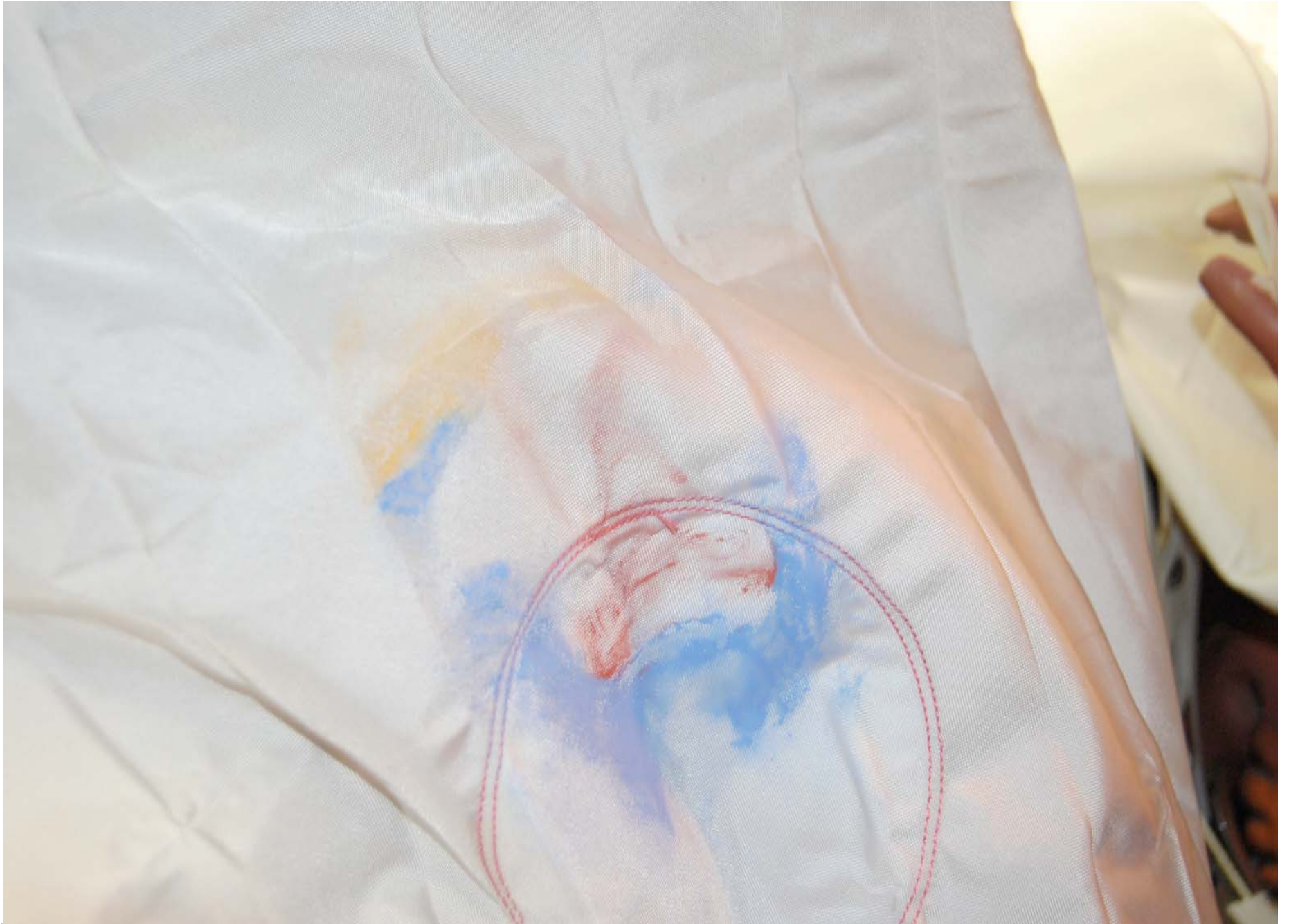
Post-Test Driver Dummy Airbag Contact
