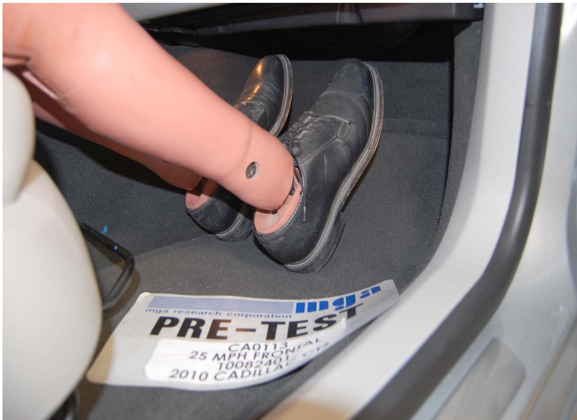
Pre-Test Passenger Dummy Feet Position
