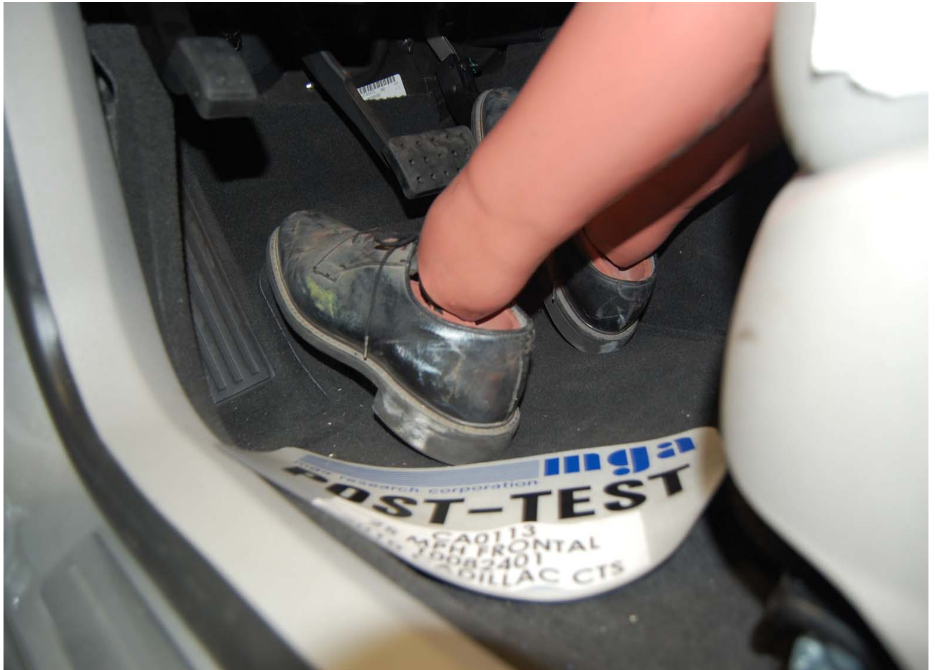
Post-Test Driver Dummy Feet Position
