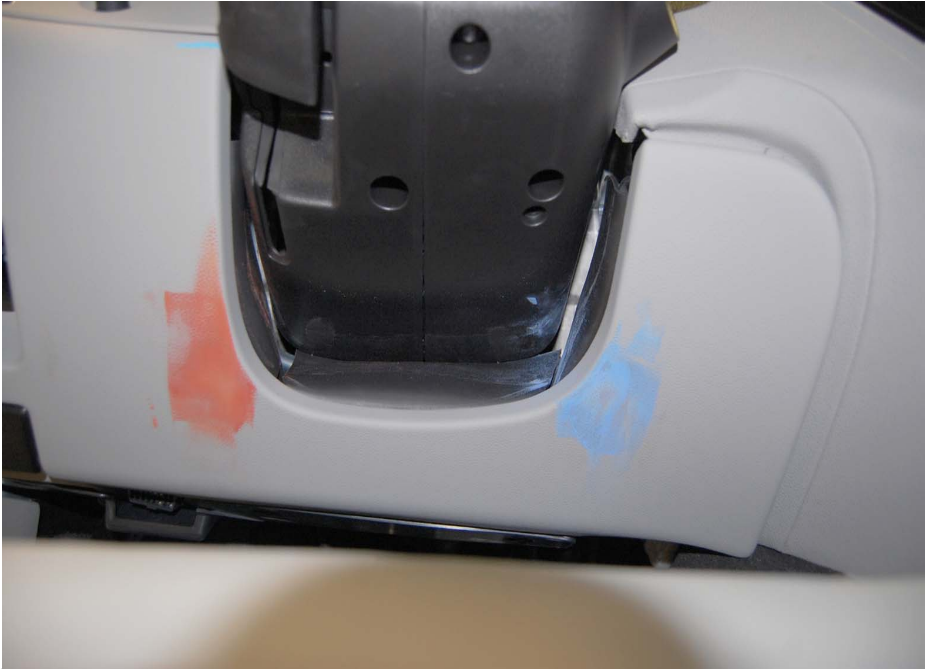
Post-Test Driver Dummy Knee Contact
