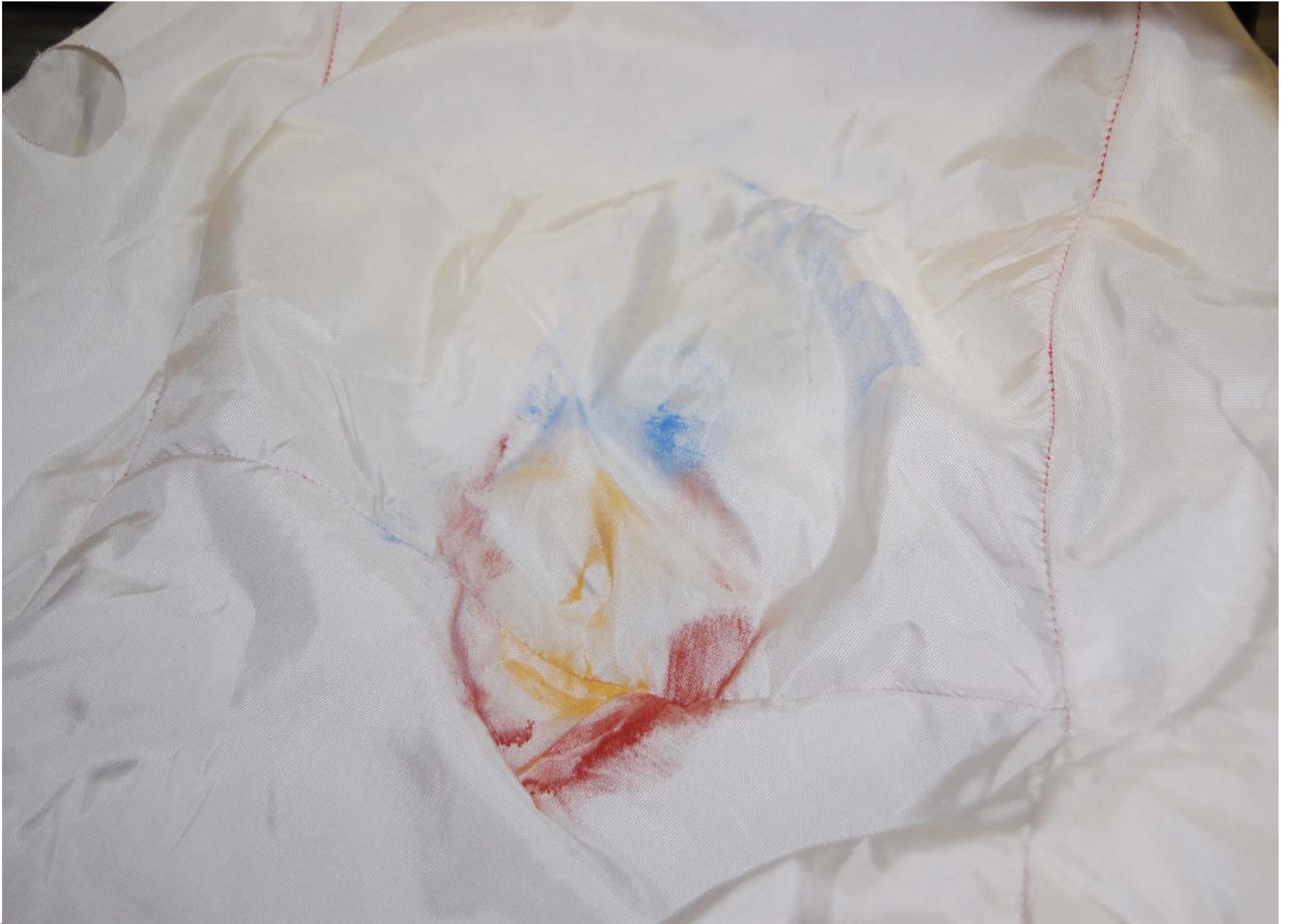
Post-Test Passenger Dummy Airbag Contact View 1
