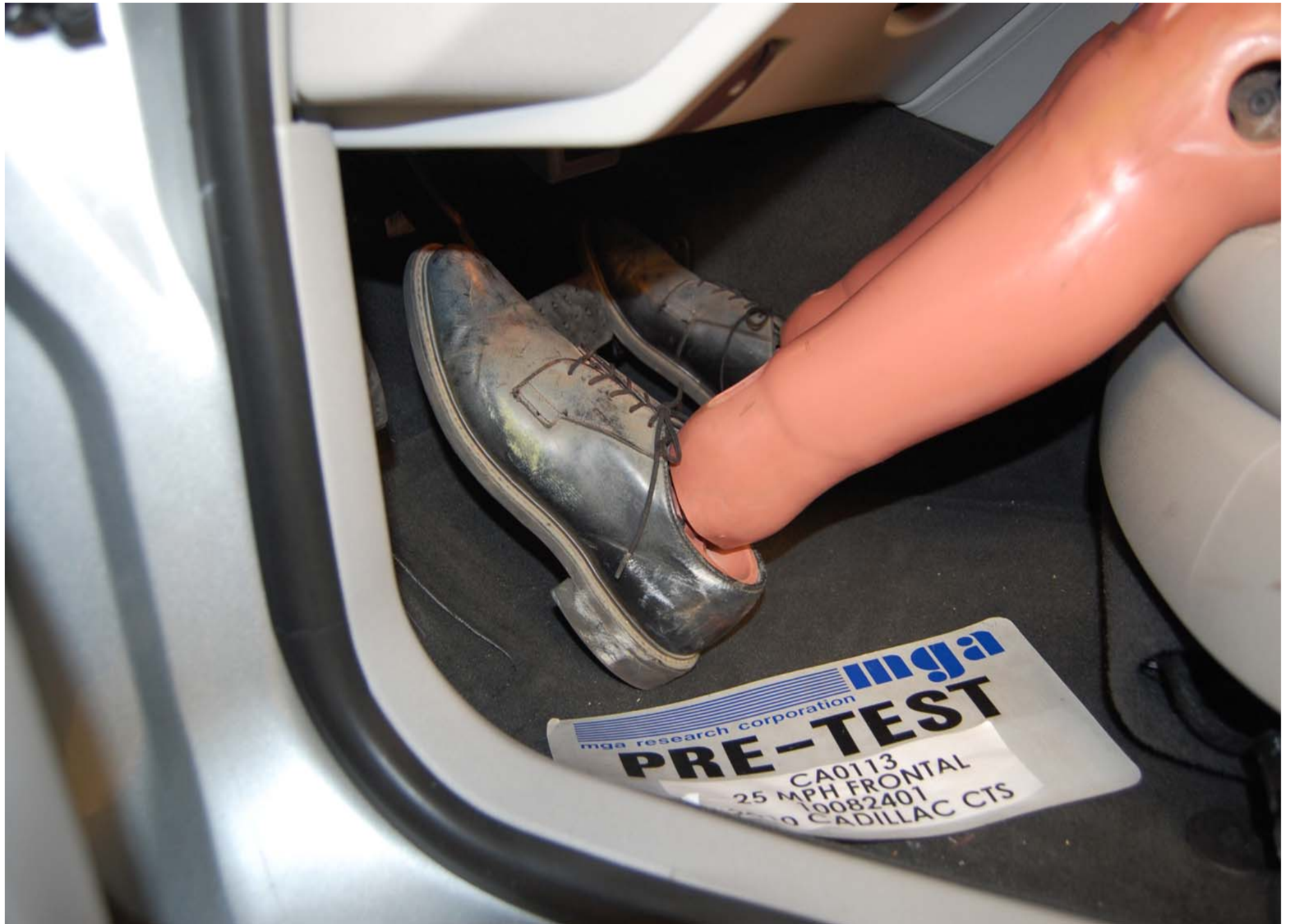
Pre-Test Driver Dummy Feet Position
