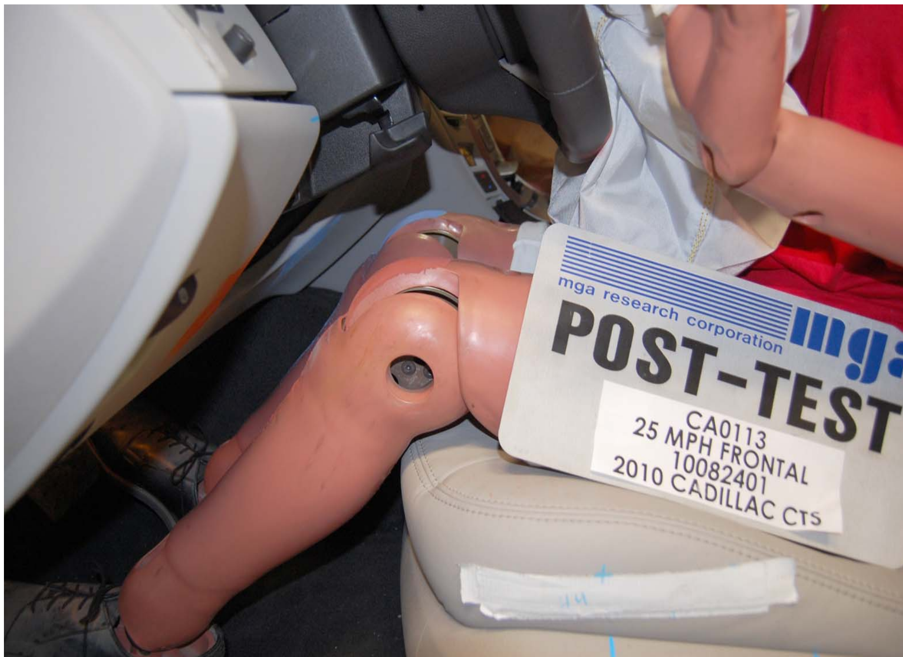
Post-Test Driver Side Knee Bolster View
