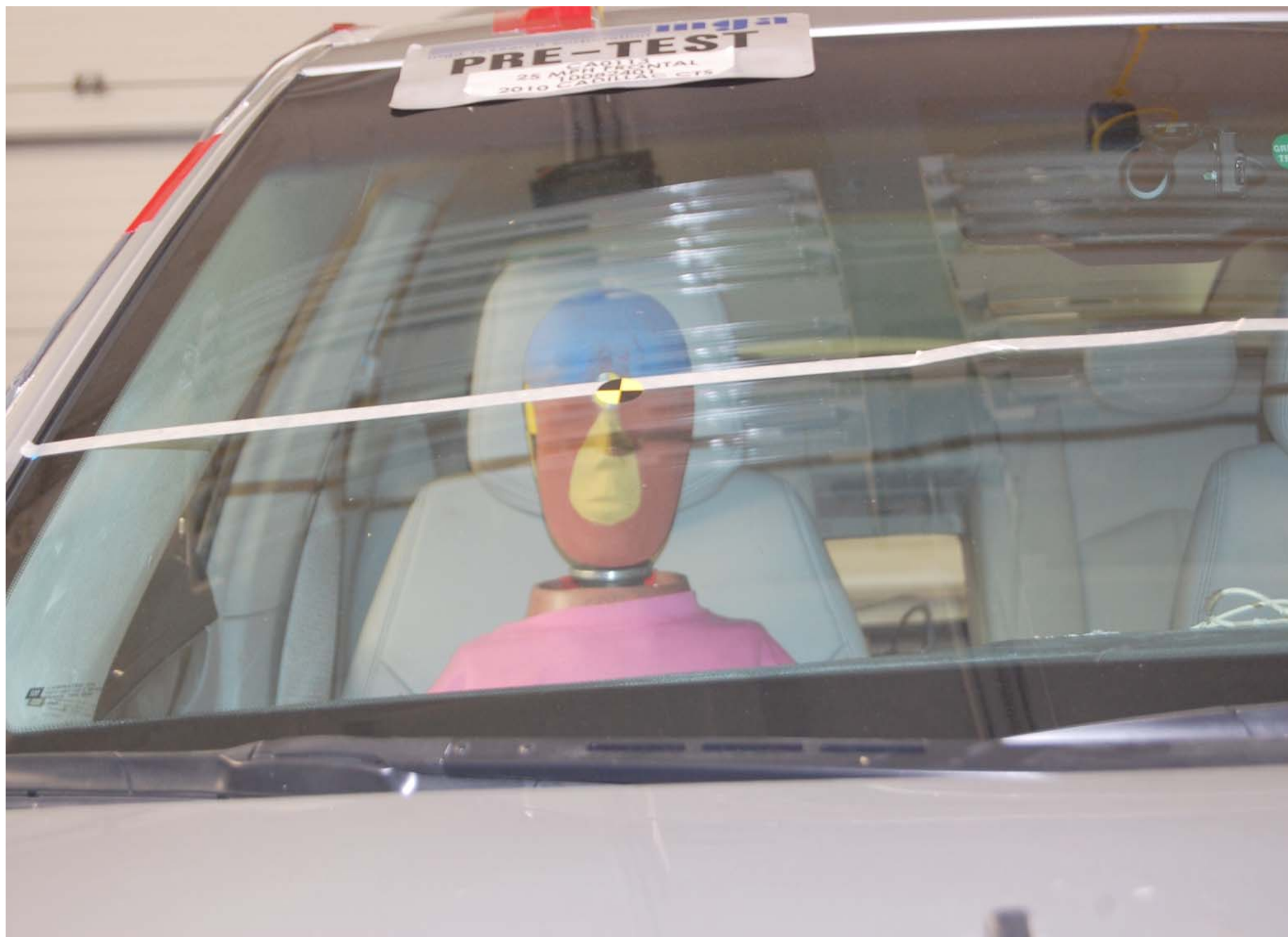
Pre-Test Passenger Dummy Front View (head position)
