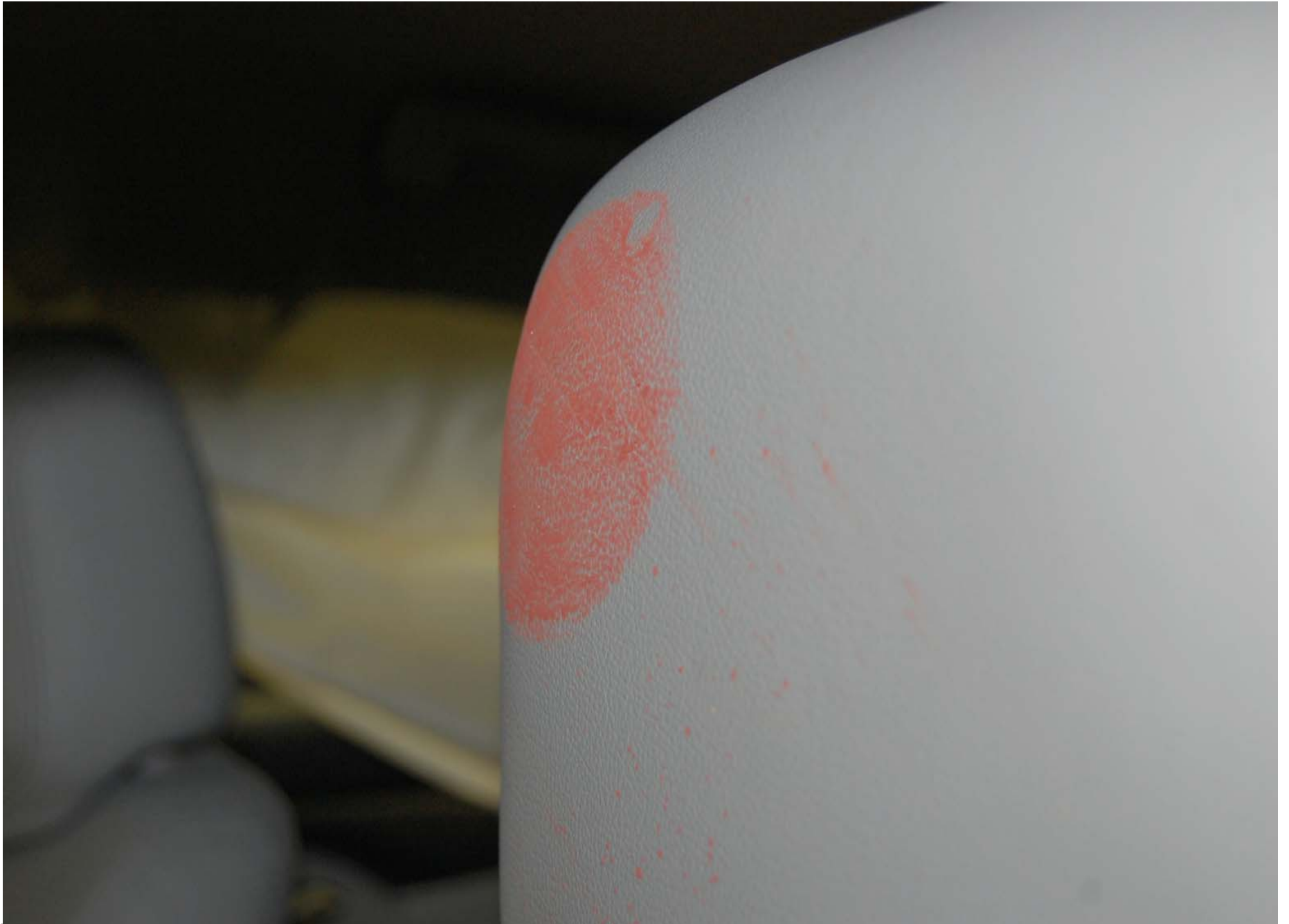
Post-Test Driver Dummy Head Contact (headrest)
