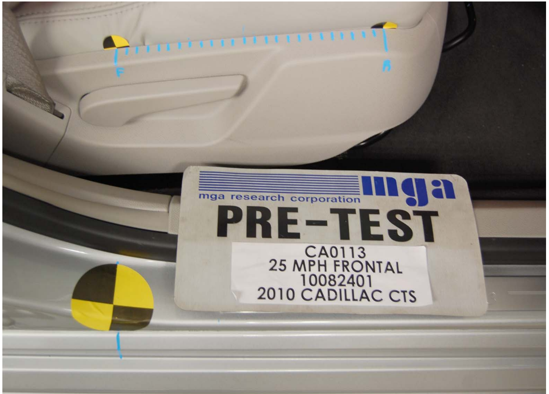
Pre-Test Passenger Dummy Seat Position
