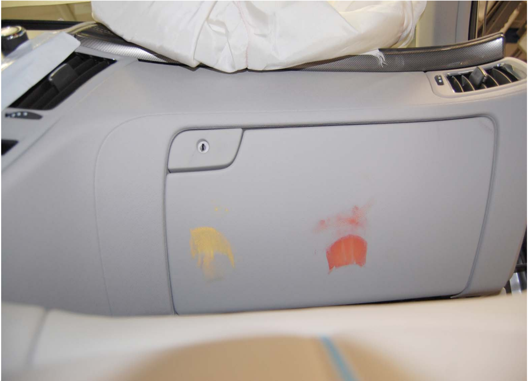
Post-Test Passenger Dummy Knee Contact
