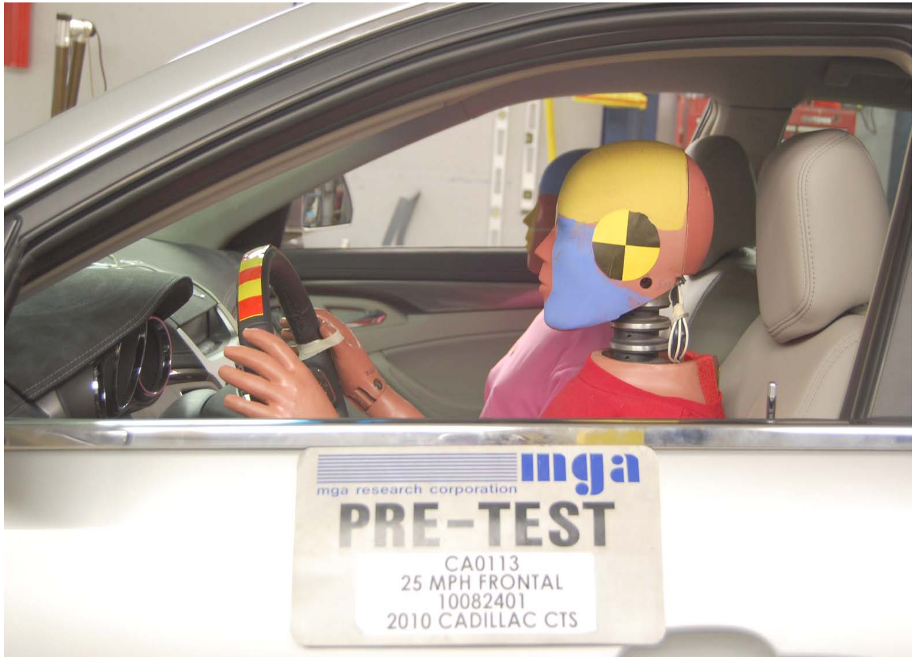
Pre-Test Driver Dummy Position Left Side View
