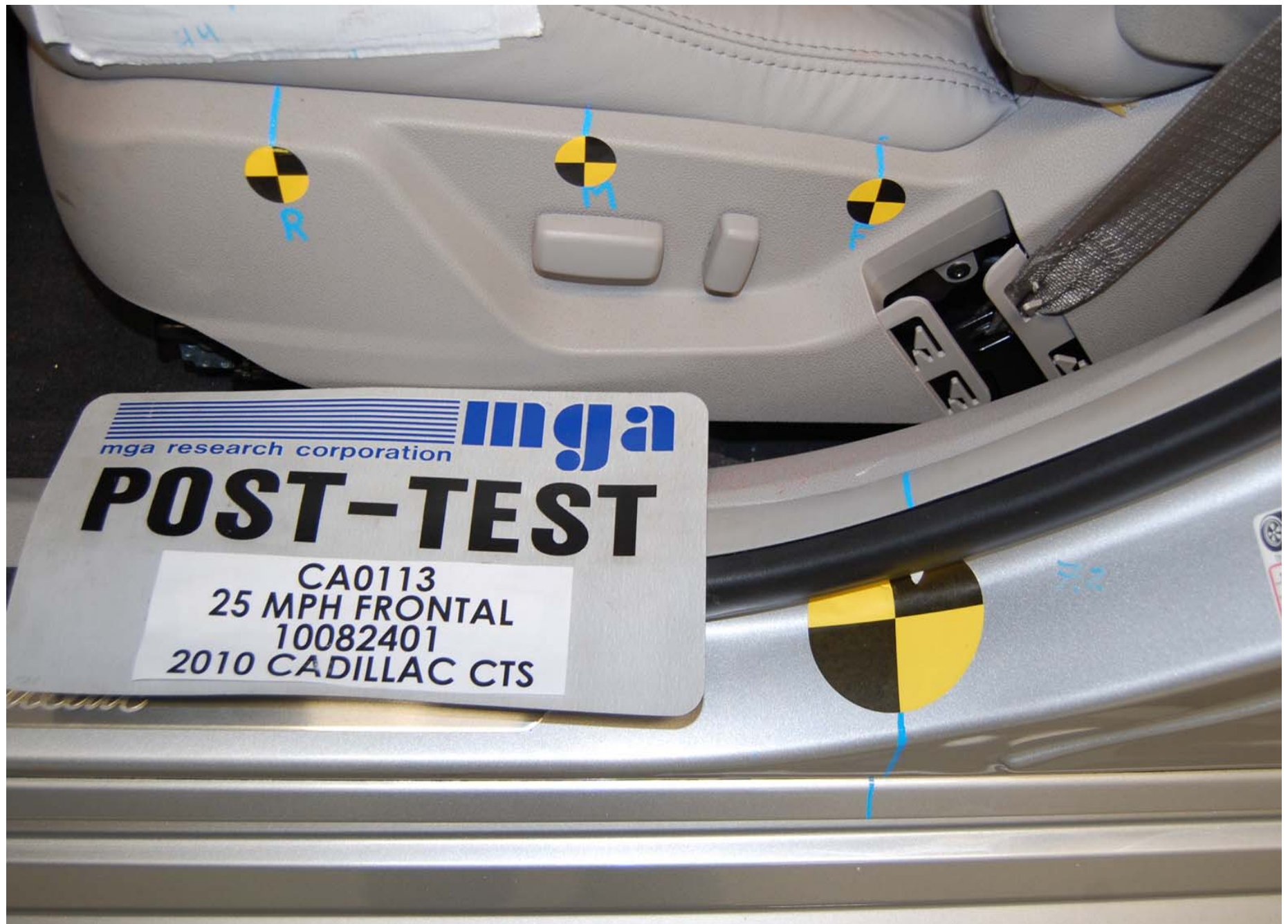
Post-Test Driver Dummy Seat Position
