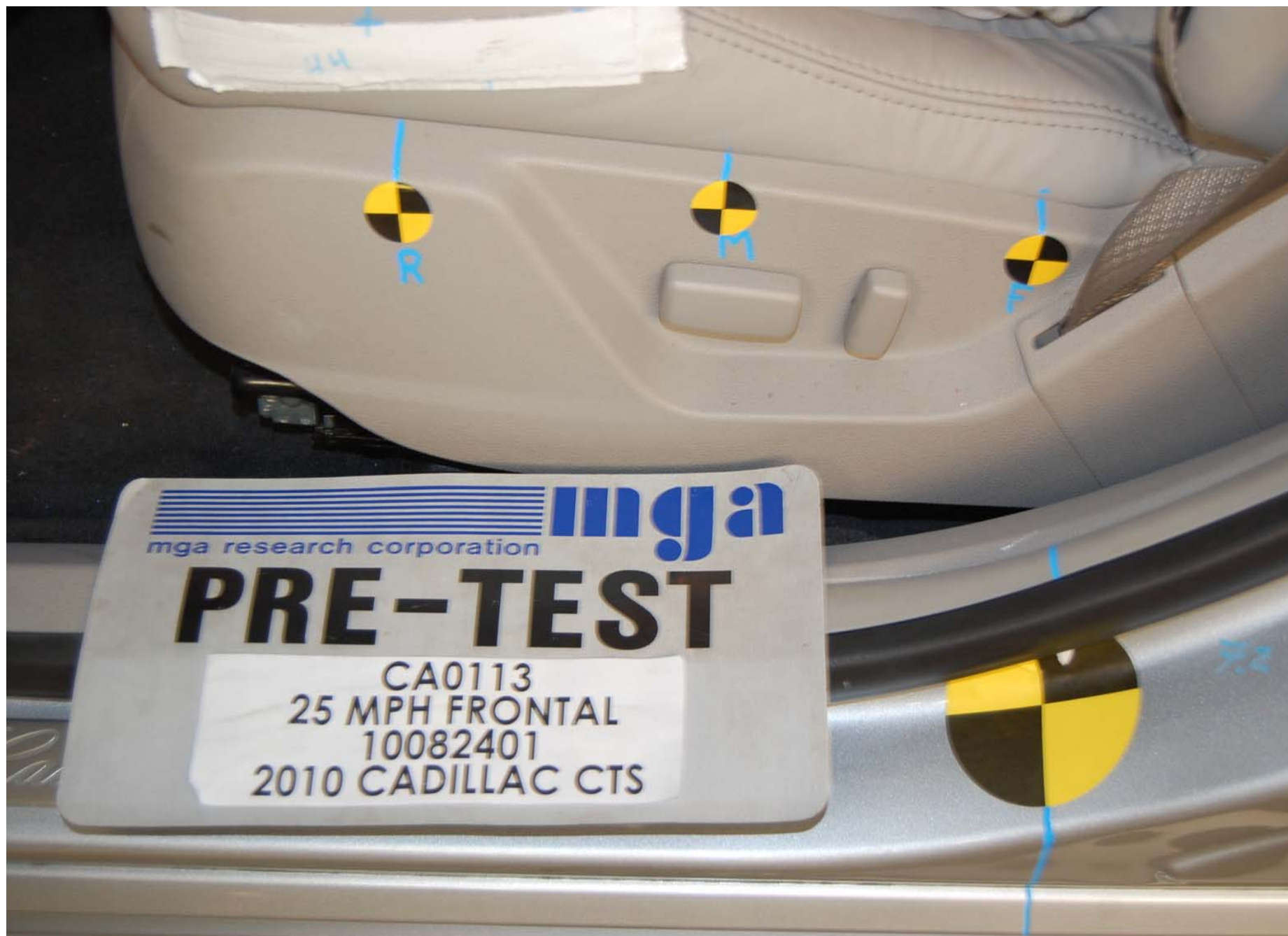
Pre-Test Driver Dummy Seat Position
