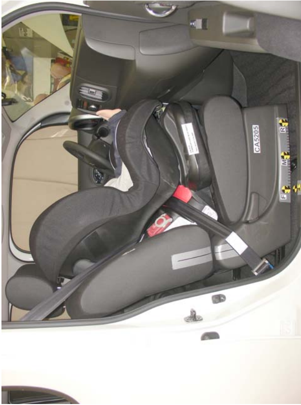
Graco Safeseat Forward Facing Belted, Forward Seat Track
