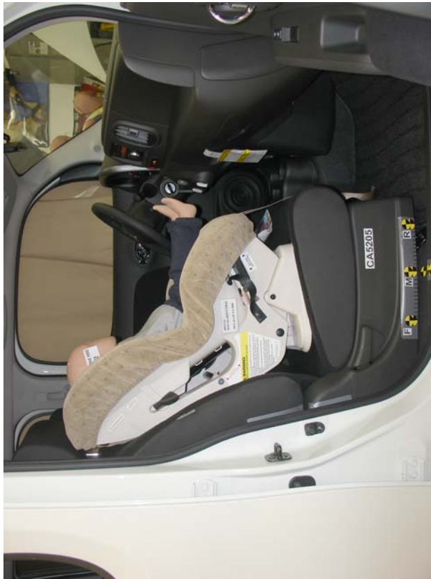
Britax Roundabout Forward Facing Unbelted, Middle Seat Track
