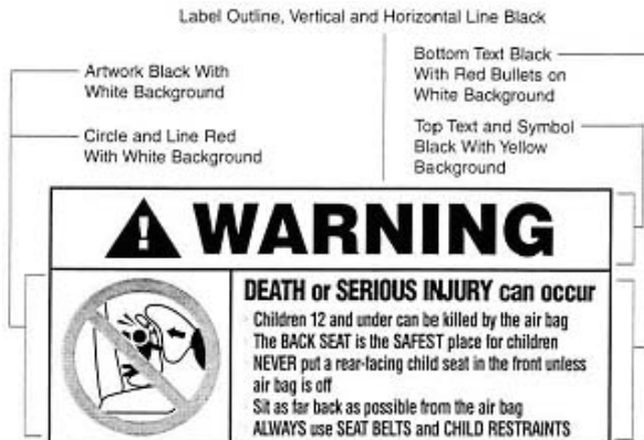
Figure 6b. Sun Visor Label Visible When Visor is in Down Position.
