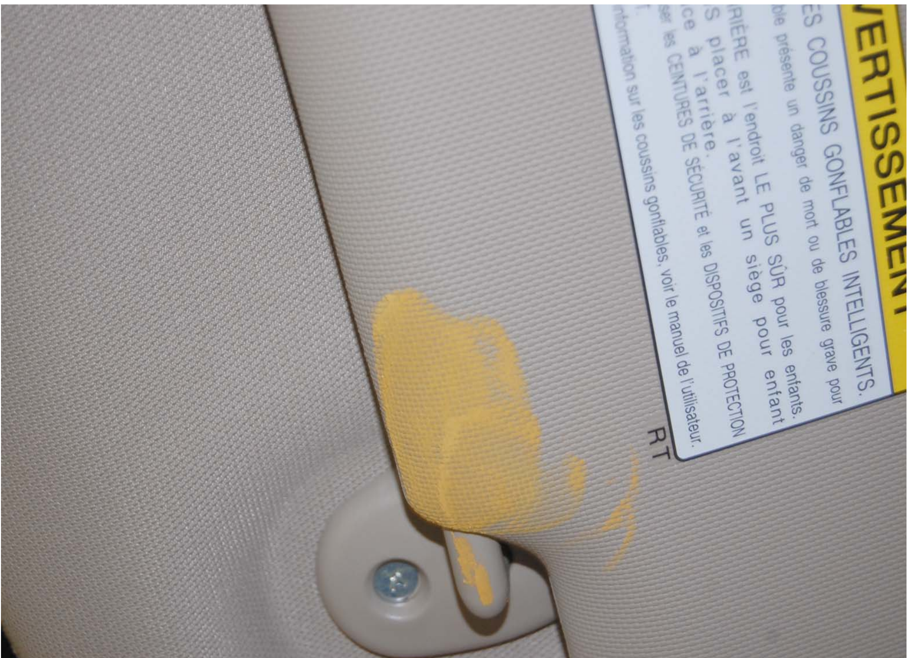
Post-Test Passenger Dummy Head Contact (visor)
