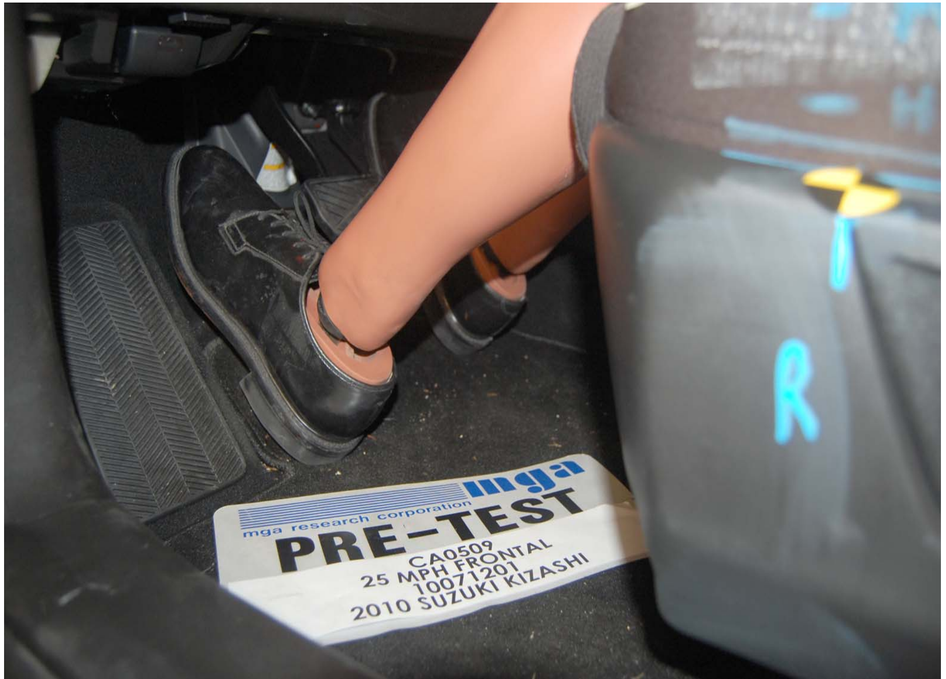
Pre-Test Driver Dummy Feet Position
