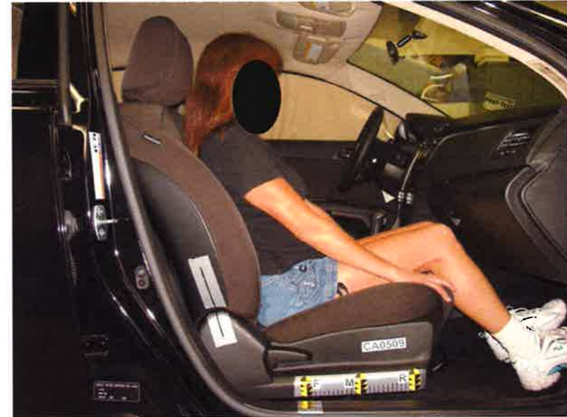
Unbelted 5th Percentile Female Reactivation, Forward Seat Track
