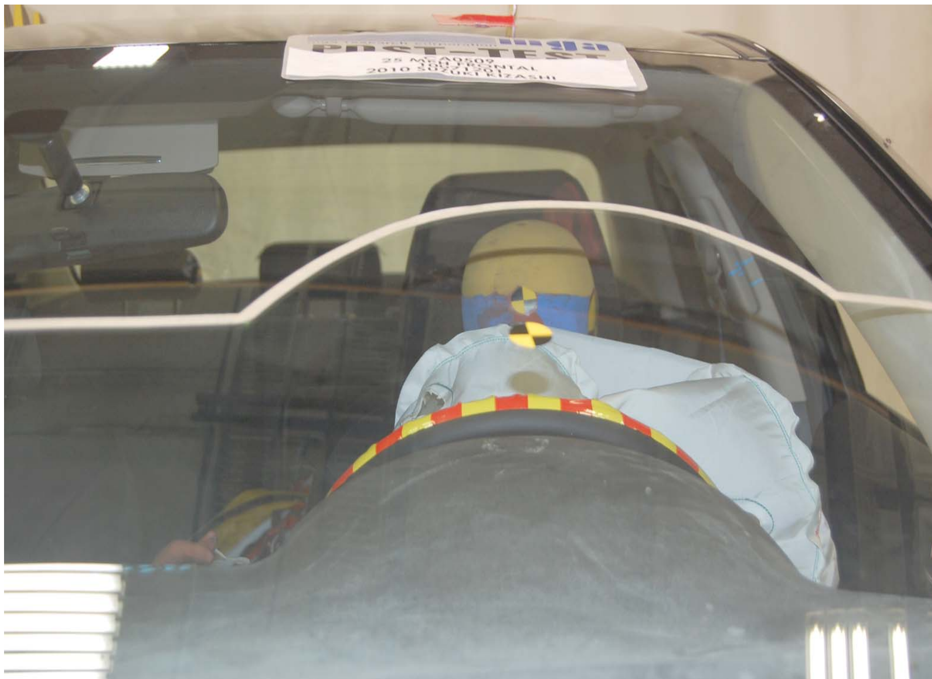
Post-Test Driver Dummy Front View (head position)
