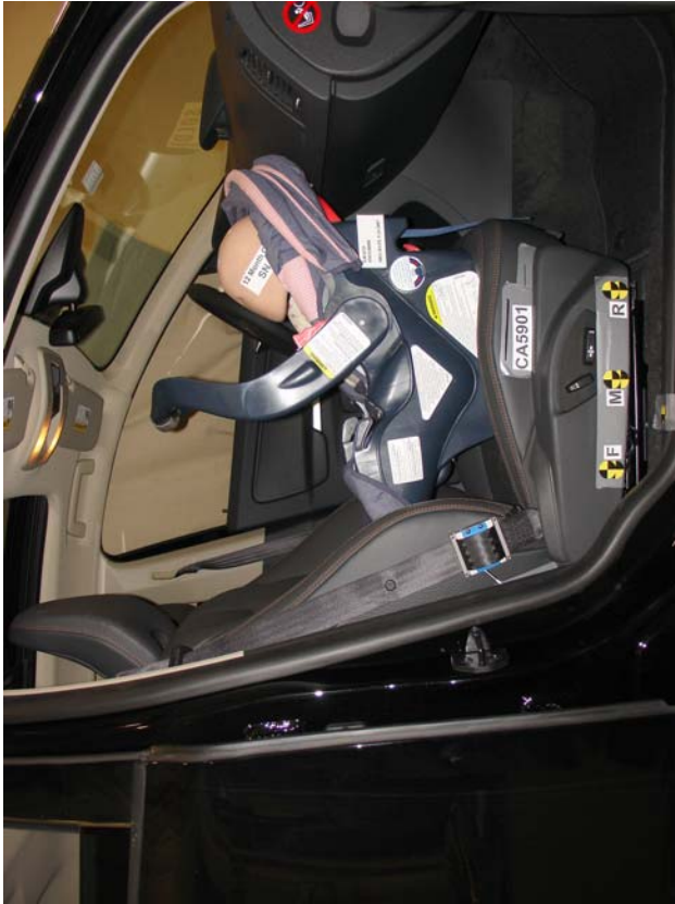
Graco Snugg Ride WOut Base, Unbelted, Rear Facing, Forward Seat Track
