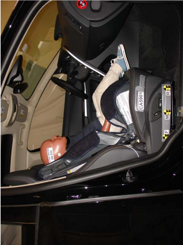
3-Year-Old Forward Facing Cosco High Back Booster Cinched With Harness, Middle Seat Track
