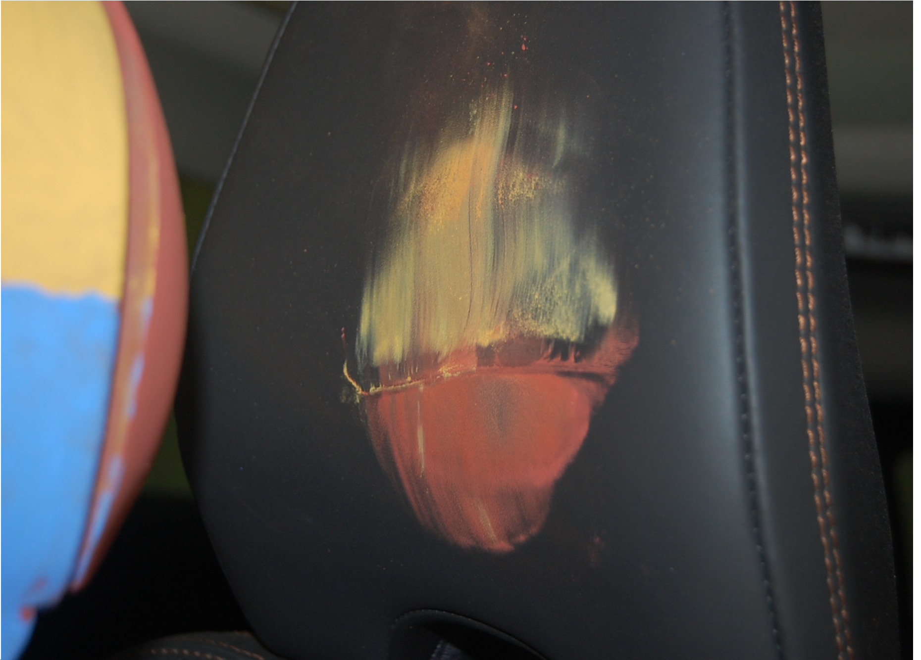
Post-Test Driver Dummy Head Contact (headrest)
