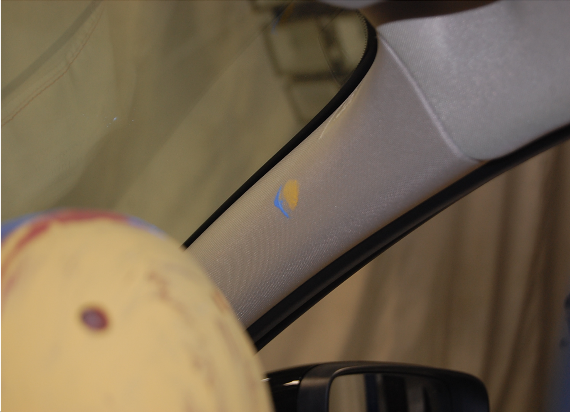
Post-Test Passenger Dummy Head Contact (C-pillar)
