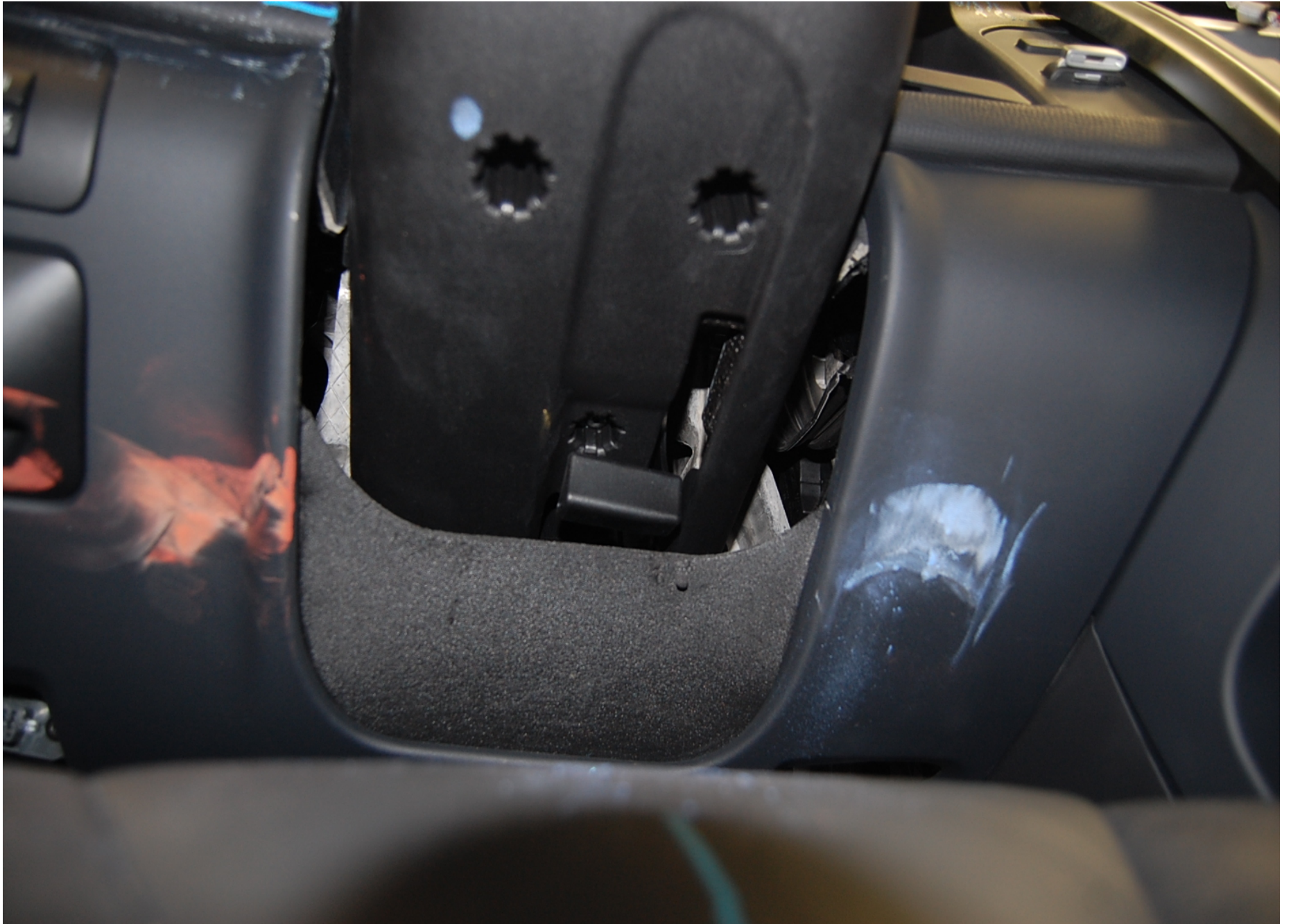
Post-Test Driver Dummy Knee Contact
