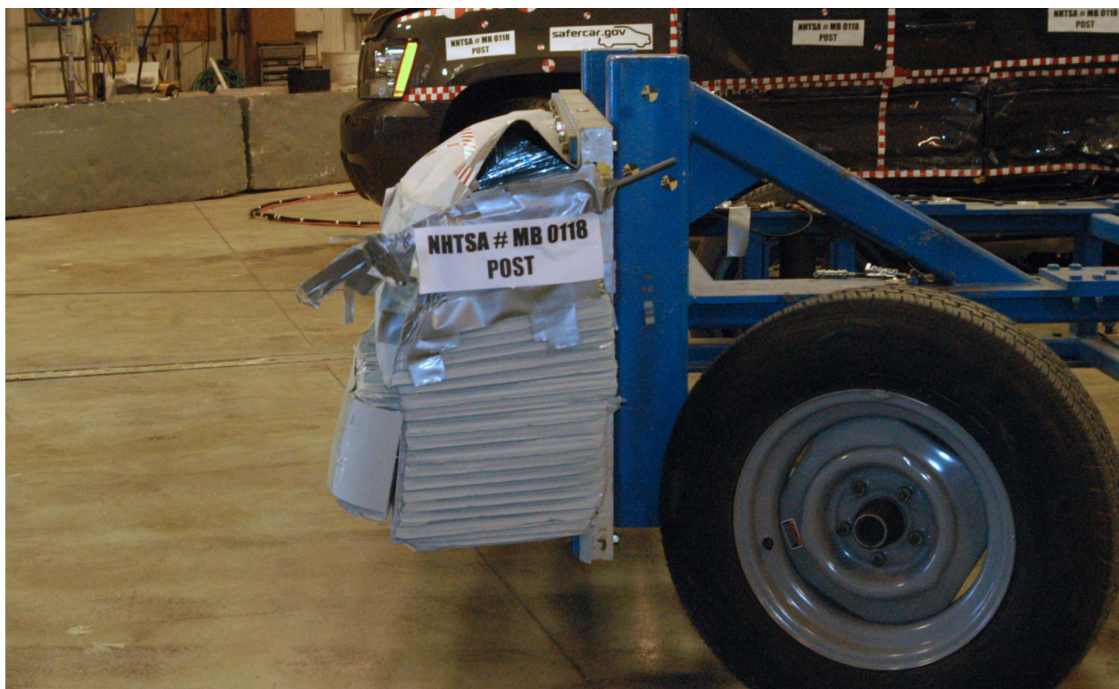
Figure A-86: Post-Test Left Side View of MDB Impactor Face
