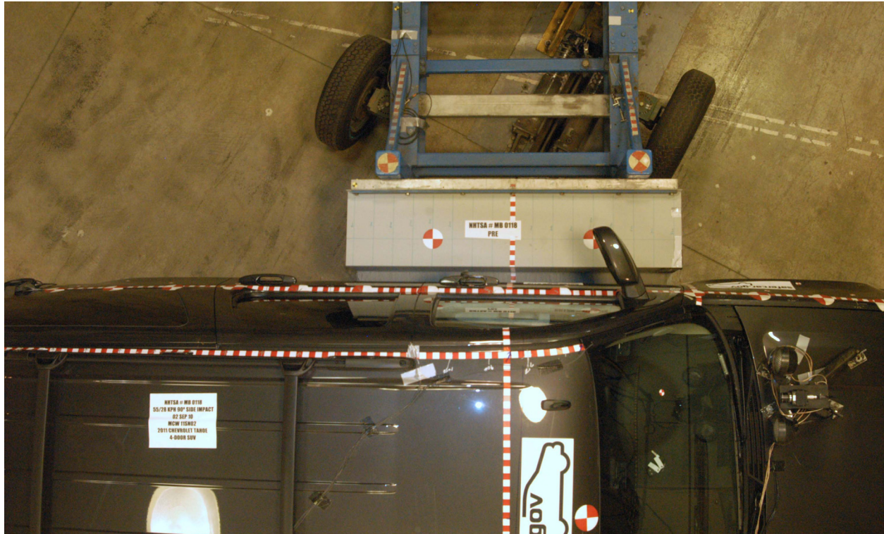
Figure A-15: Pre-Test Overhead View of Test Vehicle with MDB Positioned Against Side of Target Vehicle
