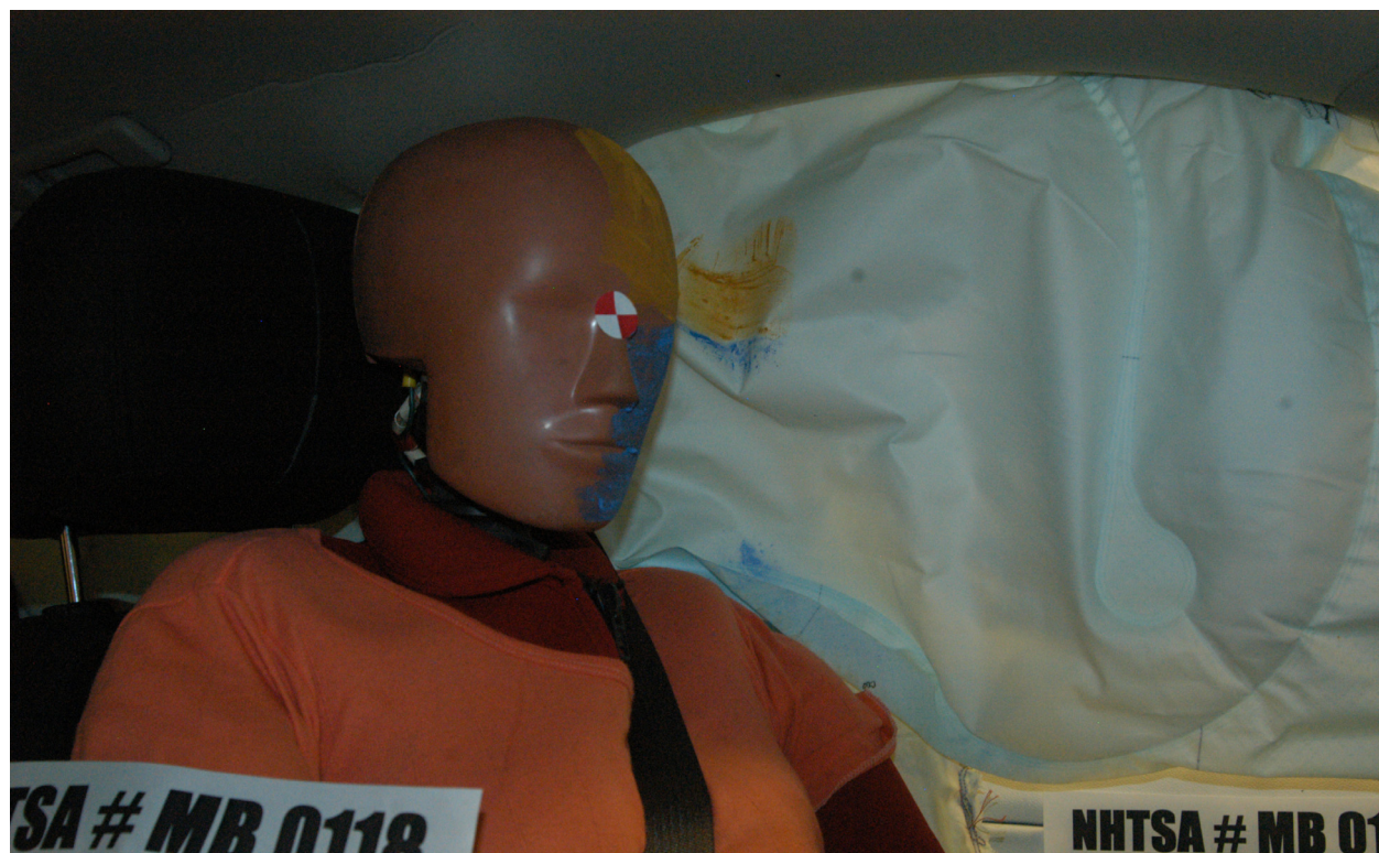
Figure A-48: Post-Test Driver Dummy Close-Up Head Contact with Side Air Bag View
