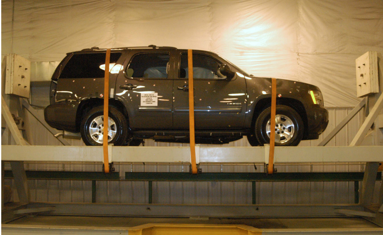
Figure A-97: FMVSS No. 301/305 Rollover 360°
