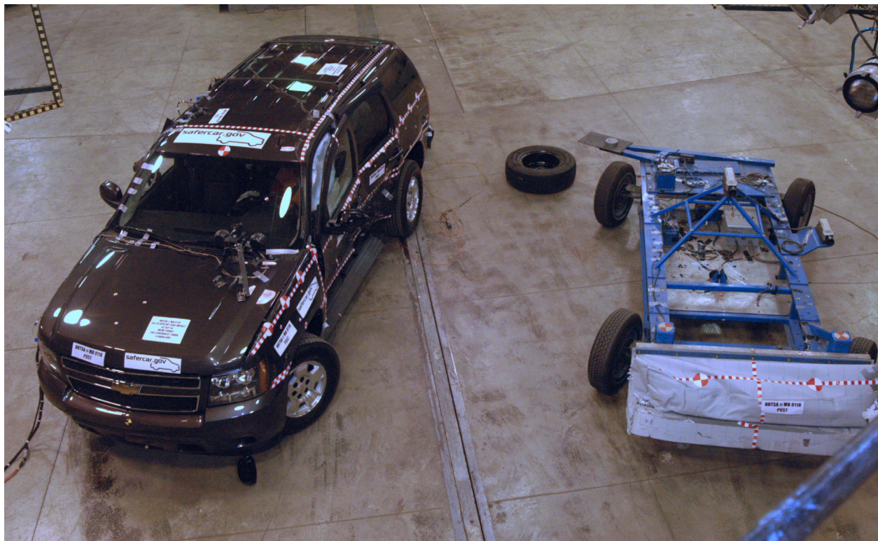
Figure A-16: Post-Test Overhead View of Test Vehicle and MDB
