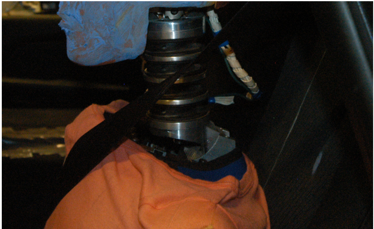
Figure A-60: Pre-Test View of Rear Passenger Dummy's Neck Showing Position of Adjustable Neck Bracket
