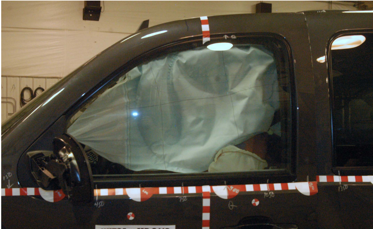
Figure A-29: Pos-Test Left Side View of Driver Dummy Shoulder and Door Top View
