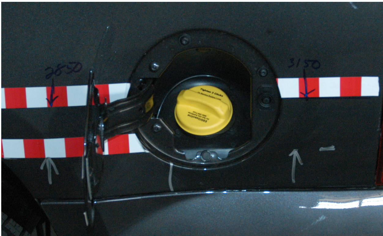
Figure A-80: Post-Test View of Fuel Filler Cap
