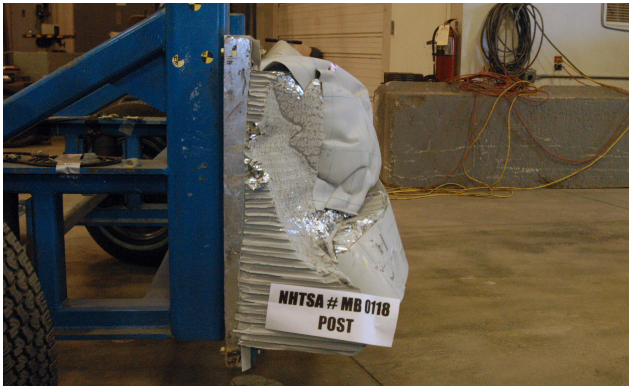
Figure A-88: Post-Test Right Side View of MDB Impactor Face
