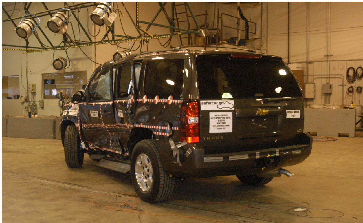
Figure A-10: Post-test Left Rear Three-Quarter View of Impact Zone
