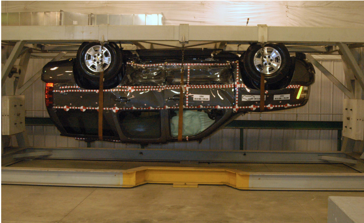
Figure A-95: FMVSS No. 301/305 Rollover 180°
