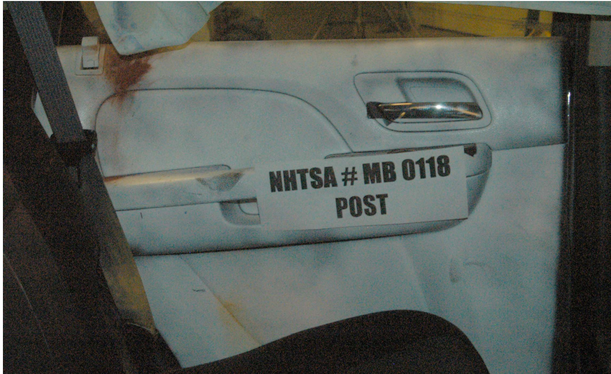
Figure A-75: Post-Test Rear Passenger Dummy Close-Up Torso Contact with Vehicle View
