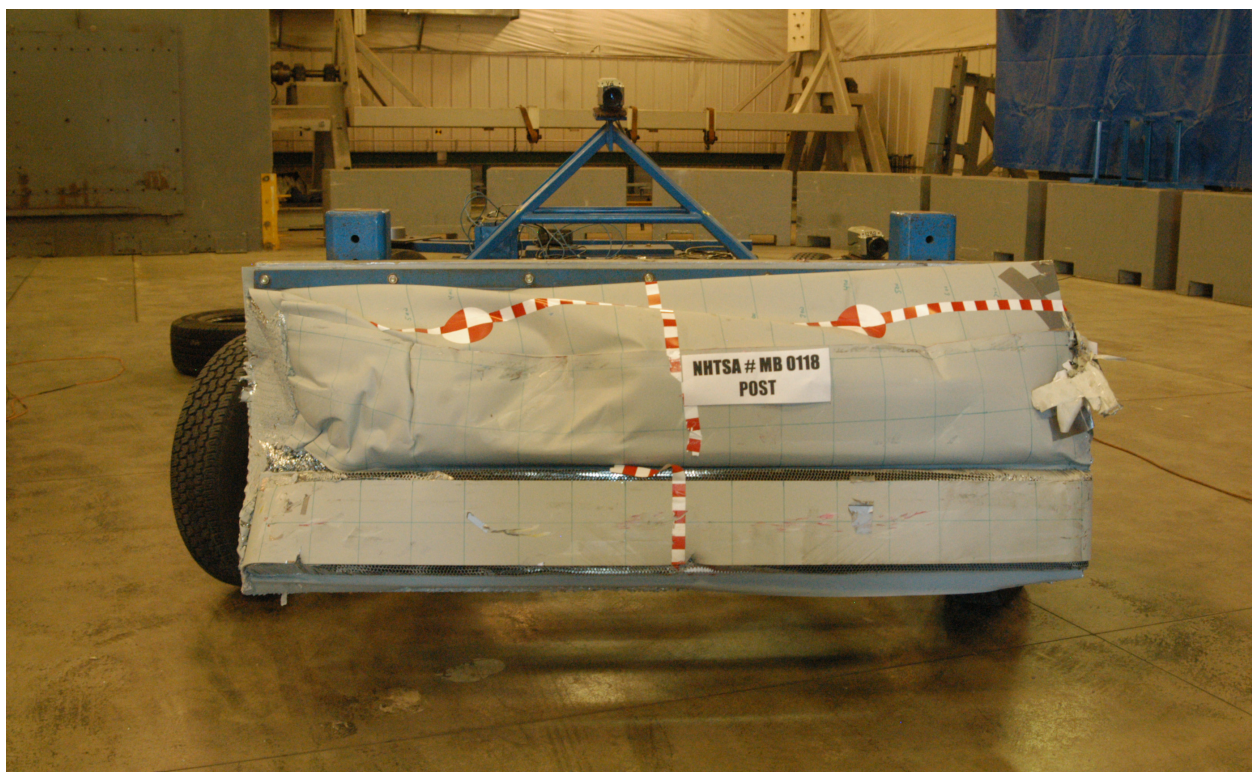
Figure A-82: Post-Test Front View of MDB Impactor Face
